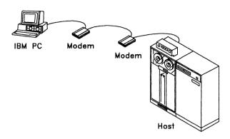
By using the IBM PC 3270 Emulation Program along with the associated hardware, you can establish a communications link with a **host computer**. The host computer, sometimes referred to as a *host processor*, or *mainframe*, usually provides services such as computation, data base access, and advanced programming functions.
