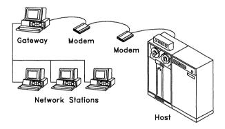
Because it serves as a communications link between the Network Stations and a host computer, a Gateway is sometimes referred to as a *communications server*. Software and hardware requirements include:
