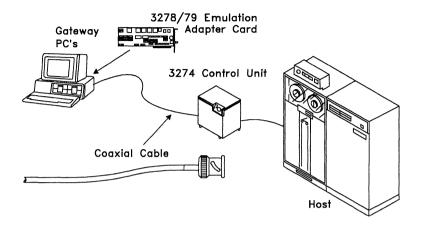
A coaxial cable is required to connect the IBM PC containing the adapter to the control unit. The control unit in turn is connected to a host computer. This type of attachment is diagrammed above.
