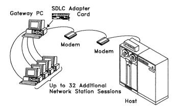
There are two different ways to attach to the host computer using the SDLC Adapter: the physical communication line can be either dedicated or switched.
