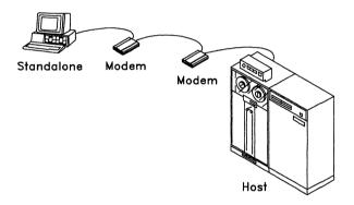
A Standalone IBM PC that is attached to a host computer using an SDLC Adapter is illustrated above. (IBM PCs that are attached by way of an IBM 3278/79 Emulation Adapter do not use modems, but do need coaxial cables.)
