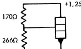
When the in-phase clamp is used  $R_3$  is replaced by network:
