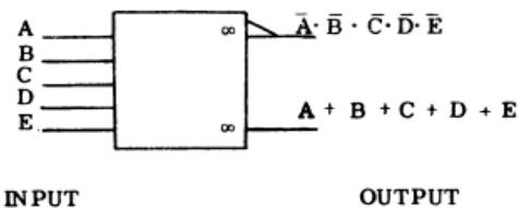
The block notation represents the basic current switch function and, unless otherwise noted within the block, is considered to perform the OR function. The presence of an infinity sign within the block implies no clamp circuit at the adjacent output.
