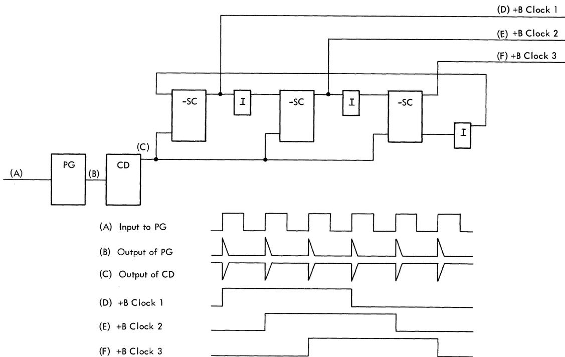
Figure 42. Shift Cell Clock Ring
