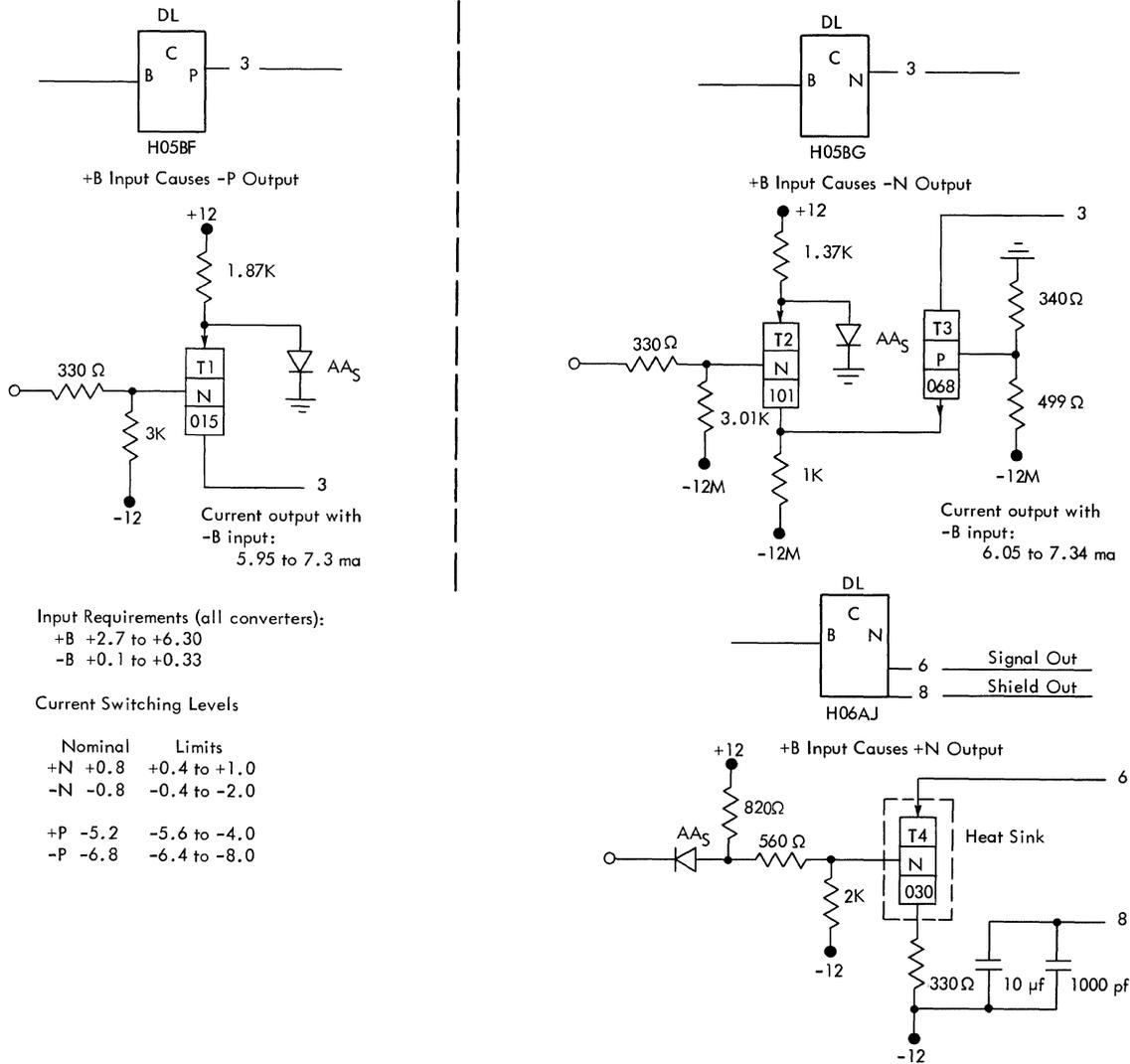
Figure 61. DDTL to Current Switching Converters
