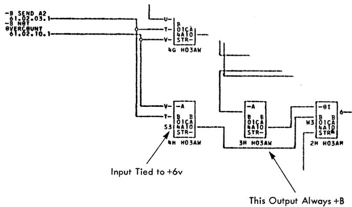
Figure 68. Unused Twin Card Circuits
