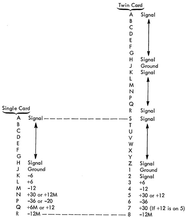
Figure 66. Single and Twin Card Voltage Assignments
