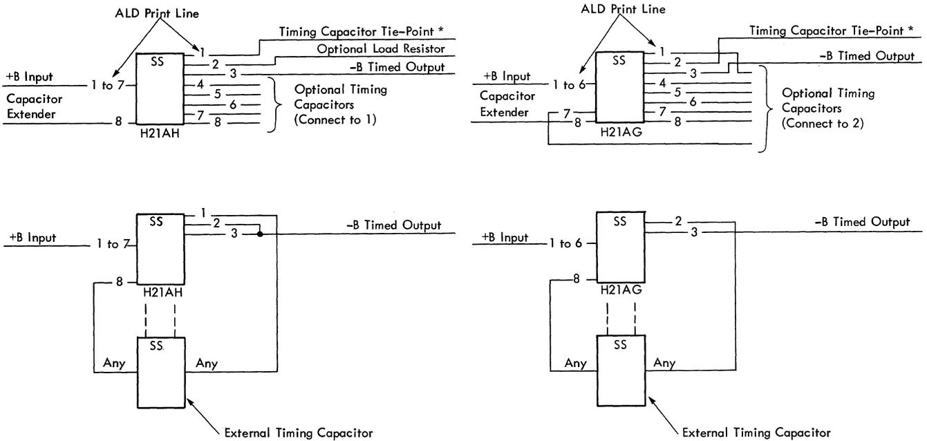
\* No internal capacitor is wired; the capacitor tie-point must be wired to a capacitor
