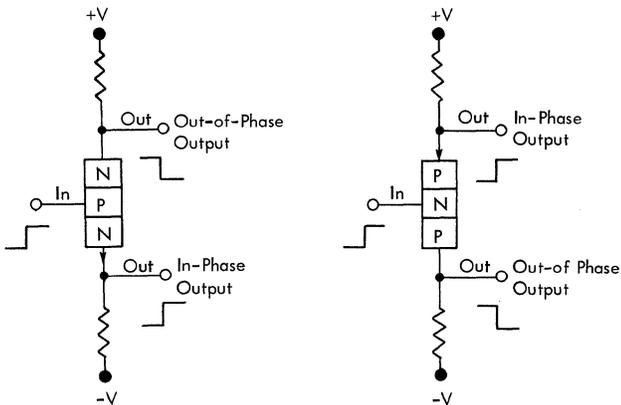
Figure 3. Split-Load Configuration
