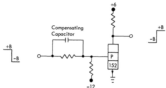
Figure 20. Logical Low Power Inverter
