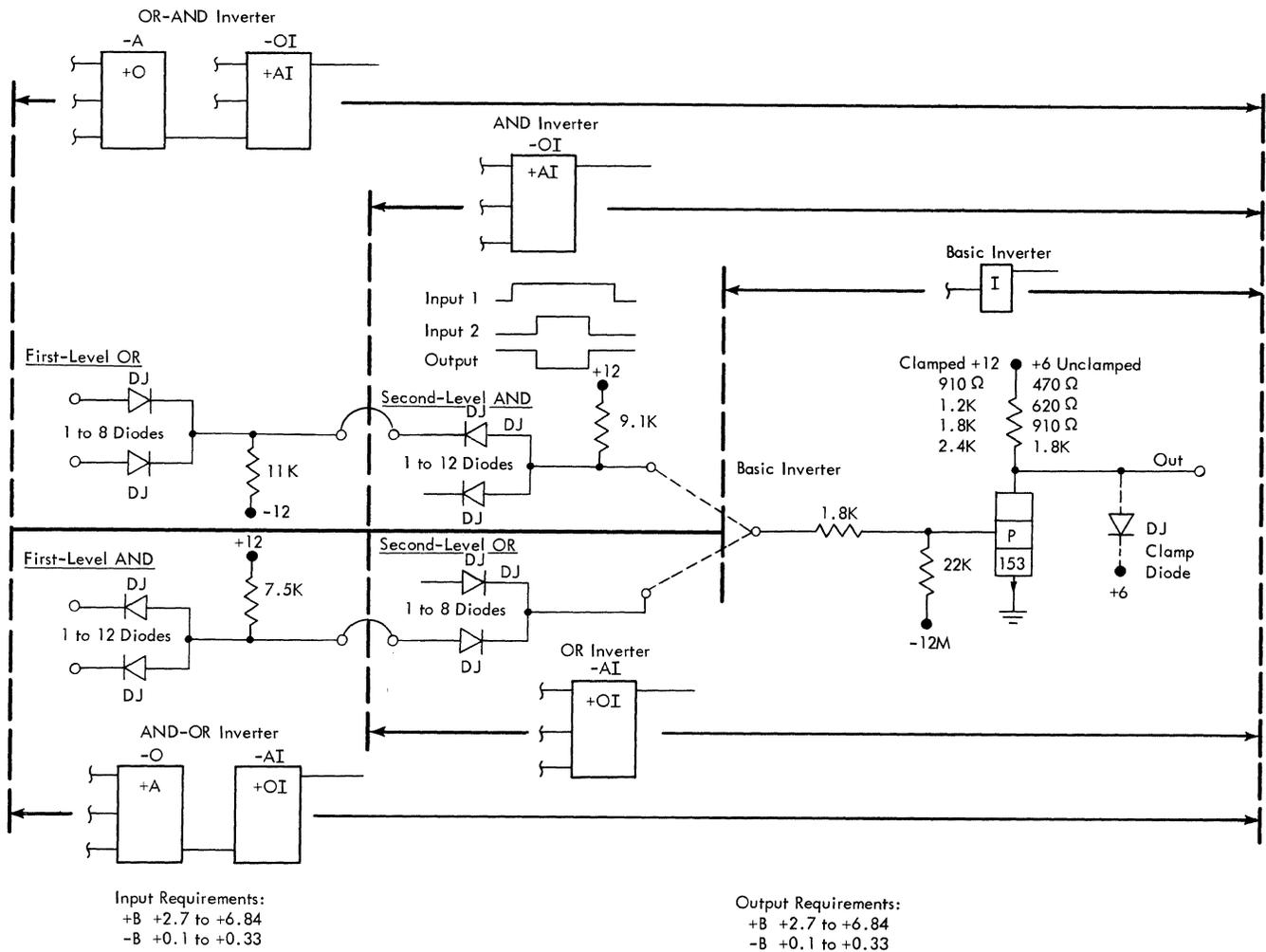
Figure 28. Basic Inverter with Diode Logic
