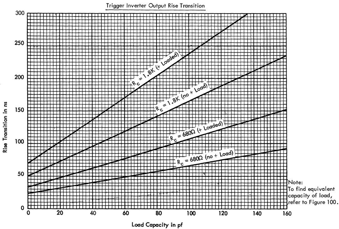
Figure 105. Binary Trigger Delays and Output Transitions
