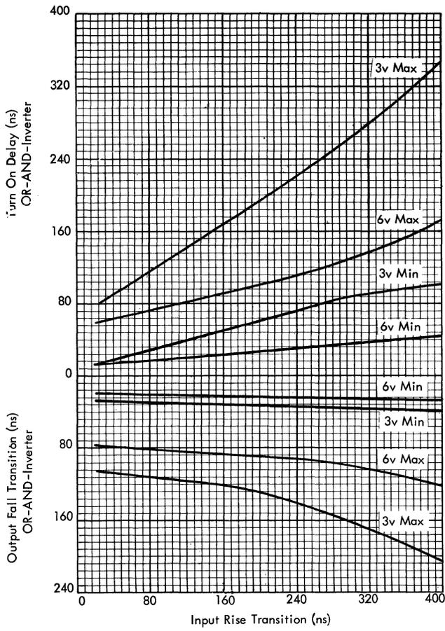
Figure 86. Turn-On Delay and Fall Transition of OR-AND Inverter
