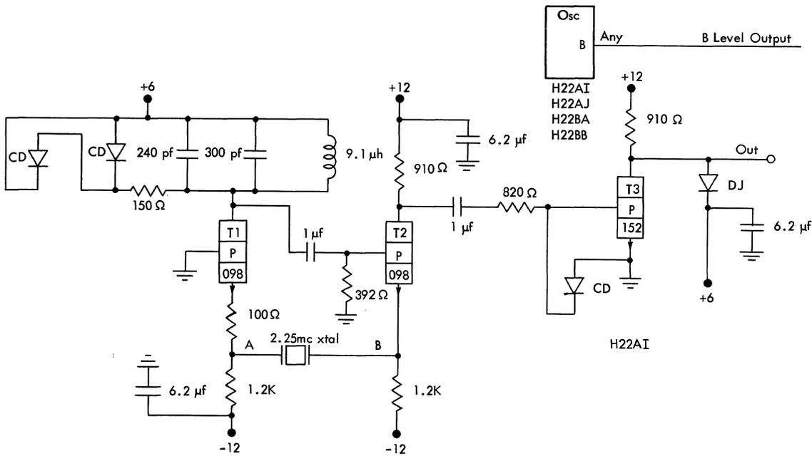
Figure 54. Crystal-Controlled Oscillator, Example 2
