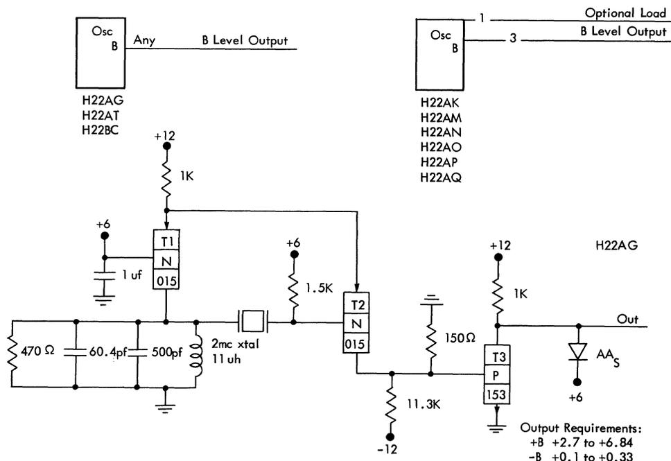
Figure 53. Crystal-Controlled Oscillator, Example 1
