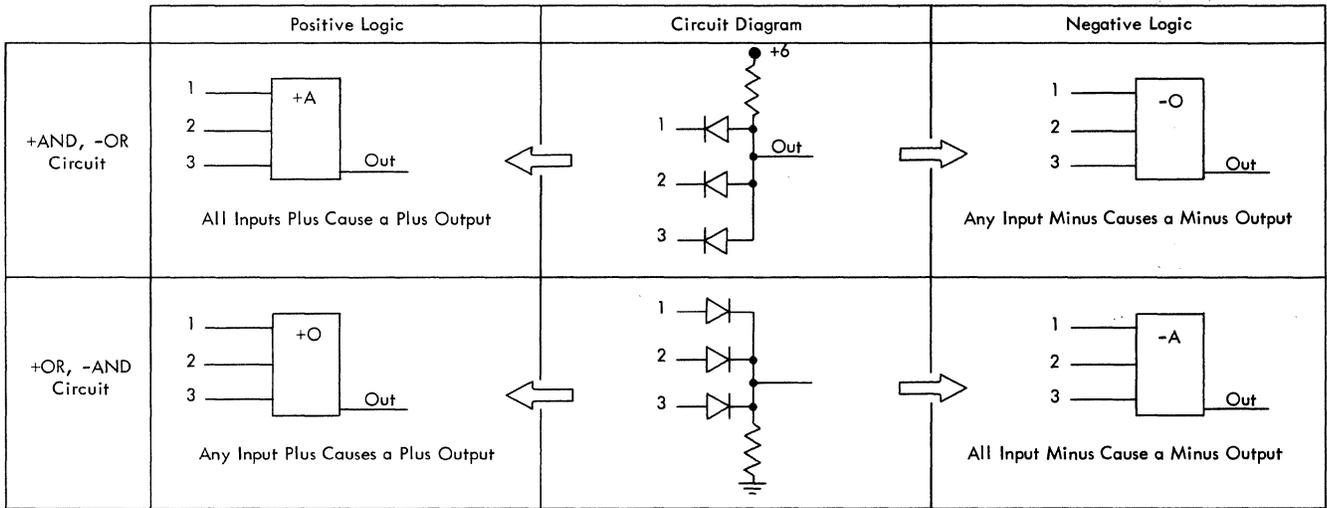
Figure 7. Positive and Negative Logic
