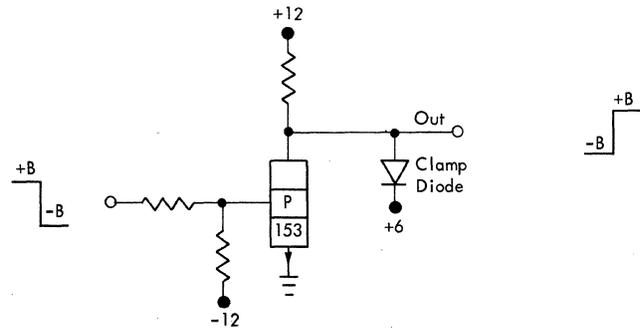
Figure 17. Basic Inverter with Clamped Output
