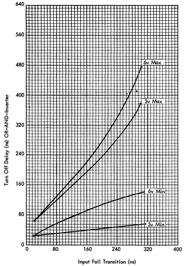
Figure 91. Turn-Off Delay of OR-AND Inverter
