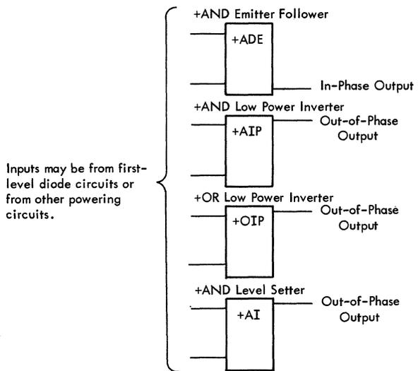
Figure 13. Combination Diode and Powering Circuit Examples
