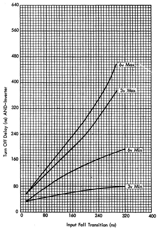
Figure 89. Turn-Off Delay of AND Inverter
