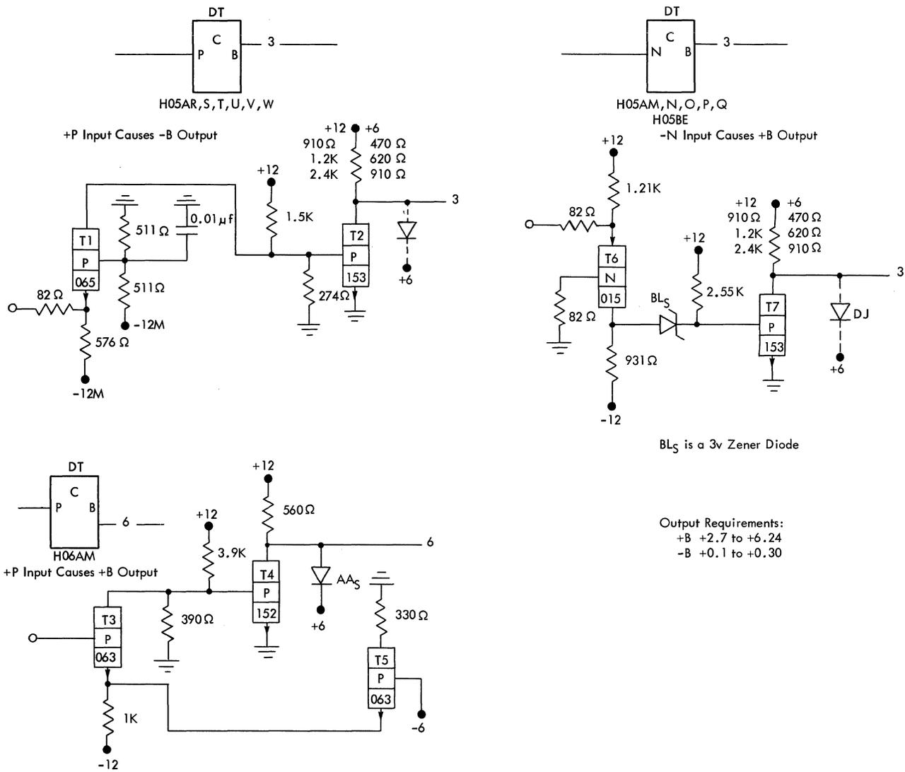
Figure 62. Current Switching to DDTL Converters
