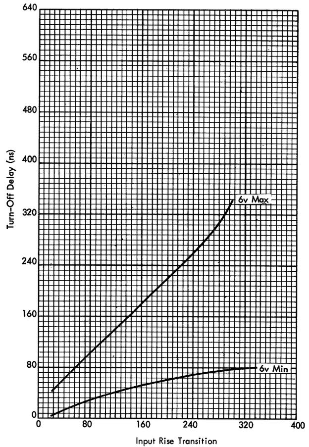
Figure 99. Turn-Off Delay of AND LLPI
