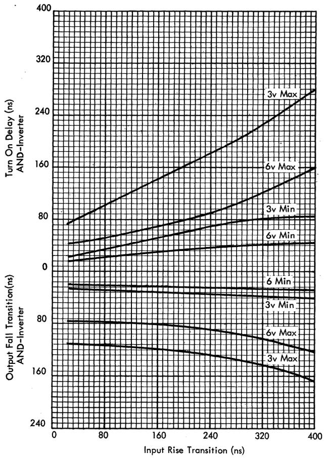
Figure 84. Turn-On Delay and Fall Transition of AND Inverter
