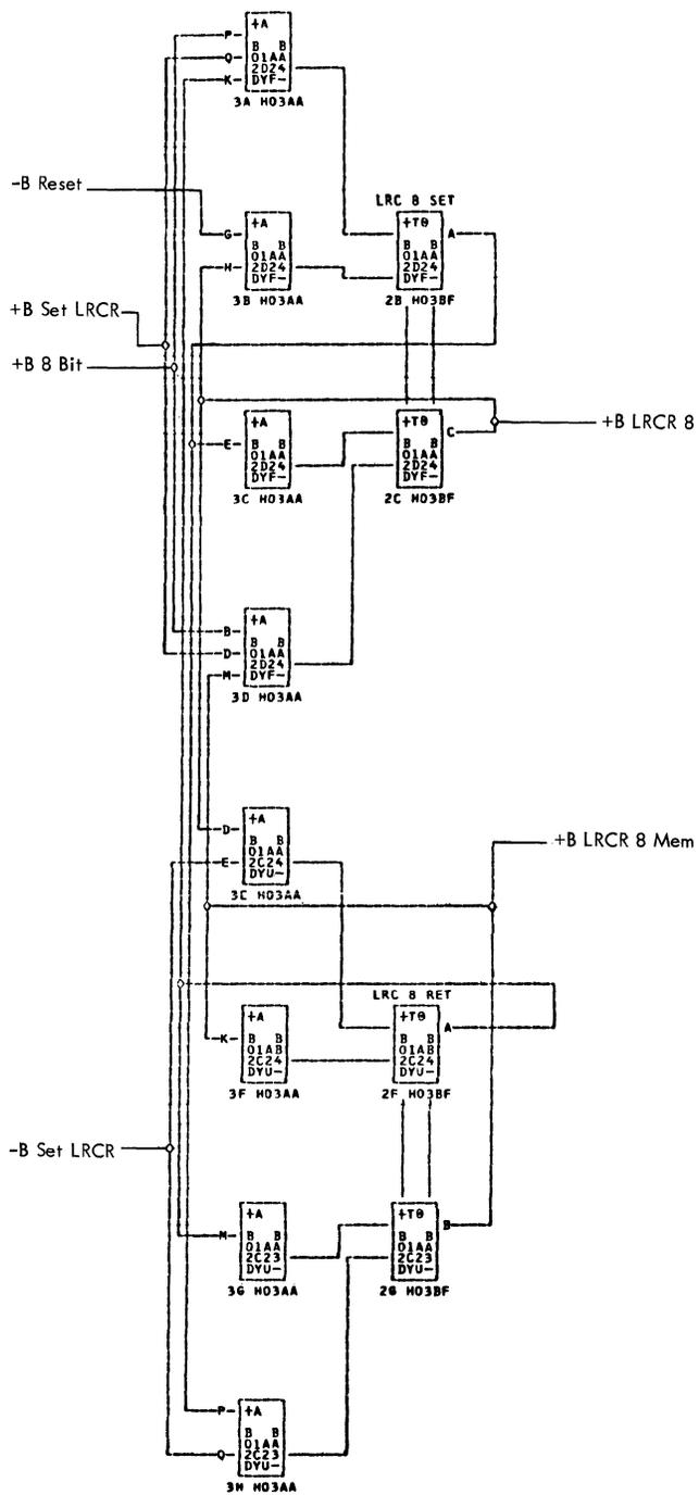
Figure 75. Latch Configuration for Binary Operation
