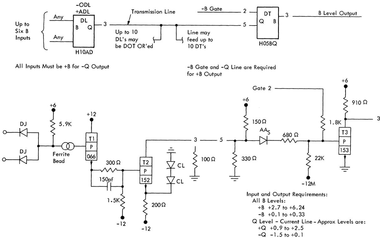
Figure 56. Line Driver and Line Terminator
