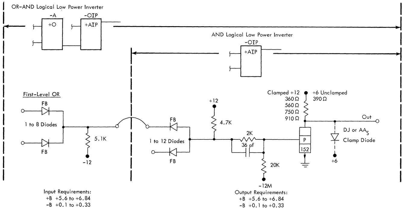
Figure 30. AND Logical Low Power Inverter
