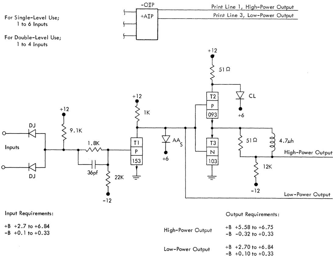
Figure 34. Powered Inverter
