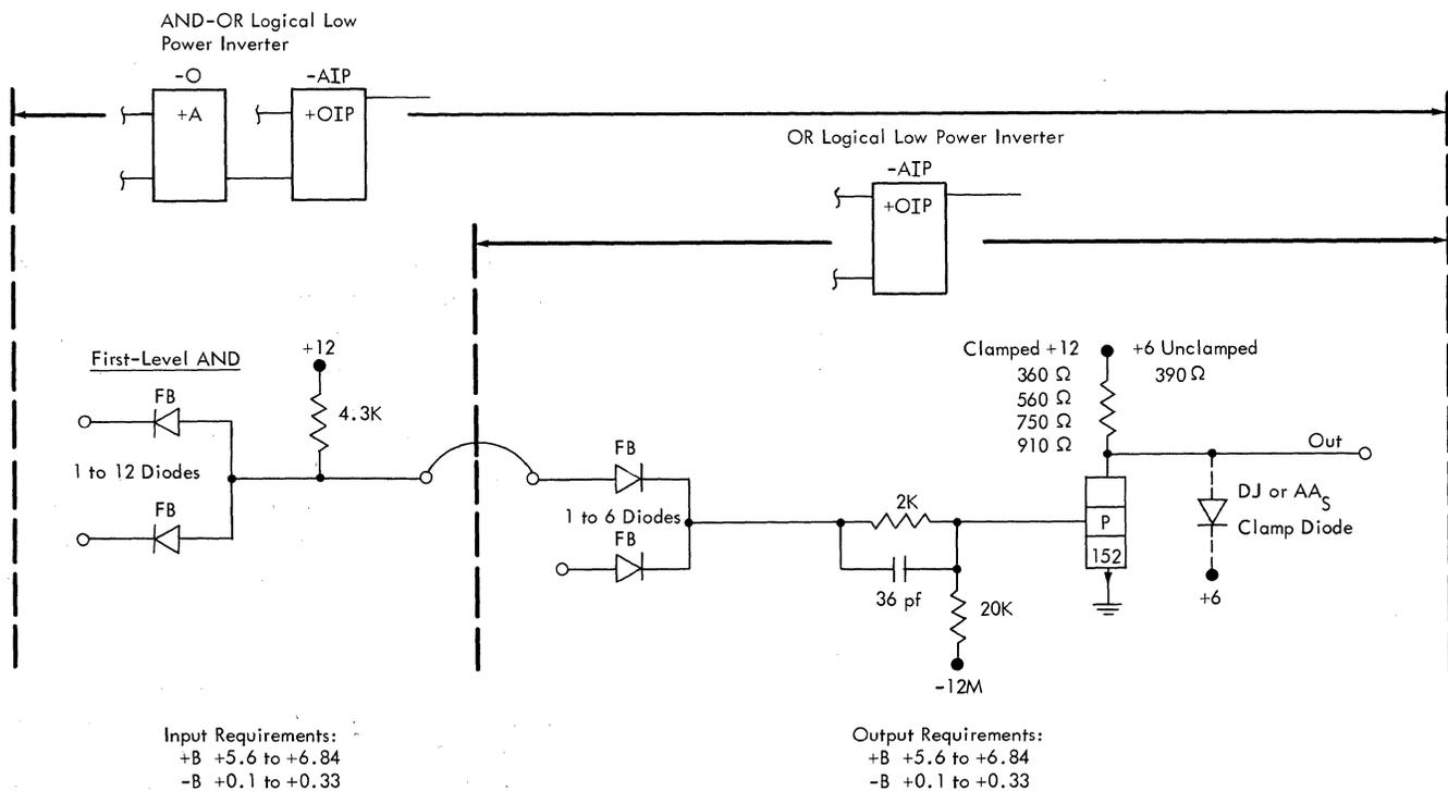
Figure 29. OR Logical Low Power Inverter
