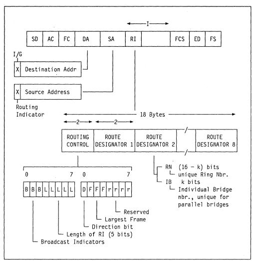
Figure 16. Token Passing Ring Frame - Routing Information Field
