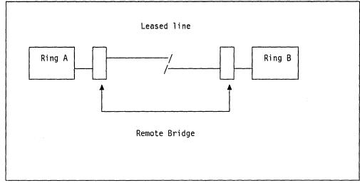
Figure 26. Remote Bridge Scheme
