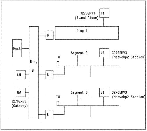
Figure 44. Mixed LAN with a Token-Ring Backbone and PC Network segments. TU stands for translator unit
