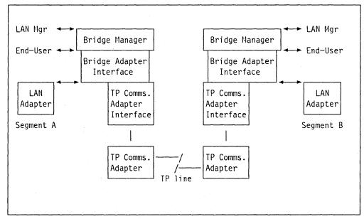
Figure 13. Remote Bridge Structure
