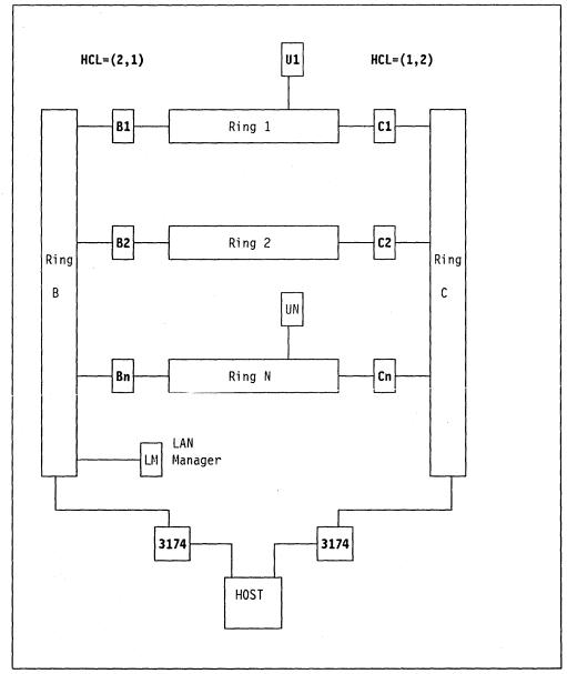
Figure 50. Host Connection via Two 3174/01L
