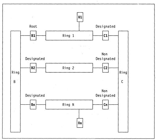
Figure 19. Single-Route Broadcast in a Dual Backbone Configuration
