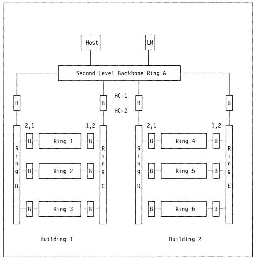
Figure 54. Three level Hierarchy with No Inter Building Connectivity
