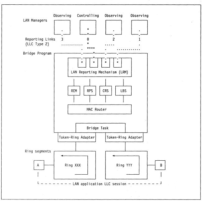
Figure 14. IBM Token-Ring Network Bridge Program V2.0 - IBM LAN Manager V2.0 Communication
