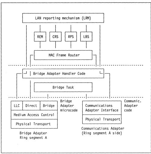
Figure 29. IBM Token-Ring Network Bridge Program V2.1 - General Bridge Structure
