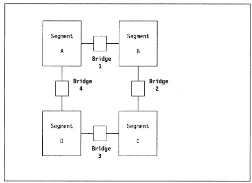
Figure 9. Loop Configuration with Four LAN Segments
