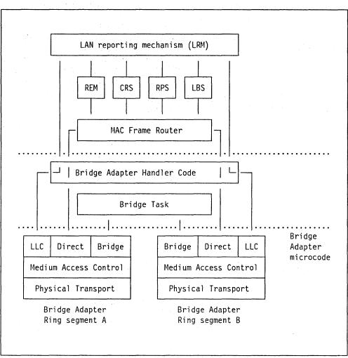
Figure 24. IBM Token-Ring Network Bridge Program V2.0 - General Bridge Structure
