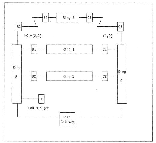
Figure 56. Parallel Remote Bridges Configuration
