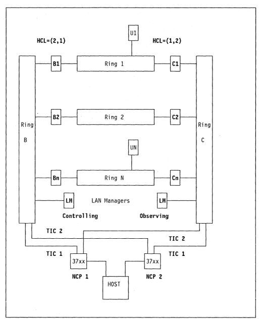
Figure 48. Host Connection via Two 37xx and Four TICs.
