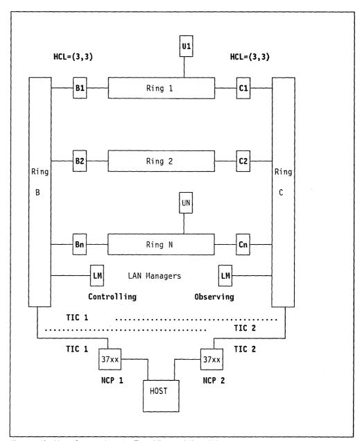
Figure 49. Host Connection via Two 37xx and Two TICs.
