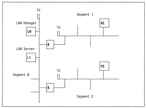
Figure 43. LAN with Multiple PC Network (Broadband) Segments. TU stands for Translator Unit. B states for PC Network Bridge
