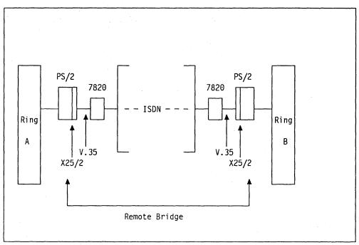
Figure 28. Remote Bridge Function across an ISDN network
