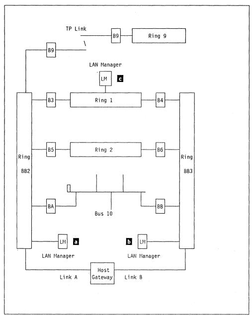
Figure 64. LAN Manager Configuration and Placement
