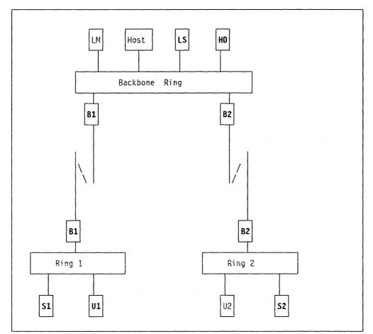
Figure 33. Remote Bridge Configuration
