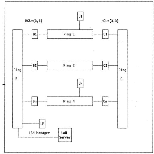
Figure 51. LAN Server Attached to a Single Backbone
