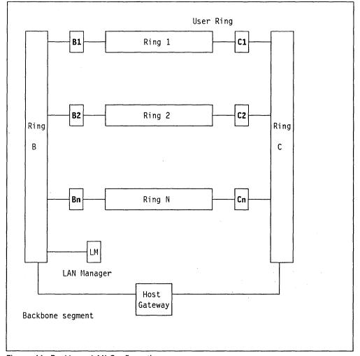
Figure 11. Backbone LAN Configuration
