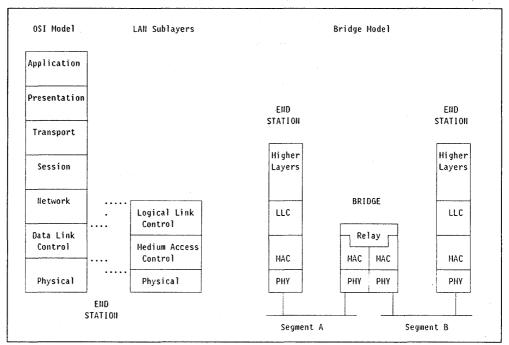
Figure 7. Model for a Bridge. Relationship between the OSI seven layer model, LAN sublayers and a model for a bridge
