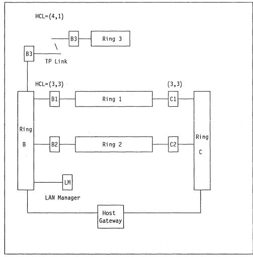
Figure 55. Remote Bridge Configuration
