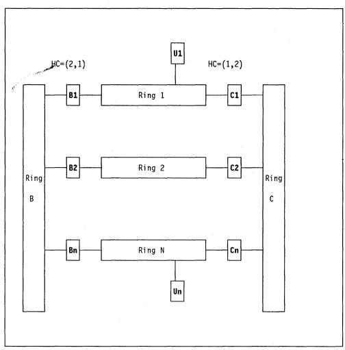
Figure 23. Dual Backbone Configuration and Hop Count Limits
