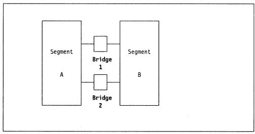
Figure 10. Parallel Configuration
