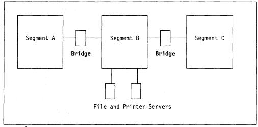
Figure 8. Serial LAN Configuration. Segment A and segment C are two separate departments with little inter-communication. They share servers attached to segment B.
