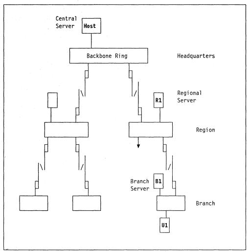
Figure 36. Example of a Cascaded Bridges Configuration
