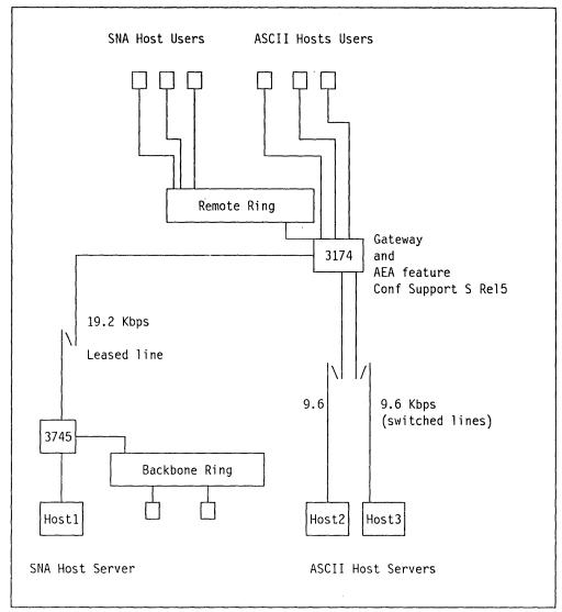
Figure 32. SNA and ASCII Traffic via 3174 LAN Gateway
