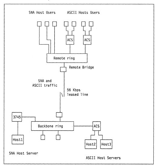
An example of a new configuration using a remote bridge with a single 56Kbps leased line is shown in Figure 31.
