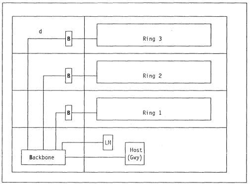
Figure 58. Distributed Bridges and Central Backbone Topology
