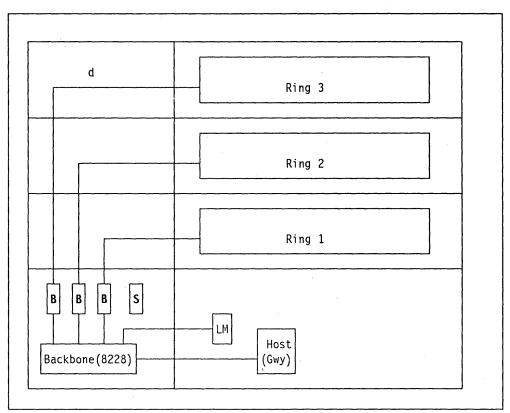
Figure 57. Centralized Bridges and Central Backbone Topology
