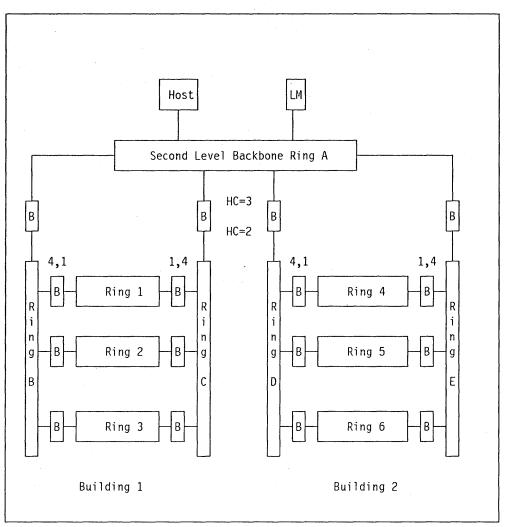
Figure 53. Three-level Hierarchy with Any-to-Any Connectivity
