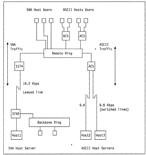
Figure 30. SNA and ASCII Traffic on Separate Links
