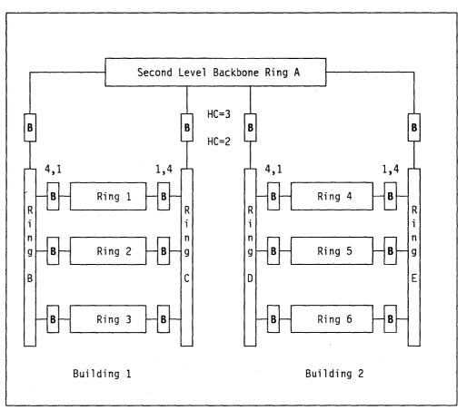
Figure 22. Hop Count Assignment for a Hierarchical Configuration. B are bridges and HC stands for hop count.
