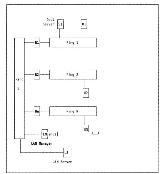
Figure 46. Simple Backbone Configuration
