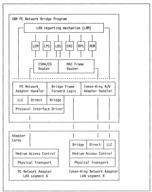
Figure 41. IBM PC Network Bridge Program - General Bridge Structure
