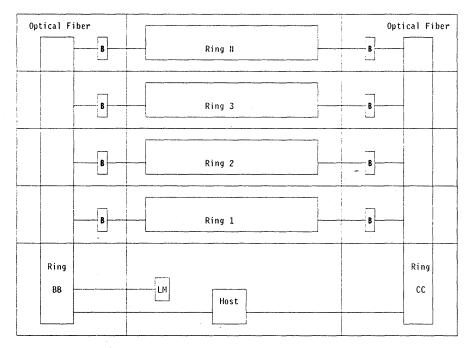
Figure 60. Distributed Dual Backbone Topology (High Building Environment)
