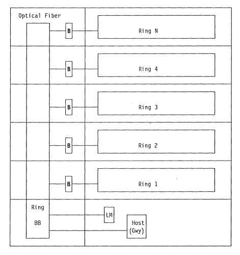
Figure 59. Distributed Backbone Topology in a High Building Environment
