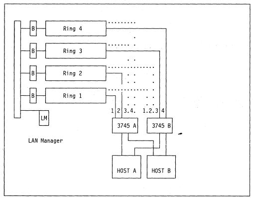
Figure 52. Host Connected User Rings. Solid lines indicate active TICs. Dotted lines are non-active backup TICs.
