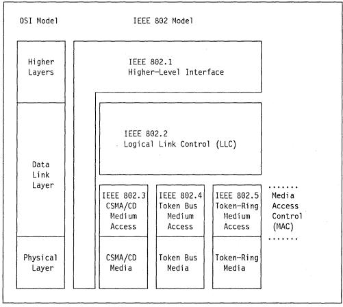
Figure 6. IEEE 802 Model Compared to the OSI Model
