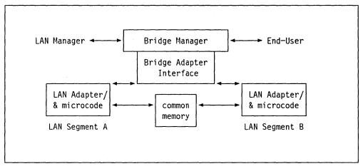
Figure 12. LAN Bridge Structure
