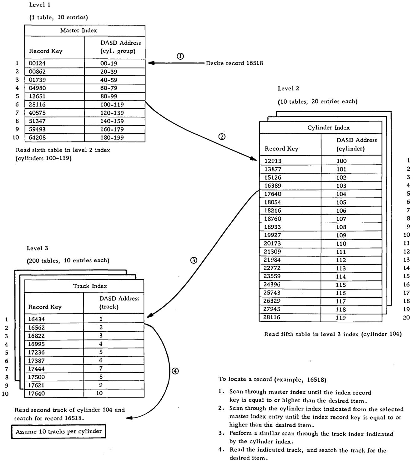
Figure 3. Generalized index system for DASD
