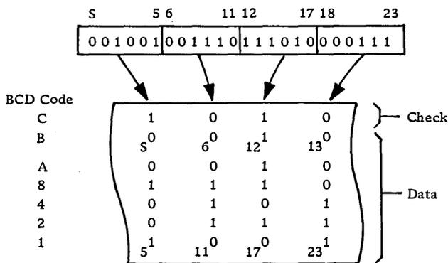
Figure 19. Magnetic tape — seven-track binary system
