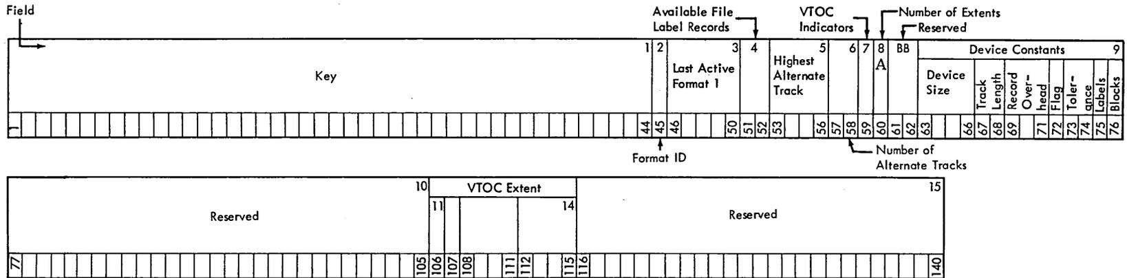
Format 4: This format is used to describe the Volume Table of Contents and is always the first file label in the VTOC. There must be one and only one of these Format 4 file labels per volume.
