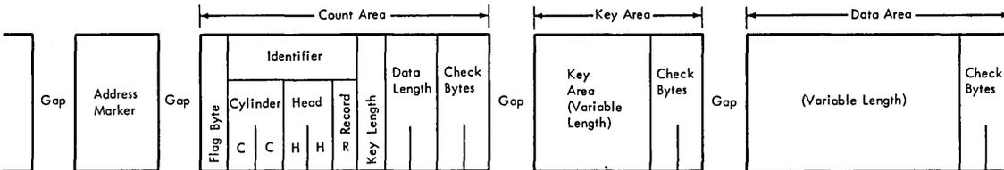
Schematic Representation of DASD Record with a Key Area
