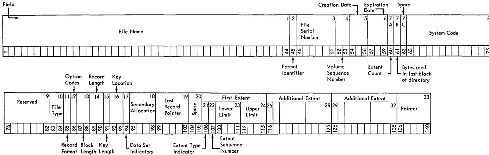
Format 1: This format is common to all data files on Direct Access Storage Devices.
