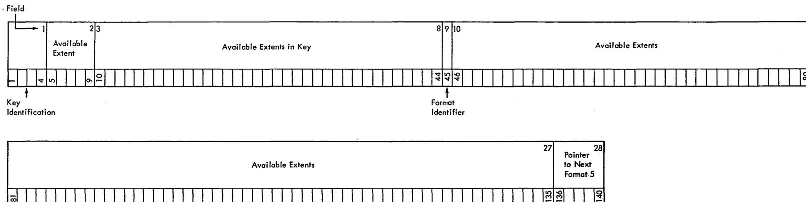
Format 5: This format is used for Direct Access Device Space Management (DADSM) only.
