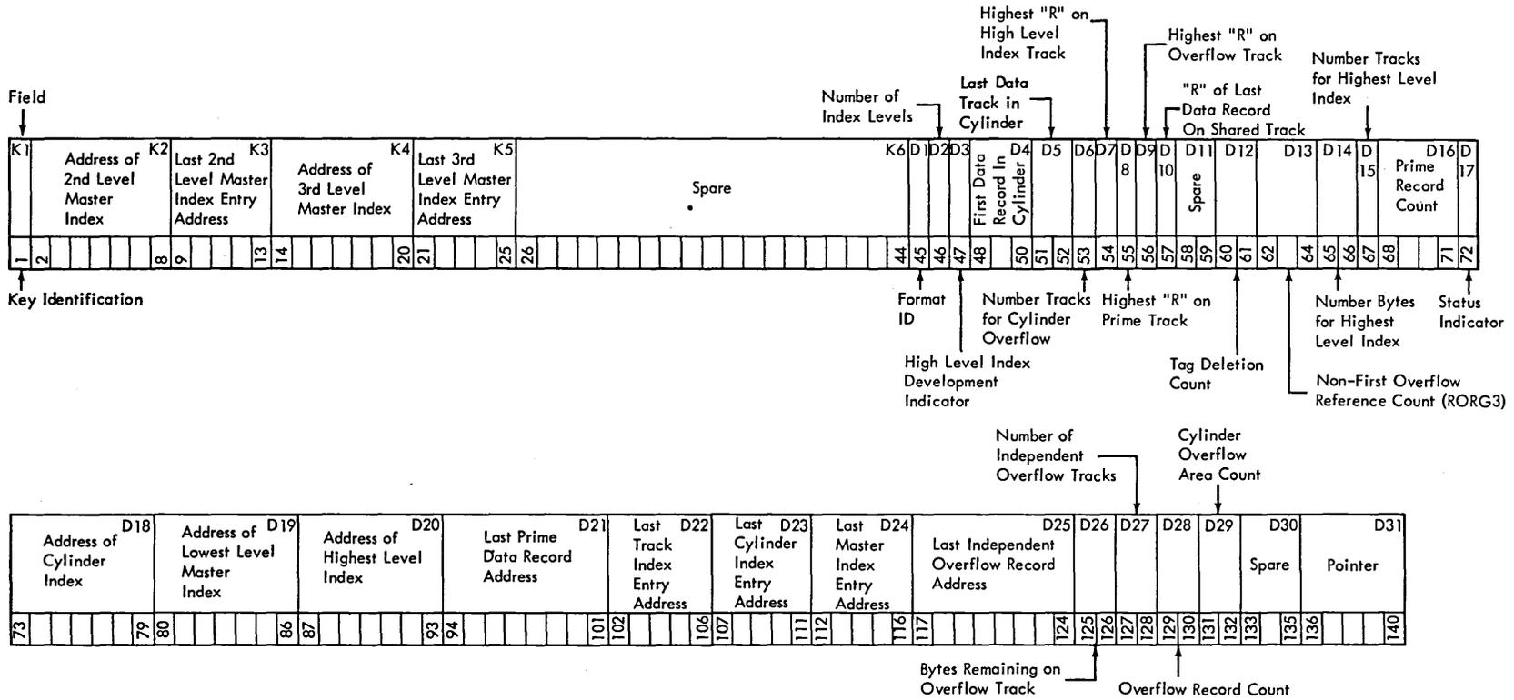
Format 2: This format is applicable only to Indexed Sequential data files. It is always pointed to by a Format 1 label.
