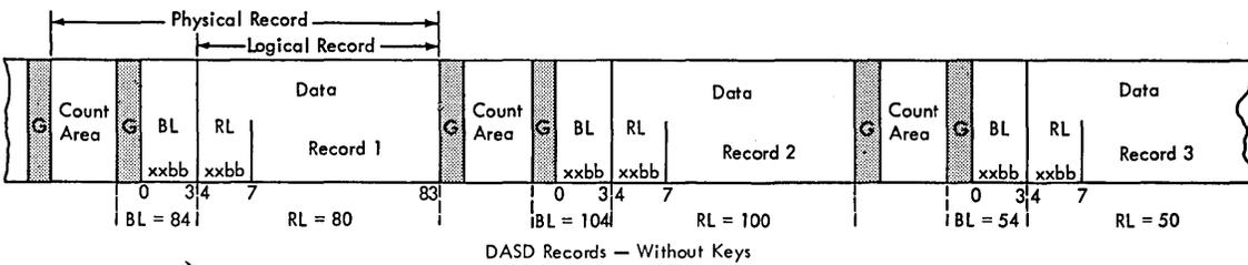
BL = Block Length } in binary half - word (16 bit) format, plus two blank bytes.
