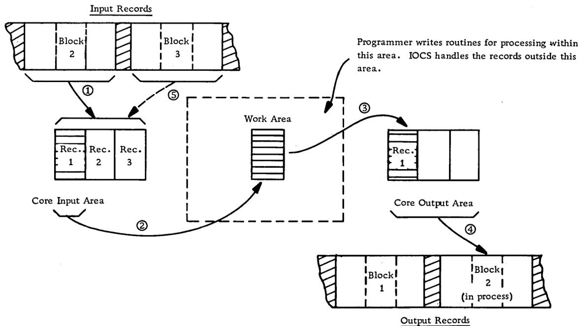
1. A data block is read into an input area in core storage.
