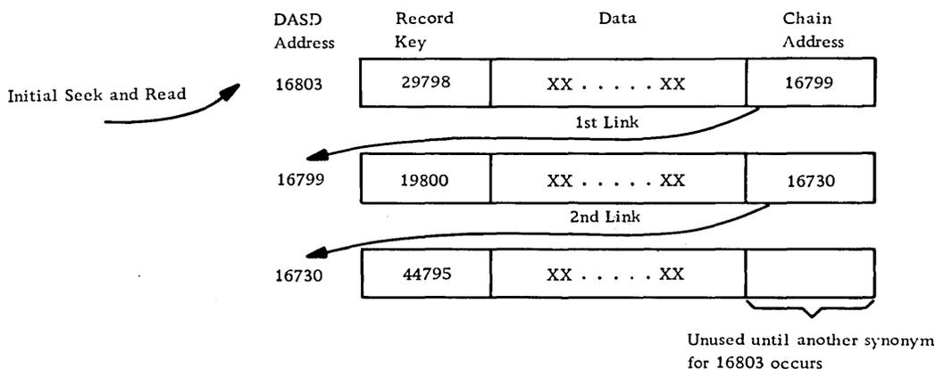
Figure 11. Example of chaining, unblocked records
