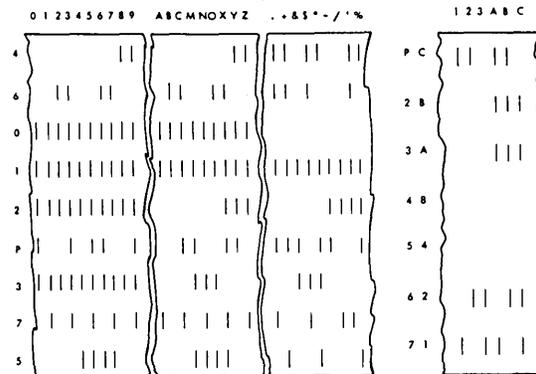
Figure 21. Nine-track and seven-track tape data format
