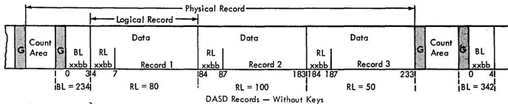
BL = Block Length } in binary half - word (16 bit) format, plus two blank bytes.
