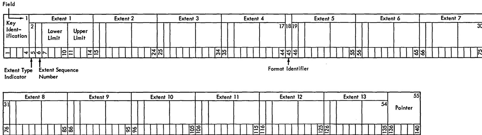
Format 3: This format is used to describe extra extent segments on the volume if there are more than can be described in the Format 1 (and Format 2 if it exists) file label. This file label is pointed to by a Format 1, Format 2, or another Format 3 file label.
