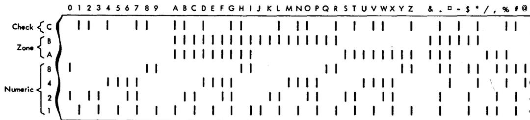
Figure 18. Magnetic tape — six-bit alphanumeric code
