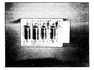
FIGURE 1-8. IBM MECURY-WETTED POLAR RELAY
