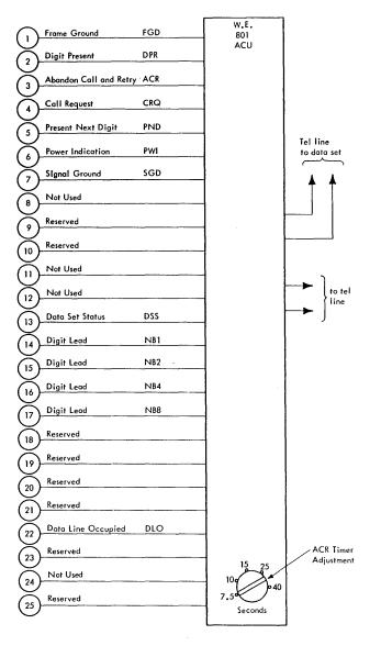
FIGURE 2-32. AUTOMATIC CALLING UNIT, WE 801A INTERFACE
