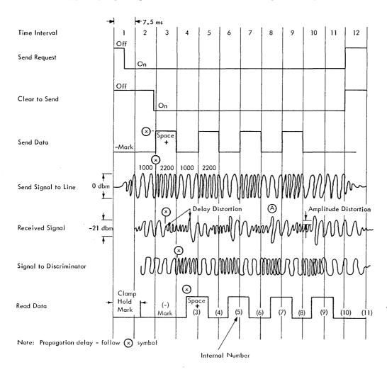
FIGURE 2-26. SIGNAL CORRELATION, IBM LINE ADAPTER
