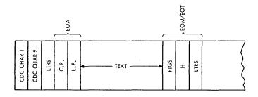
FIGURE 1-33. FORMAT OF TAPE MESSAGE, 83B2 SYSTEM
