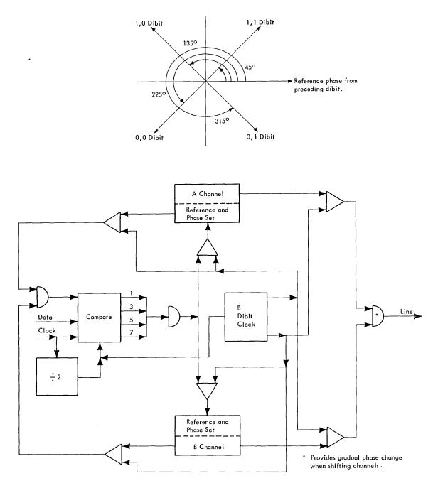
FIGURE 3-1. FOUR PHASE DATA SET - TRANSMIT CONCEPT
