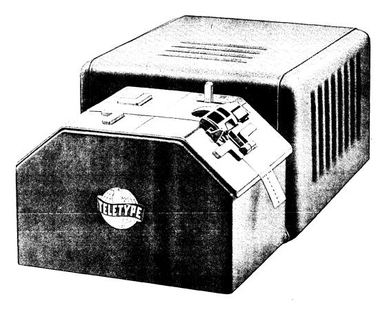
FIGURE 1-23. TRANSMITTER DISTRIBUTOR (TD)
