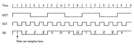
FIGURE 3-4. RELATION OF DCT, SCT, AND SD
