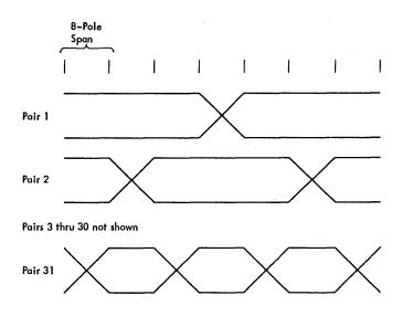
FIGURE 2-19. LINE TRANSPOSITION
