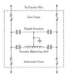
FIGURE 1-14. TELEGRAPH LINE ARRESTOR
