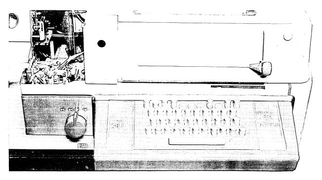
FIGURE 1-22. KEYBOARD TYPING REPERFORATOR (KTR)
