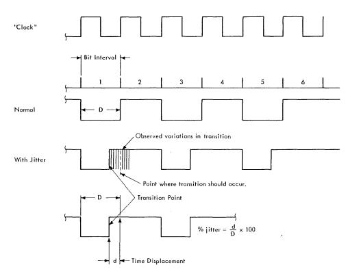
FIGURE 2-34. JITTER MEASUREMENT
