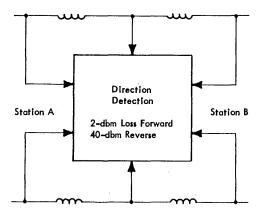
FIGURE 2-18. PRINCIPLE OF ECHO SUPPRESSION
