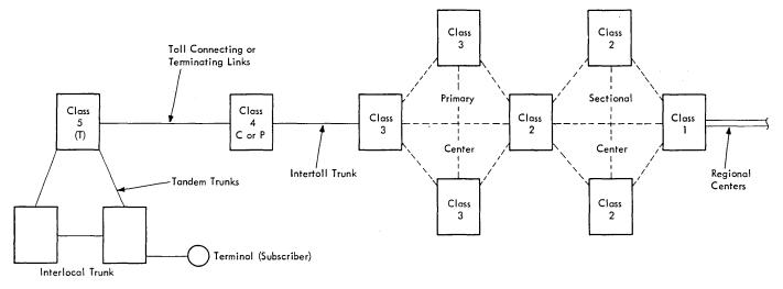
Class 4 (Center) handles inward, outward, and thru traffic. Class 4 (Point) handles outward and thru traffic. Class 1, 2, and 3 are control switching points (csp).
