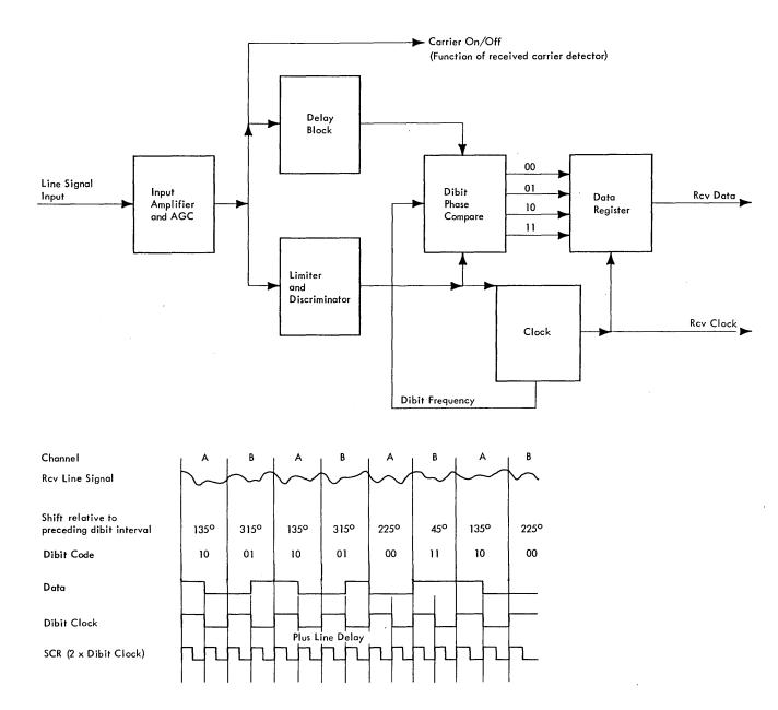
FIGURE 3-2. FOUR PHASE DATA SET - RECEIVE CONCEPT AND TIMING
