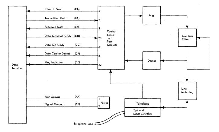
FIGURE 2-28. WE 103A DATA SET, BLOCK DIAGRAM
