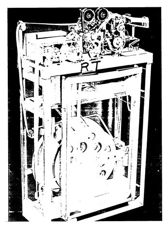
FIGURE 1-24. REPERFORATOR-TRANSMITTER (RT)
