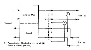
FIGURE 2-33. LOOPBACK TEST SWITCH
