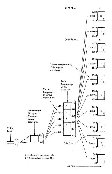
FIGURE 2-9. FREQUENCY TRANSLATION, L-1 CARRIER SYSTEM
