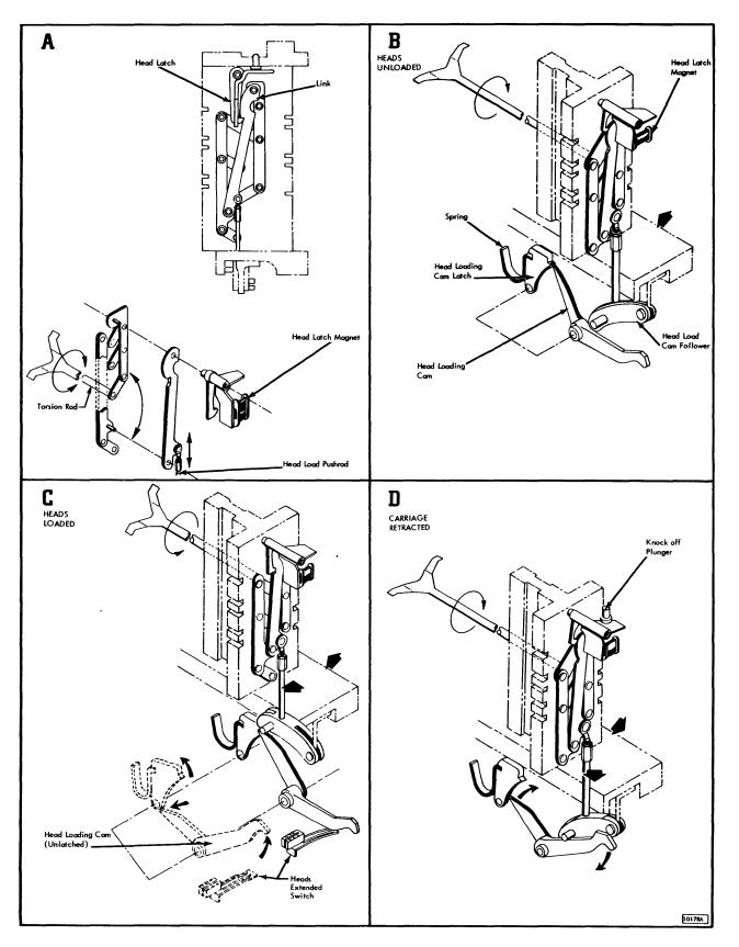
Figure 2-11. Head Load Mechanism
