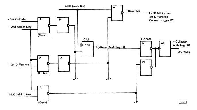
Figure 2-19. Cylinder Address Register Gating
