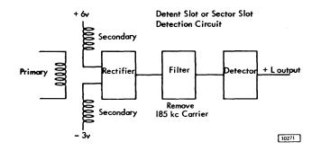
The entire transducer assembly is potted so that no adjustments are possible other than the position of the transducer assembly. Some coupling exists with the metal plate between the primary and secondary but coupling is maximum due to eddy currents when the air gap is between the coils. The two windings on the secondary coils are fed into the detection circuitry.
