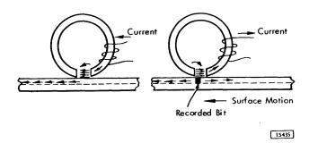
Figure 3-10. Horizontal NRZI Recording
