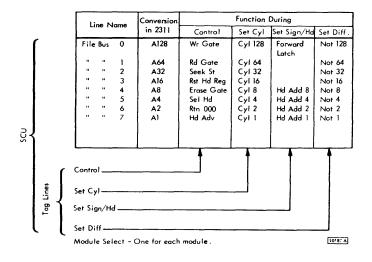
Figure 3-2. Interface Input Lines
