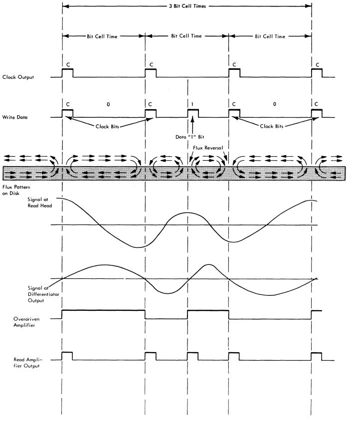
Figure 3-12. Double Frequency Recording Flux and Pulse Relationship
