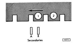
• As the cylinder slotted disk moves, each secondary will be located so each is covered. Outputs are equal; a null in the output occurs.
