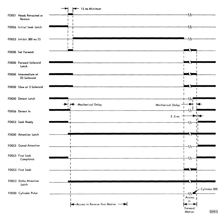
Figure 3-7. Timing for Recalibrate (Restore)
