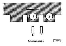
• Further movement results in each secondary being covered with another null output resulting.
