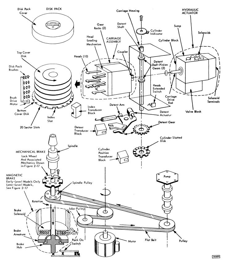
Figure 2-1. Mechanical Components
