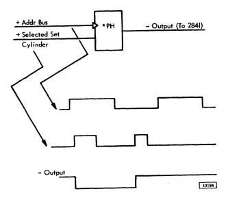
Figure 2-18. CAR Flip Latch Operation
