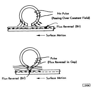
Figure 3-11. Reading Horizontal Fields with Ring Head
