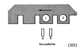
• More movement causes output A to be minimum and B maximum.
