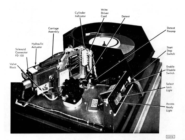
Figure 1-4. Disk Pack and Access Mechanism
