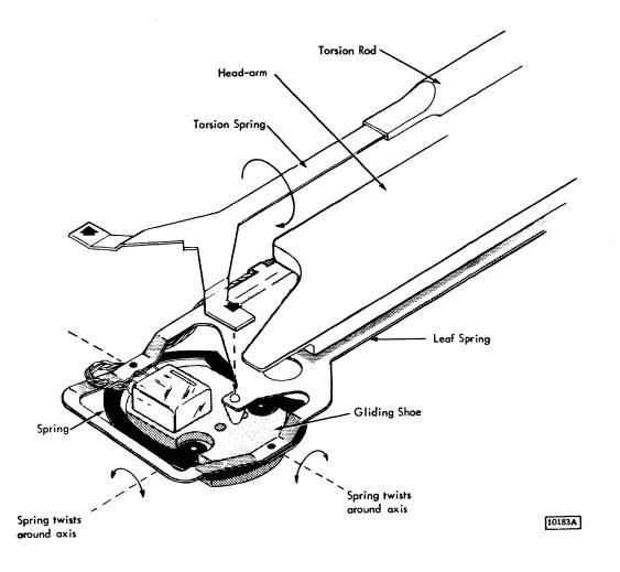
Figure 2-15. Head Assembly and Torsion Rod
