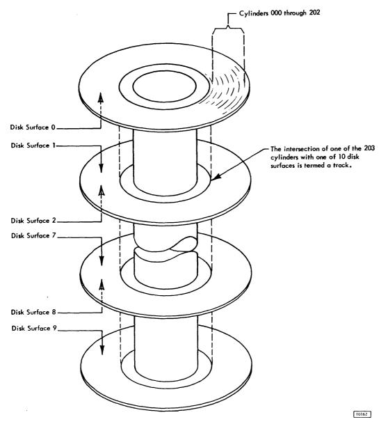
Figure 1-8. Disk and Cylinder Arrangement
