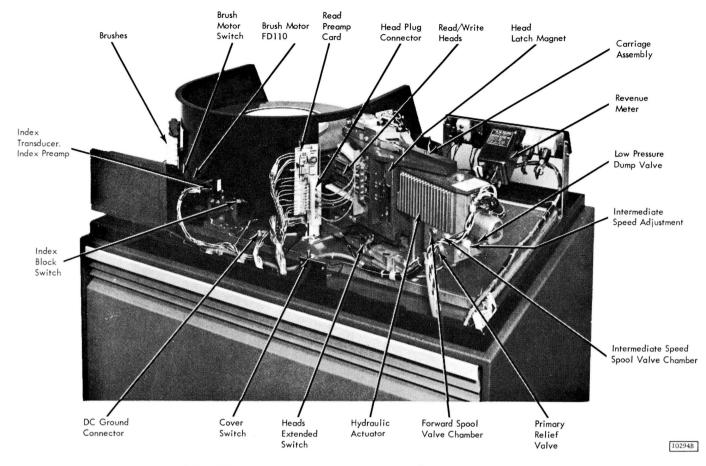
Figure 1-5. Hydraulic Mechanism, Rear View
