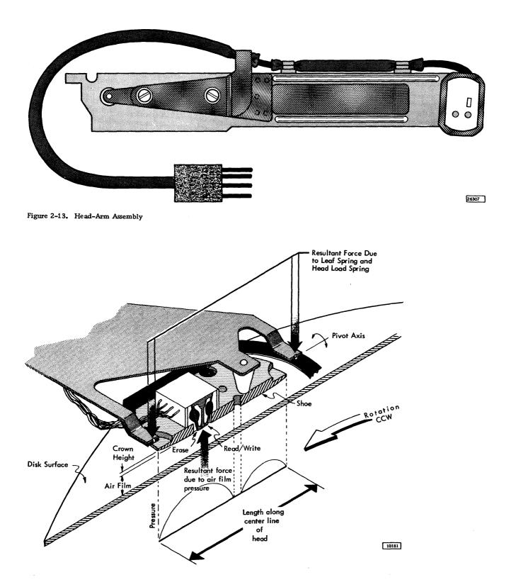
Figure 2-14. "Flying" the Read/Write Head
