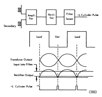
Figure 3-17. Cylinder Position Indicator
