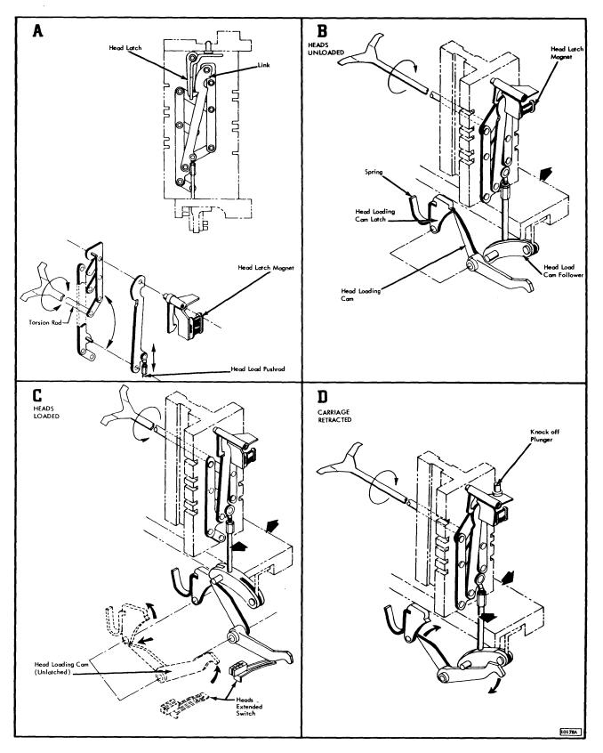
Figure 1-6. Head Load Mechanism
