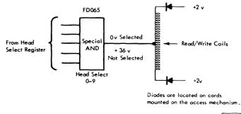
Figure 2-20. Read Write Head Selection
