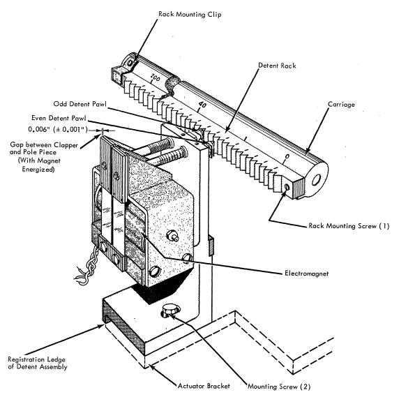
Figure 4-4. Detect Assembly, Adjustment
