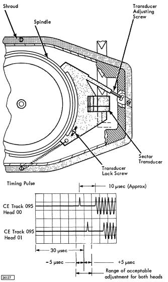
Figure 4-11. Sector Transducer Index Timing Adjustment
