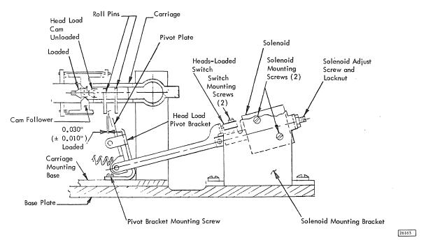
Figure 7-5. Head Load Assembly Adjustment
