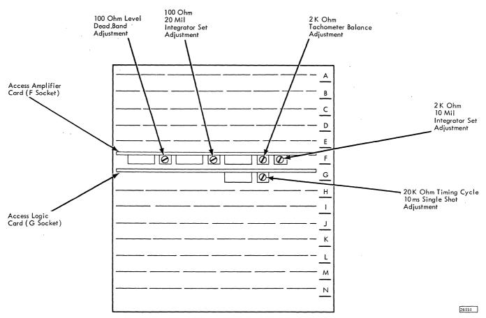
Figure 4-3. Access Adjustment, Potentiometer Locations
