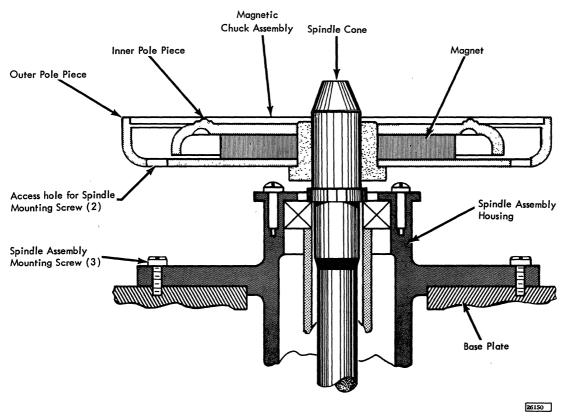
Figure 4-1. Magnetic Check and Spindle Assembly
