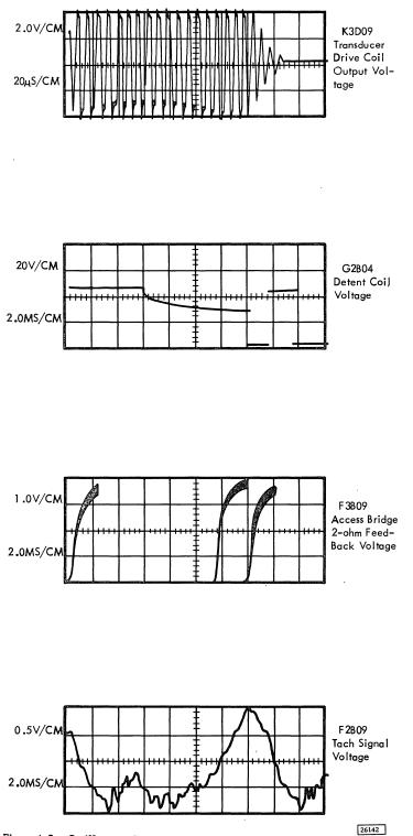
Figure 1-2. Oscilloscope Display of Access Circuits
