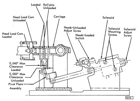
Figure 4-6. Head Load Assembly, Adjustment
