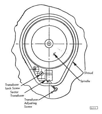
Figure 7-9. Index Timing Adjustment
