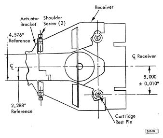
Figure 4-9. Cartridge Receiver Adjustment
