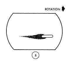
Oxide has accumulated in the pole tip area. Replace head-arm assembly.
