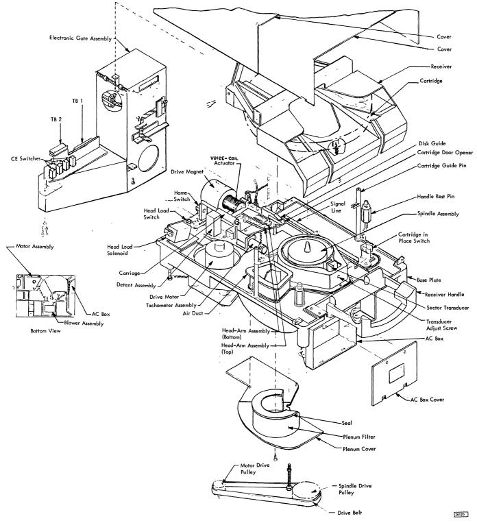
Figure 6-1 Disk Storage Drive, Arrangement of Components
