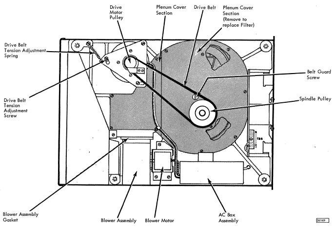
Figure 7-1b. 2310 Disk Storage Drive, Bottom View of Machine
