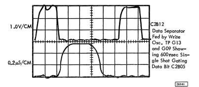
Figure 1-1. Oscilloscope Display of Read/Write Circuits
