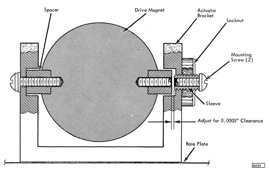
Figure 7-2. Drive Magnet Adjustment
