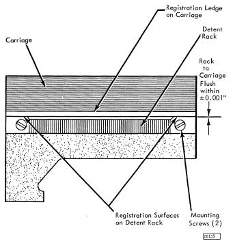
Figure 7-4. Detect Rack, Removal and Replacement
