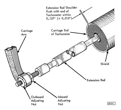
Figure 7-6. Tachometer Extension Rod Adjustment
