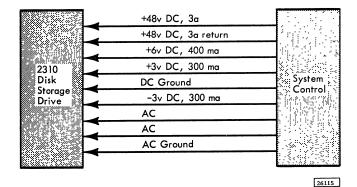
Figure 5-1 Power Lines Interface
