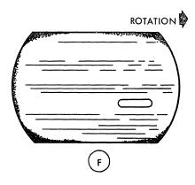
Slight oxide build-up. Clean with 91% isopropyl alcohol. Head-arm assembly may be used.
