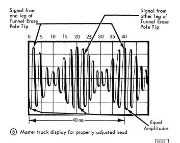
Figure 4-8. Signal Patterns for Head Alignment Adjustment
