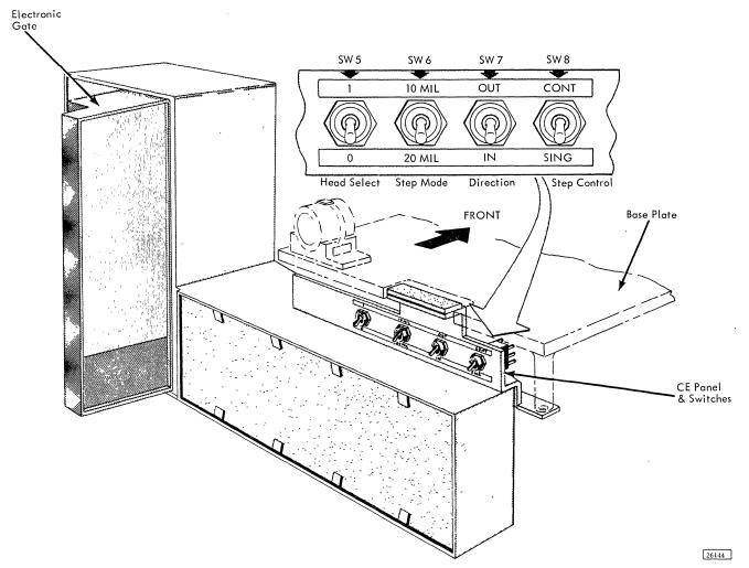
Figure 2-1. CE Panel and Switches
