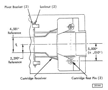
Figure 7-8. Cartridge Receiver Adjustment
