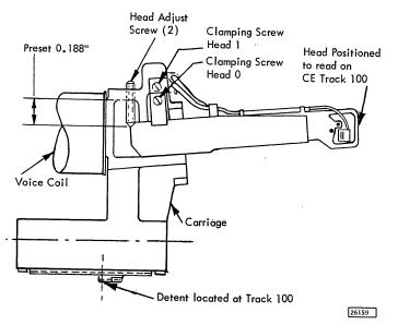
Figure 4-7. Head-Arm Assembly Adjustment
