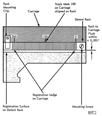
Figure 4-5. Detect Rack Removal and Replacement
