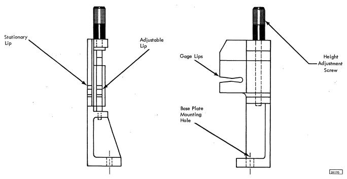
Figure 7-1a. Disk Run Out Gage
