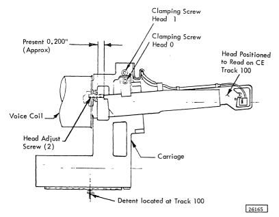
Figure 7-7. Head Arm Assembly Adjustment
