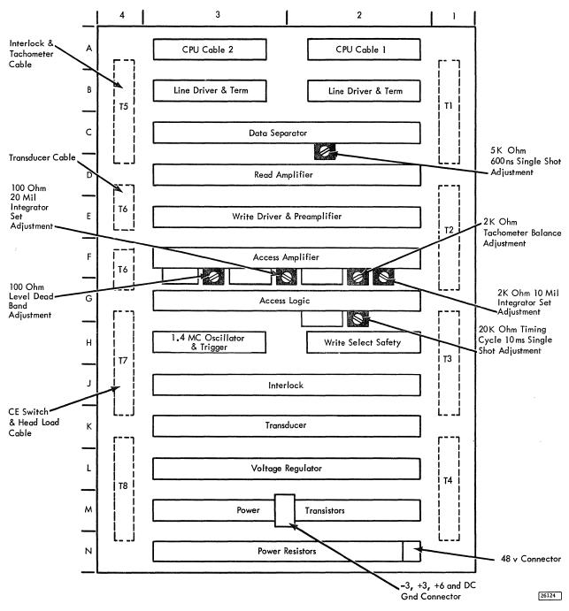
Figure 6-2. Arrangement of SLT Cards in Electronic Gate
