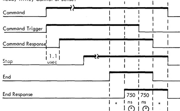
⊗ Timings shown are maximum. They are measured from the time a signal rises on the interface cable until the 7631 brings up its responding signal on the interface cable.
