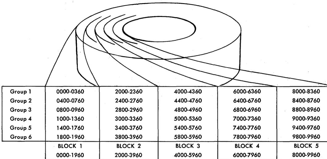
NOTE: Numbers shown in the above chart are track numbers of the lowest numbered track in each cylinder and are the "cylinder addresses."
