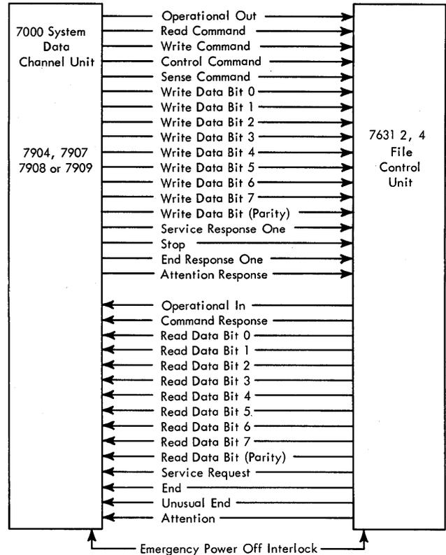
Figure 15. Operating Lines - IBM 7000 Series Data Processing Systems to/from IBM 7631-2 and 4
