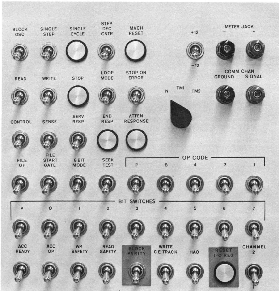
Figure 22. IBM 7631 Model 3 Customer Engineer Panel
