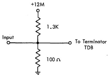
Figure 52. End of Line Terminator (TAC)
