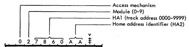
Figure 18. Core Storage Disk Address Word
