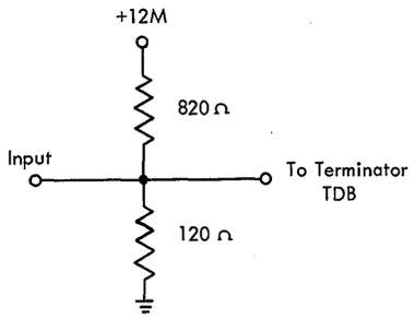
Figure 51. End of Line Terminator (TCK)
