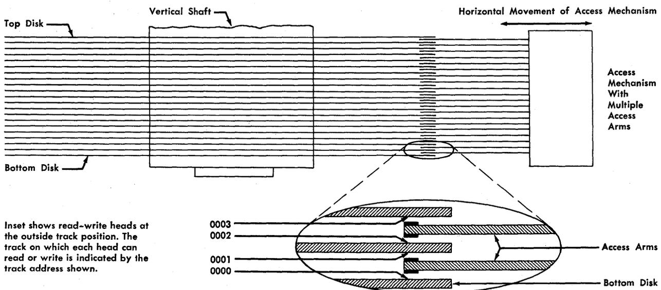
Figure 4. Module and Access Mechanism
