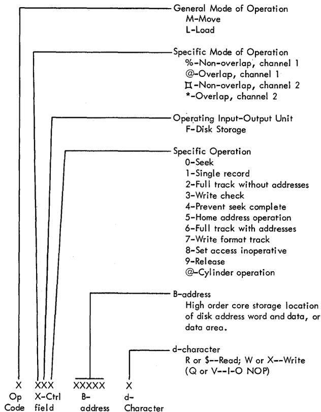
Figure 17. Disk Storage Operation Code Format
