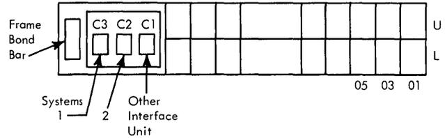
Figure 24. IBM 7631 Terminal Block Locations
