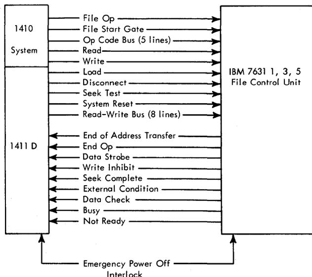
Figure 16. Operating Lines - IBM 1410 Data Processing System to/from IBM 7631 1, 3, and 5
