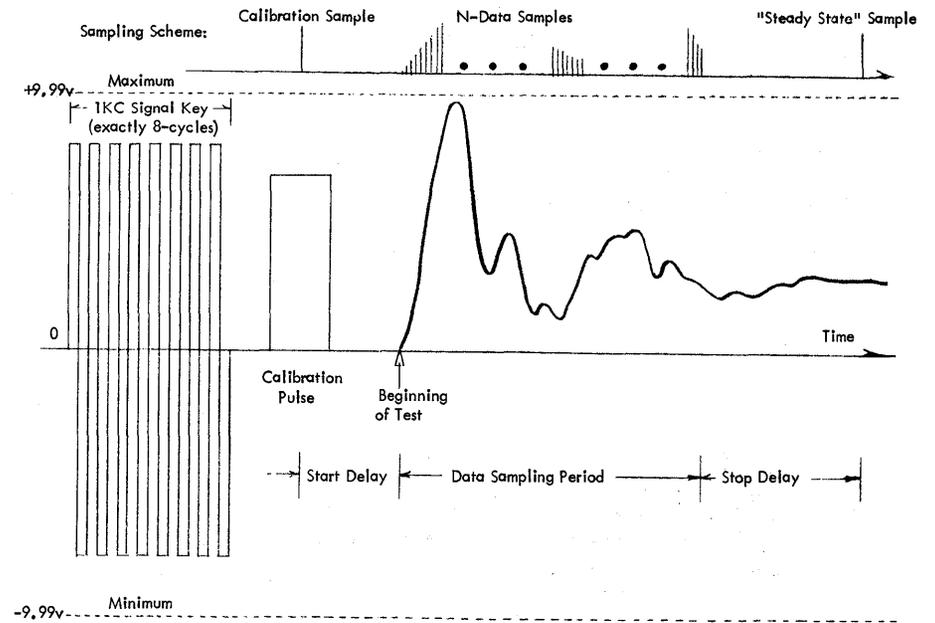
Figure 4. Format of input signal to the analog-to-digital subsystem.
