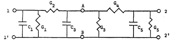
Figure 1. Network Used to Illustrate the Calculation of  $\Delta$  Using Percival's Method.
