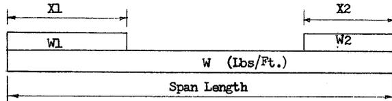
The fixed end moments are found for each span and substituted into the matrix. The simultaneous equations are solved for the final end moments. The dead load moments and shears are then found at the tenth points of each span.
