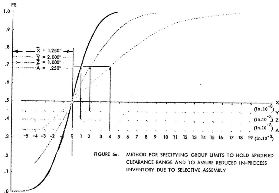
FIGURE 6e. METHOD FOR SPECIFYING GROUP LIMITS TO HOLD SPECIFIED CLEARANCE RANGE AND TO ASSURE REDUCED IN-PROCESS INVENTORY DUE TO SELECTIVE ASSEMBLY
