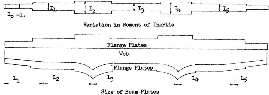
This information is then entered as input data. If the web and plate sizes are given for the section, the moment of inertia variation is computed for the girder.
