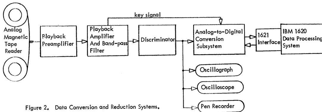
Figure 2. Data Conversion and Reduction Systems.
