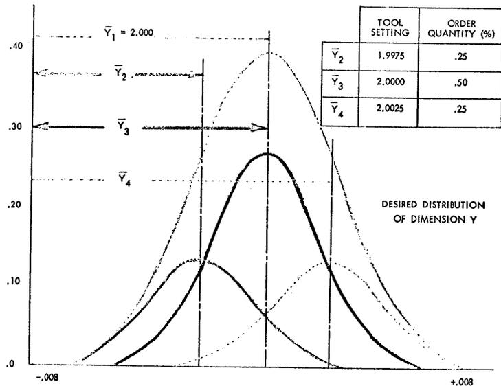
FIGURE 4. PLOT OF DISTRIBUTIONS WHOSE SUM APPROXIMATES THE DESIRED DISTRIBUTION, WITH MACHINING SCHEDULE REQUIRED TO PRODUCE DESIRED DISTRIBUTION
