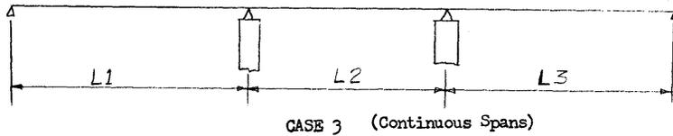
For purposes of expediency, let us say case 1 is the best solution. Our problem is now to determine the various span lengths and the section required for the girders. For highway girders the girder must carry the dead load of the bridge plus a live load as specified by AASHO.
