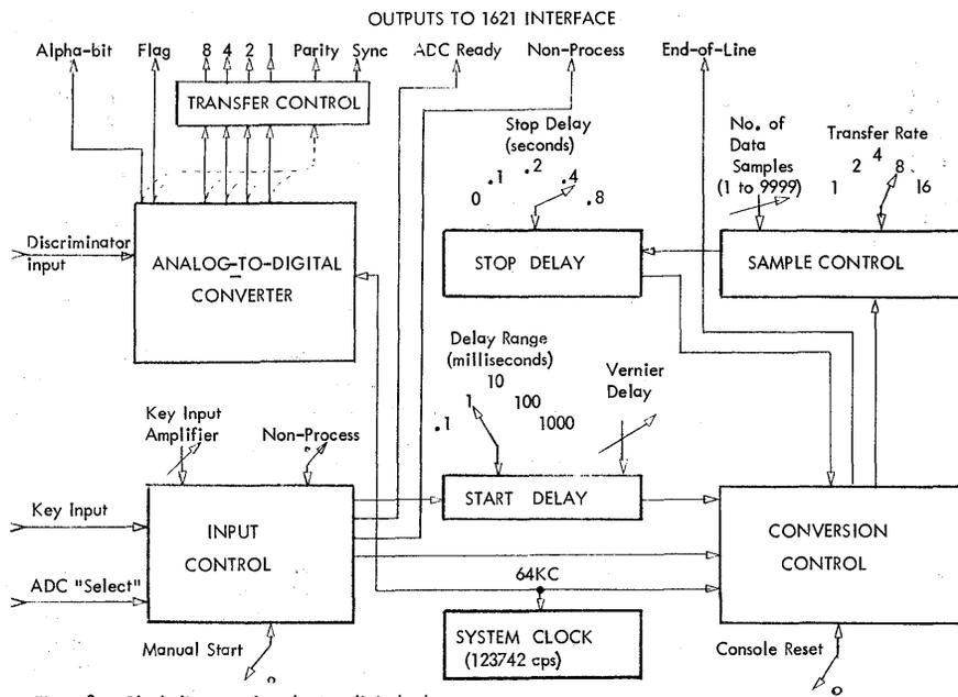
Figure 3. Block diagram of analog-to-digital subsystem.
