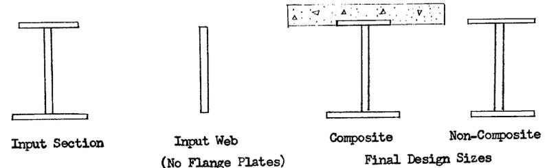
For purposes of computation the flange plates are assumed to be 16 inches wide. If the negative moment exceeds the positive moment no composite design is made.
