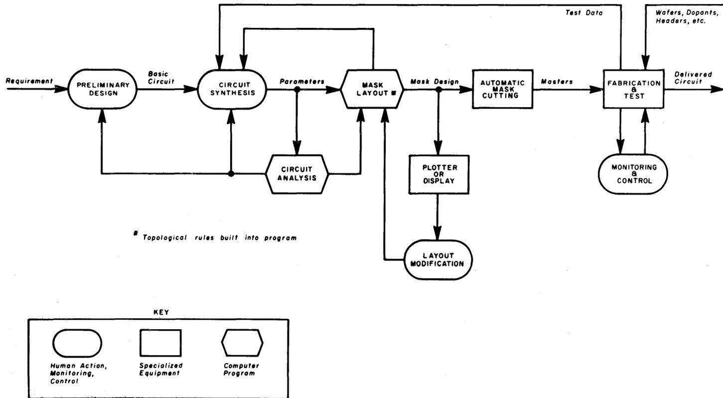
Figure 5. Computer-Aided Design and Development<sup>1</sup> of Integral Circuits.
