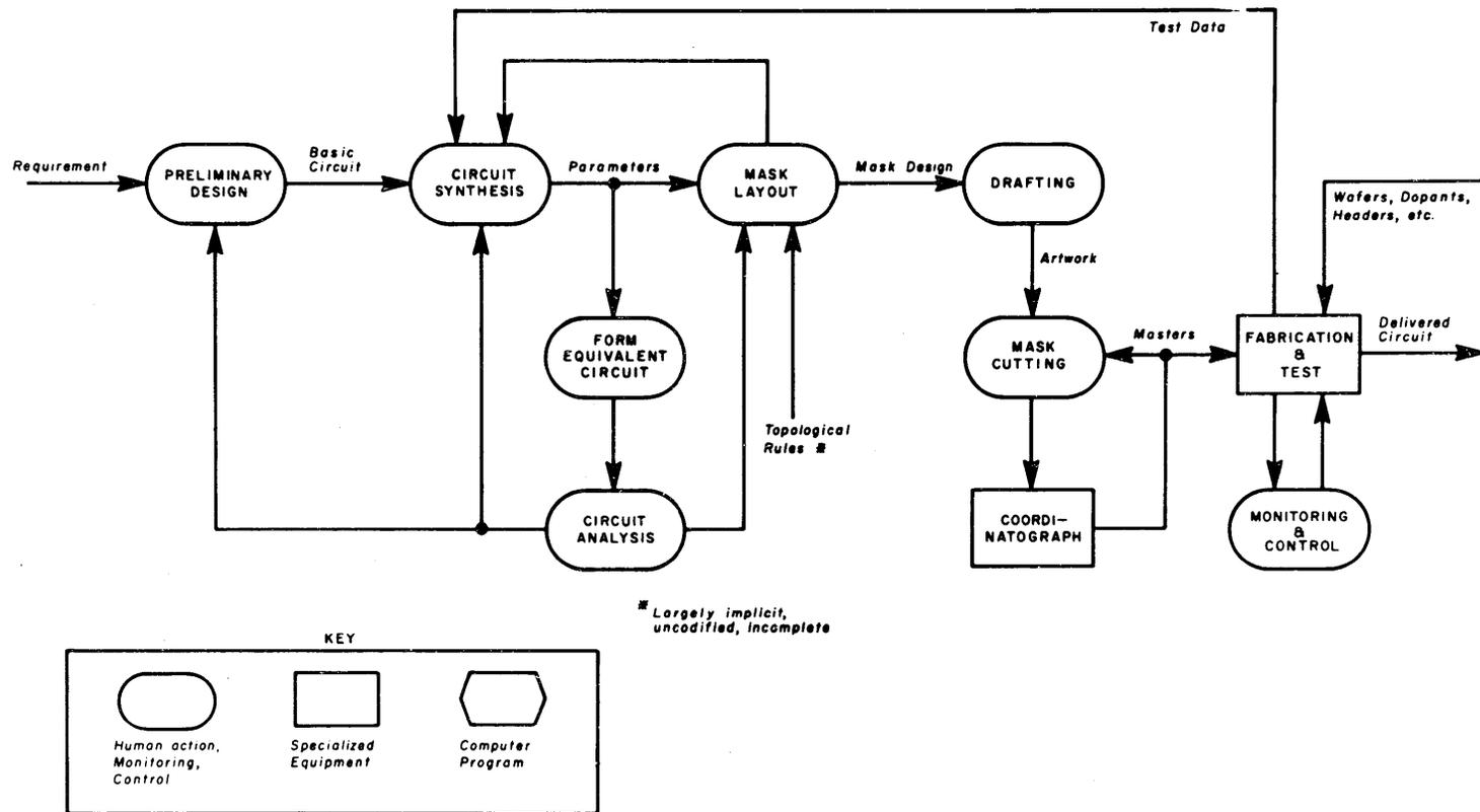
Figure 1. Conventional Design and Development of Integral Circuits
