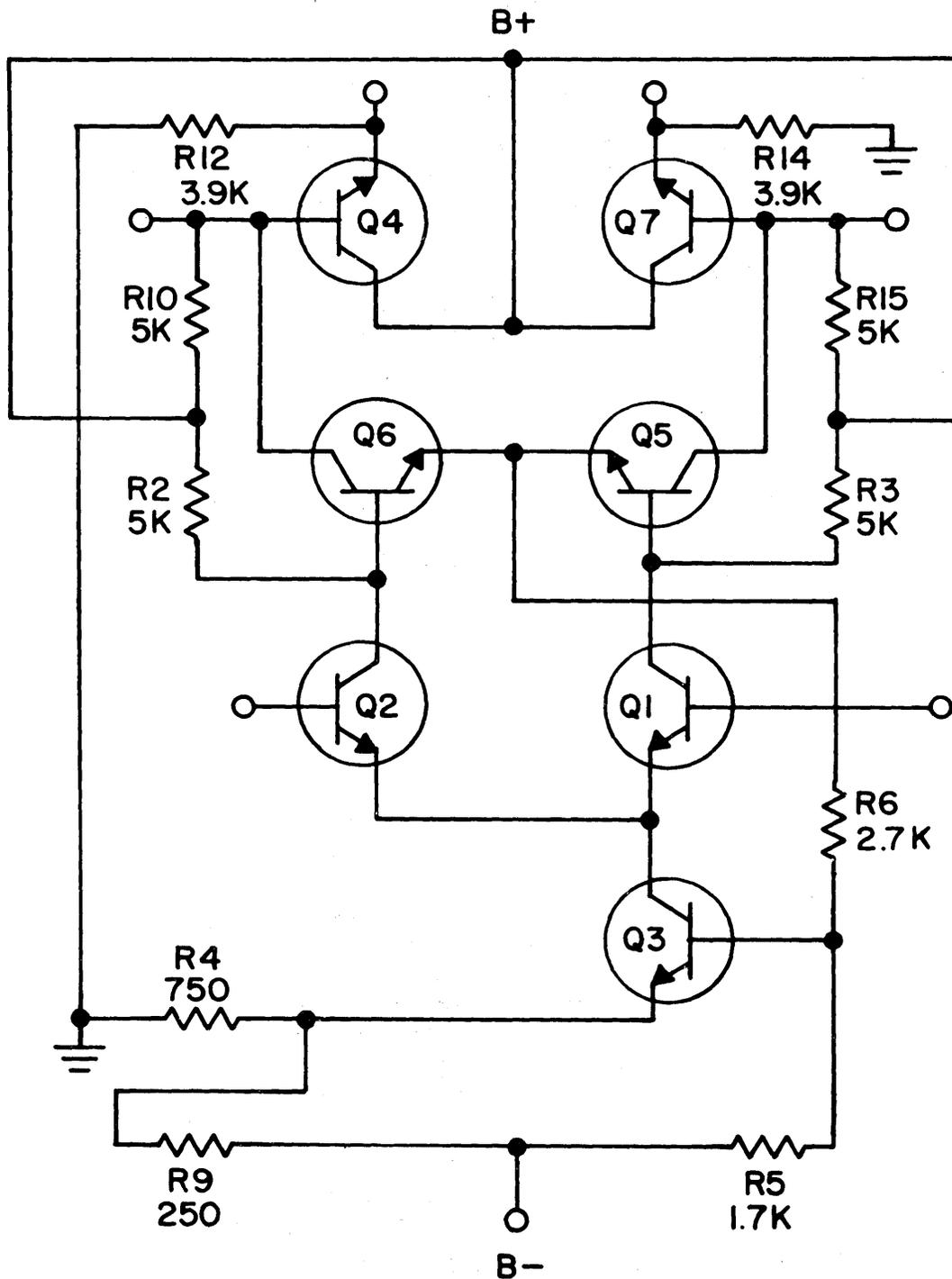
Figure 6. Two-Stage Differential Amplifier
