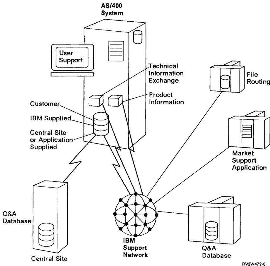
Figure 11-5. Technical Support and Information Access Functions
