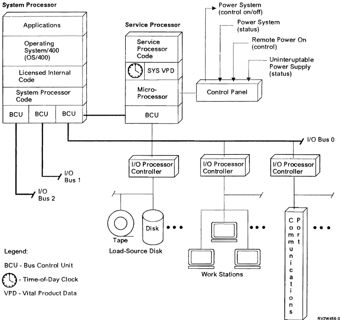
Figure 1-7. High-Level View of AS/400 Hardware and Software
