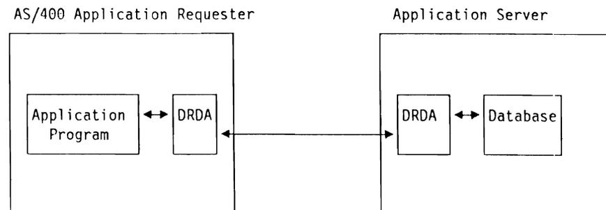
Figure 5-5. DRD Application Requester and Application Server
