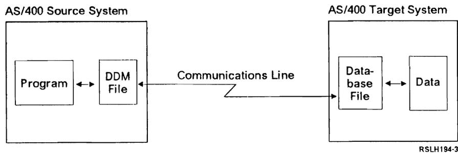
Figure 4-1. Distributed File Management Source and Target Systems
