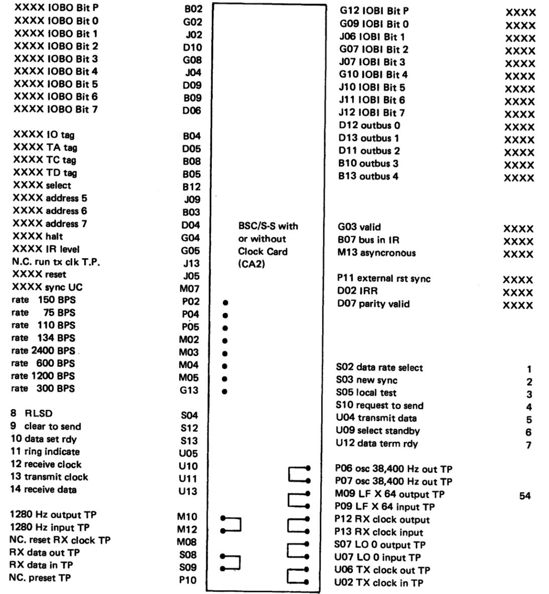
Note: When using the clocked version of BSC/S-S, ground at least one rate pin. No other jumpers are required on the board.
