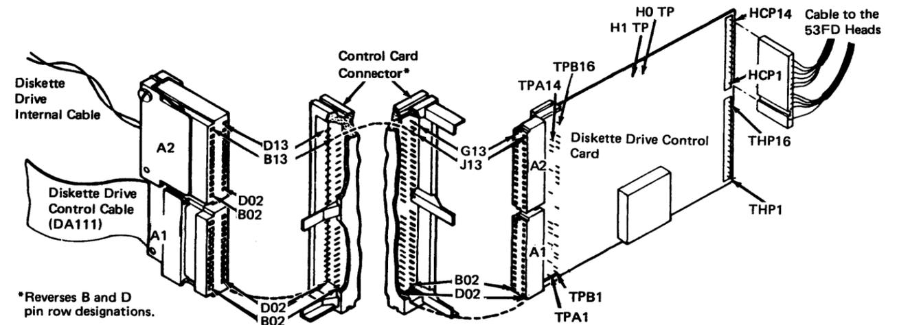
Figure DA420-3. DA3 Card, Connector, and Cable Pin Numbering
