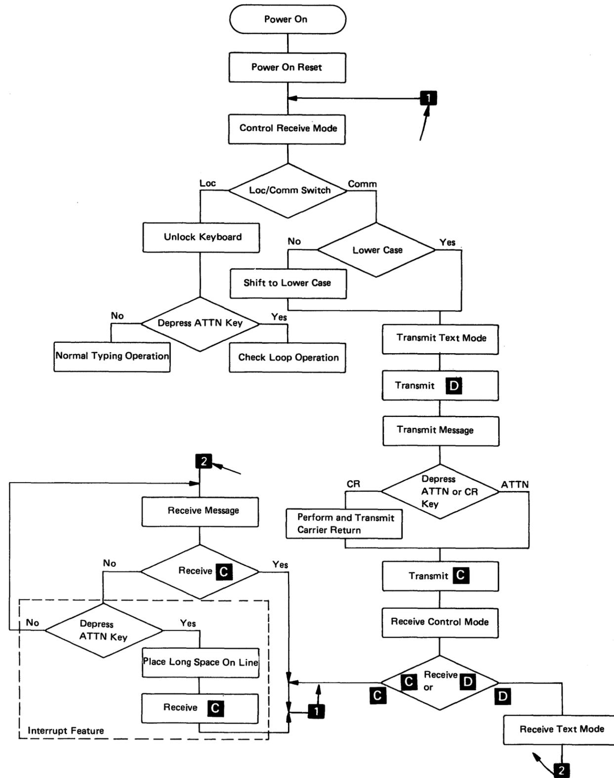
Figure CA643-2. IBM 2741 (with Interrupt Feature) Flow Chart
