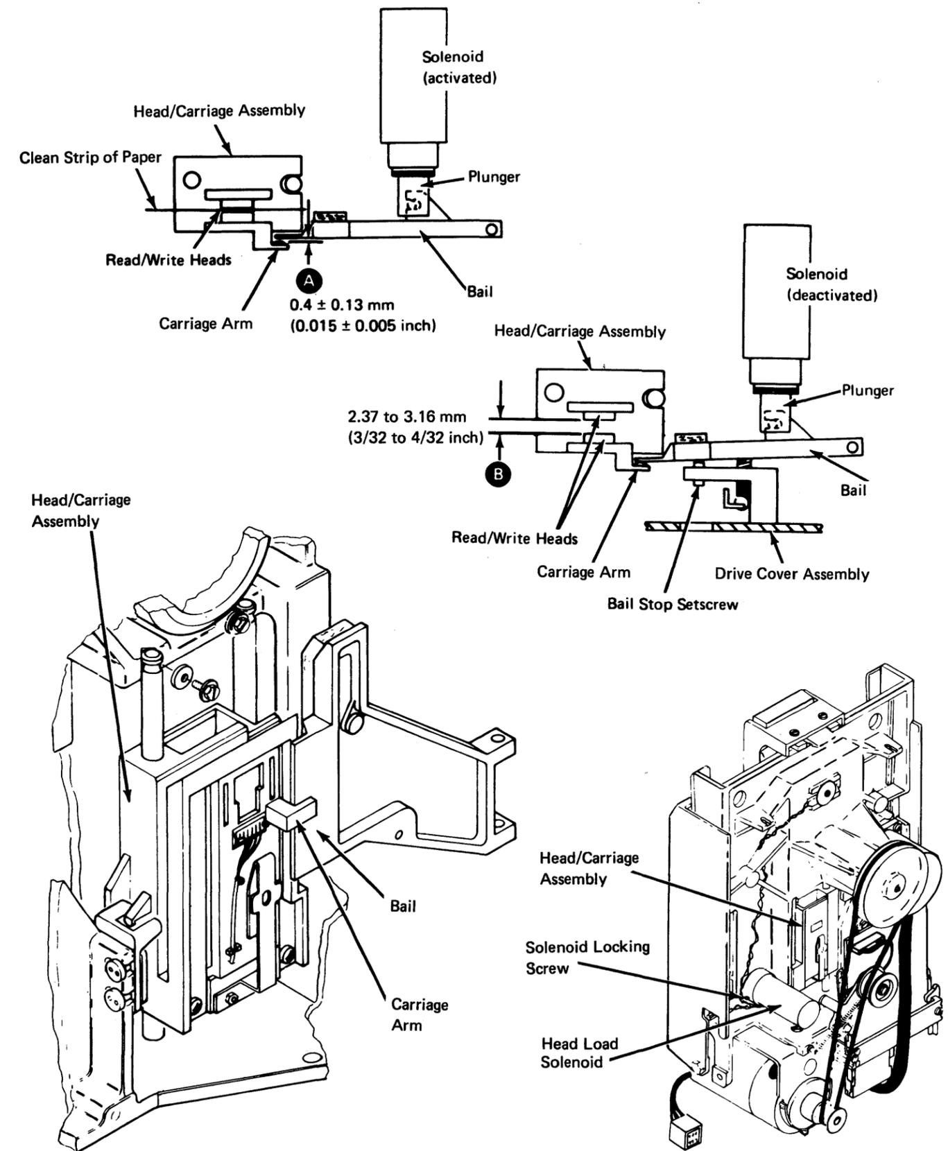
**DA563 Solenoids and Bail Assembly Removal (with Connector Block)**
