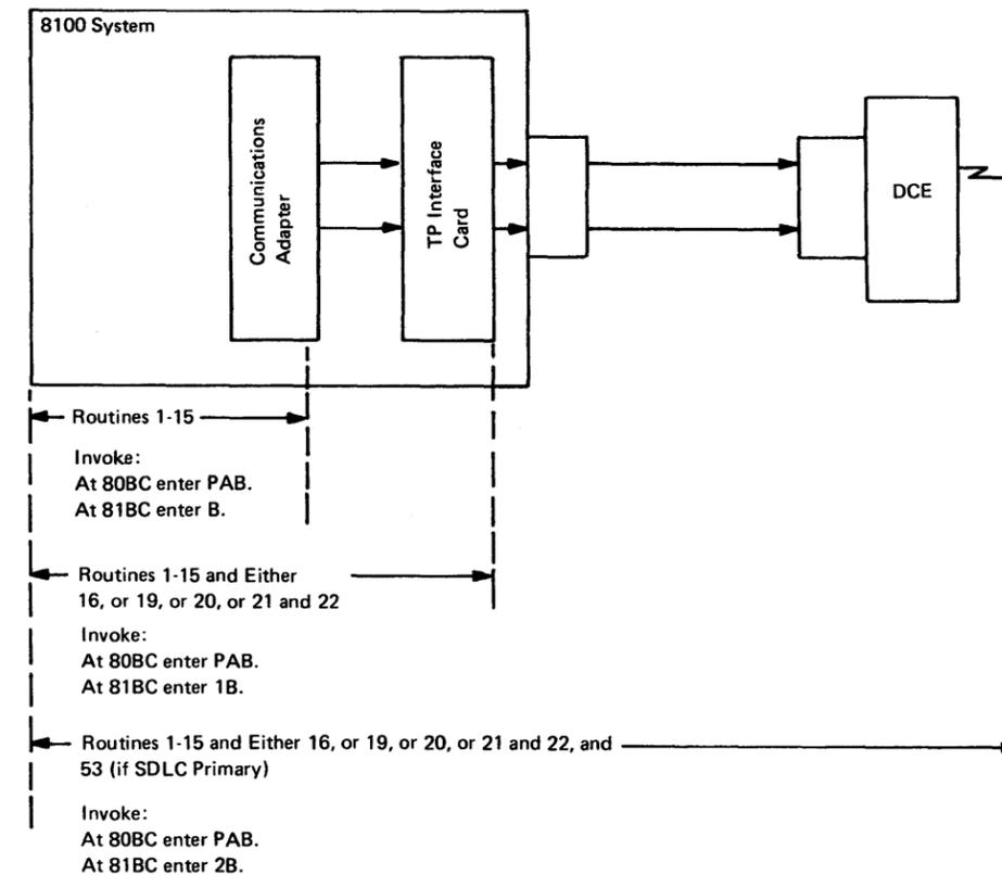
Figure CA202-2. Invocation for a Group of Tests (Level 1 Addressing Only), General TP Feature Example
