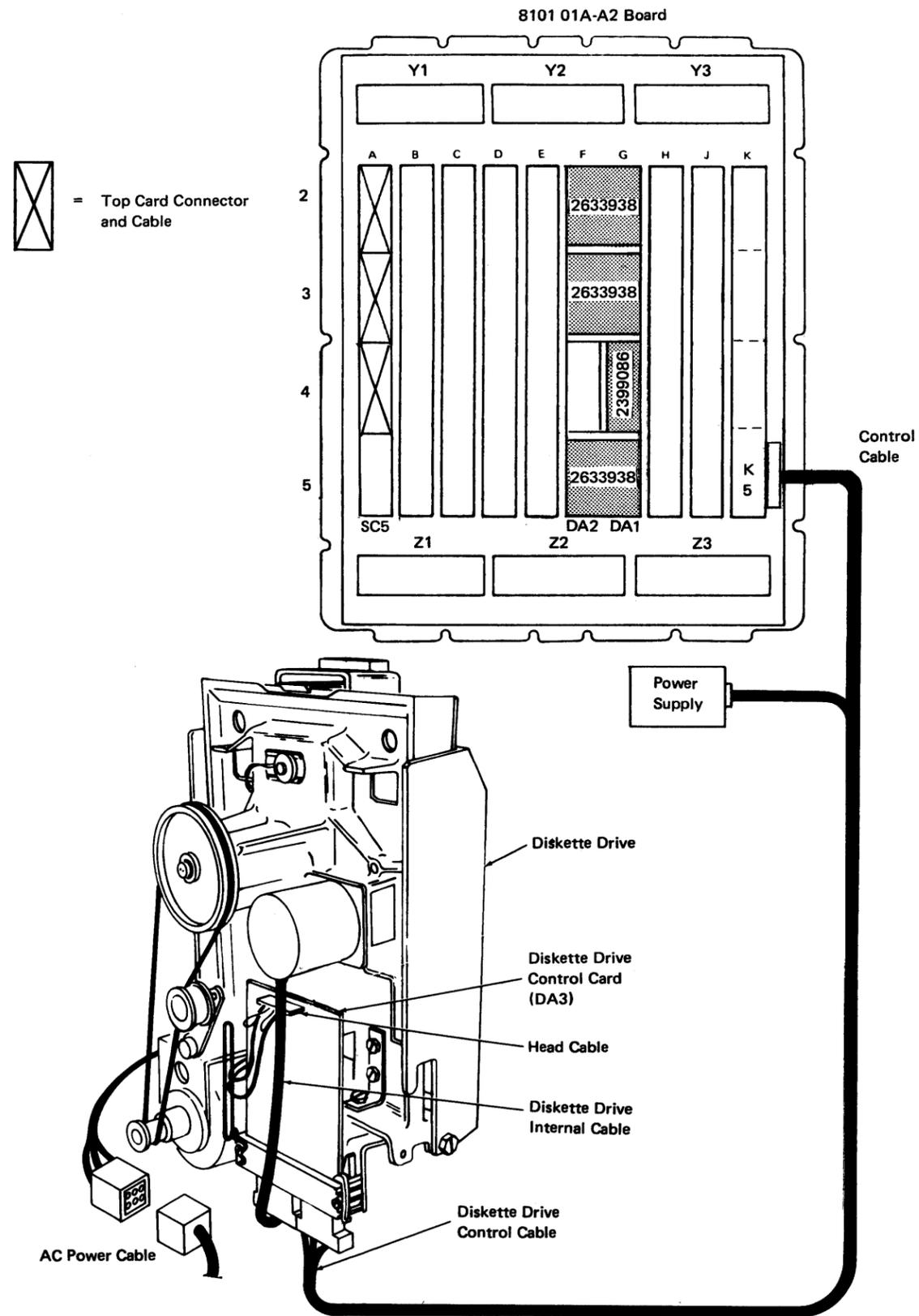
Figure DA111-3. 8101 Diskette Storage Hardware Configuration
