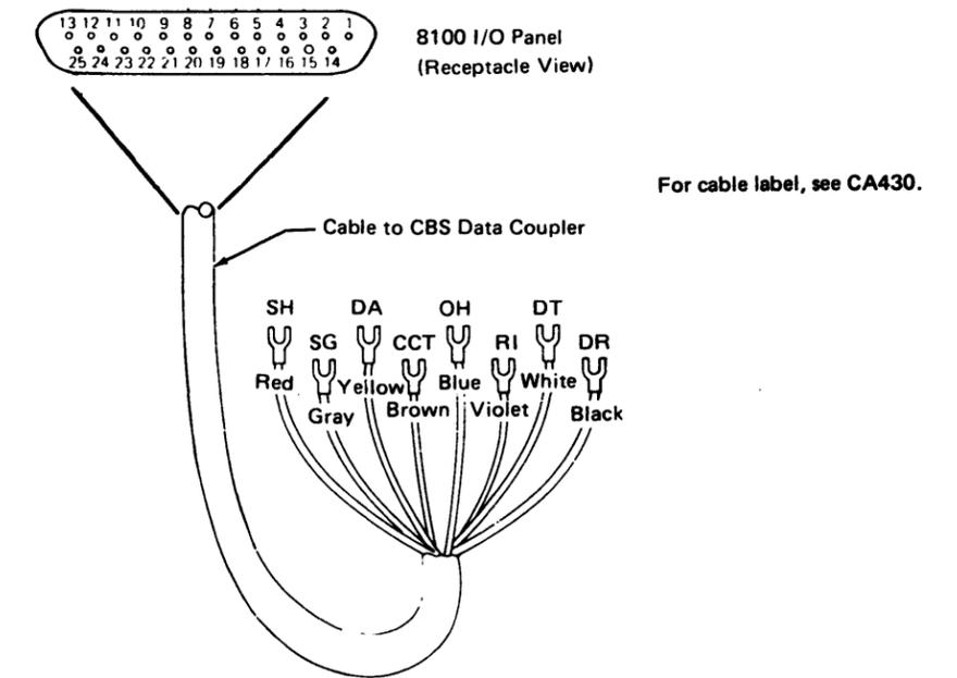
**Figure CA434-2. Integrated Modem (Switched Line) Cable (CAC9)**
