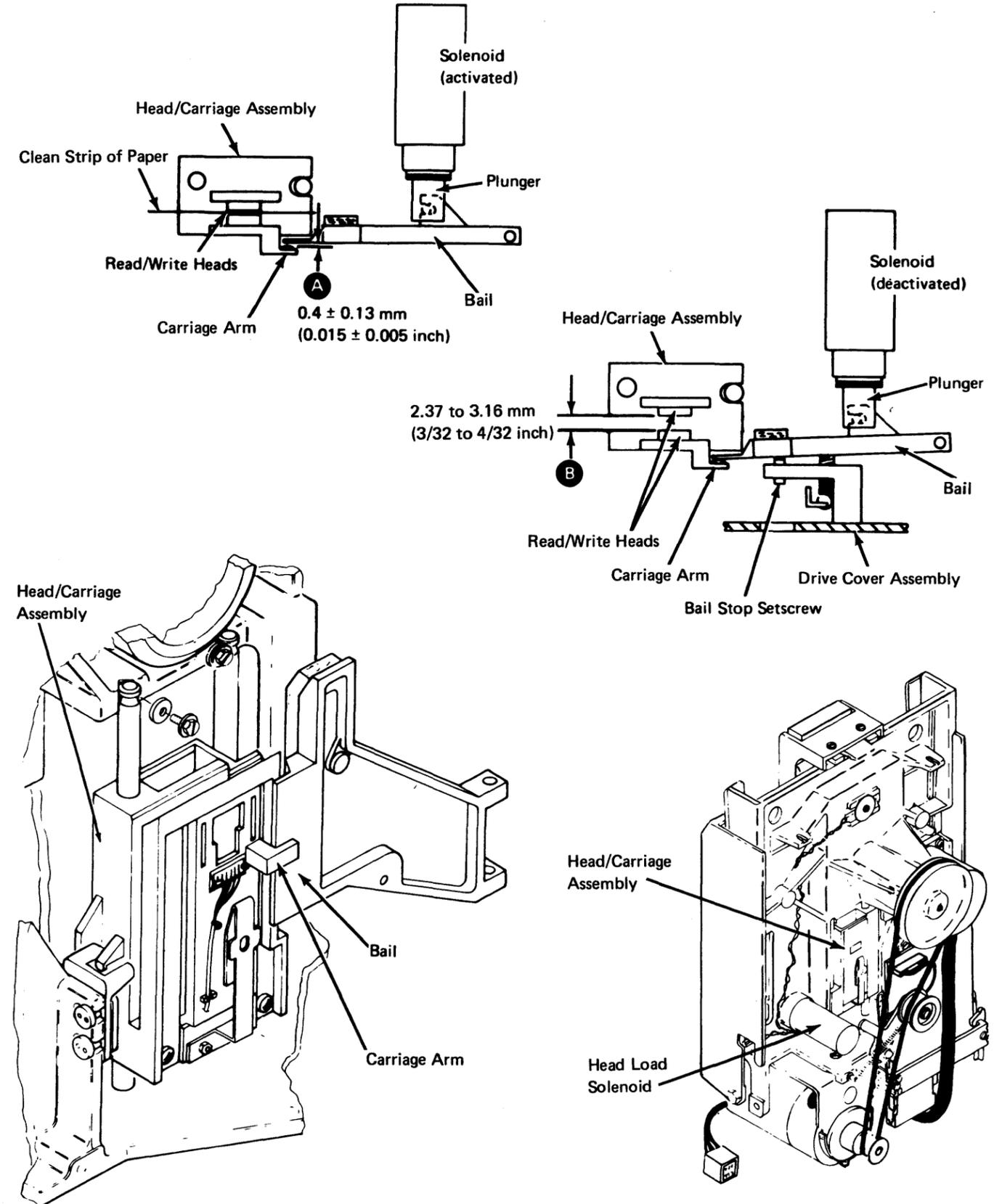
**DA562 Solenoid and Bail Assembly Adjustment**
