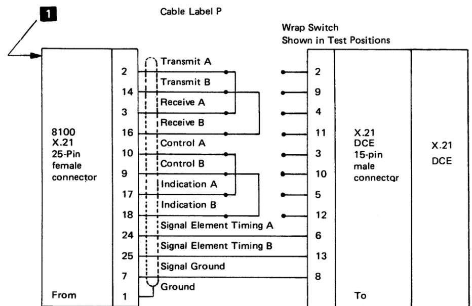
Figure CA546-1. Troubleshooting Diagram for Routine 67 and 68, X.21 (Nonswitched) External Data Wrap
