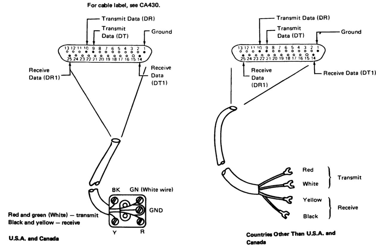
**Figure CA434-1. Integrated Modem (Nonswitched Line) Cable (CAC8)**
