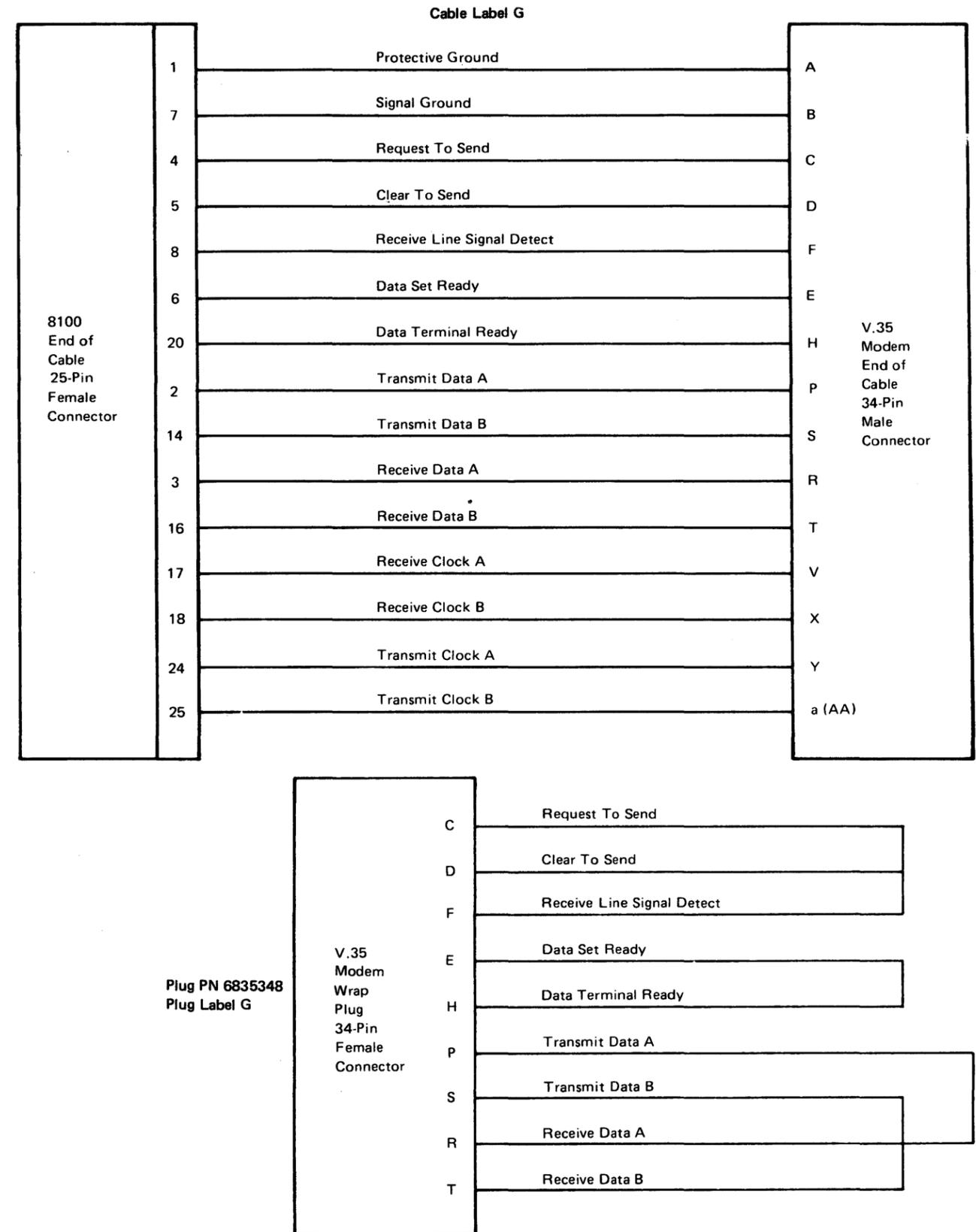
**Figure CA433-1. V.35 External Modem Cable (CAC6A) and Wrap Plug**
