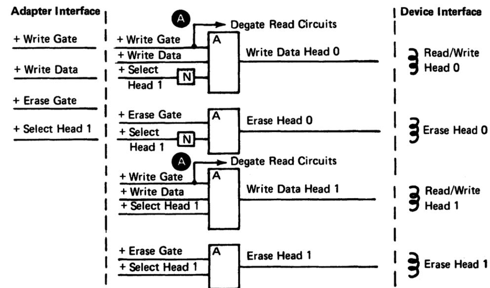
**Figure DA455-1. Write Gate and Erase Gate Logic**
