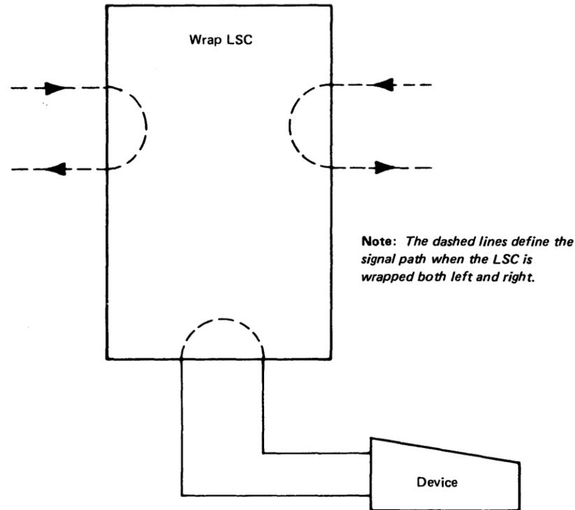
Figure CA561-2. LSC Wrapped Left and Right
