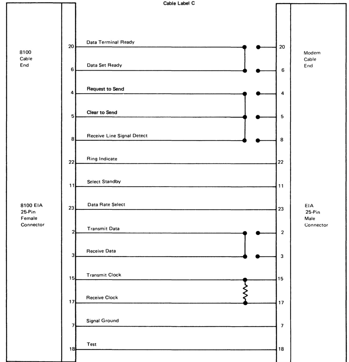
Figure CA431-1. EIA-External Modem Cable (CAC5A)
