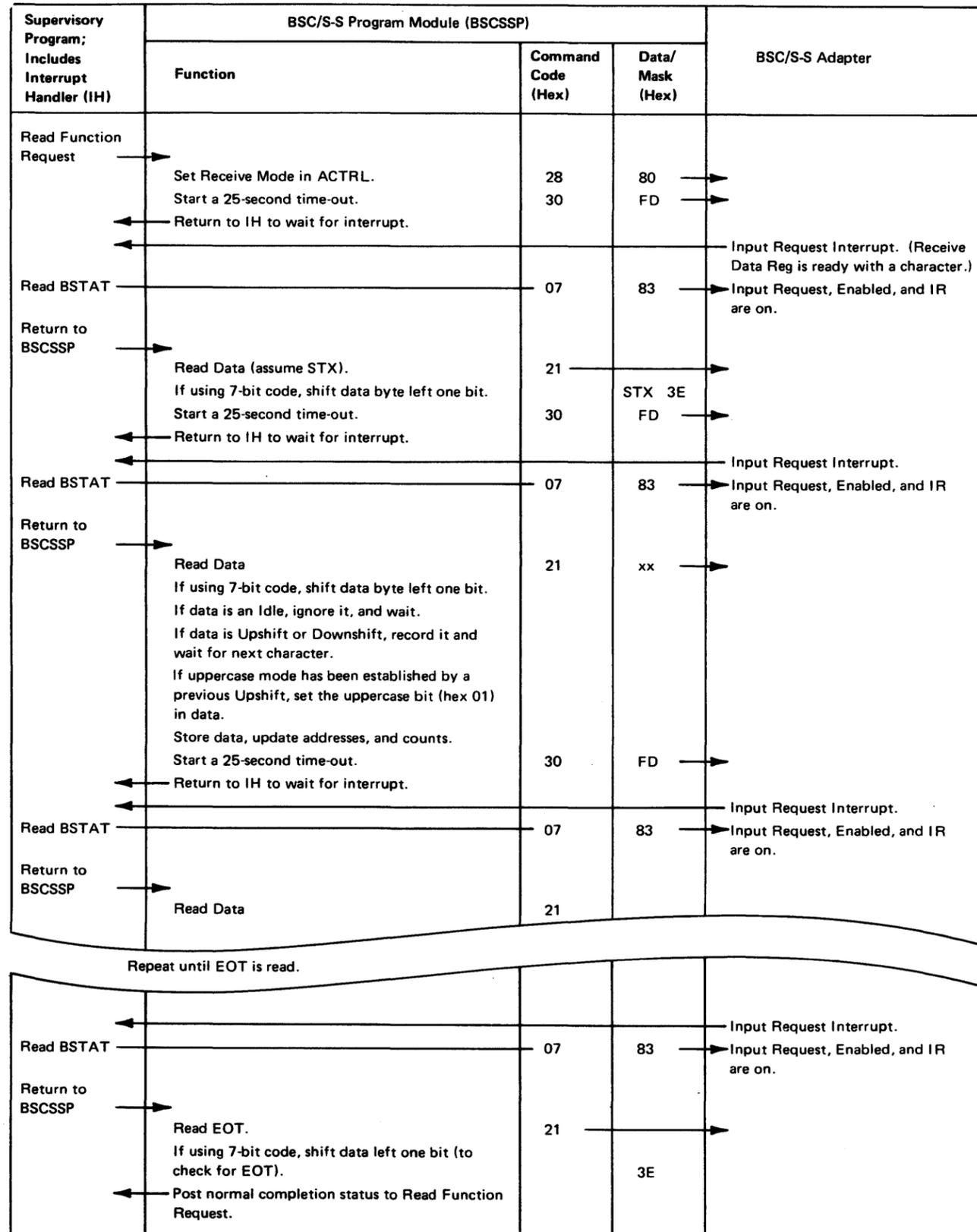
Figure CA122-7. S/S Receive Operation
