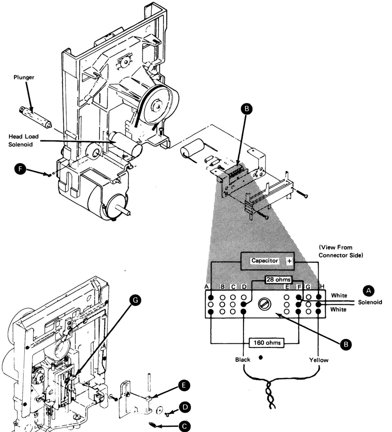
**DA564 Solenoid and Bail Assembly Installation (with Connector Block)**
