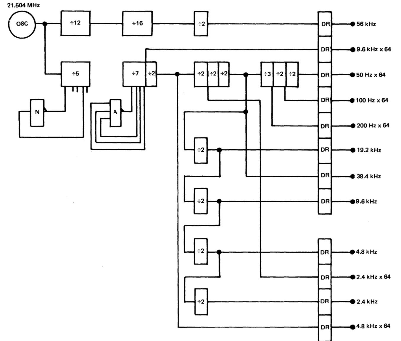
**Figure CA476-1. Multispeed Clock Card (CA10) Schematic**
