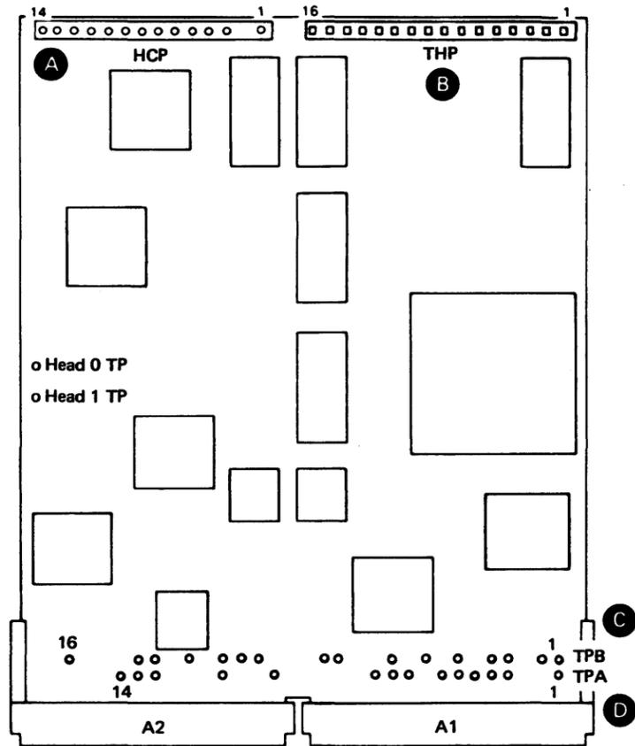
Figure DA420-2. DA3 Card Test Points and Locations
