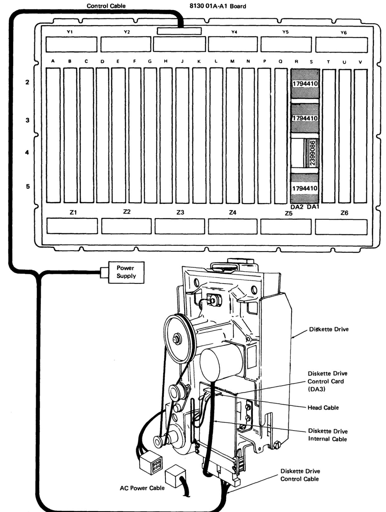
Figure DA111-1. 8130 Diskette Storage Hardware Configuration
