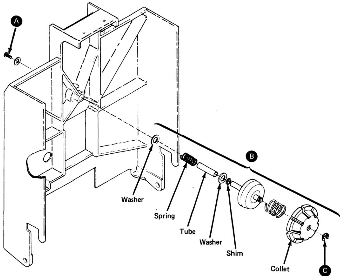
**DA550 Head/Carriage Assembly****DA551 Head/Carriage Assembly Service Check**
