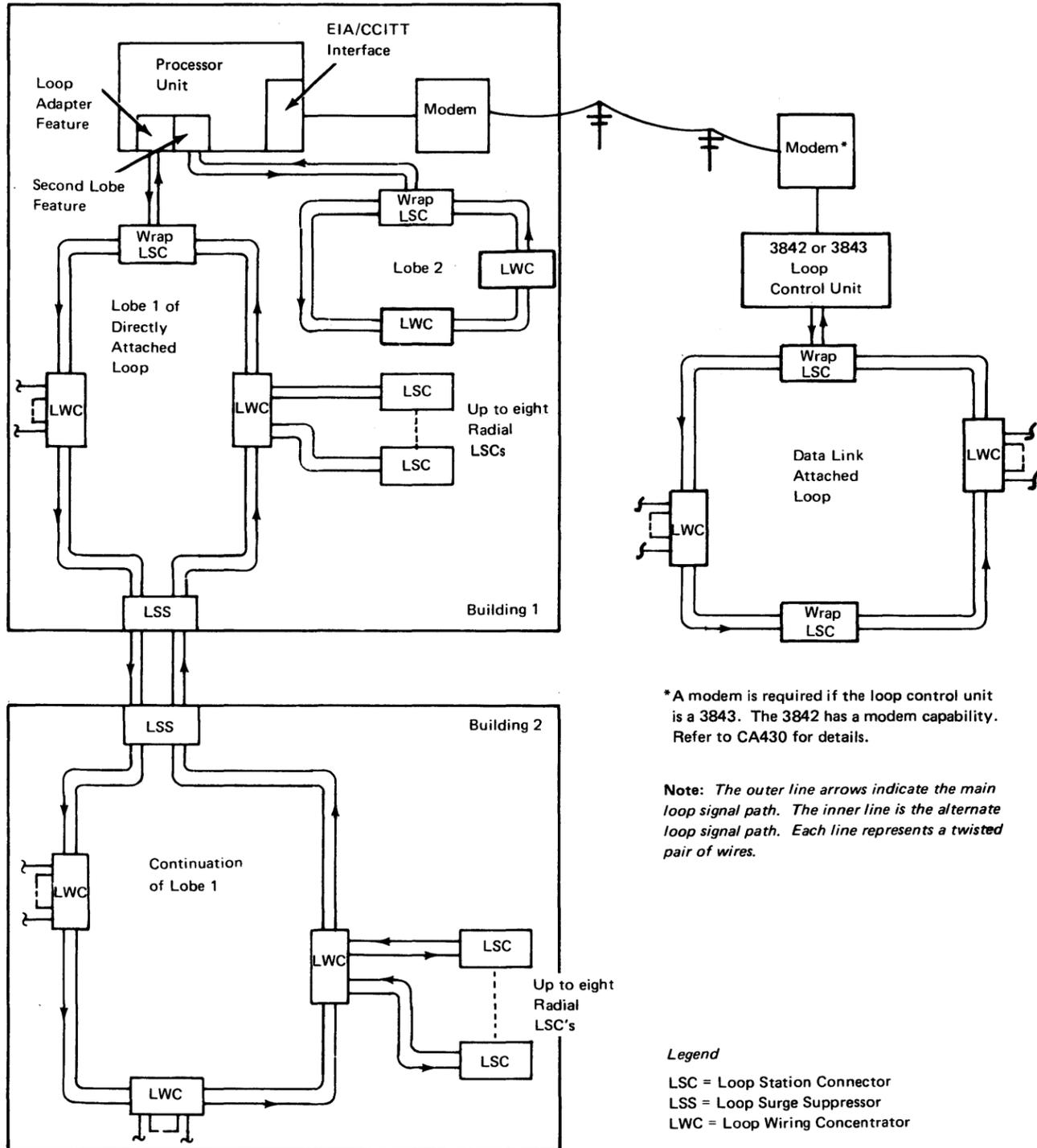
**Figure CA114-5. Sample Loop Configuration**
