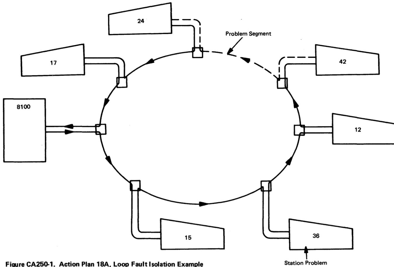
Figure CA250-1. Action Plan 18A, Loop Fault Isolation Example
