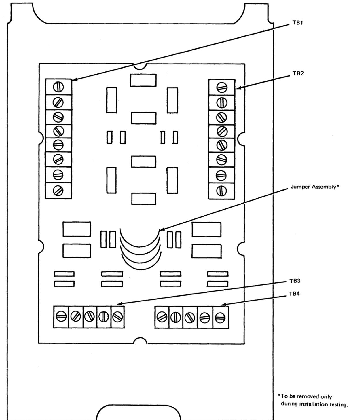
Figure CA564-1. Loop Surge Suppressor (LSS) Circuit Board Assembly
