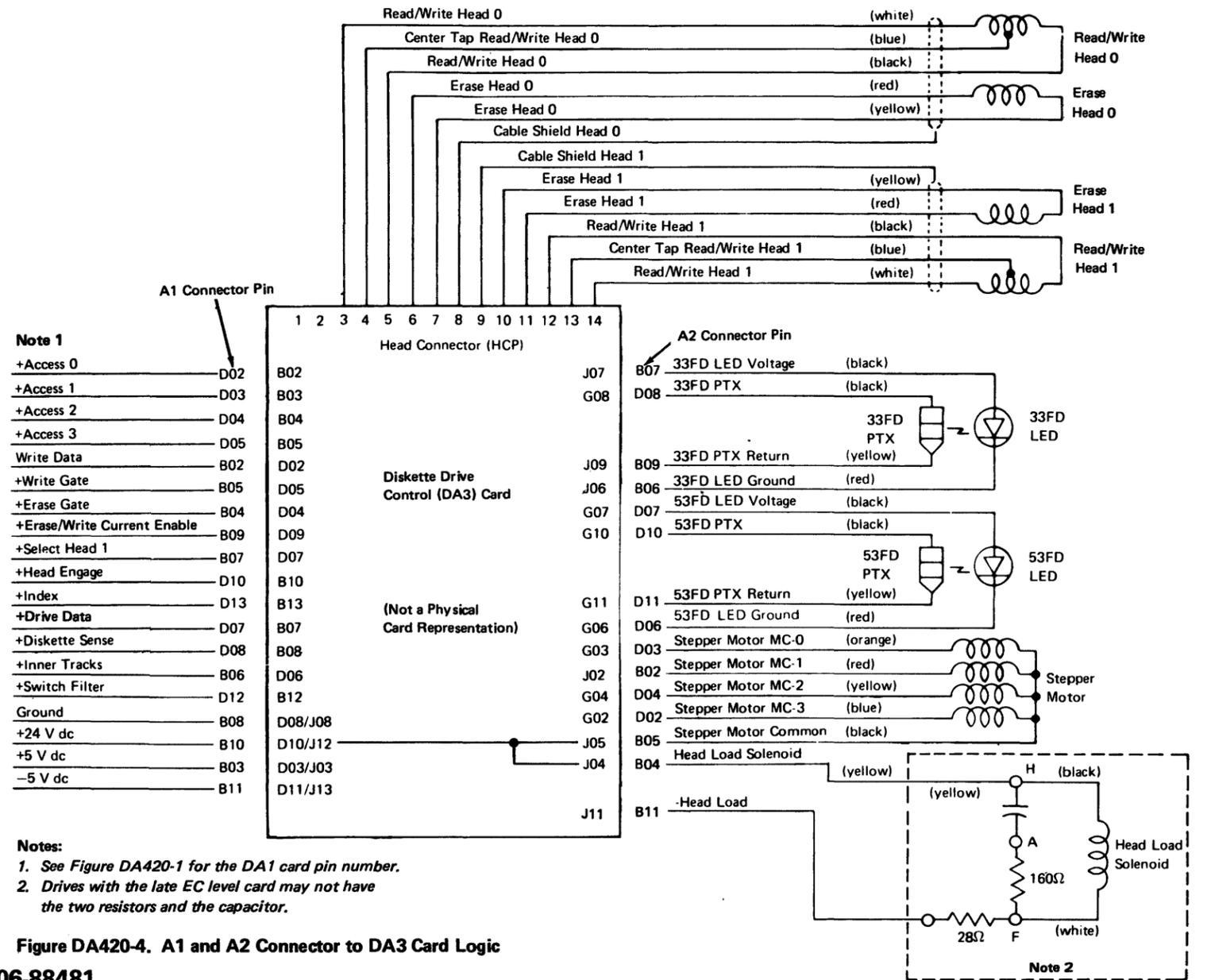
Figure DA420-4. A1 and A2 Connector to DA3 Card Logic
