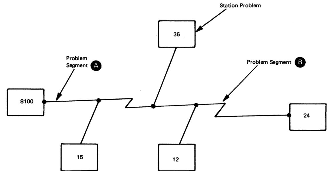
Figure CA250-2. Action Plan 18B, Data Link Fault Isolation Example
