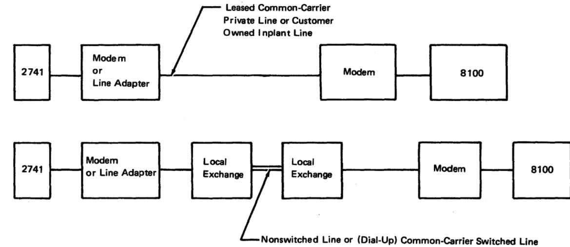
Figure CA643-1. Data Flow In a Point-to-Point Configuration
