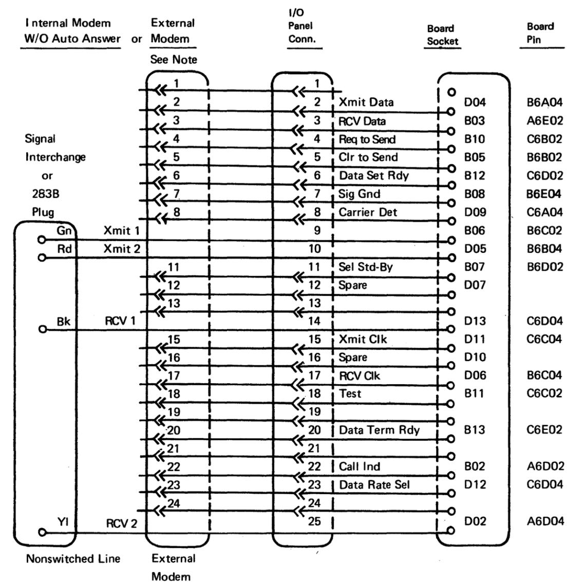
Note: West Germany has a short cable (11, 12, 16, 18, 19 wires deleted) connecting modem and cable from 8100 for D1200's modem attachment. See your TP coordinator for current requirements.
