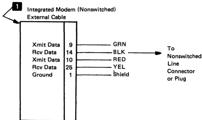
Figure CA542-1. Troubleshooting Diagram for Routine 19, Nonswitched Integrated Modem
