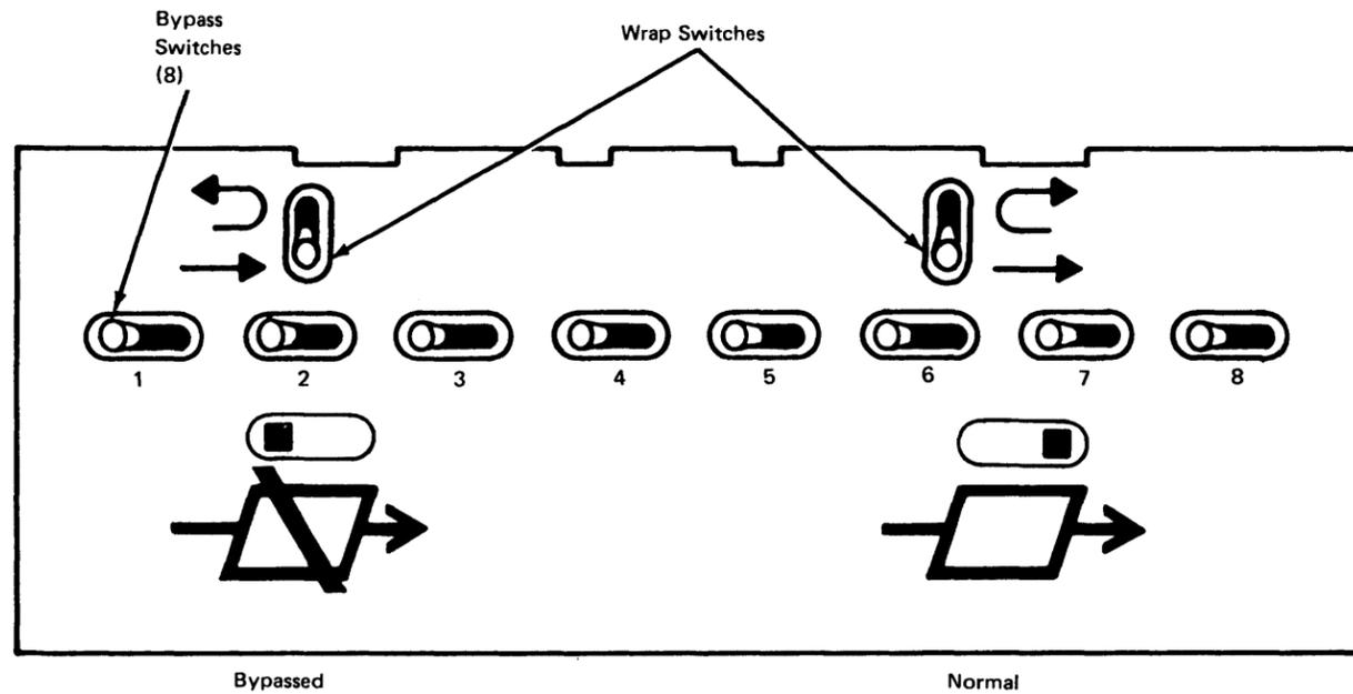
Figure CA561-3. Loop Wiring Concentrator (LWC) Switches
