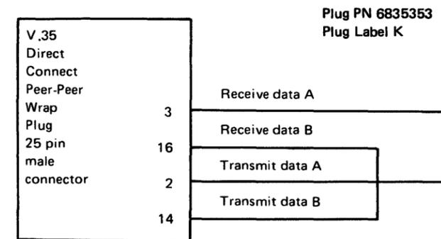
**Figure CA433-3. V.35 Direct Connect Peer-to-Peer Cable (CAC6B) and Wrap Plug**
