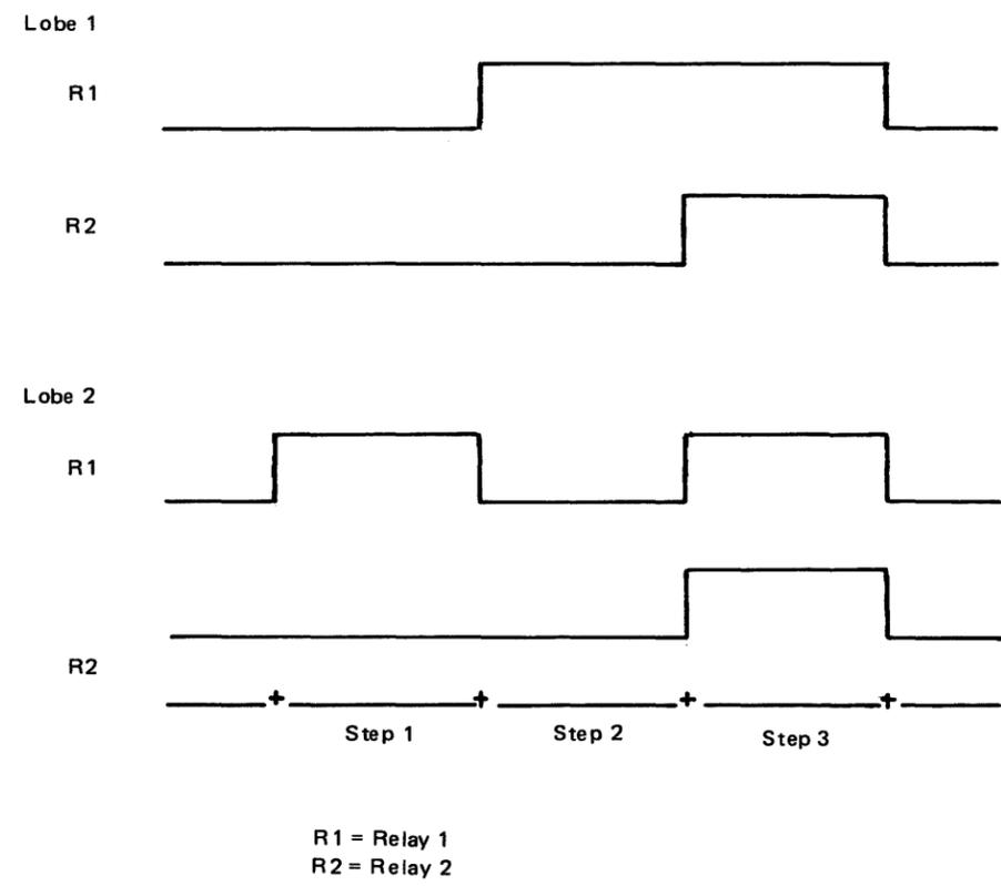
Figure CA653-3. Relay Timing
