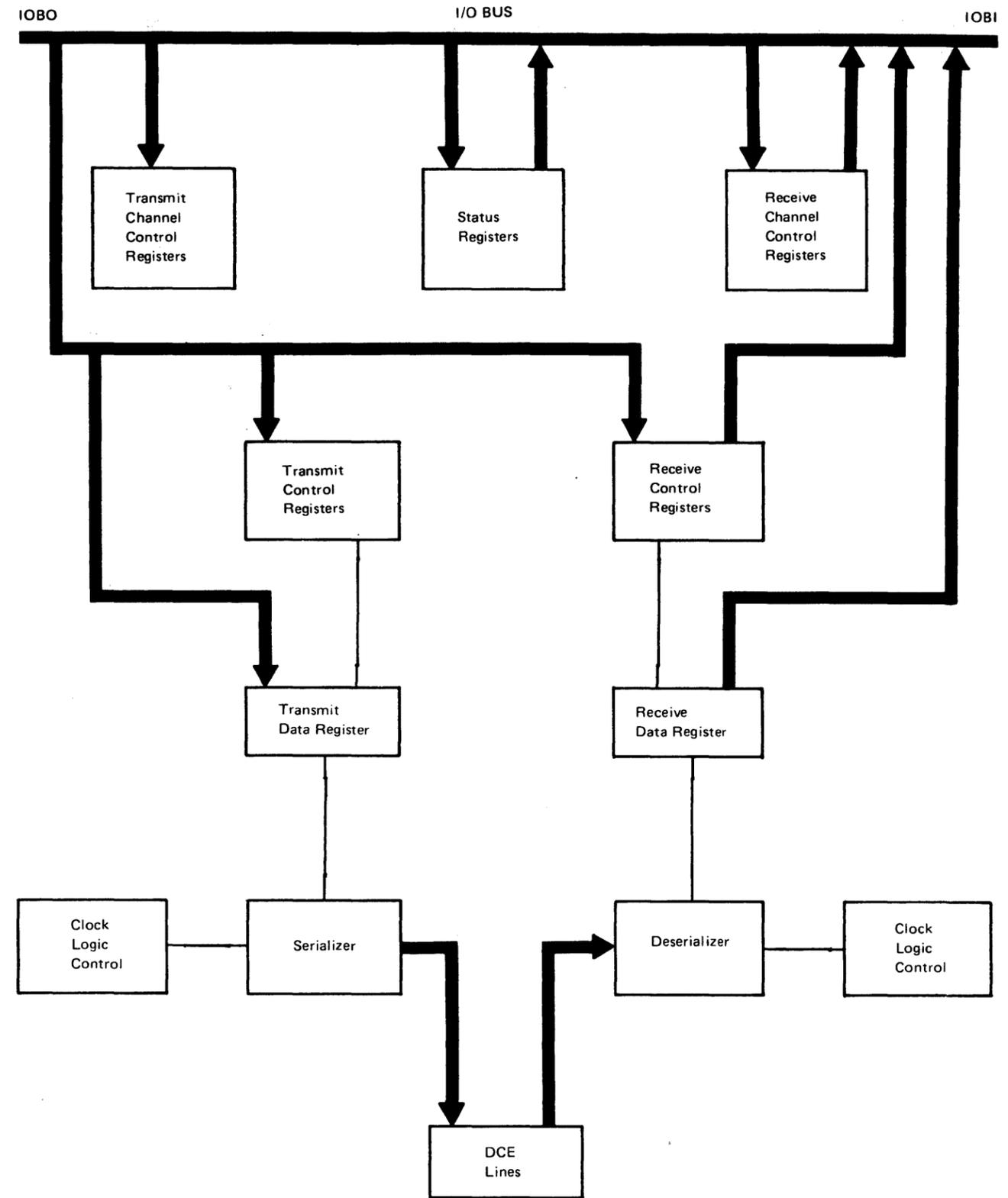
Figure CA451-1. SDLC Adapter Card (CA1) Data Flow
