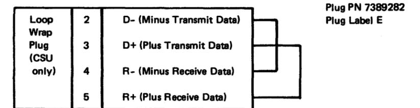
**Figure CA435-2. Loop Wrap Plug (CSU only)**
