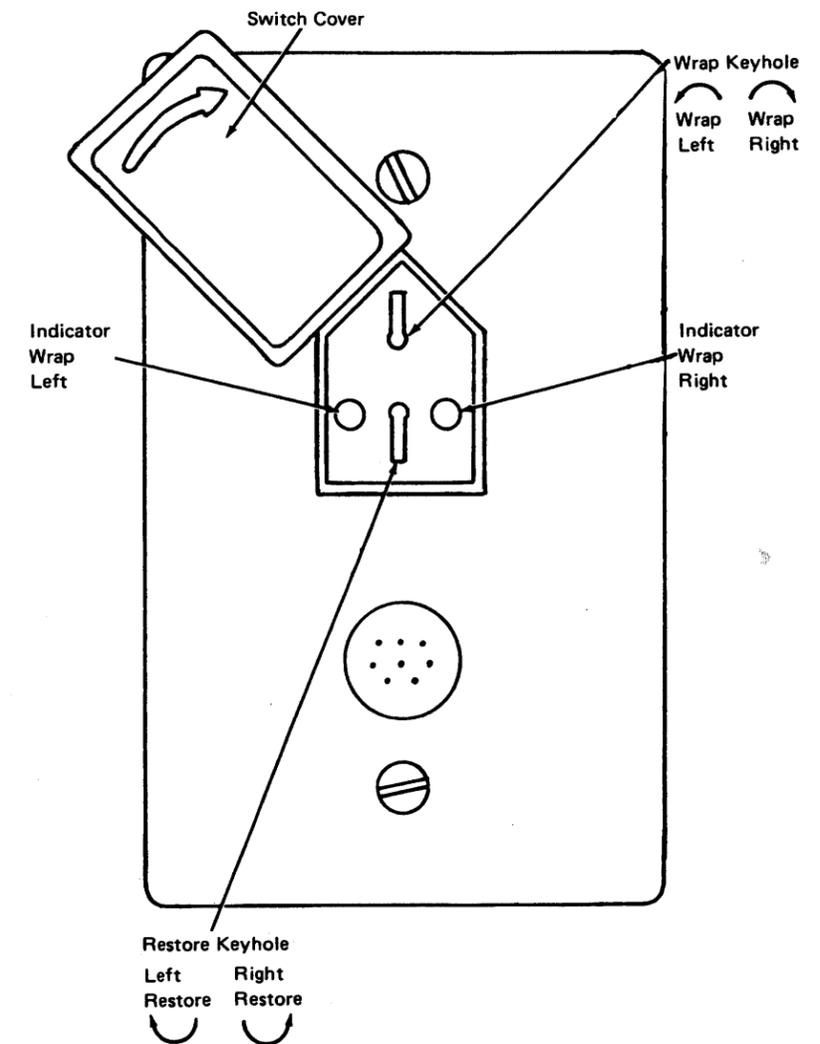
Figure CA561-1. Wrap Operation on Wrap Loop Station Connector
