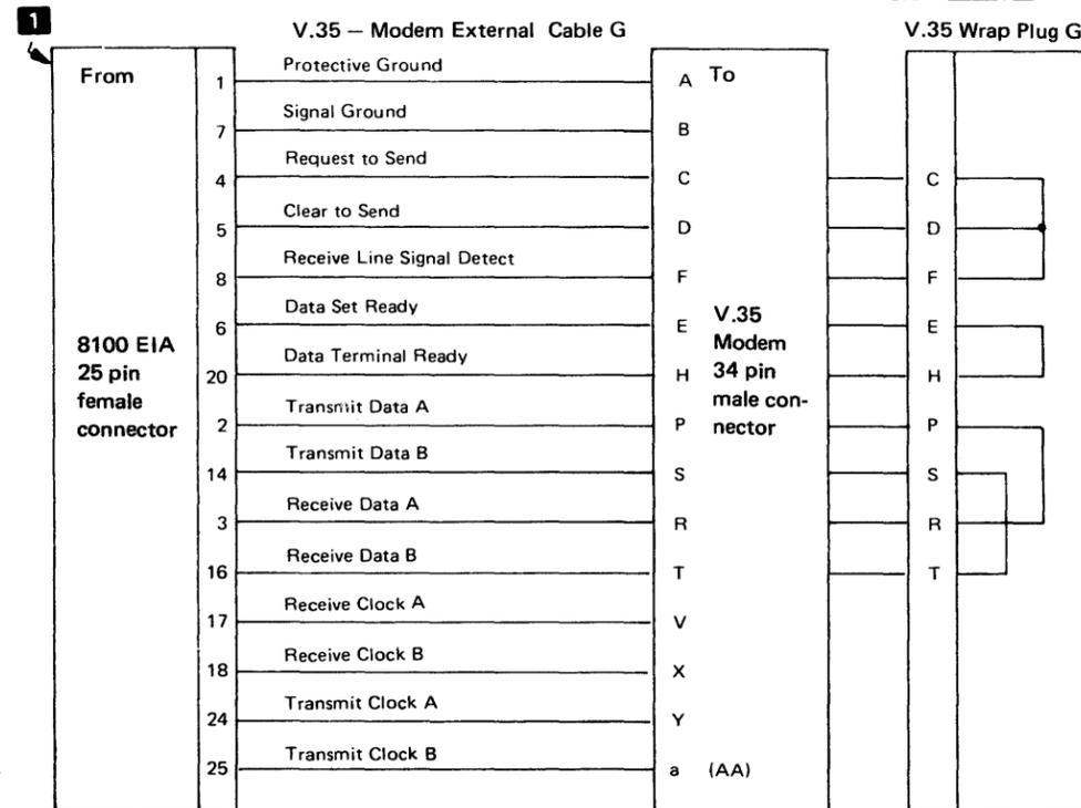
Figure CA545-2. Troubleshooting Diagram for Routine 63, V.35/Modem
