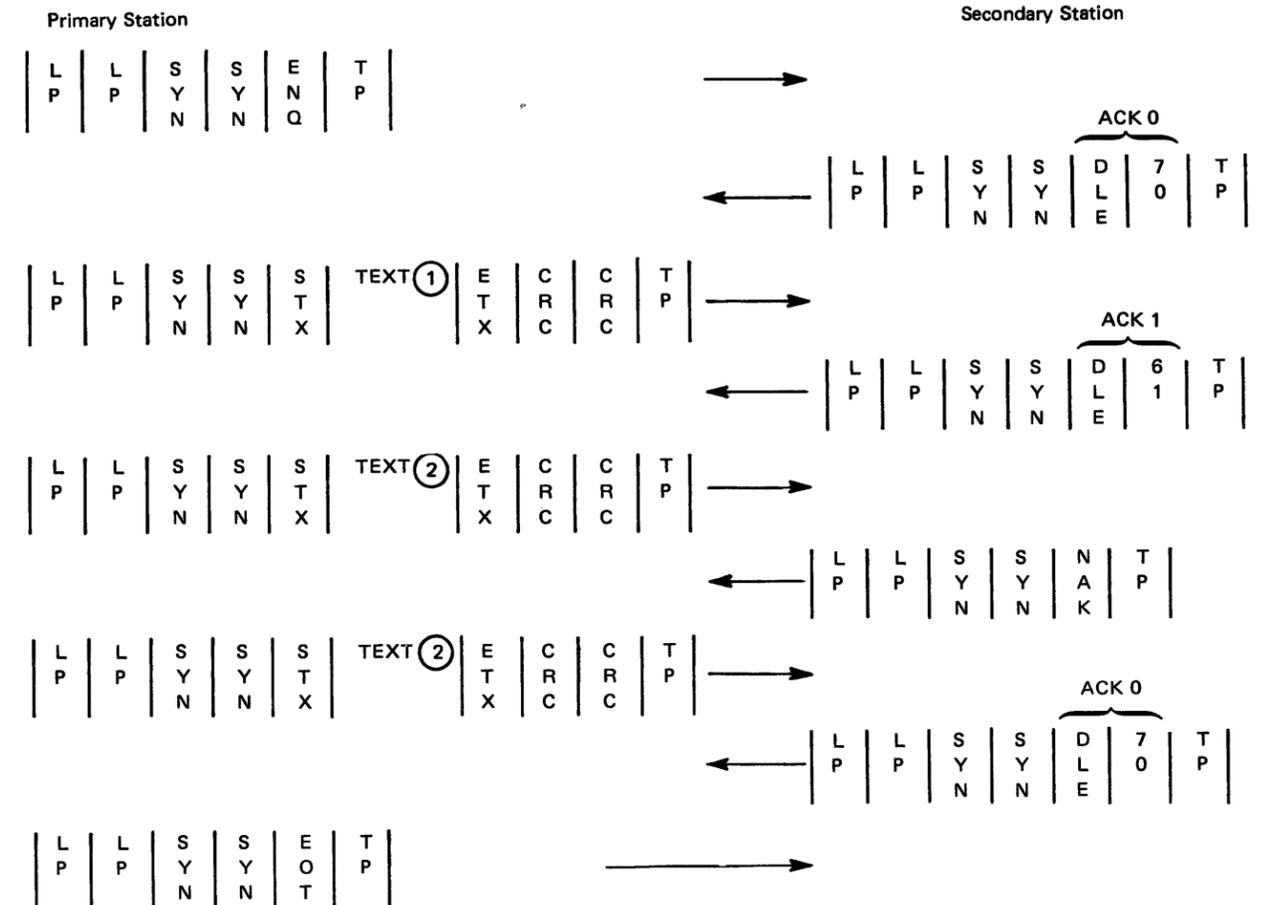
1. The primary station bids for the line by sending "ENQ". Notice framing characters (two leading Pads "LP", two synchronization characters "SYN", and trailing Pad "TP"). All messages will contain the framing sequence.
