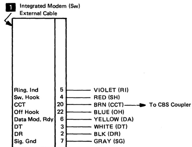
**Figure CA542-2. Troubleshooting Diagram for Routine 20, Switched Integrated Modem**
