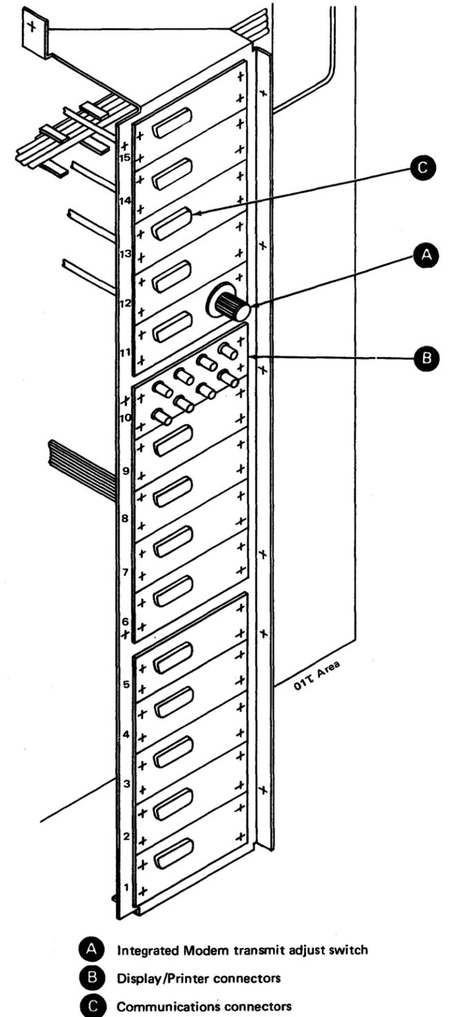
Figure CA423-1. 8140 Model BXX I/O Panel Connections (Rear View)
