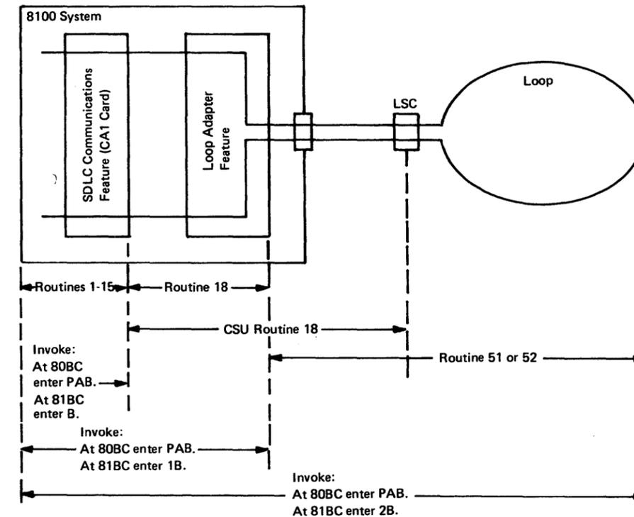
Figure CA202-1. Invocation for a Group of Tests (Level 1 Addressing Only), Loop Feature Example
