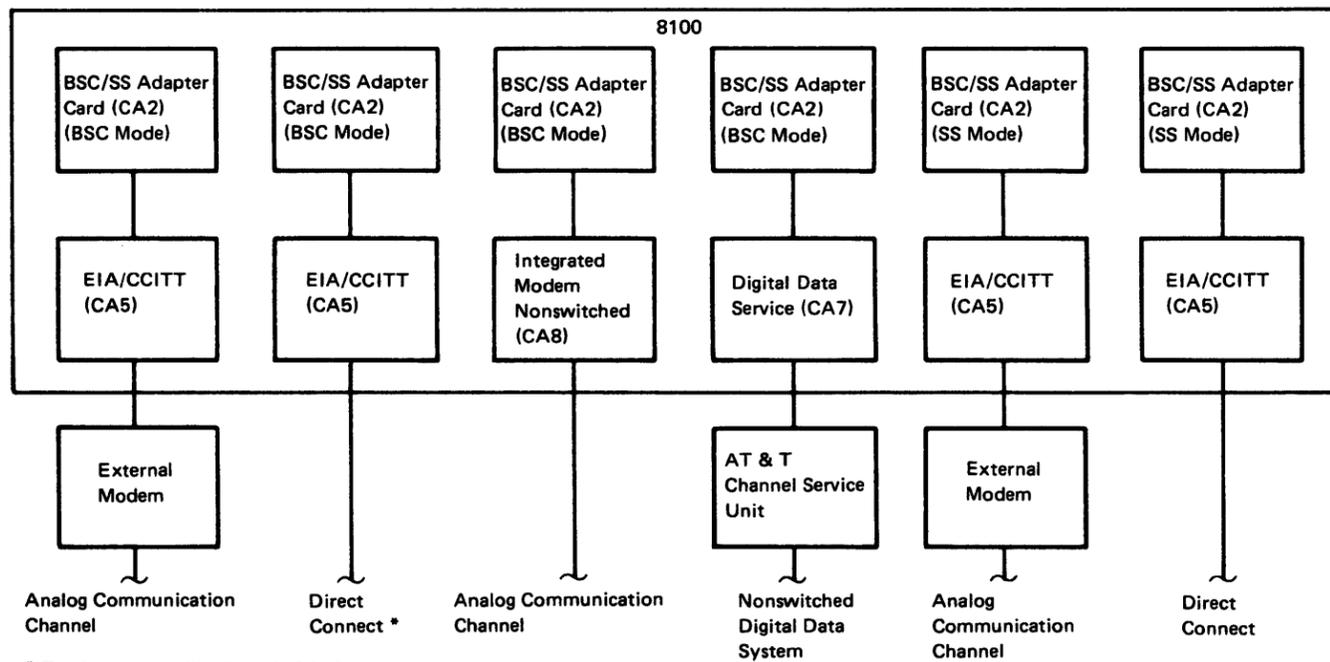
\* The Multispeed Clock card (CA10) is required for direct connect at 4800 bps and 9600 bps.
