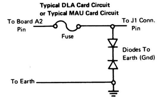
Note: When a 3277 is not attached to the 8100, the modem adapter unit (MAU) and data link adapter (DLA) cards are not used. A cable connects between A-A2Z1 and 01S-J1.
