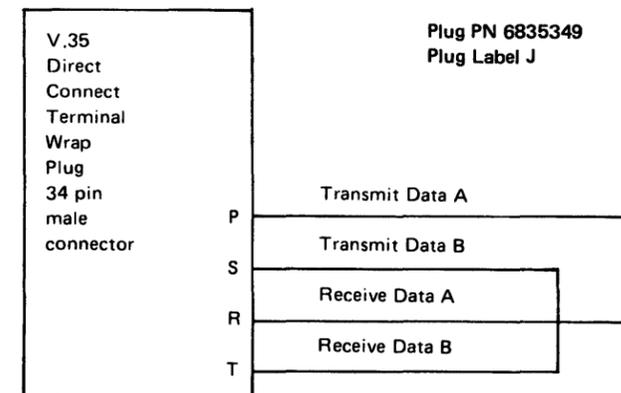
**Figure CA433-2. V.35 Direct-Connect Terminal Cable (CAC6B) and Wrap Plug**
