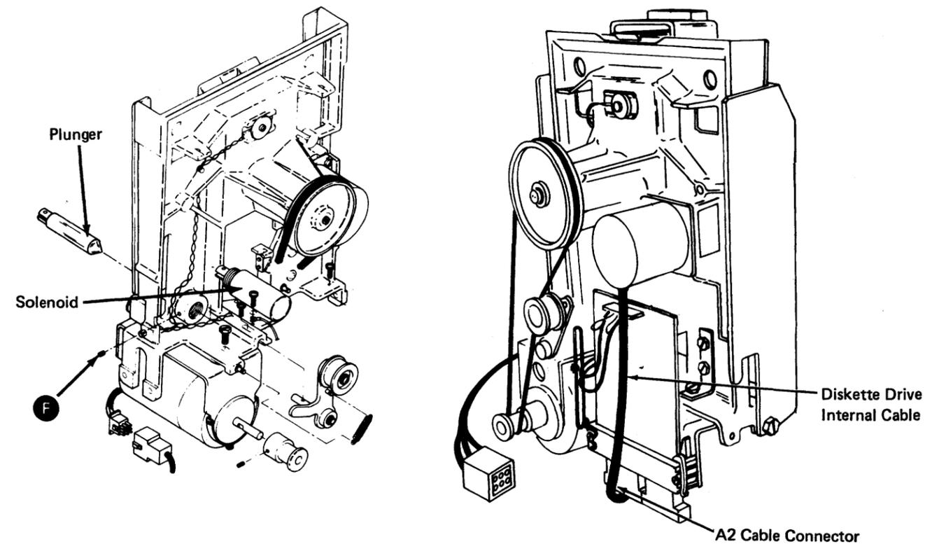
**DA566 Solenoid and Bail Assembly Installation (without Connector Block)**
