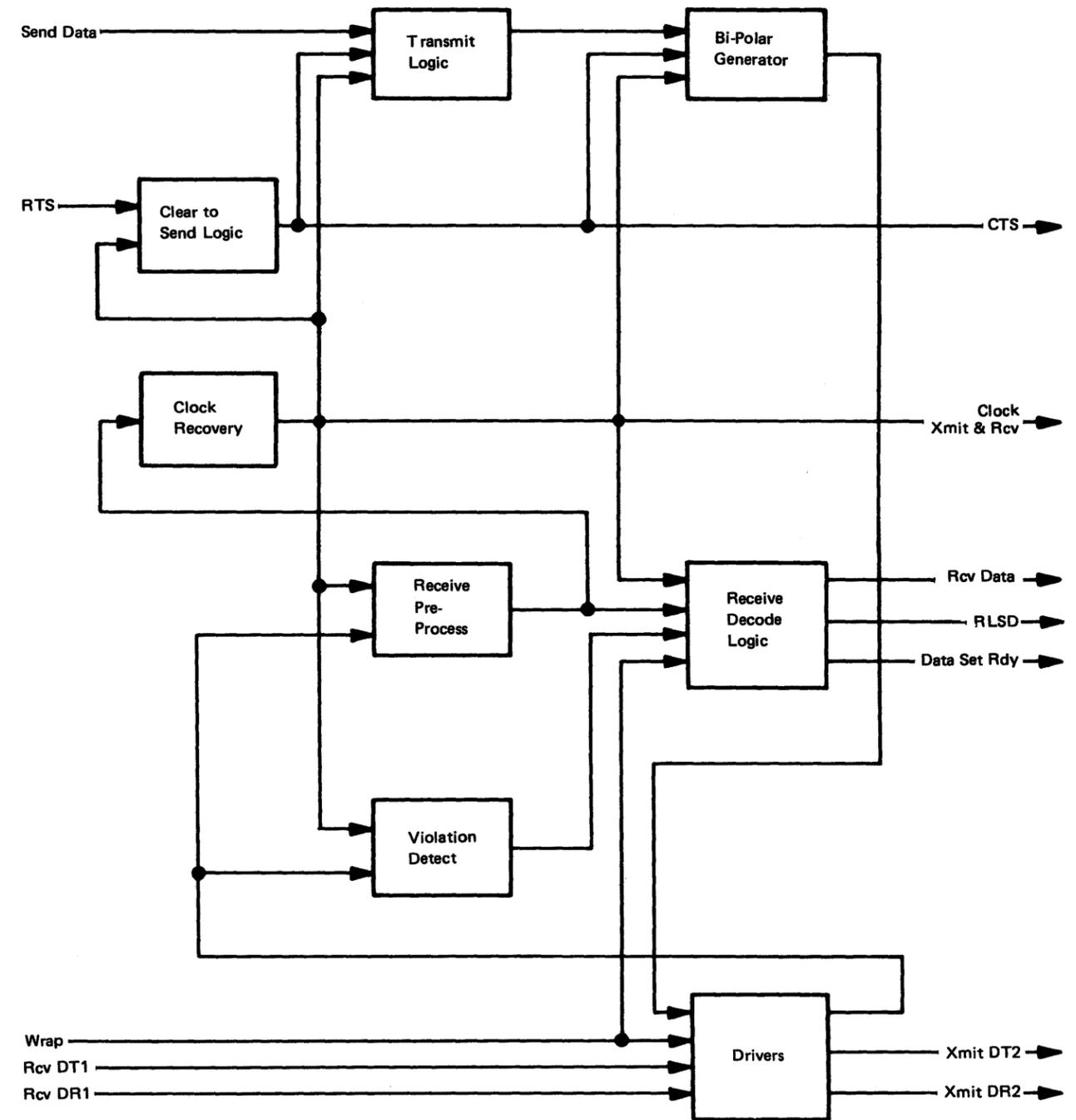
Figure CA471-1. Digital Data Service Card (CA7) Data Flow
