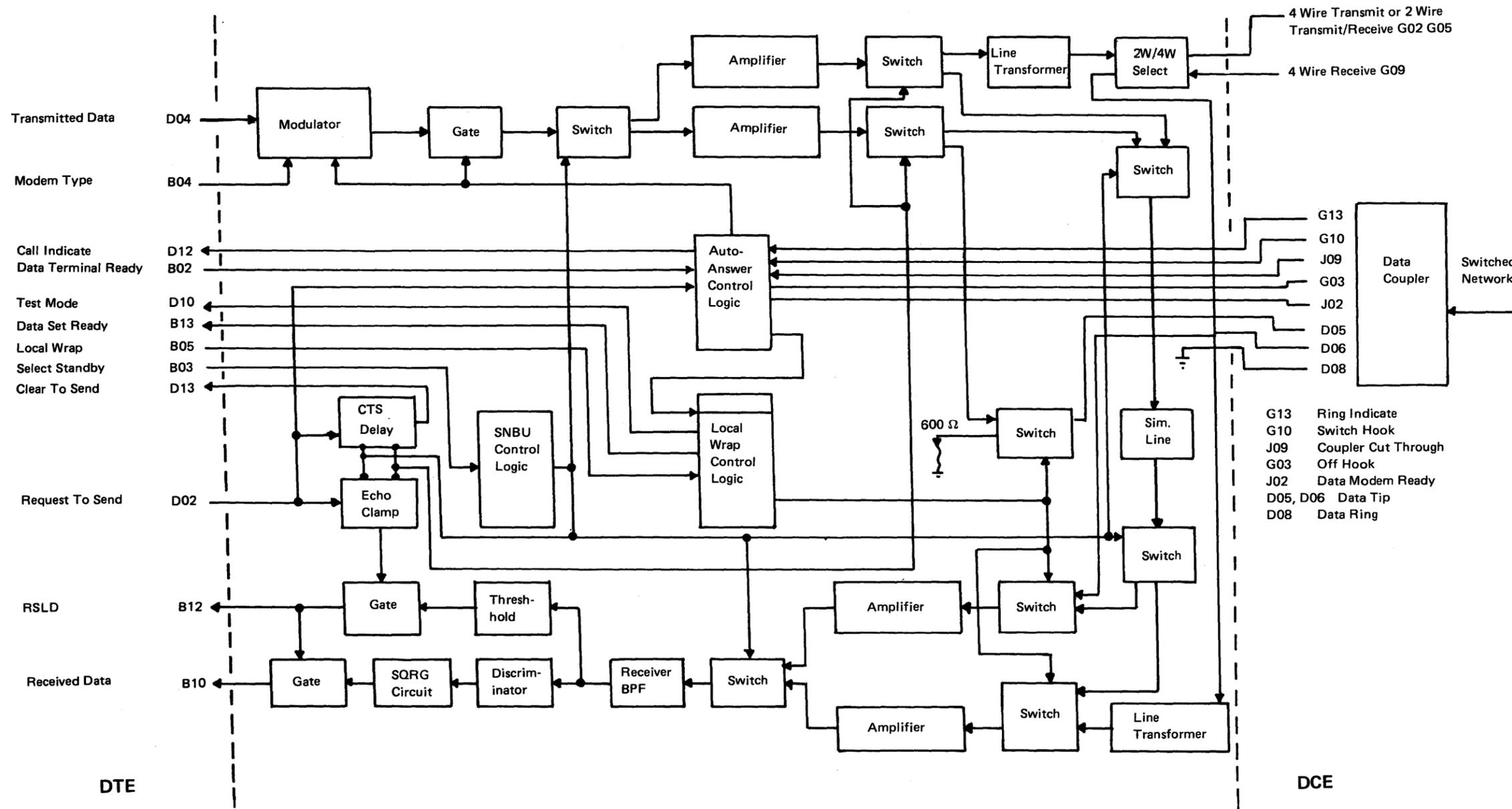
Figure CA473-1. Integrated Modem Card (CA8/CA9) Schematic
