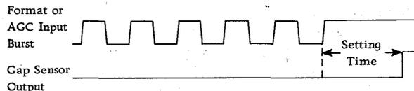
The data gap sensor should not be adjusted on a few random data bits. An AGC burst must be used.
