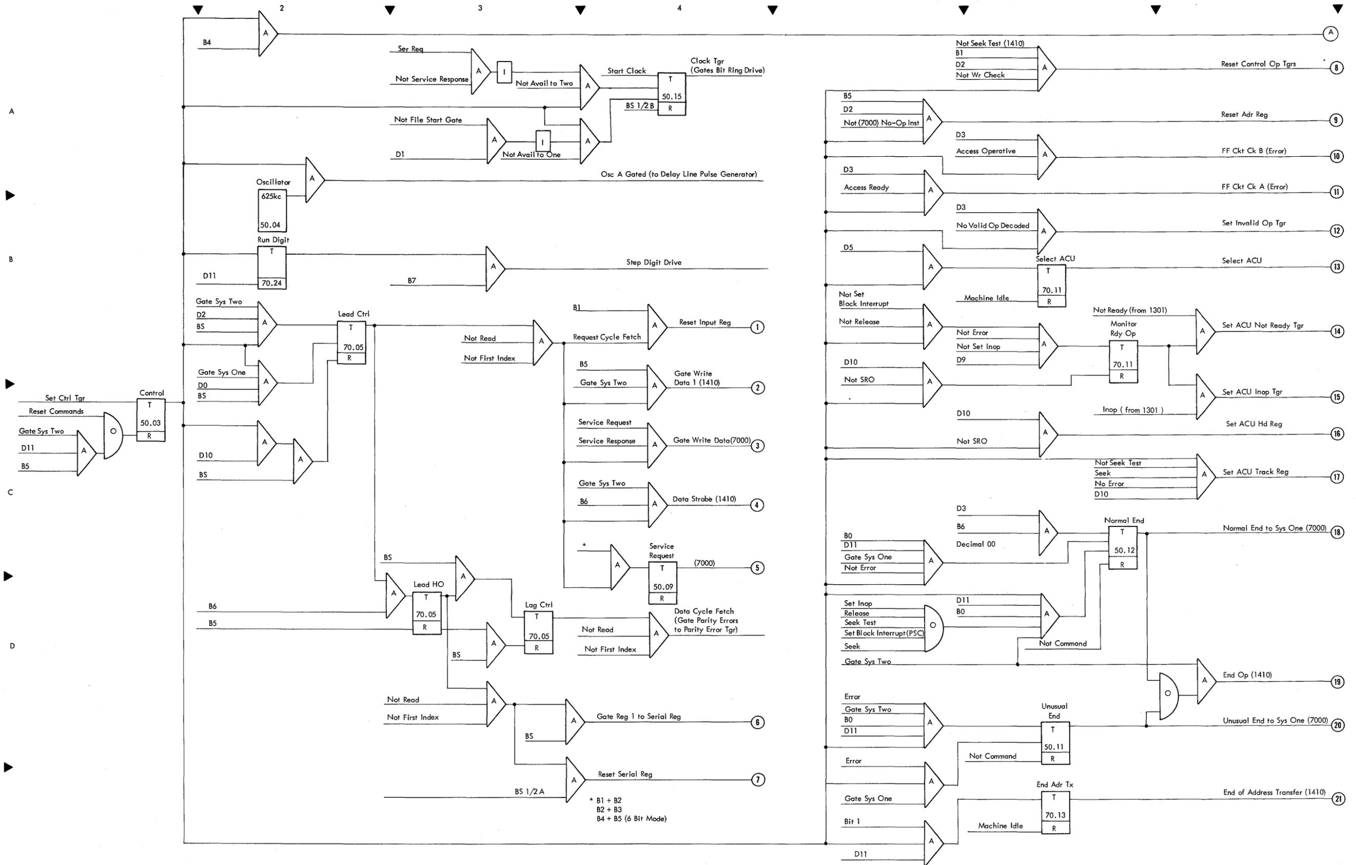
Figure 78. (Sheet 1 of 2). Control Cycle Simplified Logic
