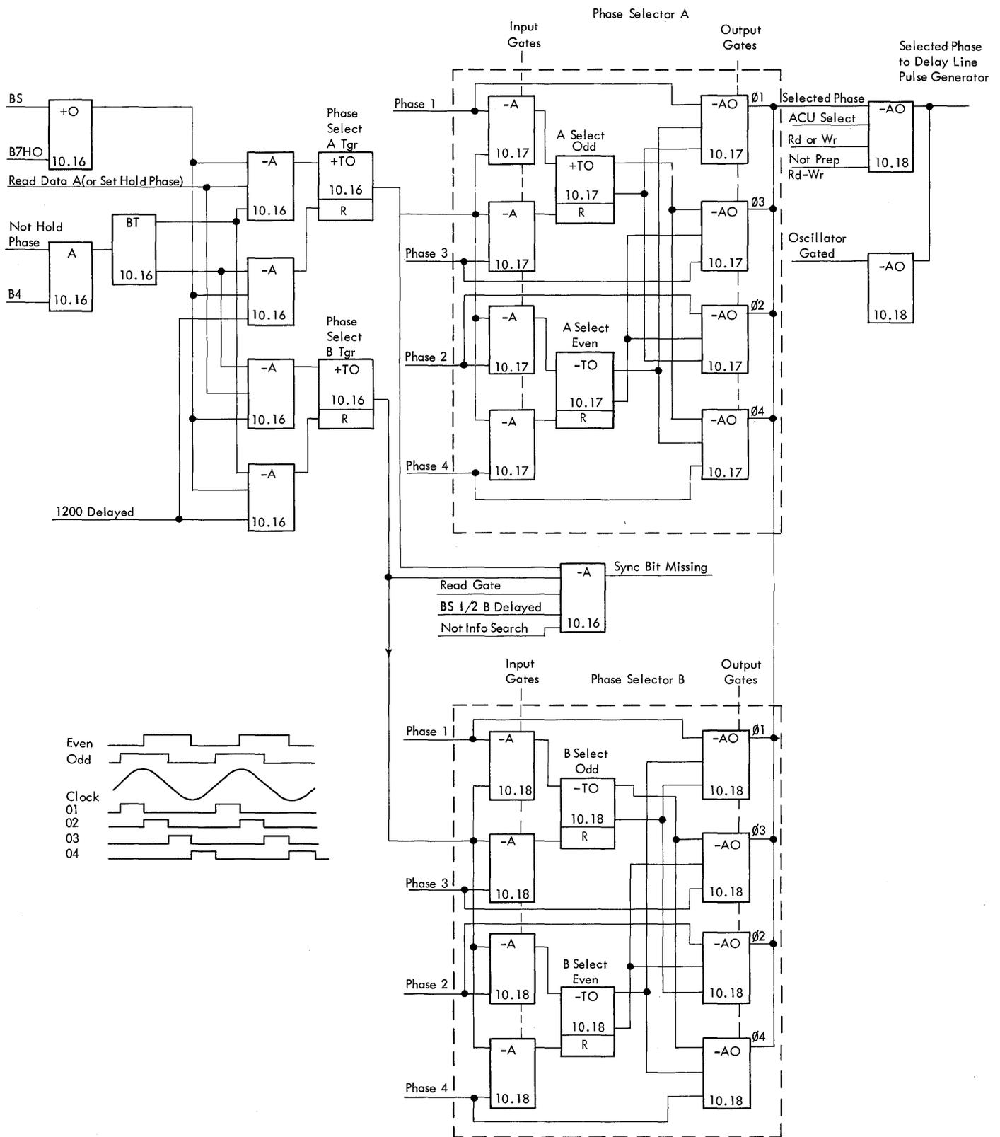
Figure 33. Phase Selector Circuits
