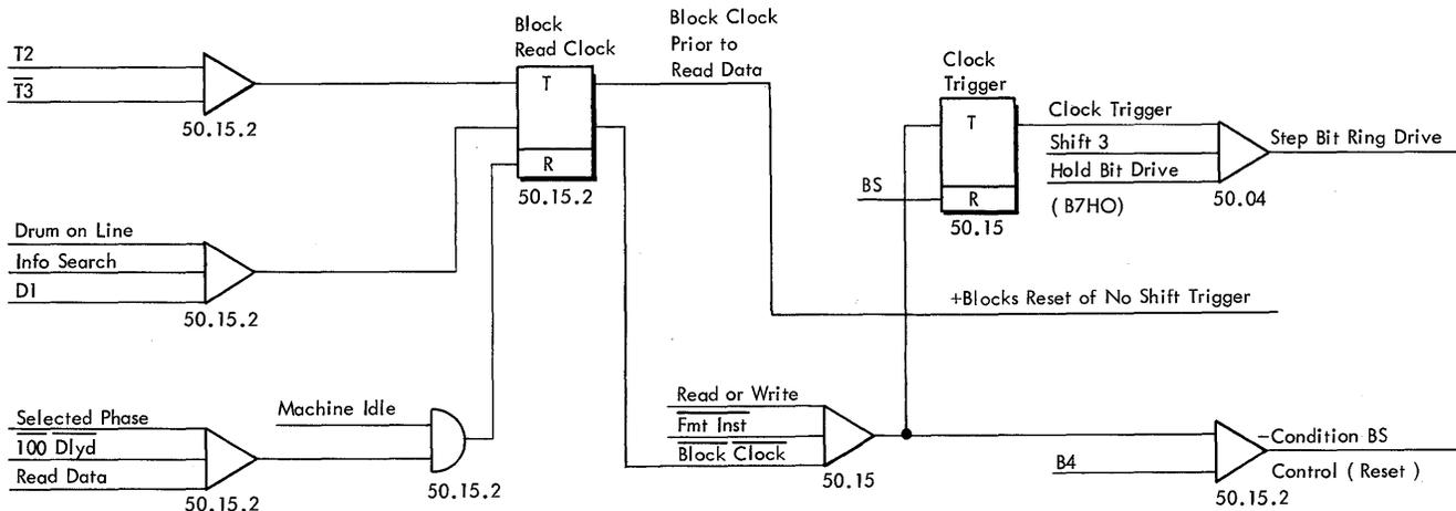
Figure 113. Clock Trigger Control
