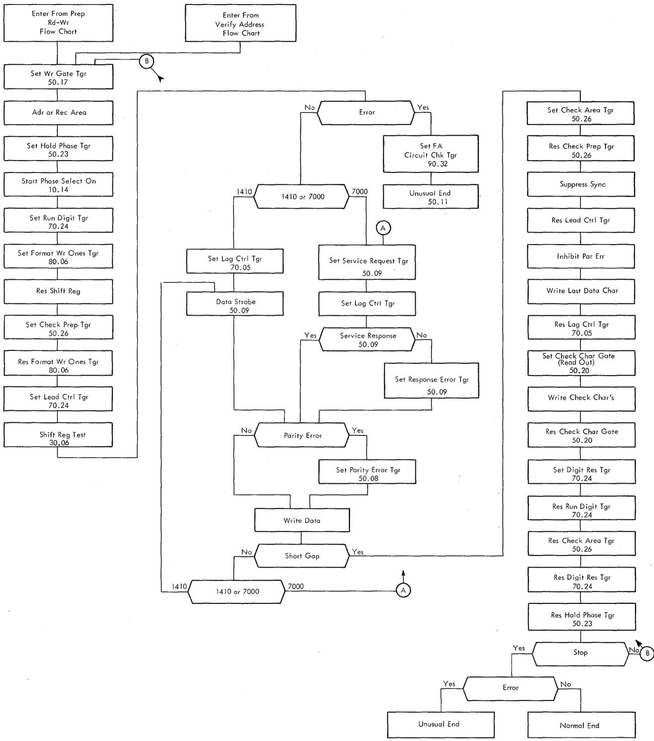
Figure 91. Write Data Cycle Flow Chart
