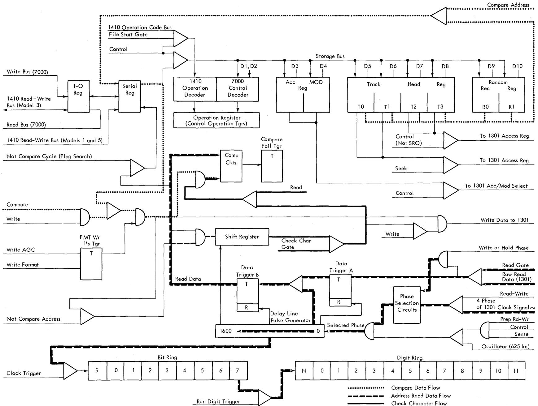
Figure 21. Verify Address Data Flow Diagram
