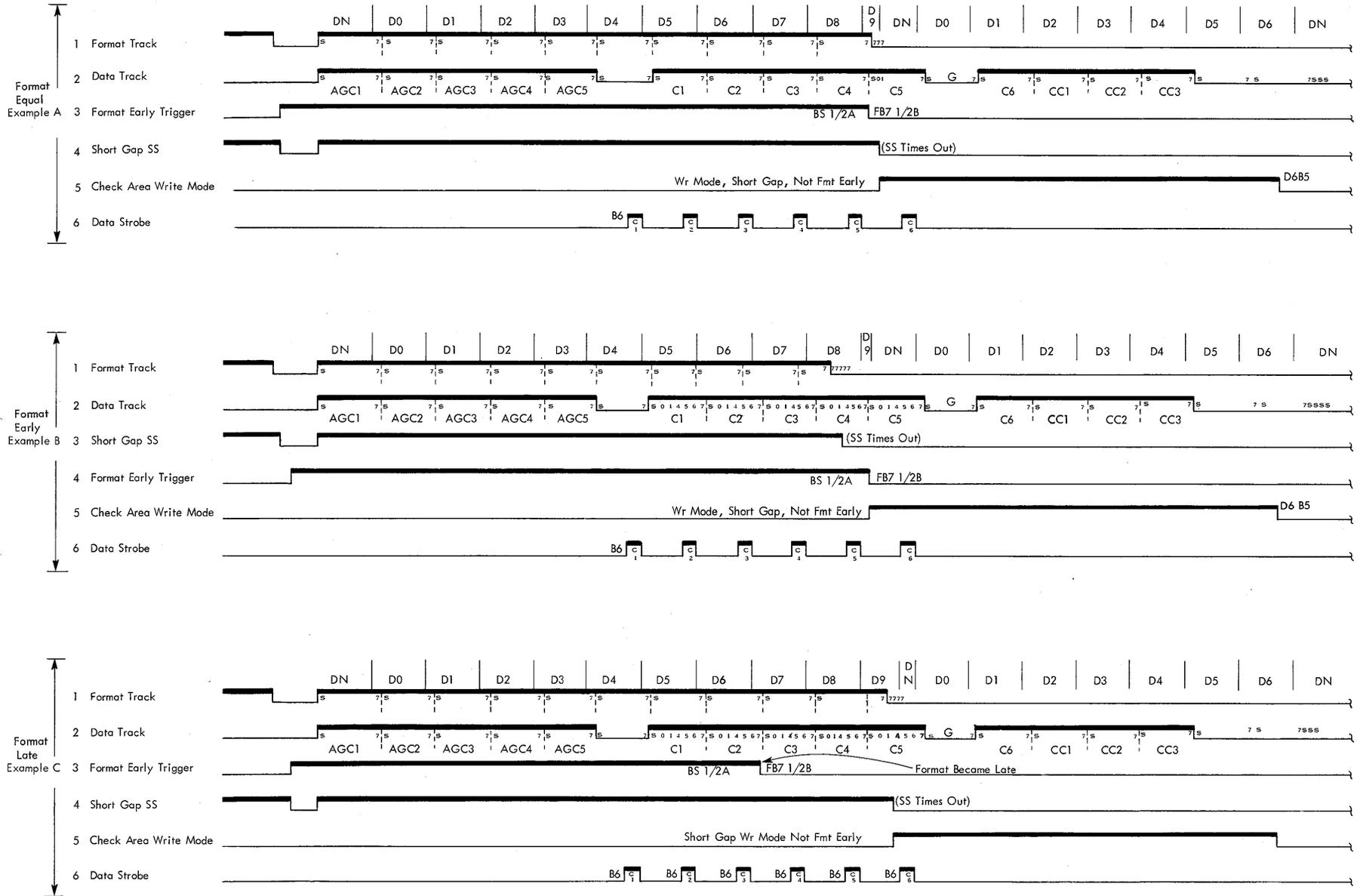
Figure 53. Format Skew Timing
