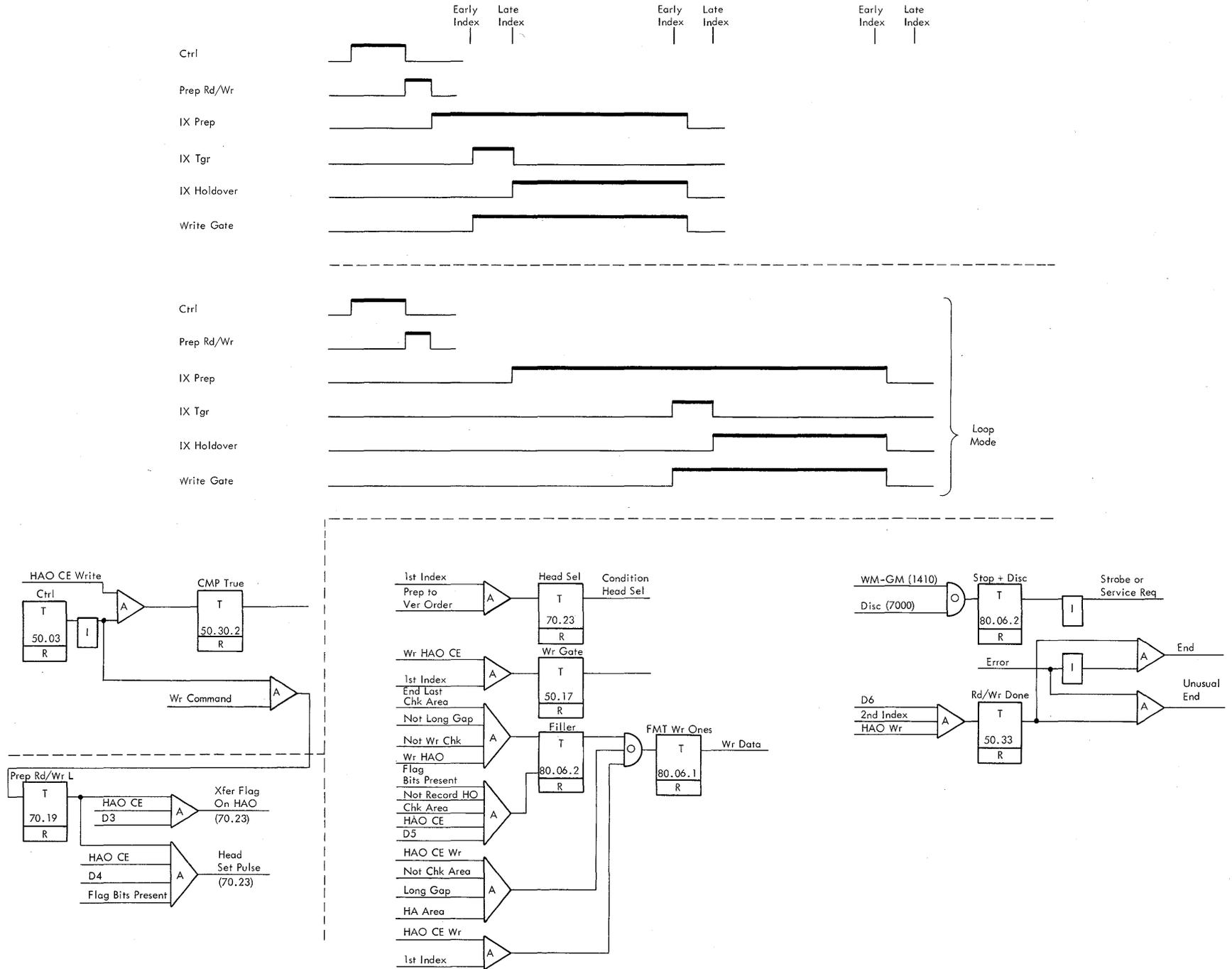
Figure 97. HAO-CE Write Sequence and Simplified Logic
