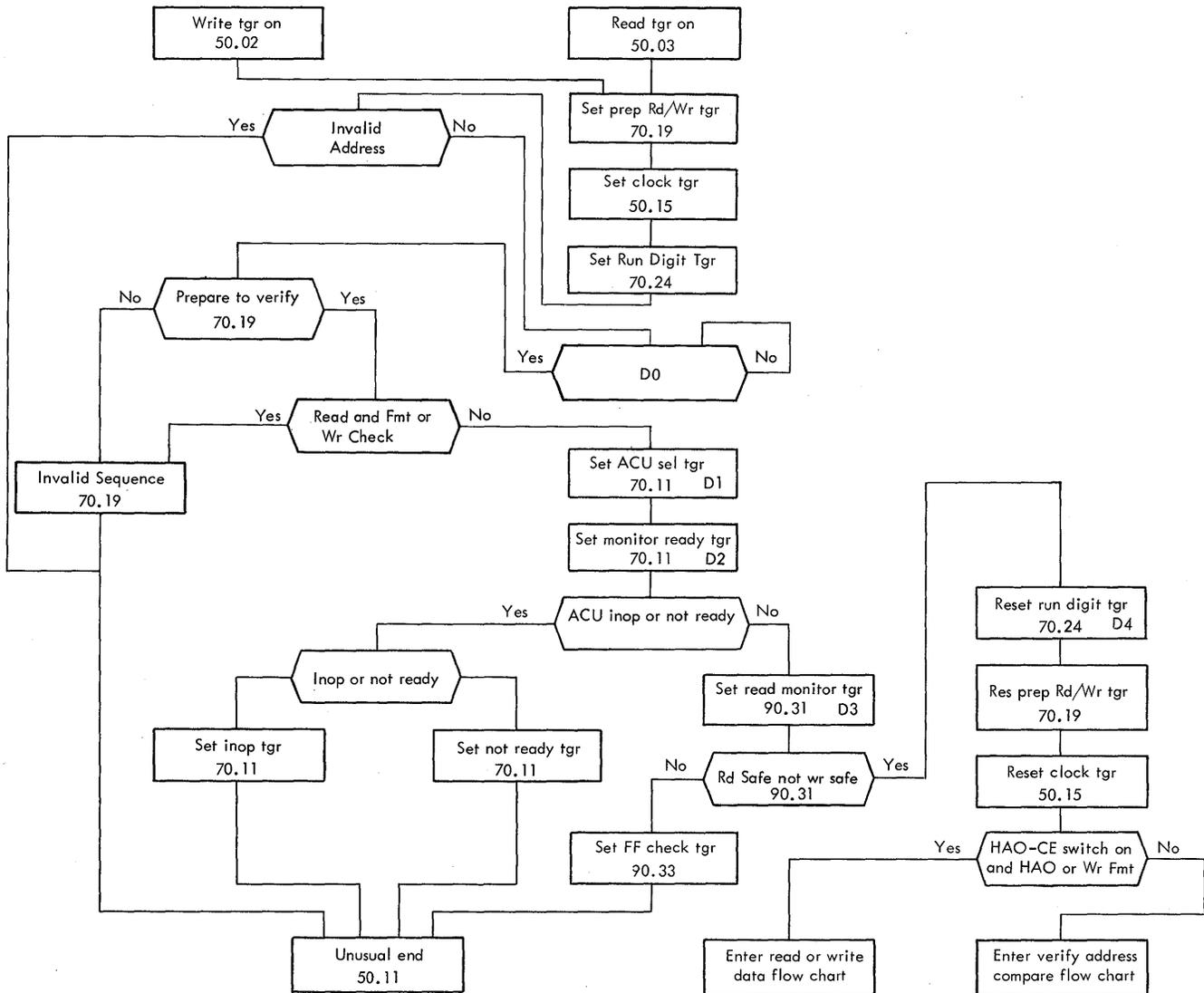
Figure 84. Prep Read-Write Cycle Flow Chart
