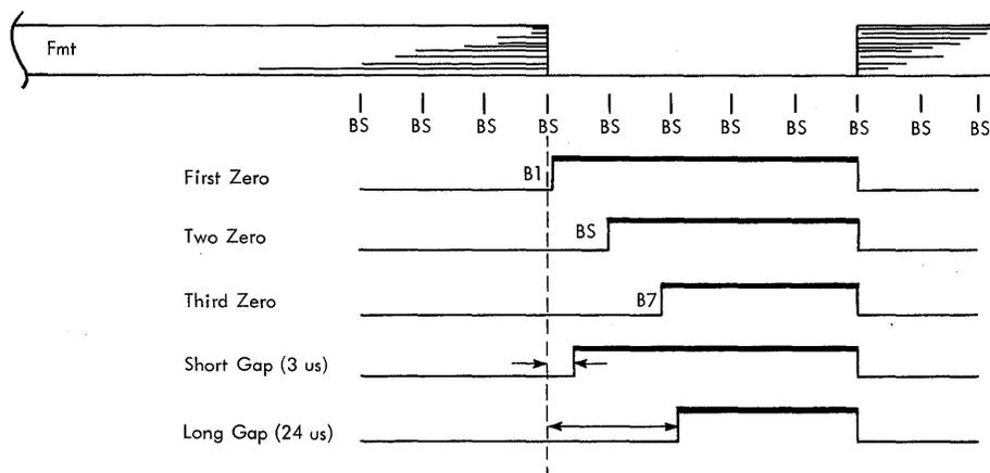
Figure 105. Format Write Check Simplified Logic
