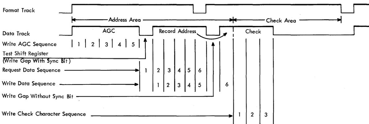
Figure 24. Write Data Sequence-Record Address
