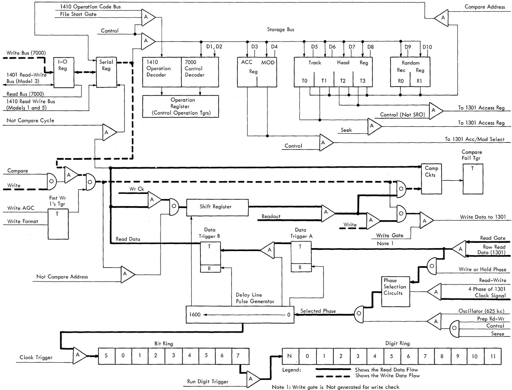
Figure 102. Write Check Data Flow Diagram
