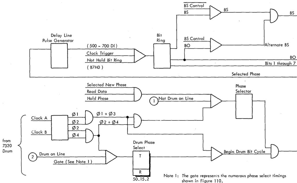
Figure 109. Phase Pulse Generation and Bit Ring Control
