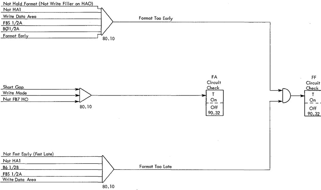
Figure 54. Format Skew Errors
