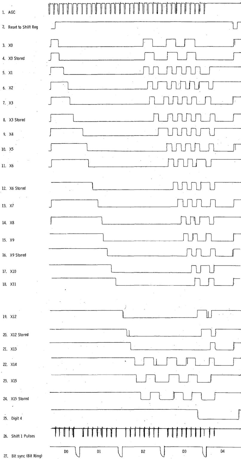
Figure 122. Shift Register Test Eight-Bit Mode
