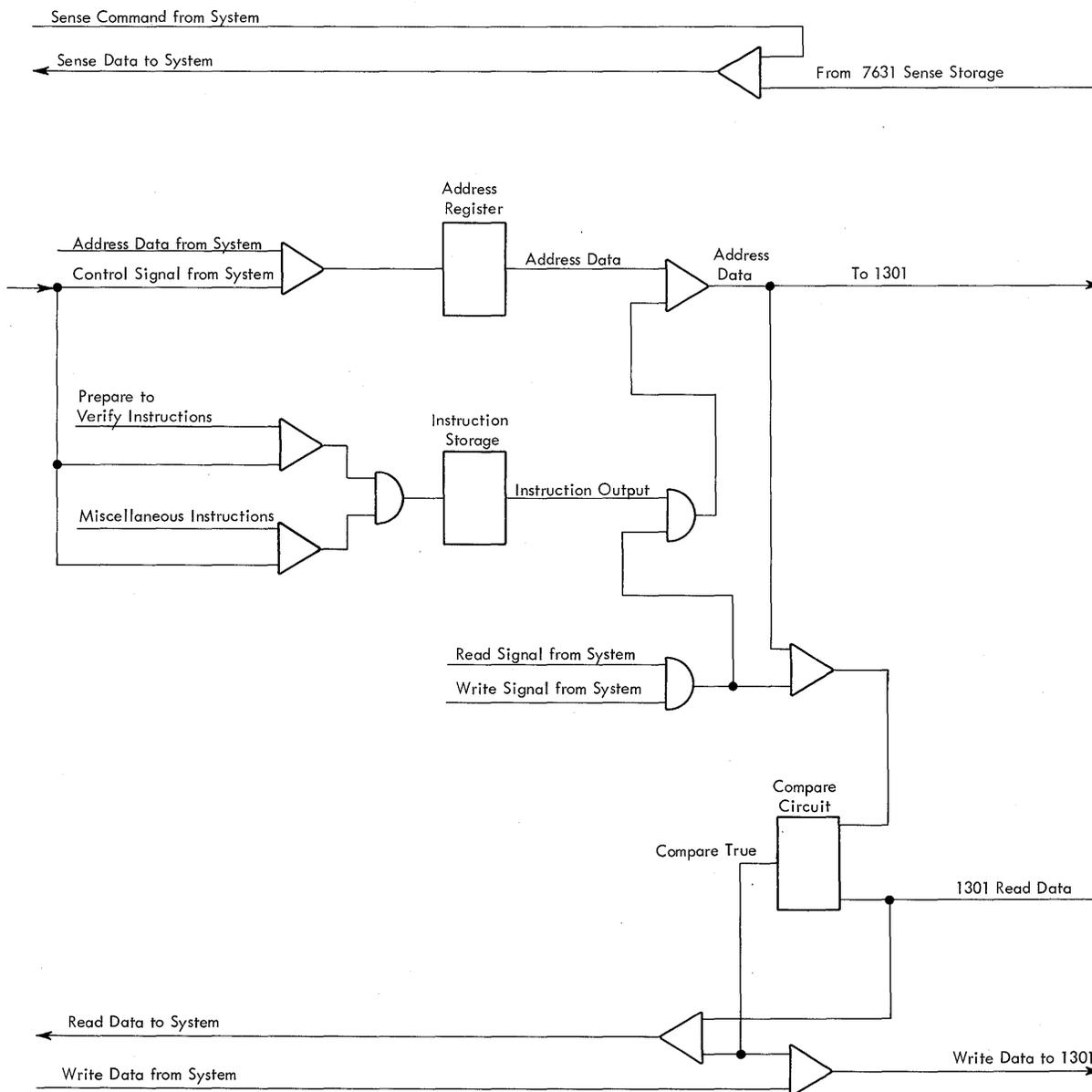
Figure 4. 7631 File Control Simplified Operations
