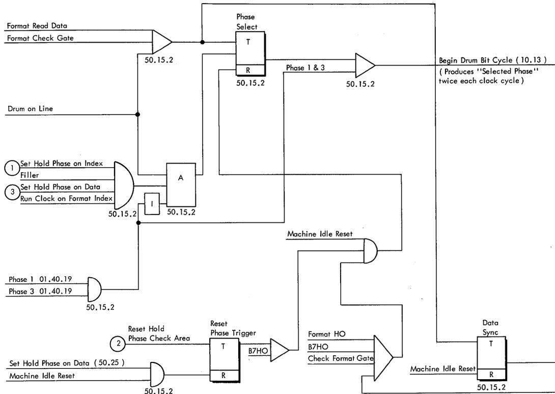
Figure 110. Drum Phase Pulse Control
