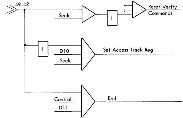
Figure 69. (Sheet 2 of 6). 1410-7631 File Control Interface Logic
