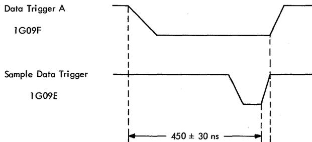
Figure 118. Read Delay Adjustment
