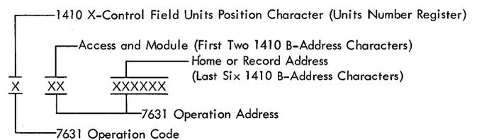
Figure 13. 1410 System Control Data for 7631
