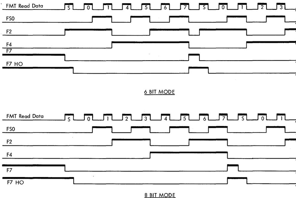
Figure 56. Format Binary Counter Timing
