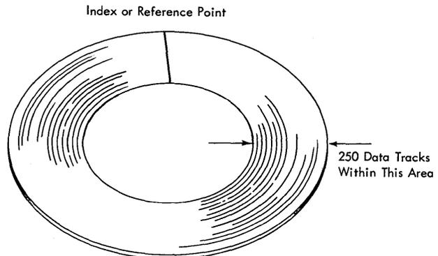
Figure 5. Magnetically Coated Disk
