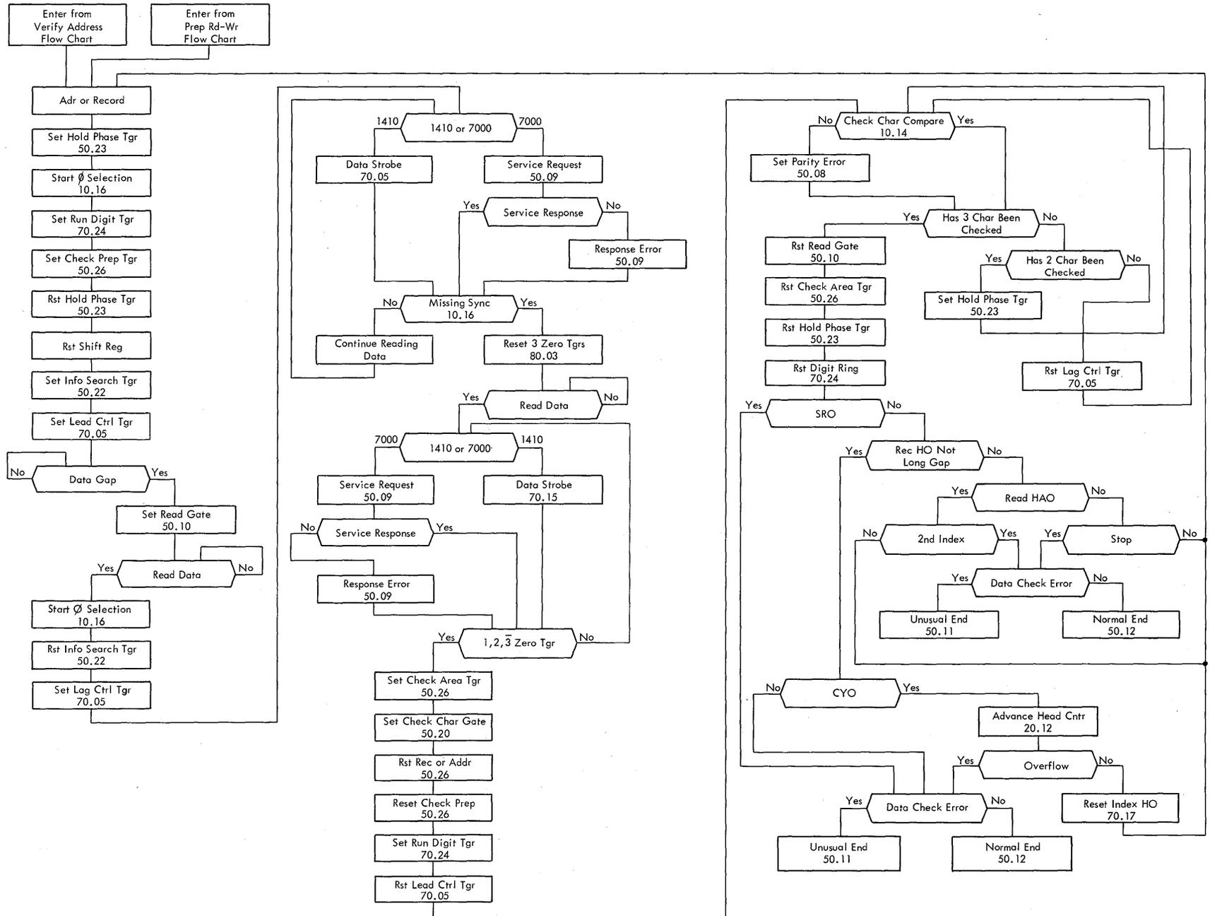
Figure 89. Read Data Cycle Flow Chart
