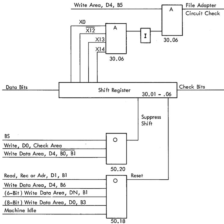
Figure 44. Shift Register Controls
