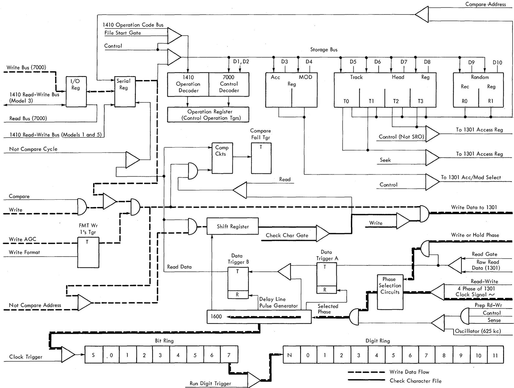
Figure 25. Write Data Flow Diagram.
