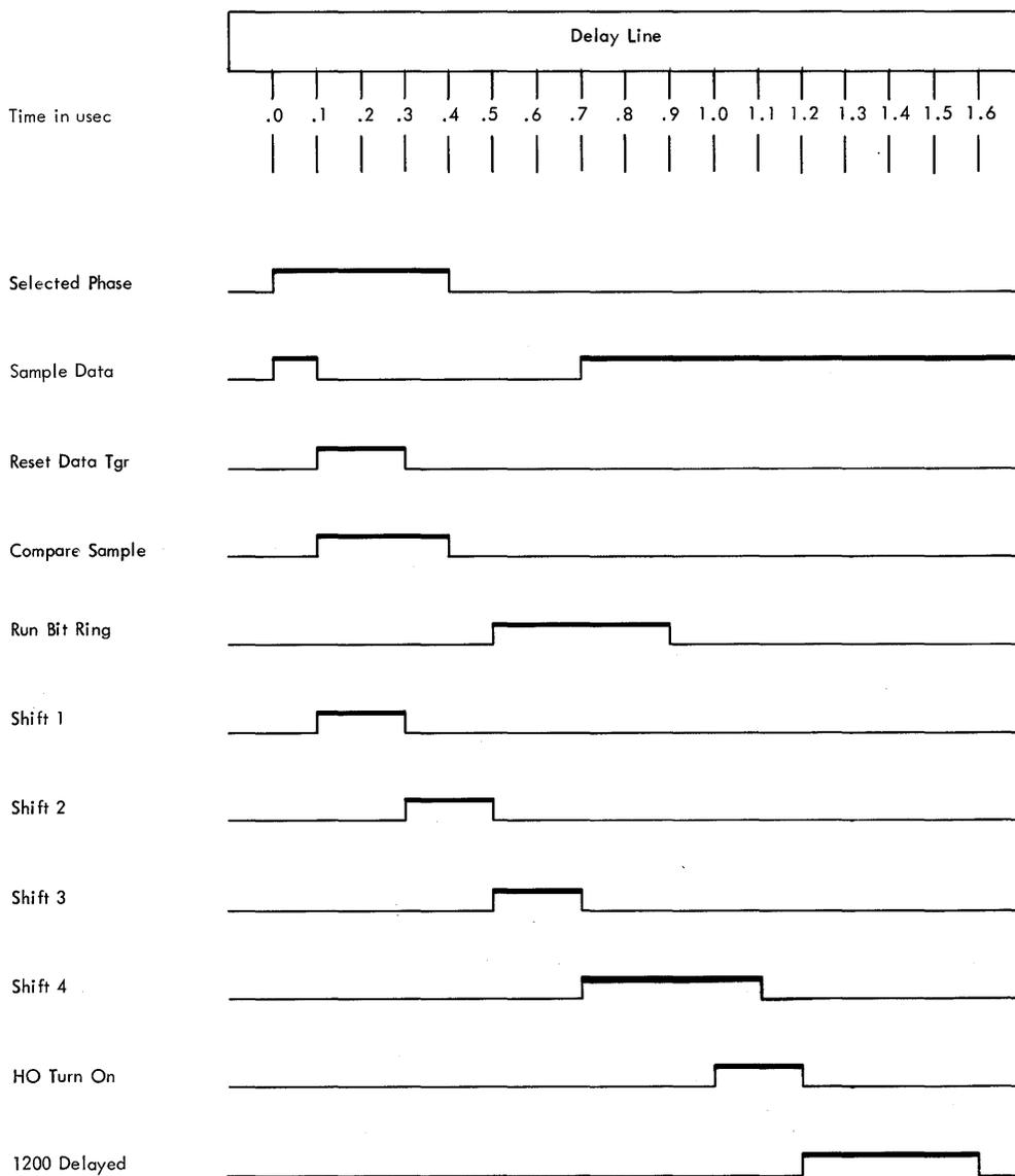
Figure 36. Delay Line Pulse Generator Timing
