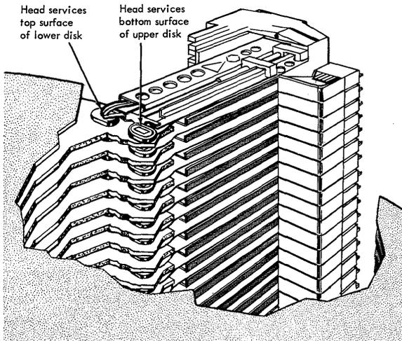
Figure 8. Read-Write Comb
