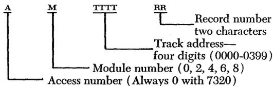
The drum unit is addressed as access 0 because multiple accesses are not meaningful with the drum. A circuit check is made to insure the use of access zero only.
