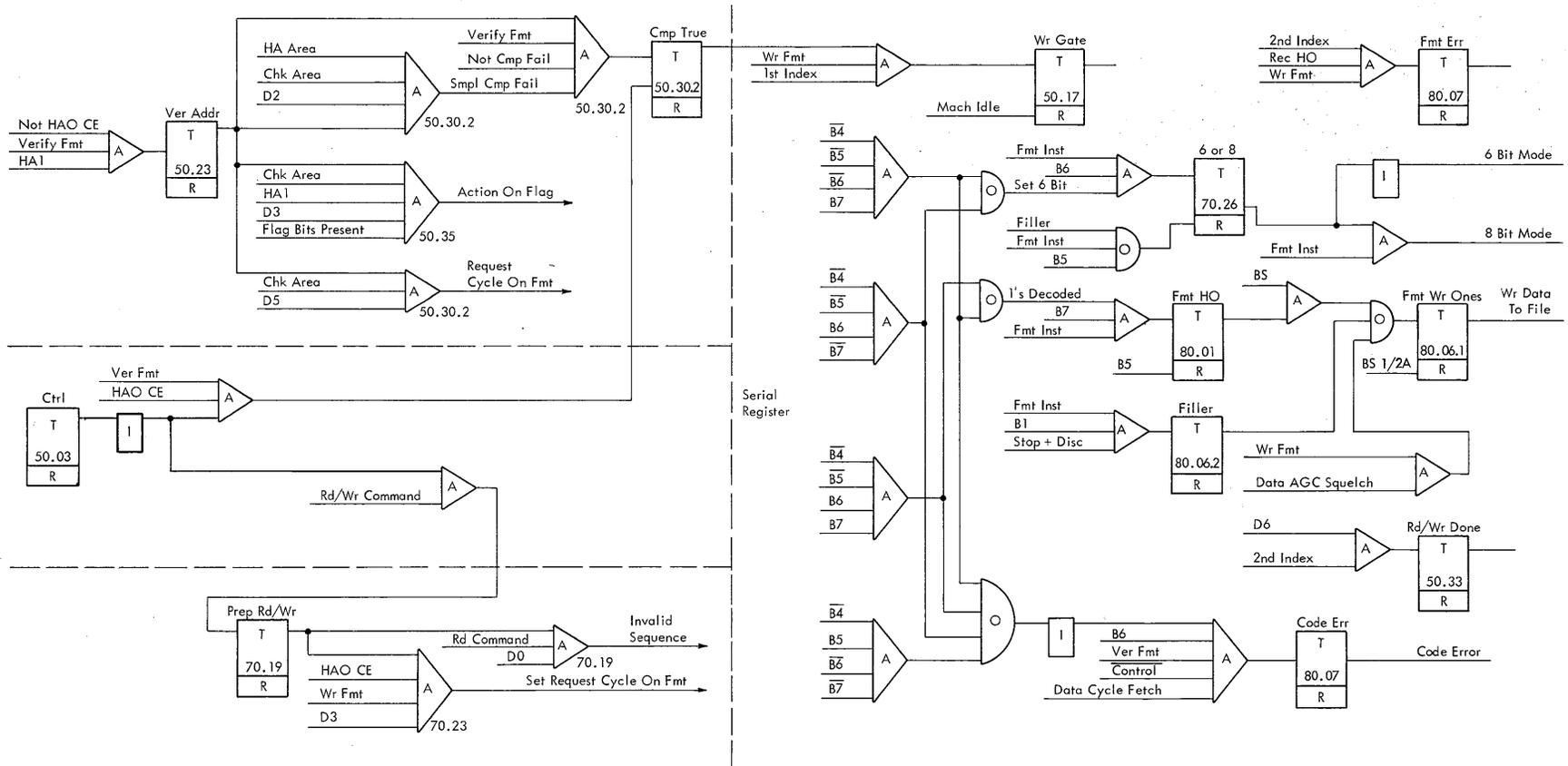
Figure 100. Format Write Sequence and Simplified Logic
