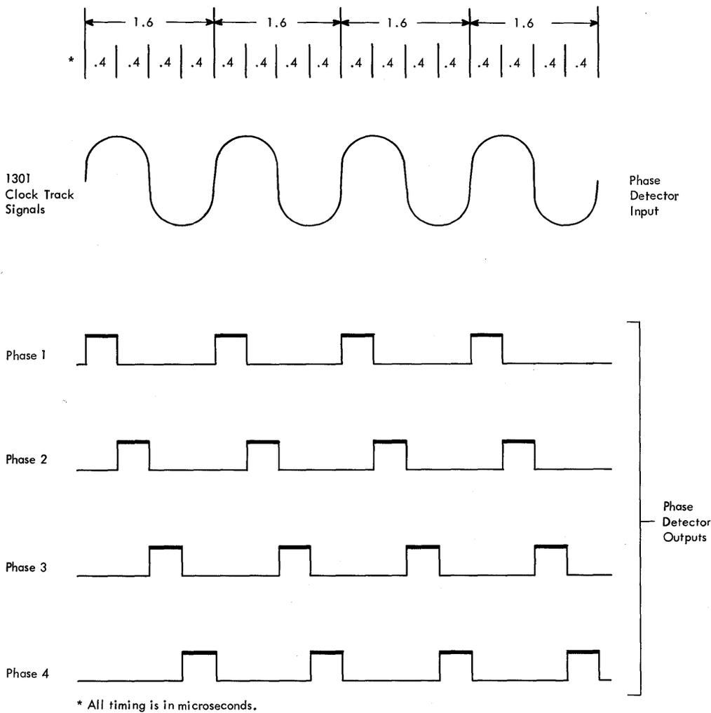
Figure 32. Phase Detector Inputs and Outputs
