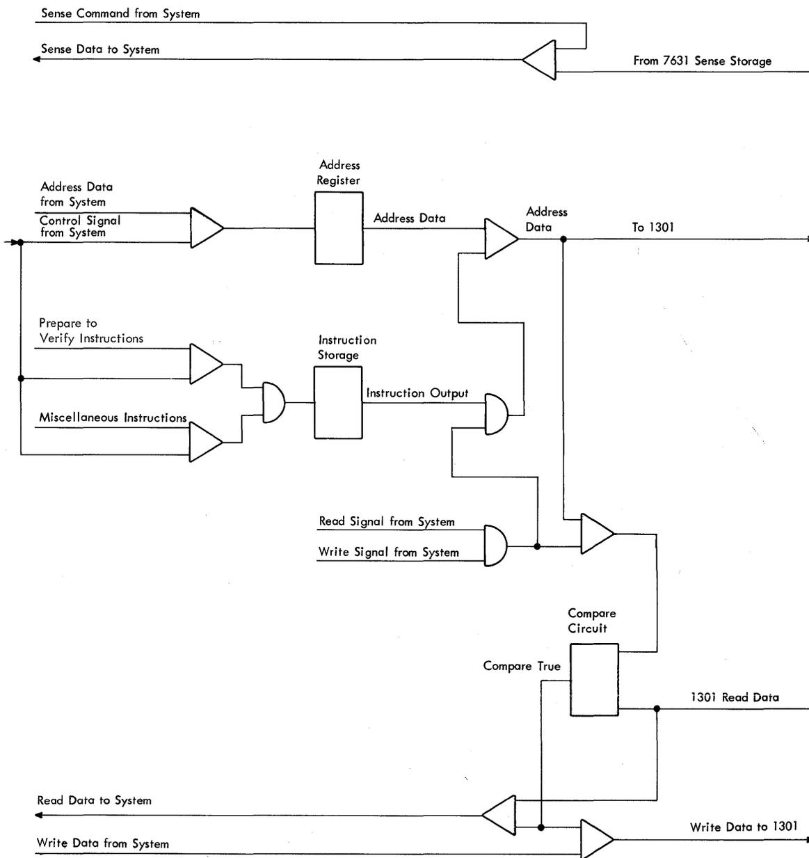
Figure 14. 7631 File Control Simplified Operations
