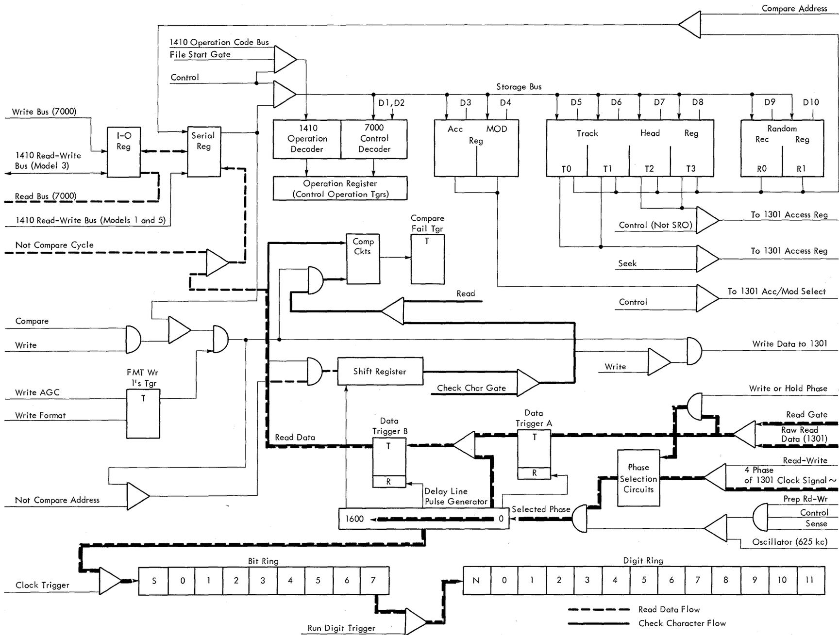
Figure 23. Read Data Flow Diagram
