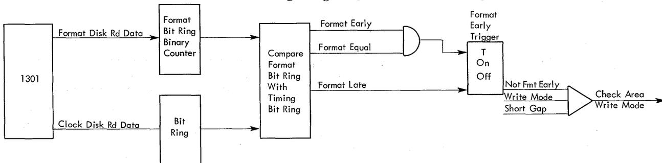
Figure 51. Format Skew Detection Circuits
