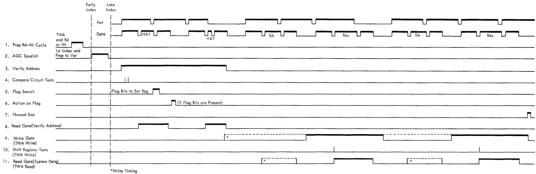
Figure 93. TWA Read and Write Sequence
