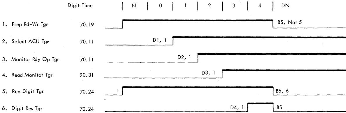
Figure 83. Prep Read-Write Cycle Timing
