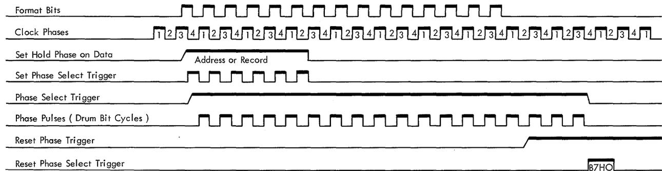
Figure 116. Read-Write Select Phase Pulses
