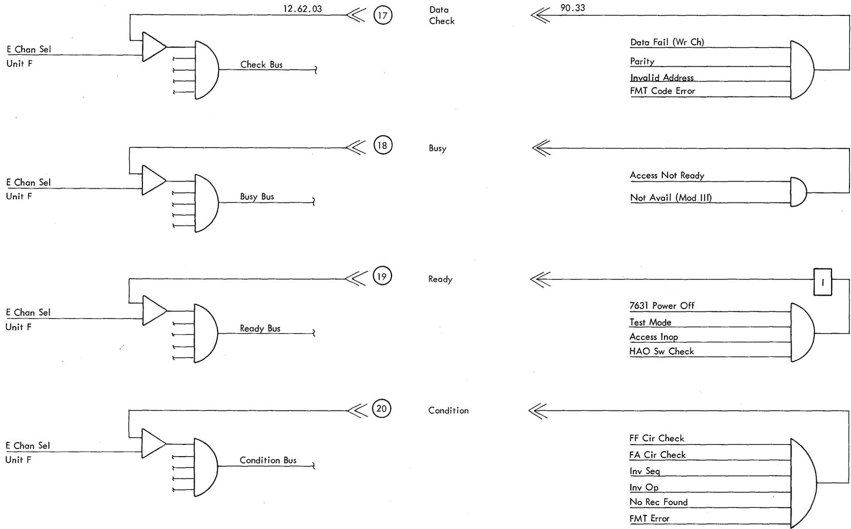
Figure 69. (Sheet 6 of 6). 1410-7631 File Control Interface Logic
