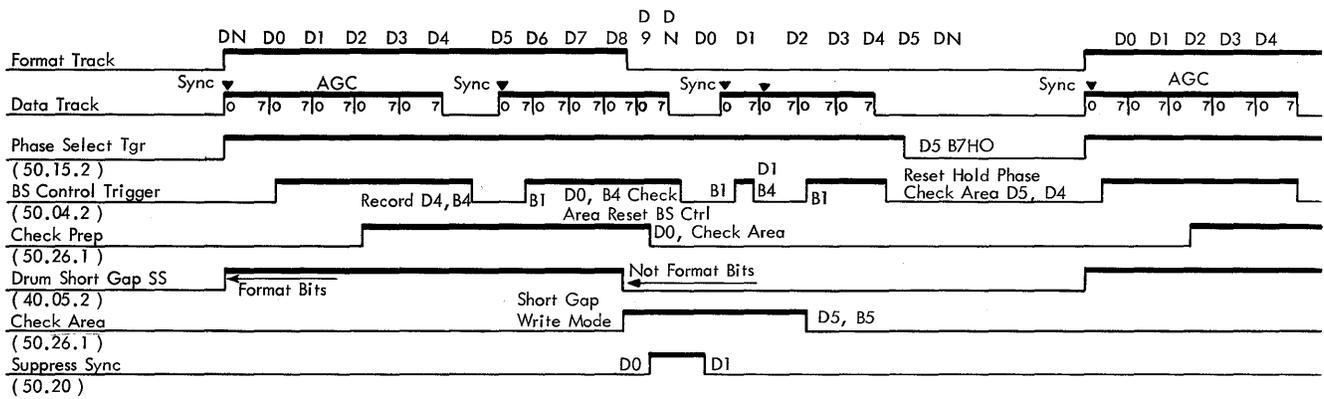
Figure 115. Drum Write Sequence
