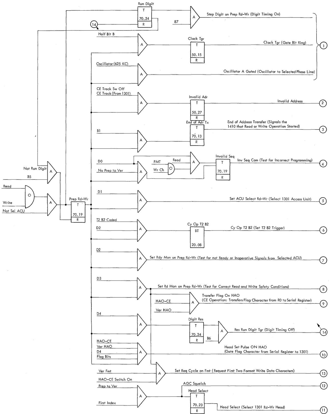
Figure 19. Prep Read-Write Cycle Simplified Logic
