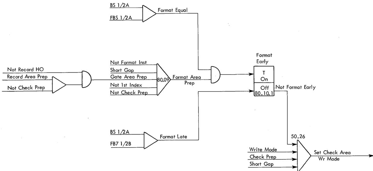
Figure 52. Format Skew Detector
