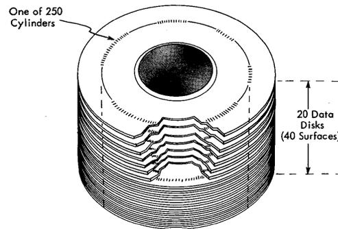
Figure 10. Cylinder Concept
