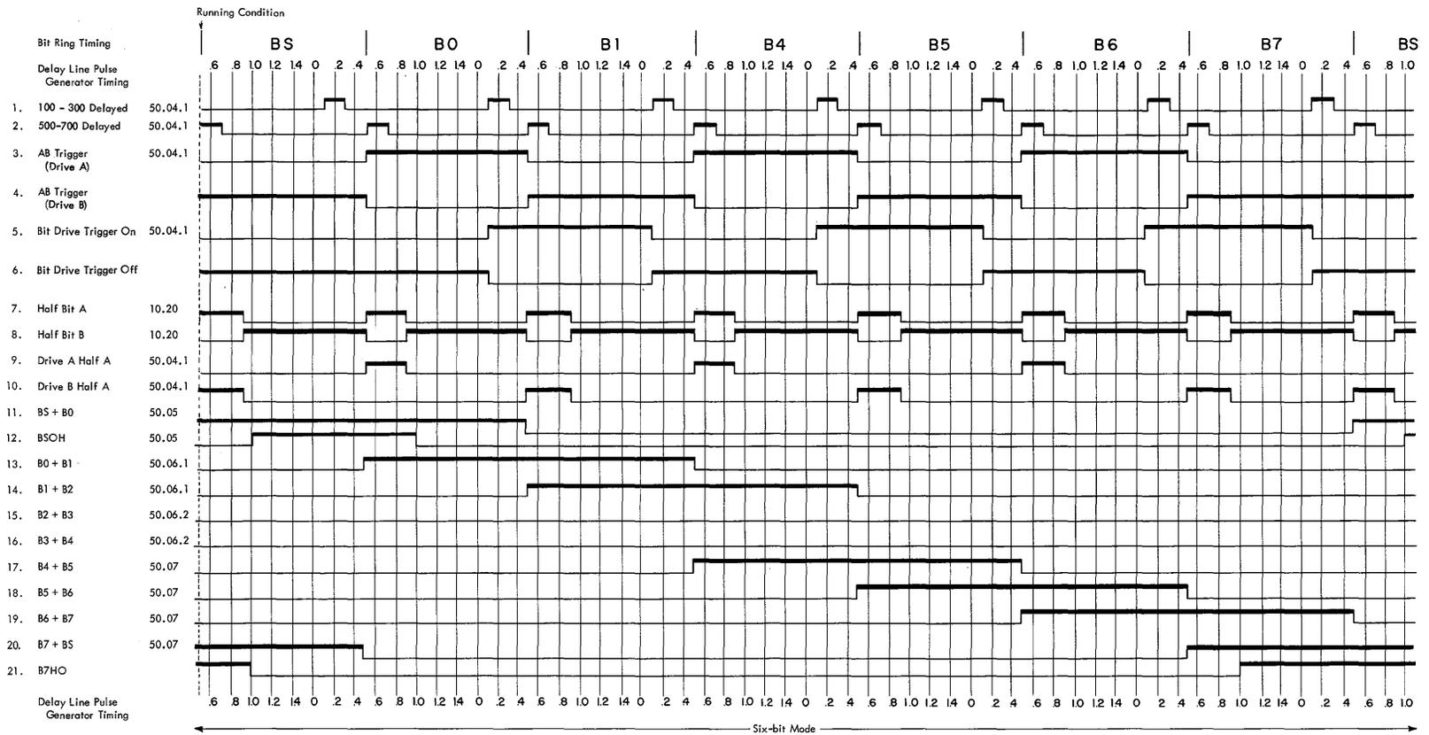
Figure 39. (Sheet 2 of 2). Bit Ring Timing—Six-Bit Mode
