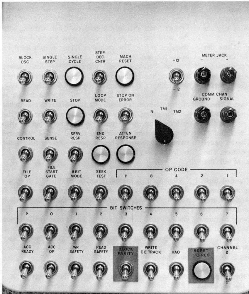
Figure 120. Customer Engineering Test Panel
