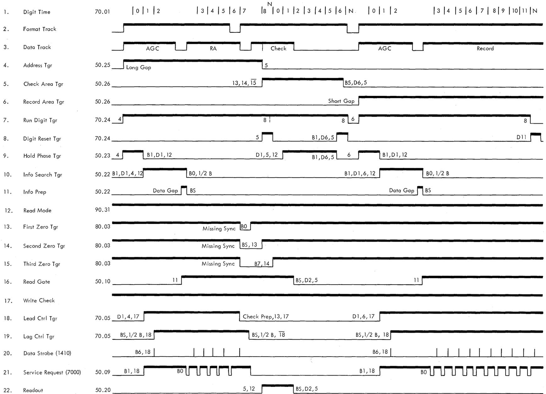
Figure 103. Write Check Timing
