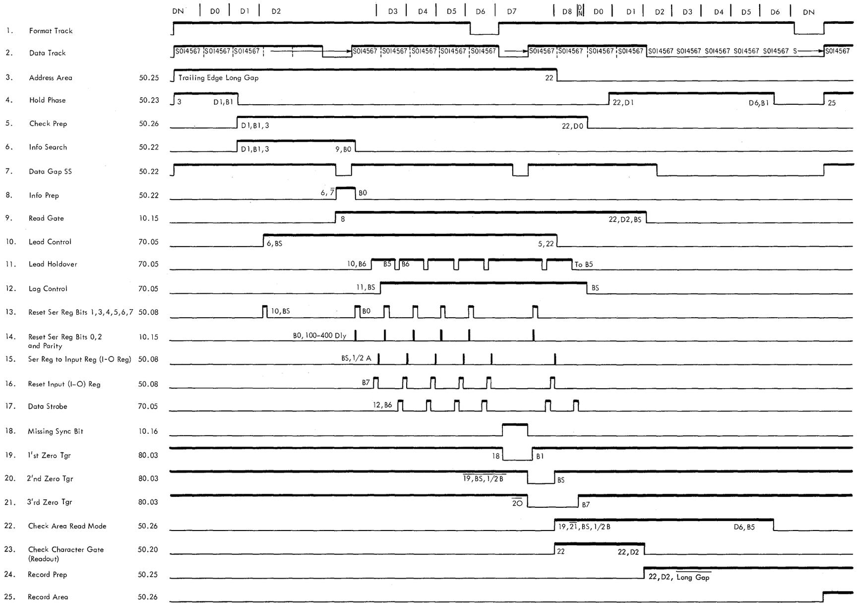
Figure 88. Read Data Cycle Timing
