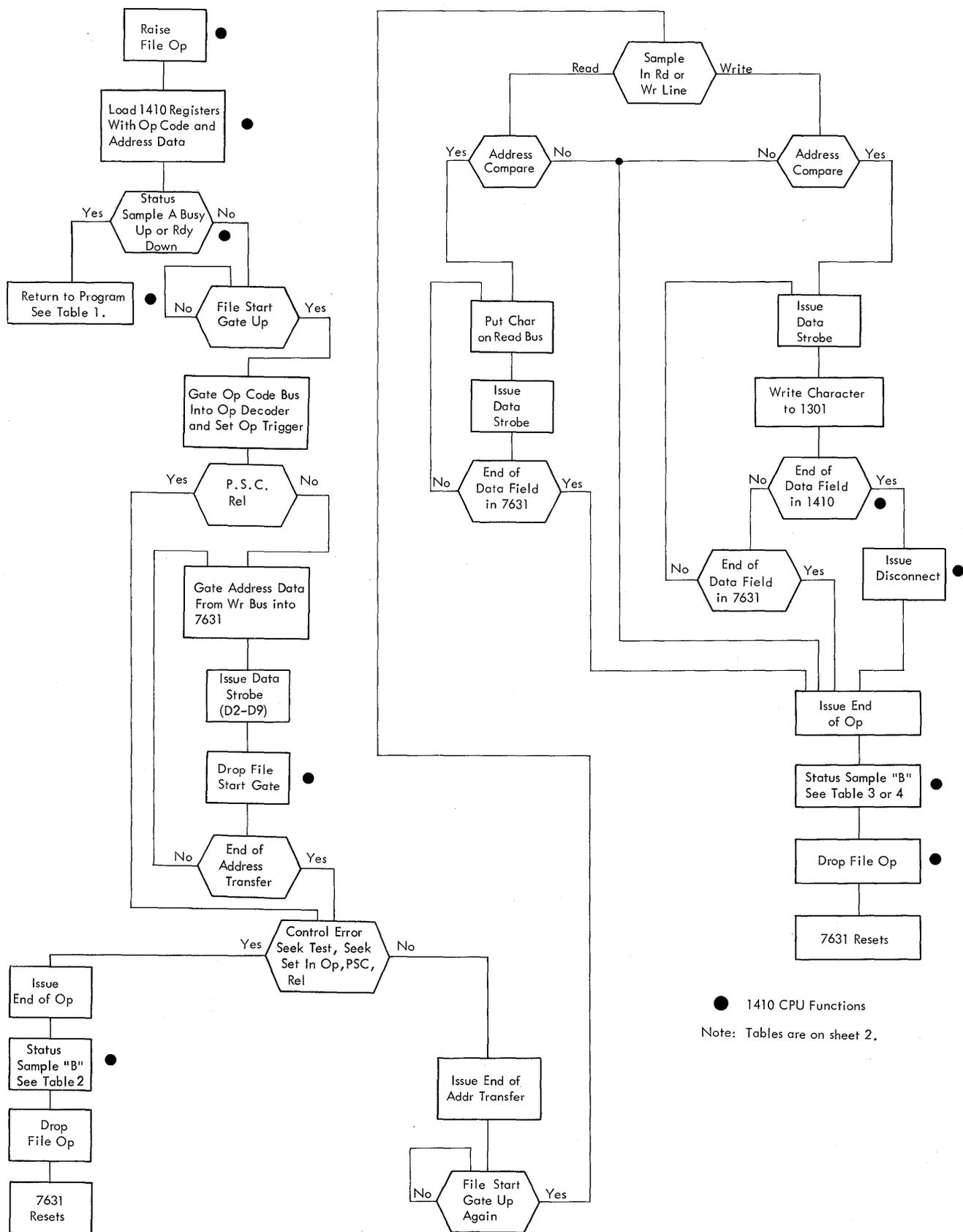
Figure 67. (Sheet 1 of 2). 1410-7631 Interface Flow Chart
