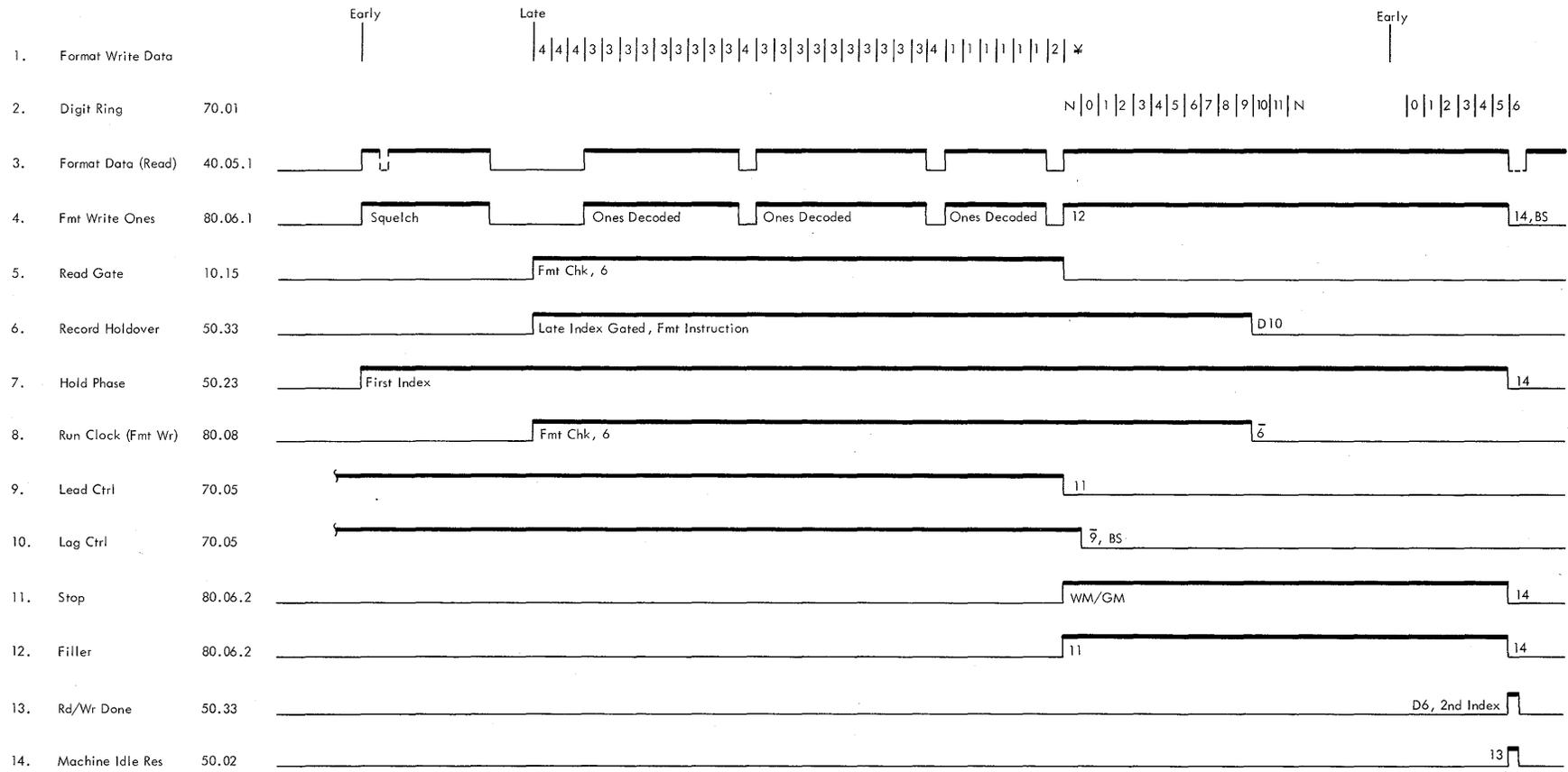
Figure 106. Format Write Check Timing
