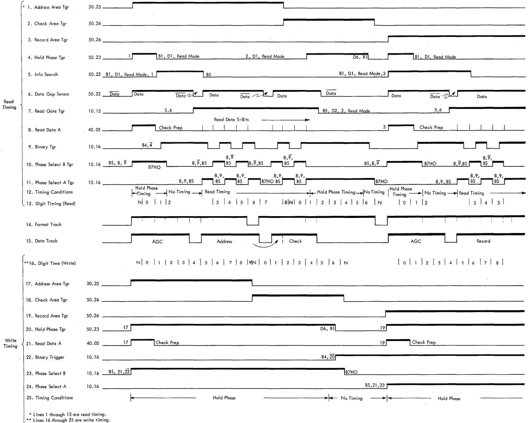
Figure 35. Phase Selection Timing
