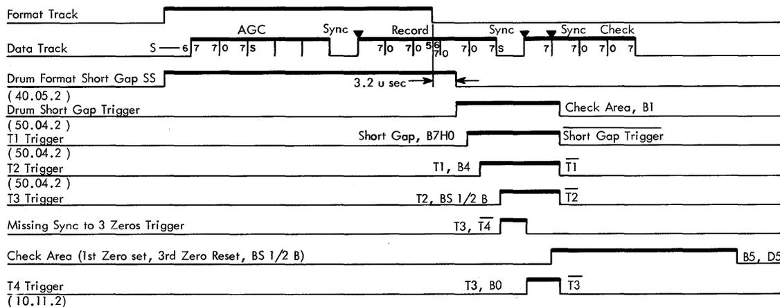
Figure 112. Missing Sync on Read
