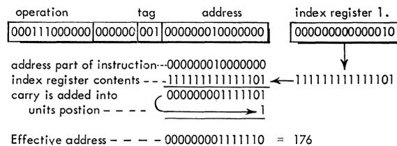
Figure 33. Index-Register Arithmetic, Subtracting
