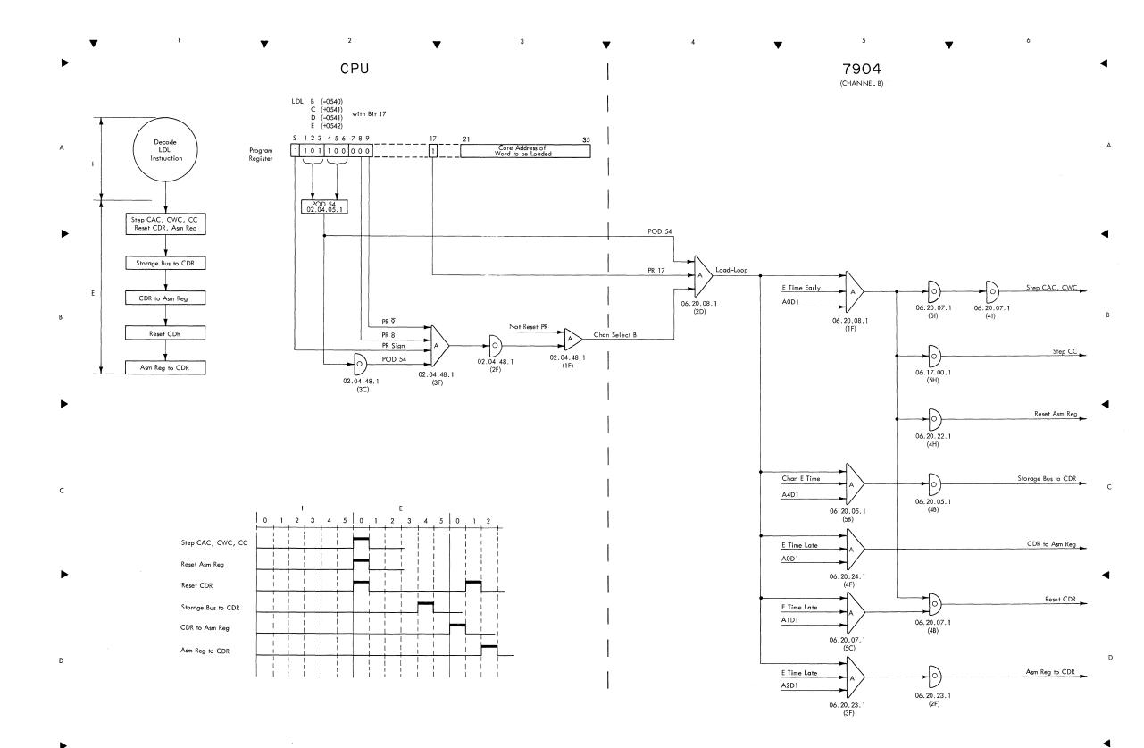
FIGURE 71. LOAD DATA REGISTER AND LOOP (LDL)
