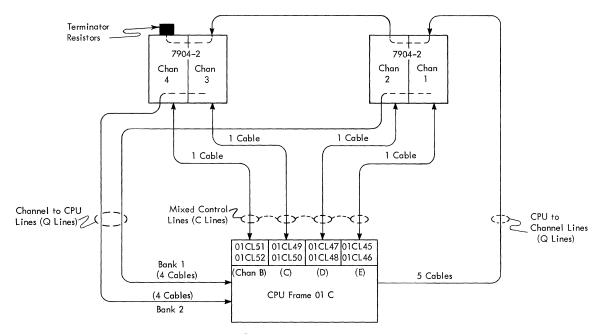
FIGURE 7. BASIC CABLE ARRANGEMENT, 7904 CHANNELS AND CPU
