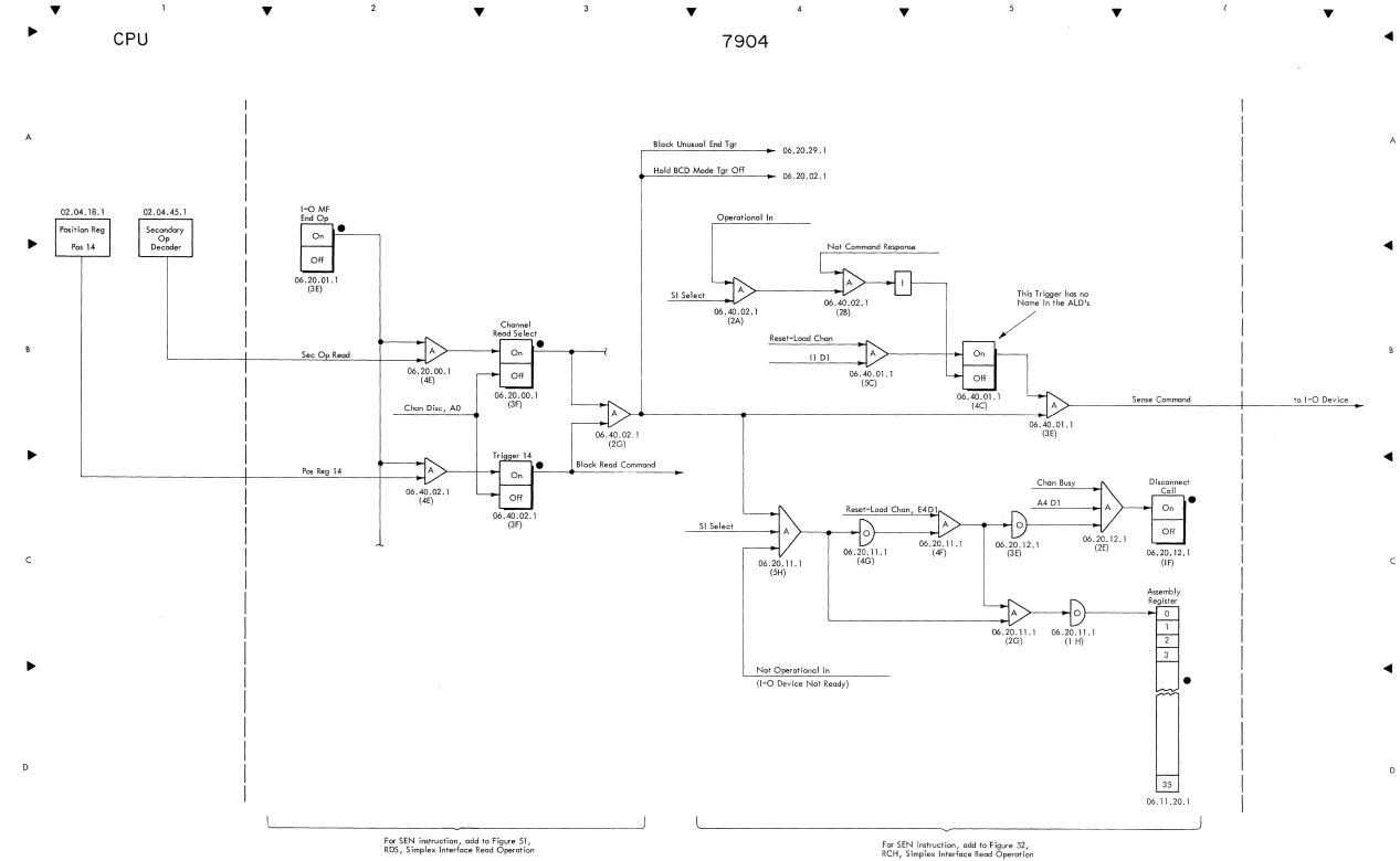
FIGURE 56. SENSE COMMAND, SIMPLEX INTERFACE SENSE OPERATION
