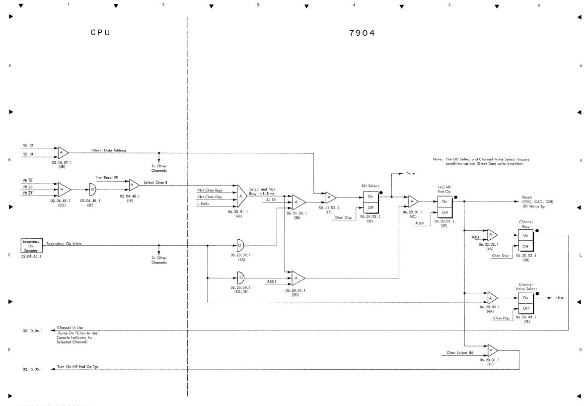
FIGURE 60. WRS, DD WRITE OPERATION
