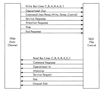
FIGURE 42. SIMPLEX INTERFACE SIGNAL LINES
