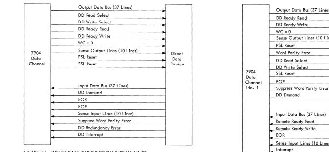
FIGURE 57. DIRECT DATA CONNECTION SIGNAL LINES
