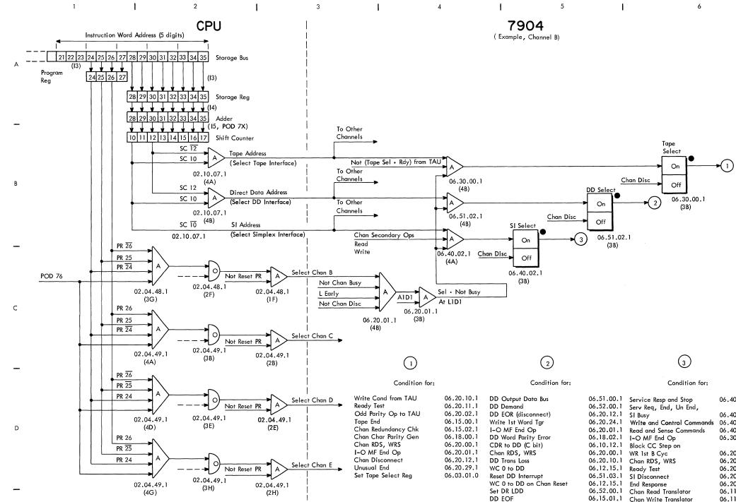
FIGURE 10. CHANNEL AND INTERFACE SELECTION
