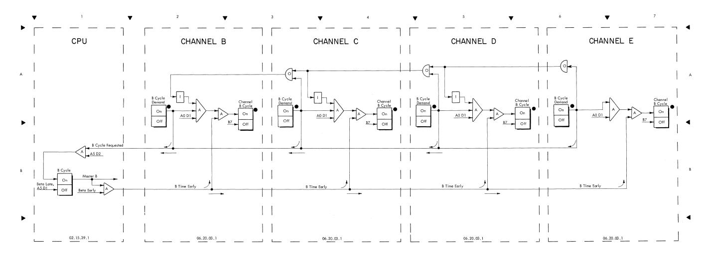
Note: Any channel's B Cycle Demand trigger on requests a B cycle of CPU. The next CPU cycle becomes the B cycle, the B cycle being granted to the requesting channel.
