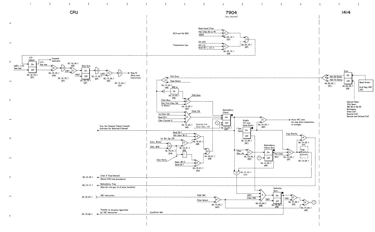
FIGURE 32. I-O CHECK AND REDUNDANCY CHECK, READ TAPE OPERATION
