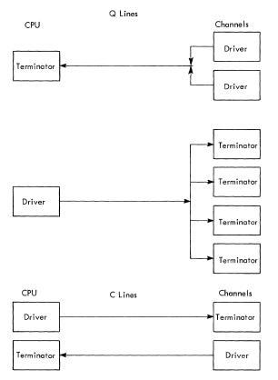
FIGURE 6. Q LINE AND C LINE EXAMPLES
