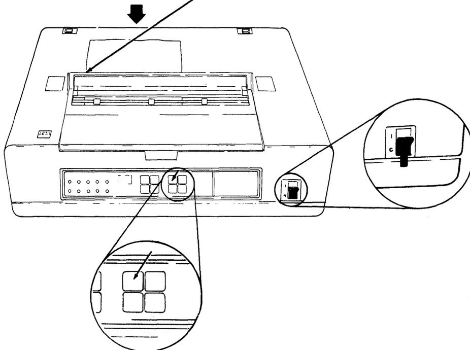
STEP 21. Press the I (POWER ON) side of the power switch.
