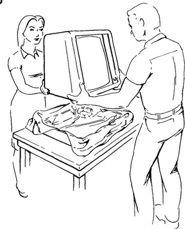
STEP 7. Place the Display on top of the Electronics Module.
