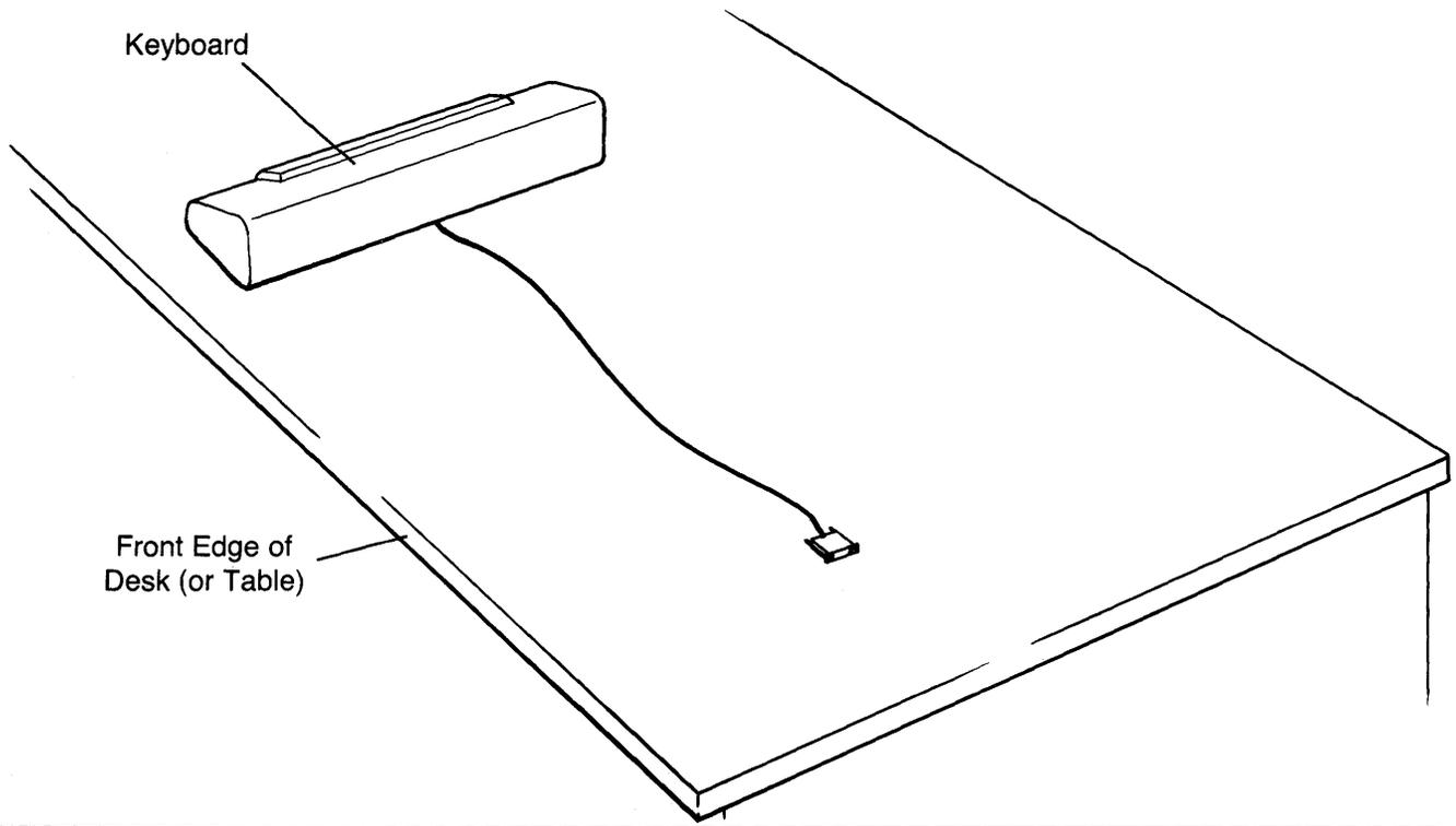
Leave sufficient space behind the Keyboard to place the other components sideways, as shown, for access to connect the cables.
