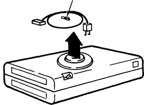
STEP 4. Place the Electronics Module over the Keyboard cable.
