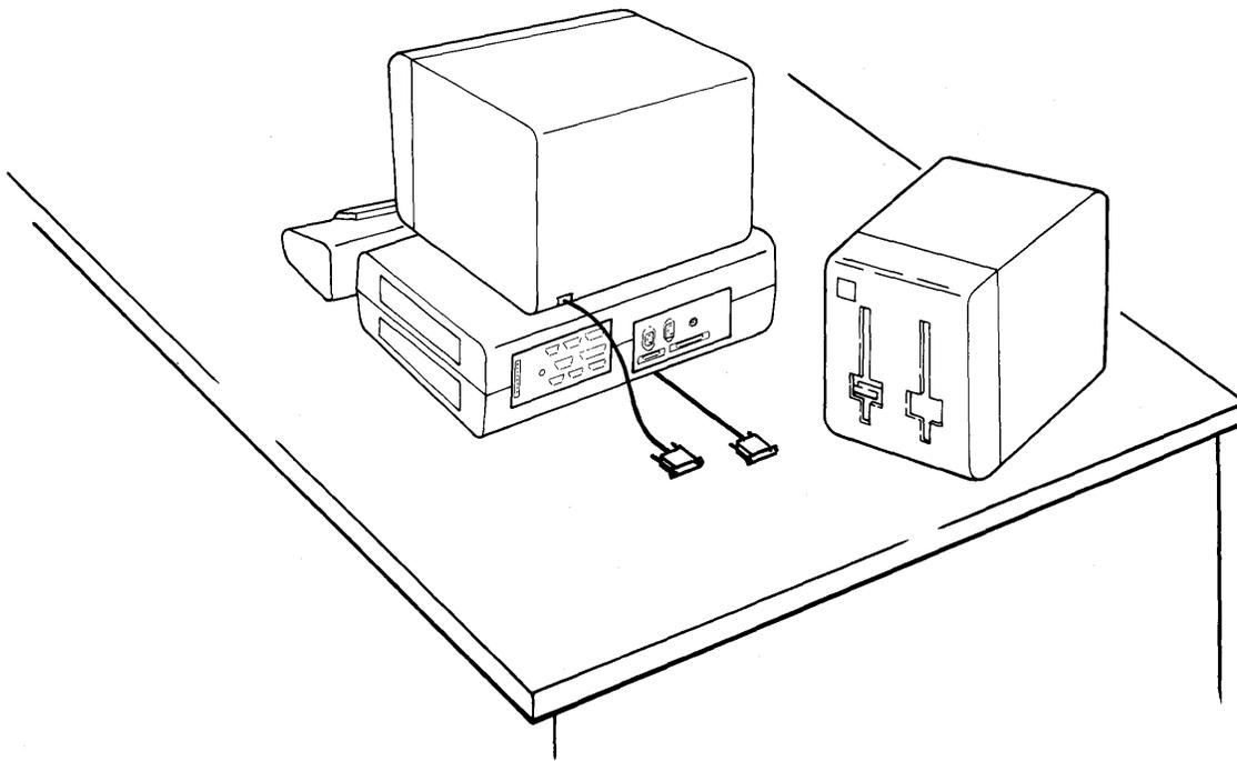
When connecting cable plugs, tighten the holding screws *finger tight* only.
