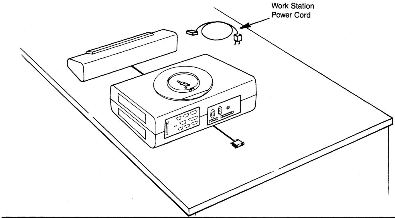
STEP 5. Write down the serial number from the back of the Electronics Module on the System Information Card (shipped with this setup guide).
