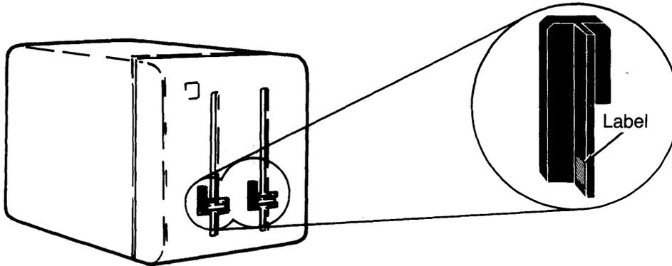
If your Diskette Unit has a
