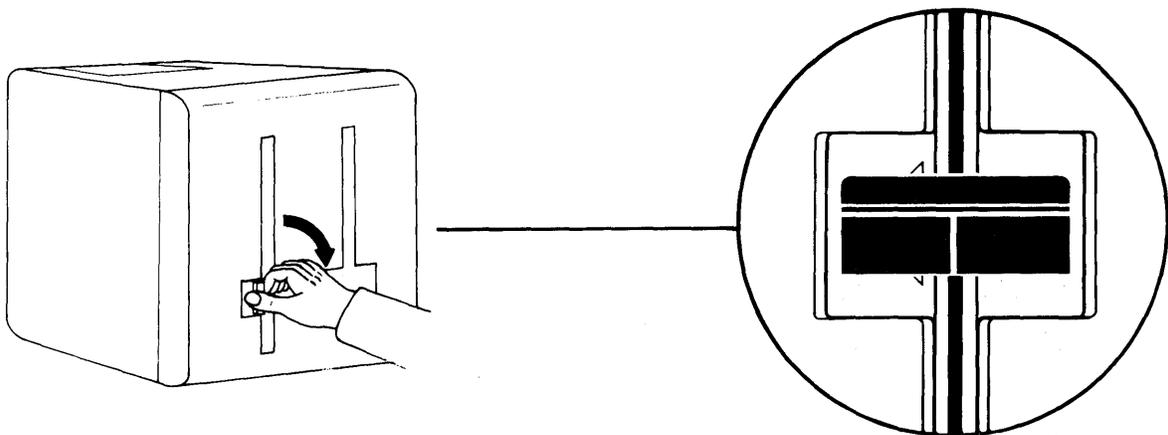
Close the load lever (the Diskette Unit should make a buzzing sound)
