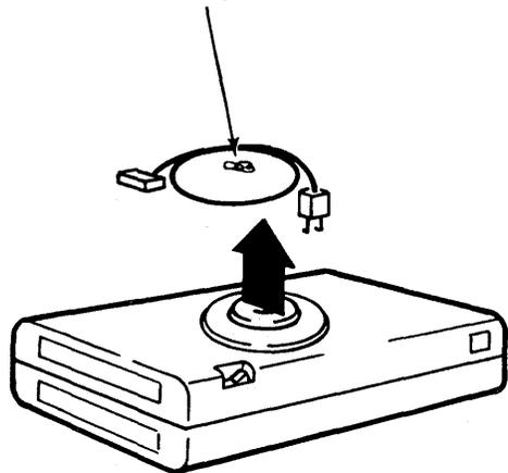
STEP 4. Place the Electronics Module over the Keyboard cable.
