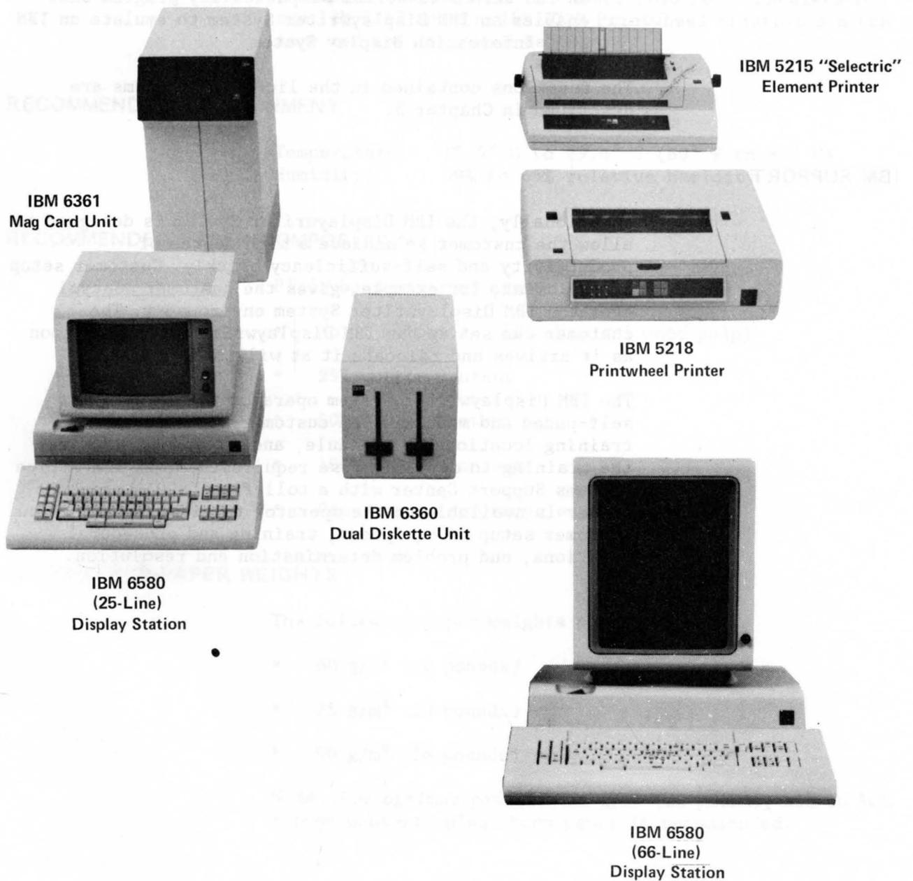
Figure 1-1. IBM Displaywriter System Components
