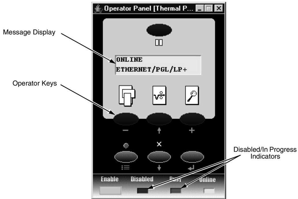
Figure 89. 6700/4400 Series Thermal Printer Virtual Operator Panel
