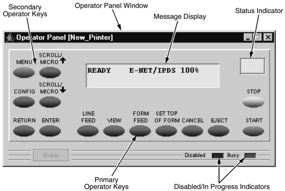
Figure 87. 6500 Series Line Matrix Printer Virtual Operator Panel
