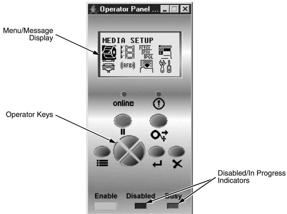
Figure 90. 6700-M40 Series Thermal Printer Virtual Operator Panel
