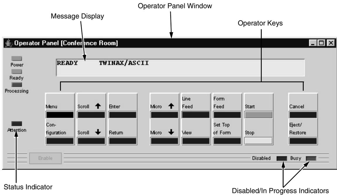
Figure 88. 6400 Series Line Matrix Printer Virtual Operator Panel
