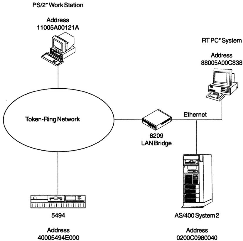
Figure D-4. 8209 LAN Bridge Addressing
