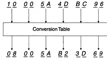
Figure D-5. An Example of Token-Ring Address Conversion
