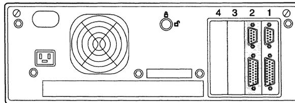
Figure 3-2. Back View of 5494 with Twinaxial Expansion Adapter in Slot 2
