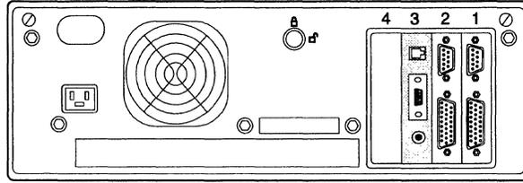
Figure 3-4. Back View of 5494 with 5494 Ethernet Adapter in Slot 3
