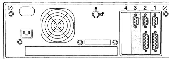
Figure 3-3. Back View of 5494 with 5494 Token-Ring Adapter in Slot 3
