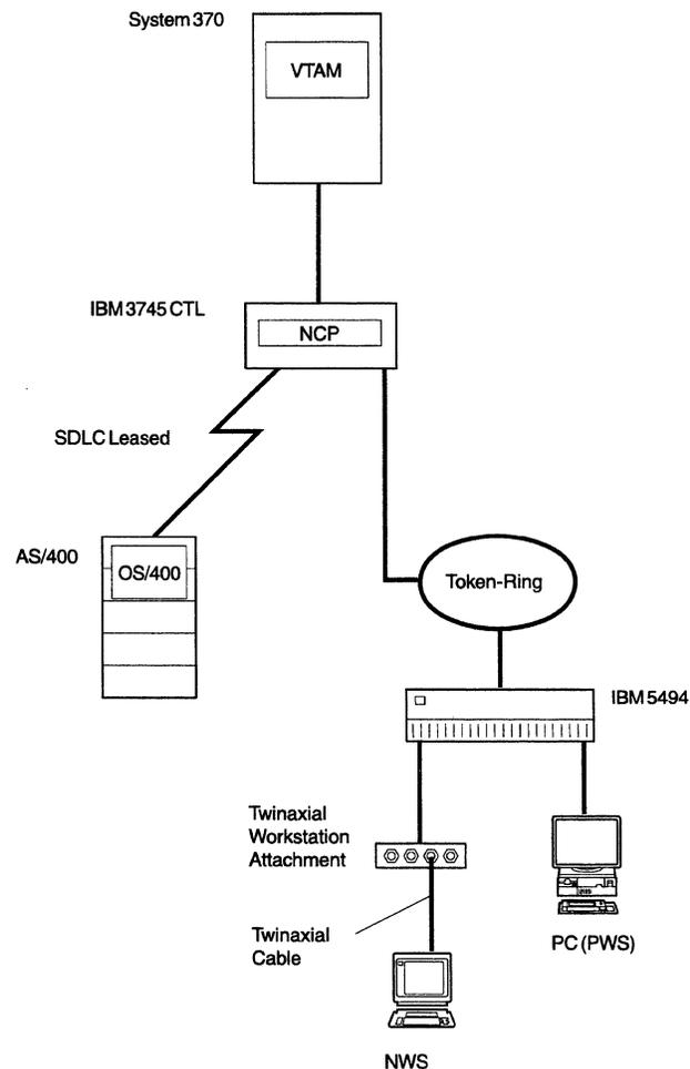
Figure C-2. Example of Physical Attachment of an AS/400 System, IBM 3745, and IBM 5494
