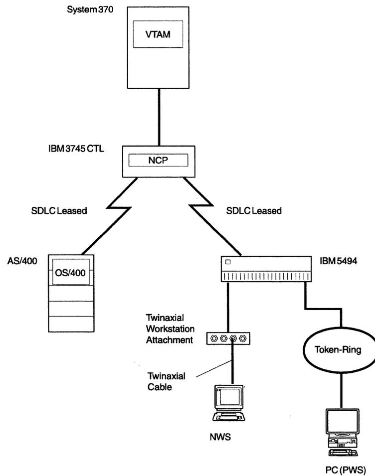
Figure C-1. Example of Physical Attachment of an AS/400 System, IBM 3745, and IBM 5494
