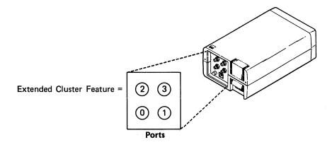
3. Determine the number of ports you will use. Then draw a line between the port(s) and work station(s) that make up your configuration. In the following example, three ports are used.
