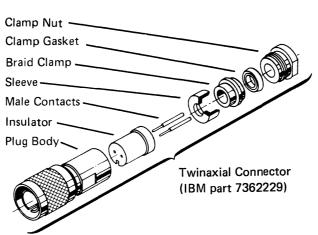
2. Cut the end of the cable sharp and square. Then slide a clamp nut and clamp gasket over the cable jacket and trim the jacket to the dimension given. Push the wire shield back to expose the inner insulation core, and cut the core and conductors to the dimension shown (16 millimeters [0.63 inch]). Slide the wire shield back over the core, and taper it to a point for ease of braid clamp assembly in step 3.
