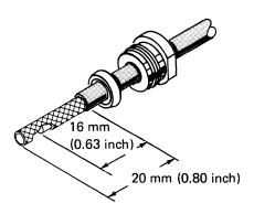
**Note:** If you are assembling a Teflon cable, install the heat shrink tubing before you continue with step 3.
