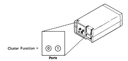
c. If your 5294 Control Unit will have four ports (Extended Cluster feature), the maximum number of work stations that can be attached to it is eight. Of these eight, up to seven can be attached to a single port using Cable Thru. Any combination of work stations (up to seven) is permitted on a port.
