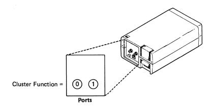
The Extended Cluster feature consists of two additional ports for a total of four ports, and allows an additional four work stations for a maximum of eight work stations that can be attached to a 5294 Control Unit. Of these eight, up to seven can be attached to a single port (using Cable Thru). Any combination of work stations is permitted on a port.
