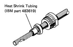
Slide a braid clamp over the braid so that its inner shoulder butts against the cable jacket. Then, fold the shield back over the braid clamp and trim below the shoulder.
