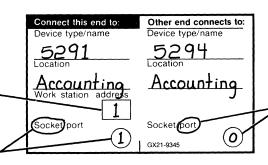
This is the port and port number on the 5294 where the other end of the cable is connected.
