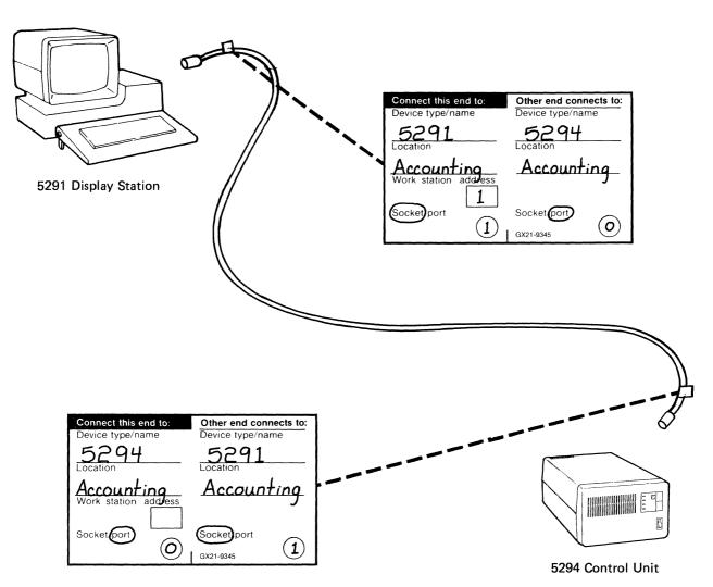
4. If an end of a cable will be connected to a station protector, each end of the cable should have a label attached to it as shown below. Instead of indicating on the label that the cable connects to a certain station protector, indicate what is connected to the station protector.
