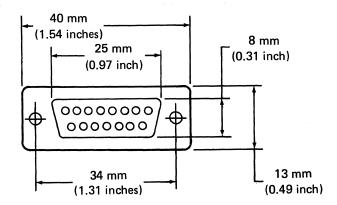
Figure 8-8. 15-Pin Connector
