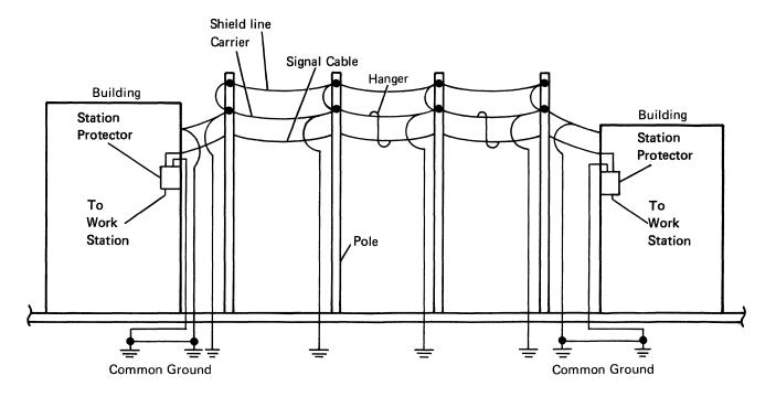
Note: When the cable is run jointly with the power line, the carrier wire should be bonded to the multiground neutral (MGN). The MGN can be used instead of an earth-driven grounding rod. Bond all ground points to the power company multiground neutral.
