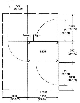
Note: Signal cables connect into the back of the machine.
