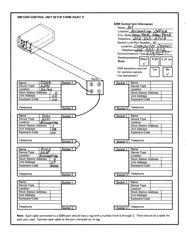
Figure D-4 (Part 1 of 2). Completed 5294 Setup Form for the Second Example
