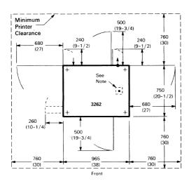
Note: Both the signal cable and power cable can be routed through a single 64-mm (2-1/2 inch) hole in raised floor. Recommended location for the hole is centered between the front and back of the machine, and 100 mm (4 inches) in from the right side.
