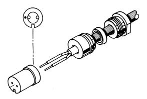
8. Insert the assembly into the connector body, aligning the polarizing slot in the insulator with the polarizing pin inside the plug body. Tighten the clamp nut with 5.7 to 6.8 N·m (Newton meters) (50 to 60 inch lbs) torque. (The cable and plug body should not be allowed to twist as the clamp nut is tightened.)
