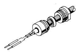
Bend the conductors and the contacts out at right angles to the cable axis (approximately 6.4 millimeters [0.25 inch]). Then bend the conductors and contacts back parallel to each other.
