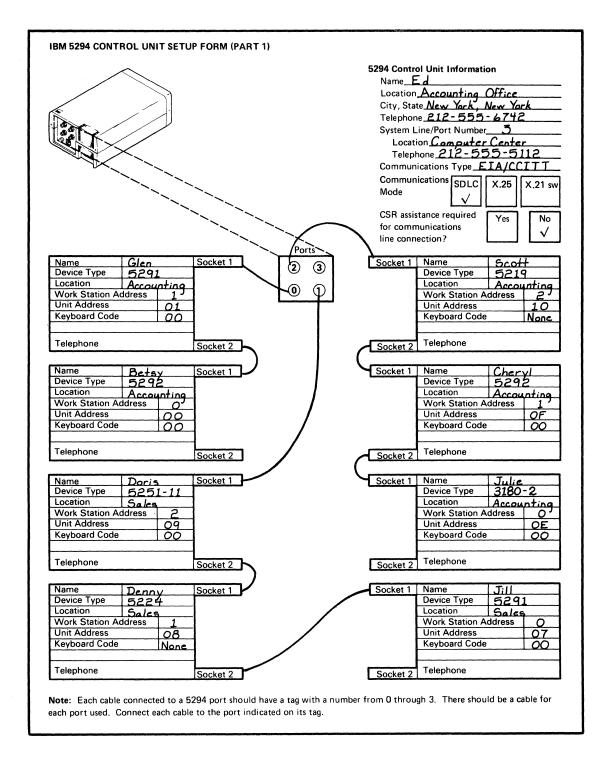
Figure D-2 (Part 1 of 2). Completed 5294 Setup Form for the First Example
