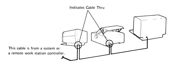
Ordering Cable Thru on all work stations initially will make future additions to your configuration easier. Cable Thru is standard on the 3180 Model 2, 5291, 5292, 5219, and 5224. It is a feature on the 5251 Model 11, 5225, and 5256.
