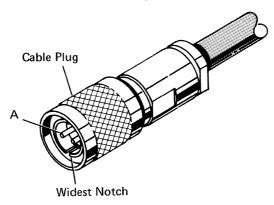
The polarity of the line must be maintained for each cable segment and for the entire cable run to ensure proper machine operation.
