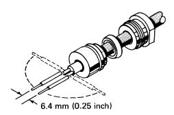
Slide the insulator over the contacts and the cable so that the insulator butts against the sleeve. Press all parts together. The contact on the bare copper lead of the cable goes into the insulator hole that has a dot next to it.
