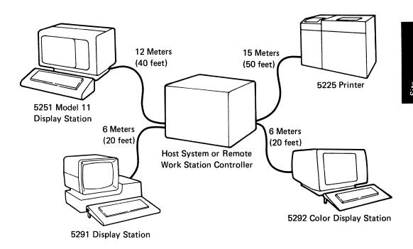
Even when work stations will not be on a Cable Thru line, ordering Cable Thru on work stations initially makes future additions of work stations easier.
