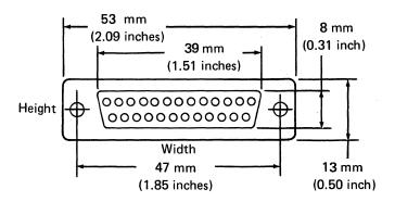
Figure 8-7. 25-Pin Connector
