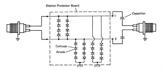
Use a VOM (volt ohm meter) with 50,000 to 100,000 ohms per volt. Set on the ohms x 100 or ohms x 200 scale.
