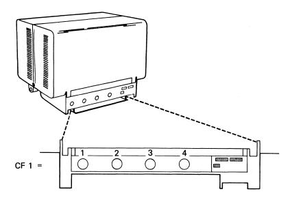
With the Cluster feature, you can attach a maximum of four work stations to a 5251 Model 12. These work stations may be distributed in several ways over the four ports. Your choices range from one work station on each port to a maximum of four work stations on one port.
