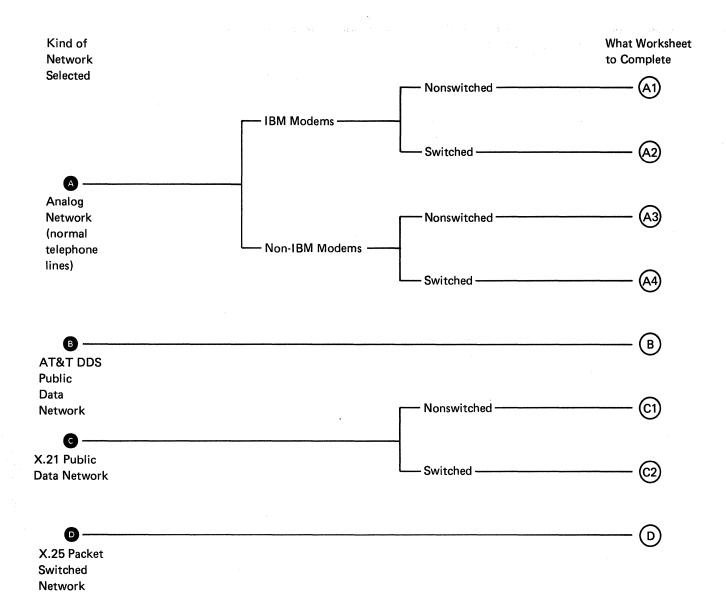
Figure 5-3. Kind of Network and What 5294 Control Unit Communications Worksheet to Complete
