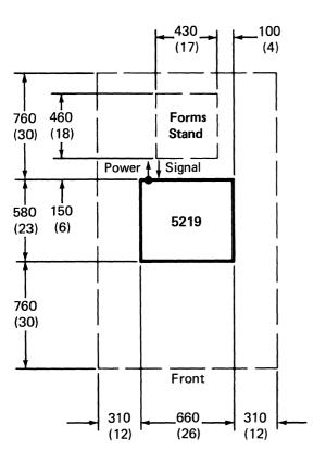
Note: Signal cables connect into the back of the printer.
