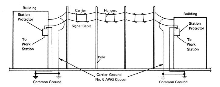
Note: For overhead cables, avoid having the twinaxial cables as the highest point in the area.
