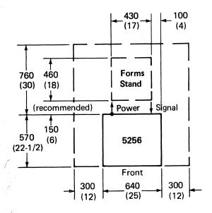
Note: Signal cables connect into the back of the machine.
