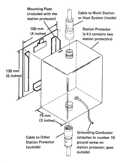
**Note:** It is important that the grounding conductor is on the same side of the station protector as the cable leading to the outside of the building.
