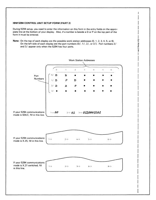
Figure D-2 (Part 2 of 2). Completed 5294 Setup Form for the First Example
