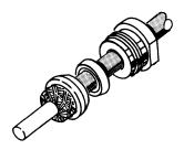
**Note:** Placement of braid wires over the braid clamp must be uniform to provide good rf (radio frequency) connection of the shield, and to prevent breaking the shield strands.
