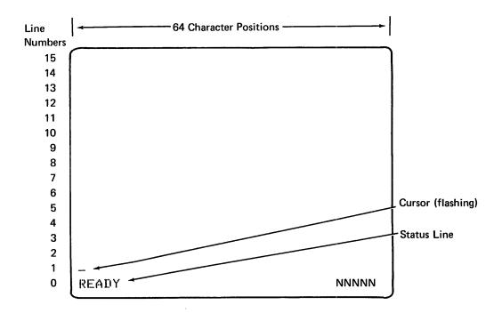
Figure 2. The 5110 Display Screen Format
