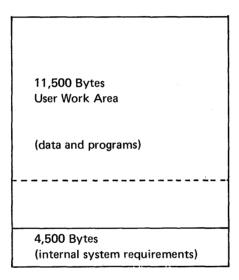
Figure 5. Storage Allocation for a 16K System
