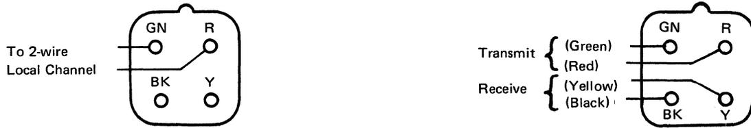
**Note:** When two half-duplex leased line (2-wire) common carrier facilities are used to service a 3603 Model 1, and they are terminated in two jacks, the jacks must be installed within 254 mm (10 in) of each other, and adapter IBM PN 1741656, or equivalent, is used in conjunction with cable assembly IBM PN 1745350, or equivalent.
