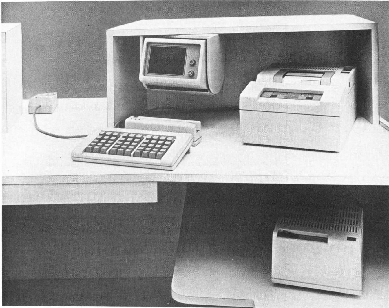
Figure 3-4. Basic Teller Work Station with the Control Module
