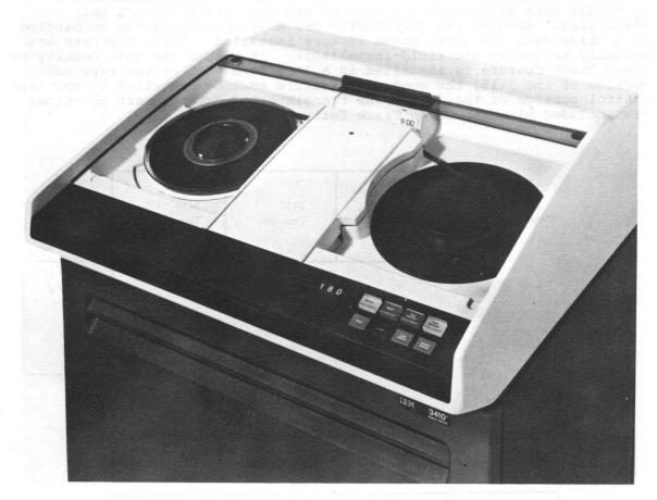
Figure 20.22.1. The 3410 Magnetic Tape Unit
