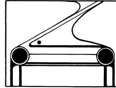
Figure 4 indicates a dirty (plugged) left air bearing or worn left stubby column glass bead tape.
