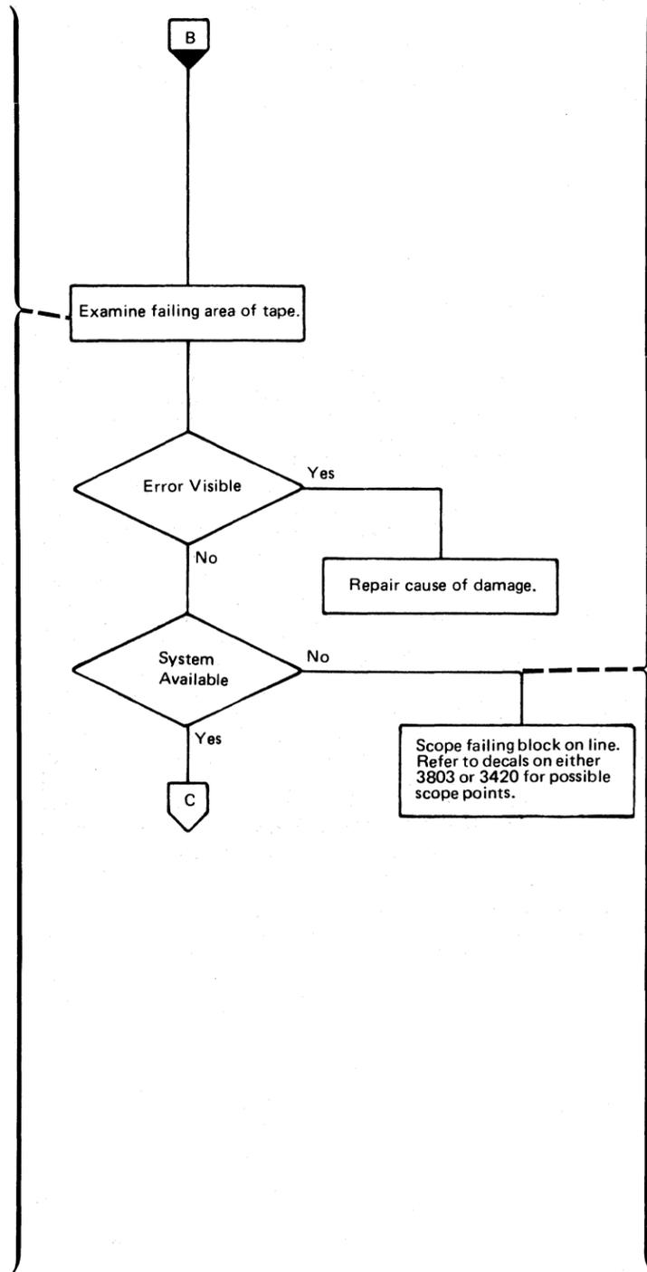
**Scope Failing Block Offline**
