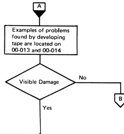
**Analysis of Damaged Tape Errors**
