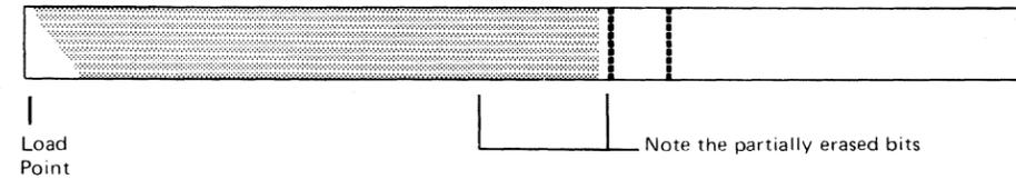
This tape lift came from a different customer account with the same tape problem. However, this failure indicated a permanent read error after the tape had been used at least once. This could be a big problem in most accounts if a master file has to be re-created. The magnetized heads will decrease the signal strength each time the tape passes over the heads.
