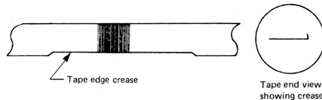
Developing the tape shows that the bits were written on the tape and then the tape was damaged. This type of damage is usually caused by improper tape handling.
