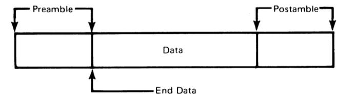
Sync the scope on END DATA while scoping one of the digital data tracks at the tape drive or control unit.
