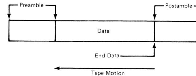
Sync the scope on End Data and scope one of the data tracks at the tape drive or control unit. Measure the length of the postamble in microseconds. Then enter the following commands:
