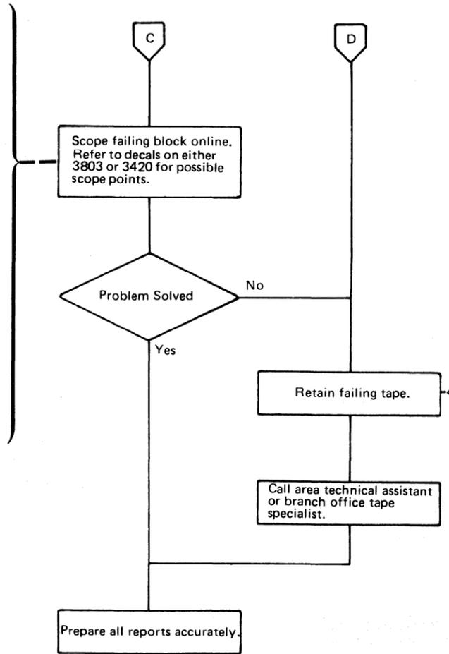
If cause of the permanent read error cannot be determined, save the tape and any information gathered for use by branch office or area tape specialist. A permanent read error can cost the customer considerable reconstruction and rerun time, especially if the tape was written a month or more prior to the time of reading it. **There should be no undefined permanent read errors.**
