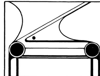
Figure 3 indicates a dirty (plugged) left air bearing, low air bearing pressure, high vacuum, or improper vacuum door glass to column seal.
