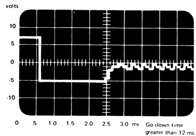
**Note:** Check timings for  $\pm 10\%$  deviation. Check Voltages for  $\pm 5\%$  deviation.
