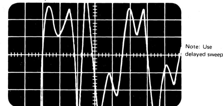
If signal between amplitude nulls and ground reference drops below 50 mv errors can occur.
