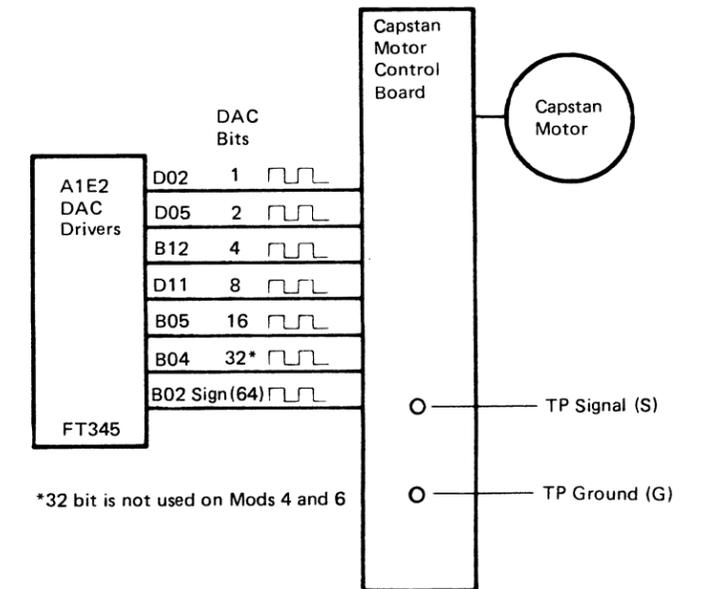
Figure 2. Tape Unit Set-Up
