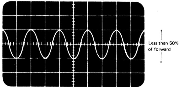
6. If there is a read backward problem, and the amplitude in the backward direction is less than that of the forward direction by 50% on any one track, or 60% on the remaining tracks, the read/write head should be replaced. If head replacement is required, perform the removal/replacement procedure on 08-250, do required adjustments and return to the MAP that sent you here or 00-030. If replacement is not required return to the MAP that sent you here.
