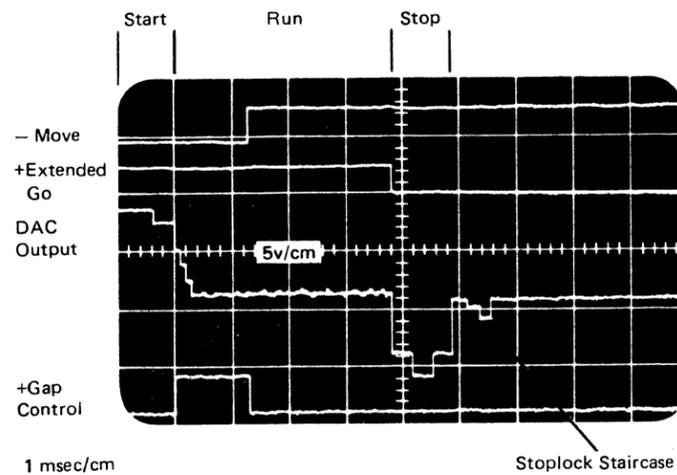
**Note:** Waveform is for Model 6. The time after gap control will vary depending on tester setup and tape unit model.
