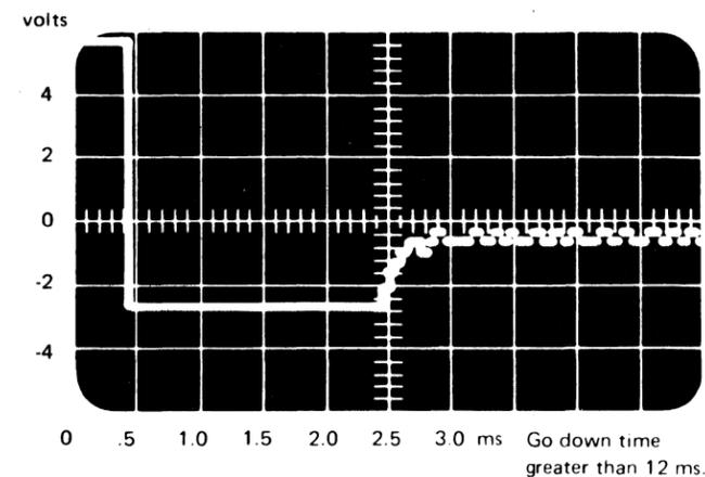
**Note:** Check timings for  $\pm 10\%$  deviation. Check voltages for  $\pm 5\%$  deviation.
