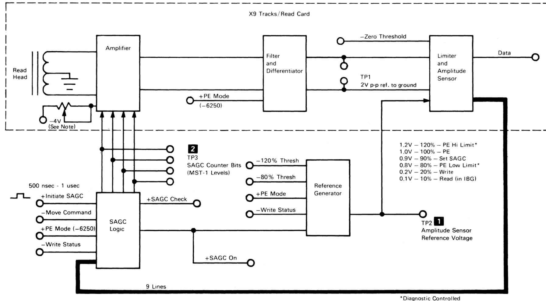
**Note:** Potentiometers are used to set amplitude in 1600 bpi mode. SAGC sets Read signal amplitude automatically in 6250 bpi mode. A 6250 bpi single density tape unit retains the track 1 potentiometer to adjust the gain for reading the ID burst.
