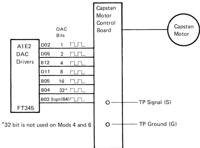
Figure 2. Tape Unit Set-up.
