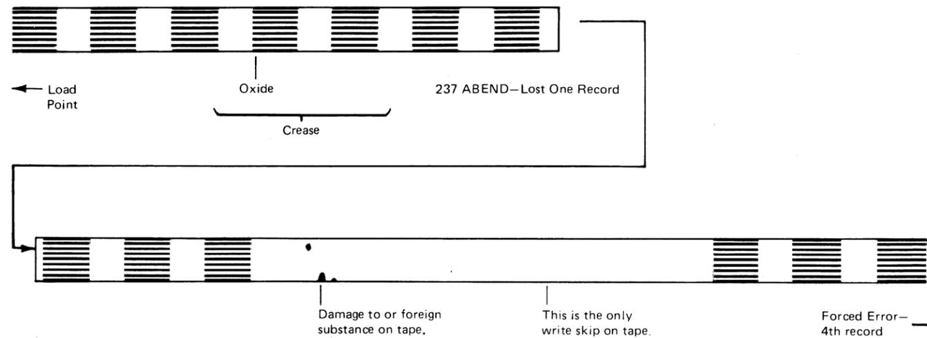
One record lost when compared to the trailer label count. This can be mistaken for one write error when the tape is created. It is actually caused by the tape crease. If the crease is smoothed out, the count is corrected. Tape crease was caused by excessive capstan to stubby bar clearance.
