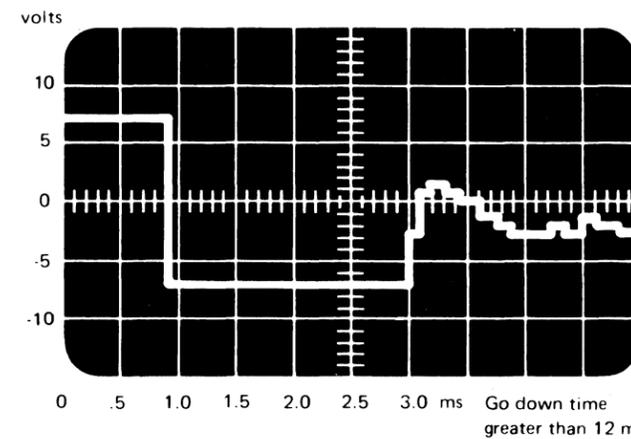
**Note:** Check timing for  $\pm 10\%$  deviation. Check voltage for  $\pm 5\%$  deviation.
