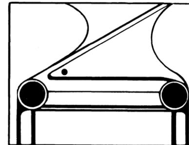
Figure 2 indicates a dirty (plugged) right air bearing, low air bearing pressure, high vacuum, or improper vacuum door glass to column seal.
