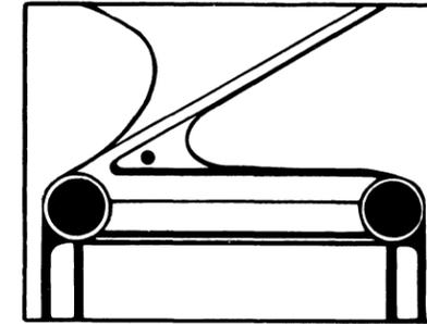
Figure 5 indicates a dirty (plugged) right air bearing or worn right stubby column glass bead tape.
