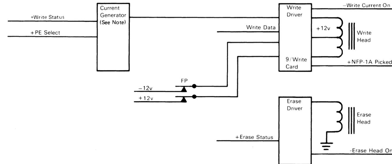
**Note:** The Current Generator sets the appropriate write driver currents for 1600 bpi and 6250 bpi operations.
