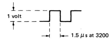
**F** Set Up Scope Horizontal to 1μs Vertical to 10v scale
