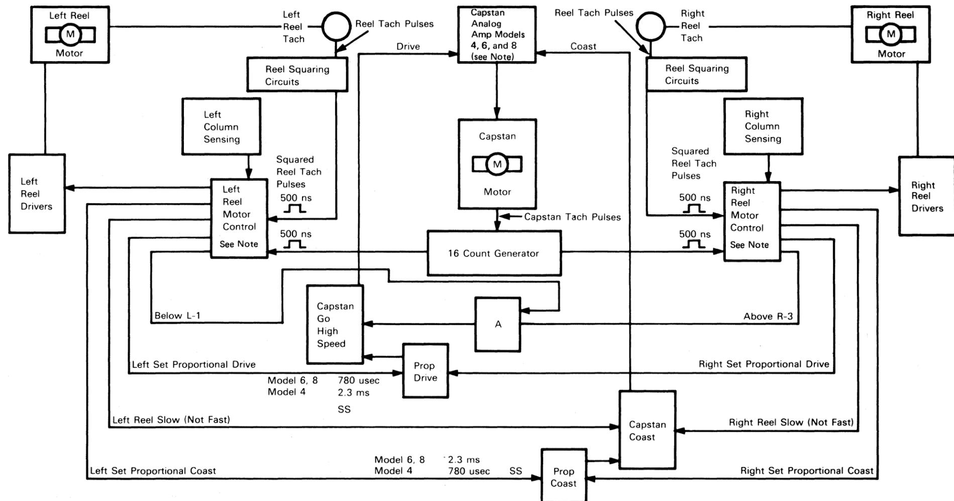
**Note:** The Reel Fast latch either causes the capstan to drive or lets it coast, depending on the position of tape in the columns. If the right and left circuits make different demands at the same time, coast overrides drive.
