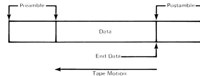
Sync scope on END DATA and scope one of the data tracks at the tape drive or control unit. Measure the length of the postamble in micro-seconds. Then enter the following commands:
