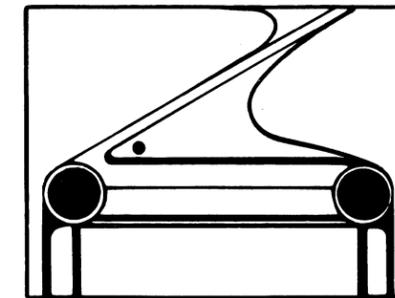
Figure 4 indicates a dirty (plugged) left air bearing or worn left stubby column glass bead tape.
