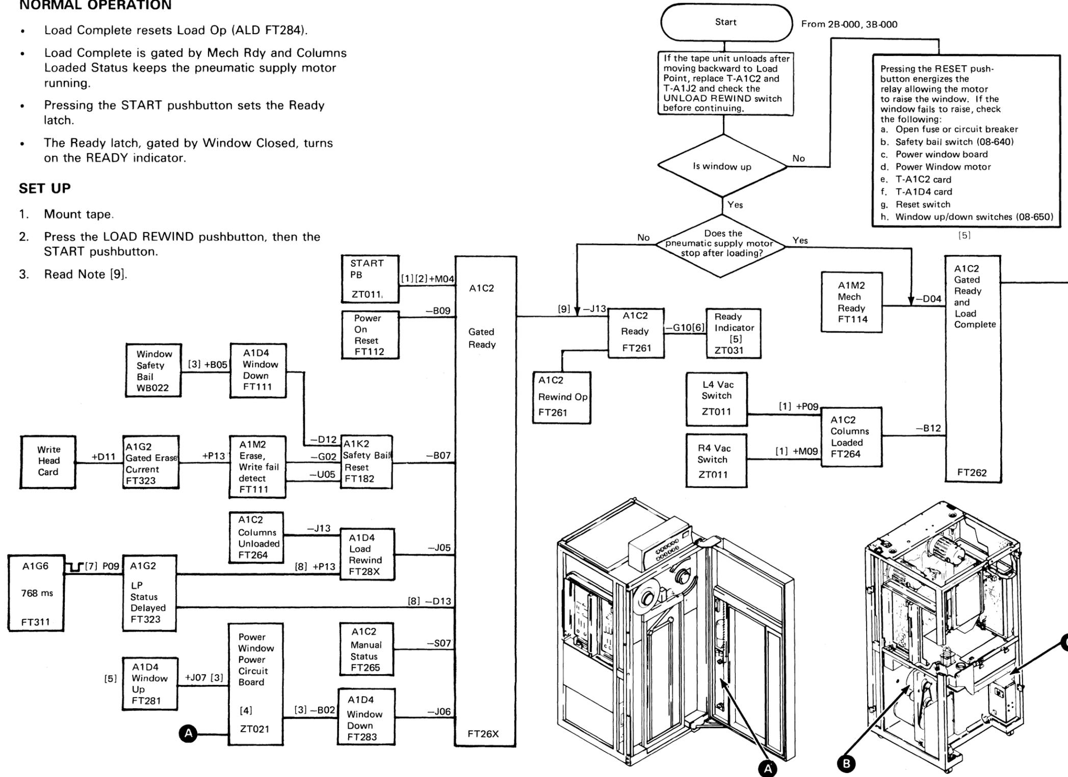
Pressing the RESET push-button energizes the relay allowing the motor to raise the window. If the window fails to raise, check the following:
