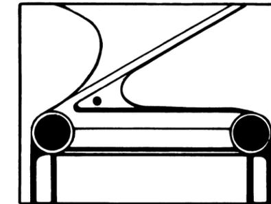
Figure 5 indicates a dirty (plugged) right air bearing or worn right stubby column glass bead tape.
