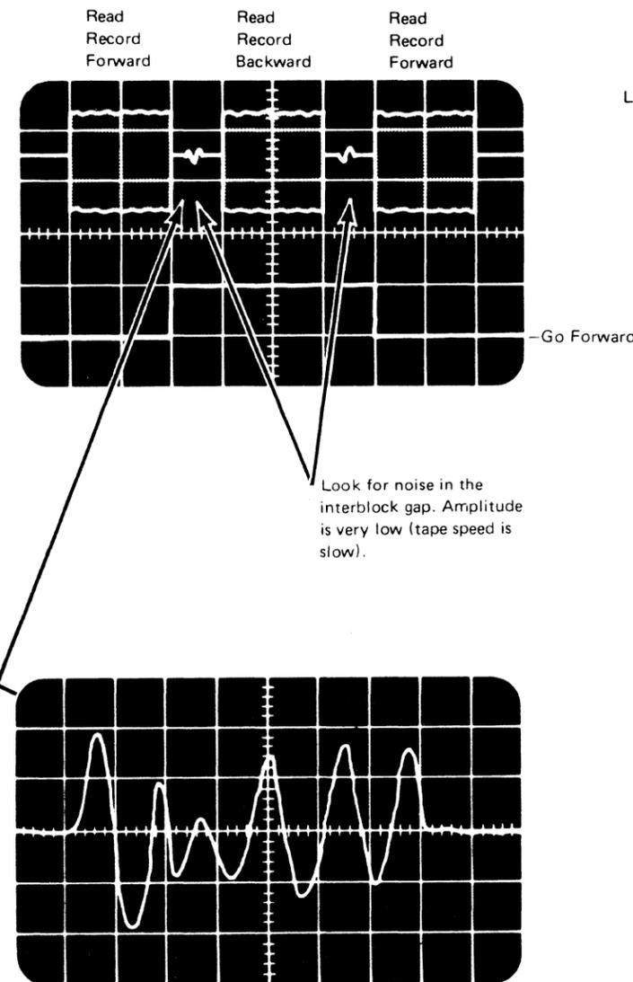
Look for noise in the interblock gap. Amplitude is very low (tape speed is slow).
