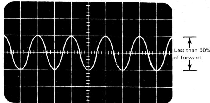
7. If there is a read problem, and the amplitude in one direction is more than double the amplitude in the opposite direction on any one track, replace the read/write head. If read/write head replacement is required, perform the removal/replacement procedure on 08-250, do required adjustments and return to the MAP that sent you here or 00-030. If replacement is not required return to the MAP that sent you here or 00-030.
