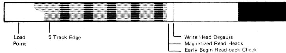
This error is a result of magnetized read heads. Notice where the read heads stop and where the write heads are degaussed. Figure 1A shows a failure that occurred while the customer was using the drive. If magnetized tools are used, or a resistance check is made on the head, be sure to degauss the transport before returning the tape unit to the customer.
