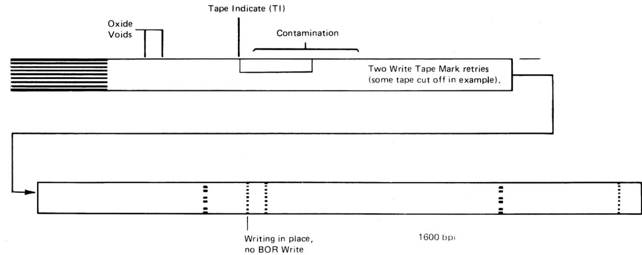
This tape was marginal before this error occurred. Oxide voids caused by contaminates sticking to the next wrap, contamination from the cleaner blade, caused the failure illustrated.
