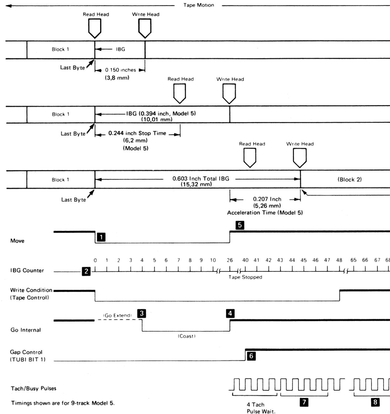
1. Tape position when MOVE drops for block 1.
