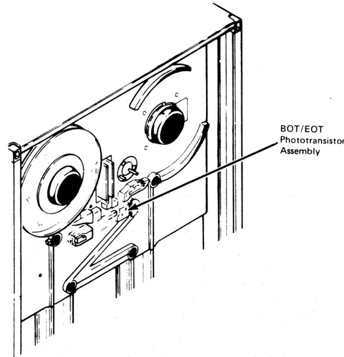
BOT/EOT Phototransistor Assembly
