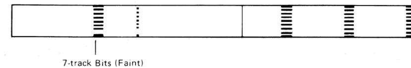
Seven track tape lift, caused faint 7-track bits. If the write head card is defective, nothing is visible in this track.
