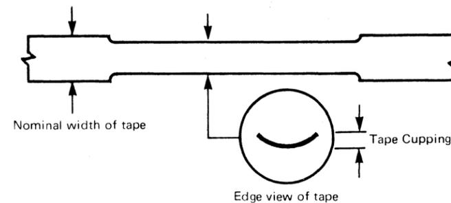
When the stretched section of tape is held in a loop it distorts. Stretched tape usually occurs near the beginning of the reel or in areas of high speed to slow speed rewind.
