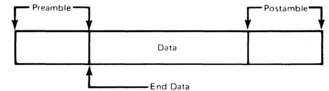
Sync the scope on End Data while scoping one of the digital data tracks at the tape drive or the control unit.
