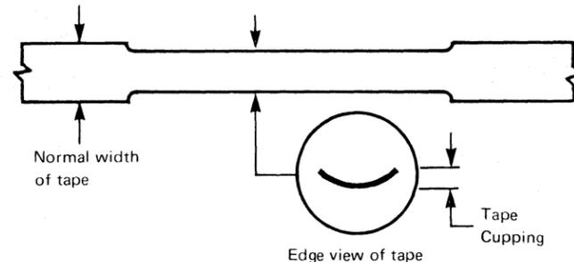
When the stretched section of tape is held in a loop it distorts. Stretched tape usually occurs near the beginning of the reel or in the area of high speed to slow rewind.
