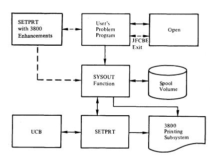
Figure 2. An Overview of SYSOUT Processing to the 3800
