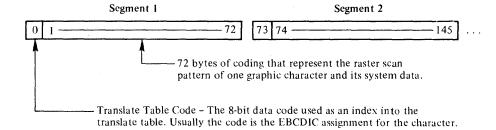
When a graphic character is to be modified, the 3800 uses the translate table code to index into the translate table. The contents found at that location (a 1-byte WCGM code) determine the WCGM location into which the 72 bytes of scan pattern and system data are to be placed.
