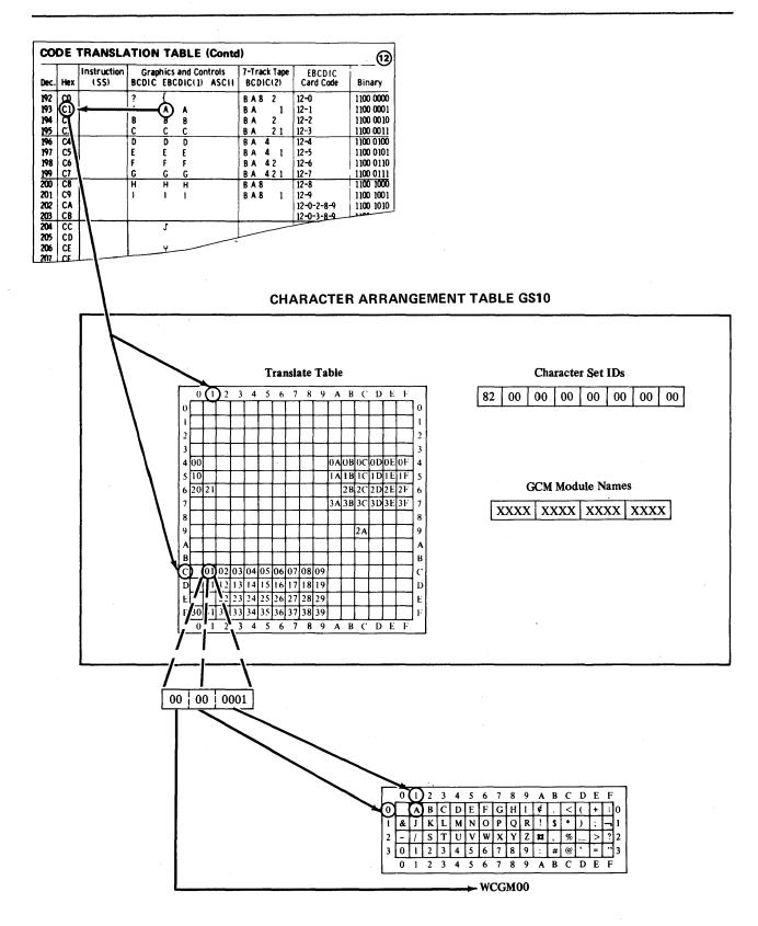
Figure 5. How an 8-bit Data Code is Translated into a WCGM Location
