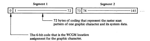
A library character set is loaded directly into a WCGM. SETPRT uses the 6-bit code, contained in the first byte of each 73-byte segment, as the address of the WCGM location into which the remaining 72 bytes are loaded.
