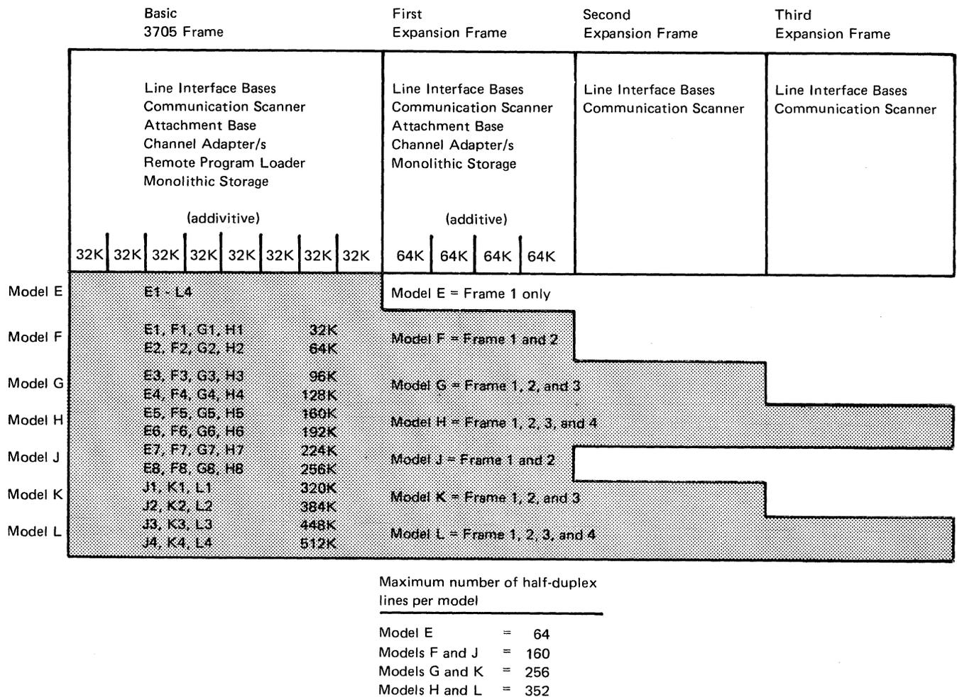
Figure 1-4. IBM 3705-II Line Attachment and Storage Capacity by Model
