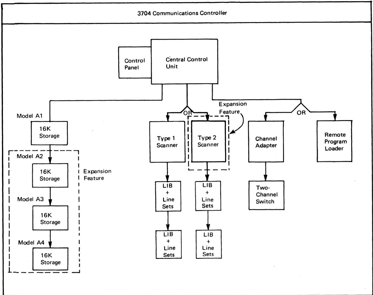
Figure 1-2. Maximum Hardware Configuration of the 3704 Communications Controller
