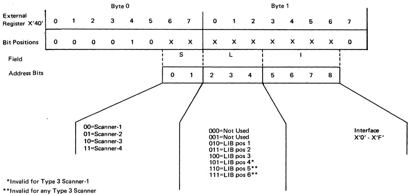
Figure 3-4. Types 2 and 3 Scanner Interface Address Bits
