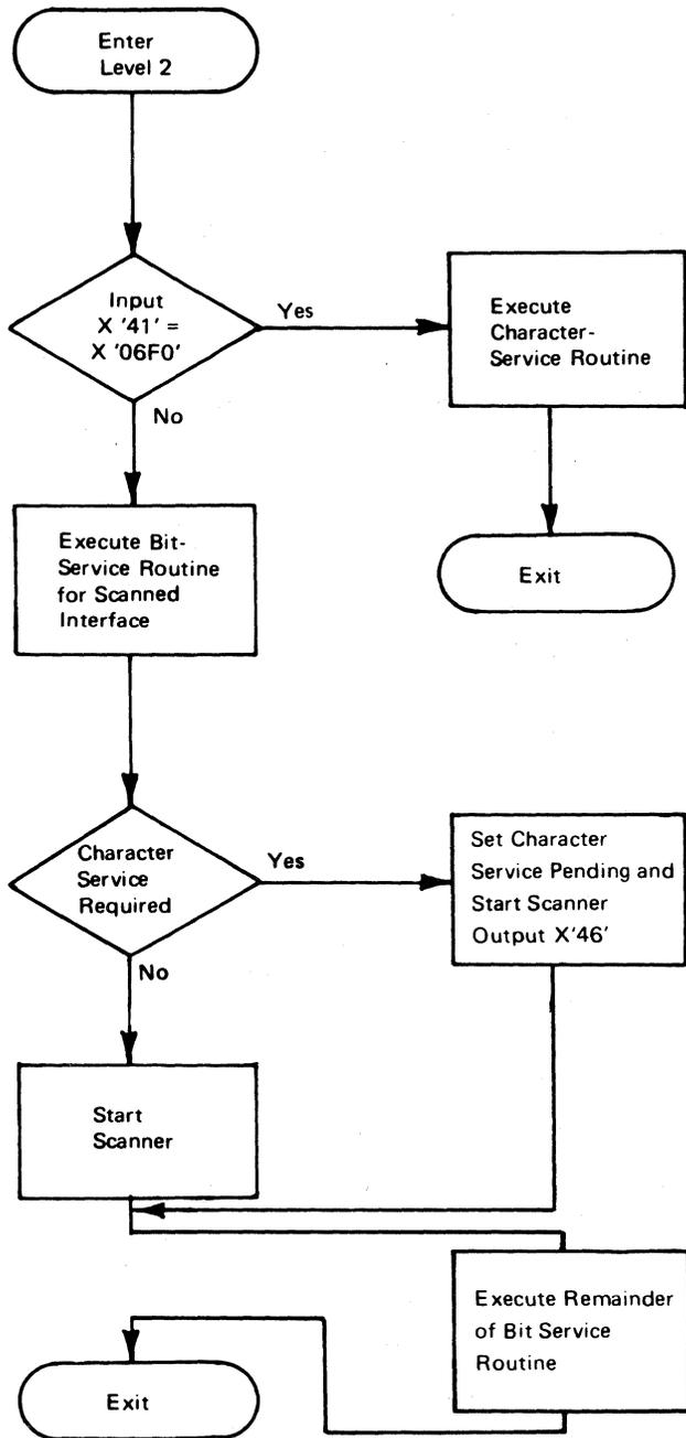
Figure 6-2. Level 2 Program Flow (Type 1 Communication Scanner)
