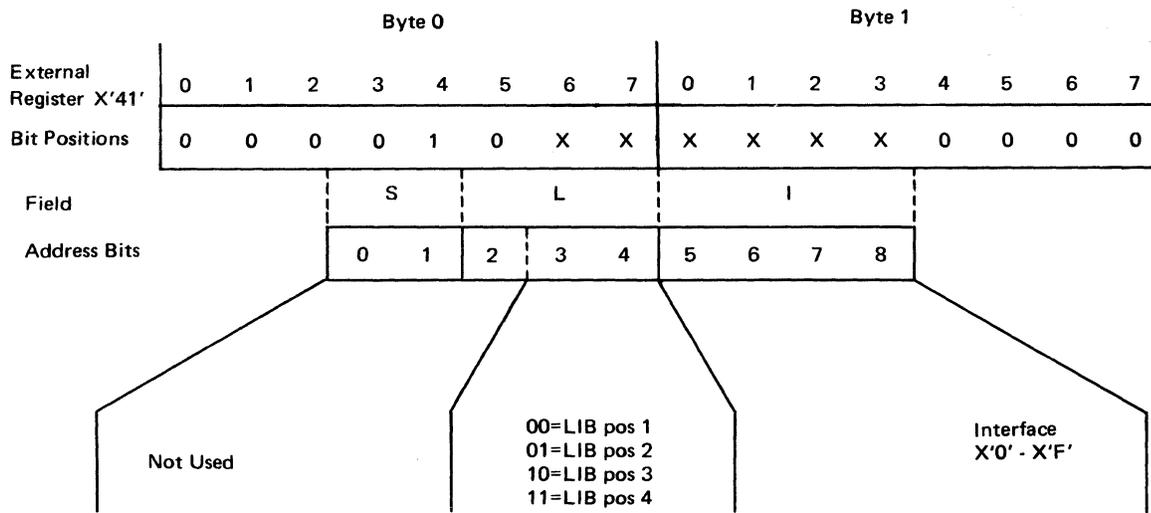
Figure 3-3. Type 1 Scanner Interface Address Bits
