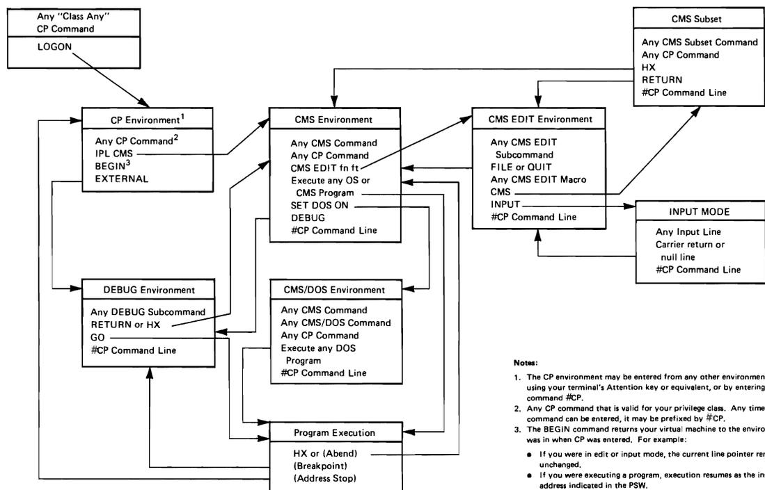
Figure 2. VM/SP Environments and Mode Switching
