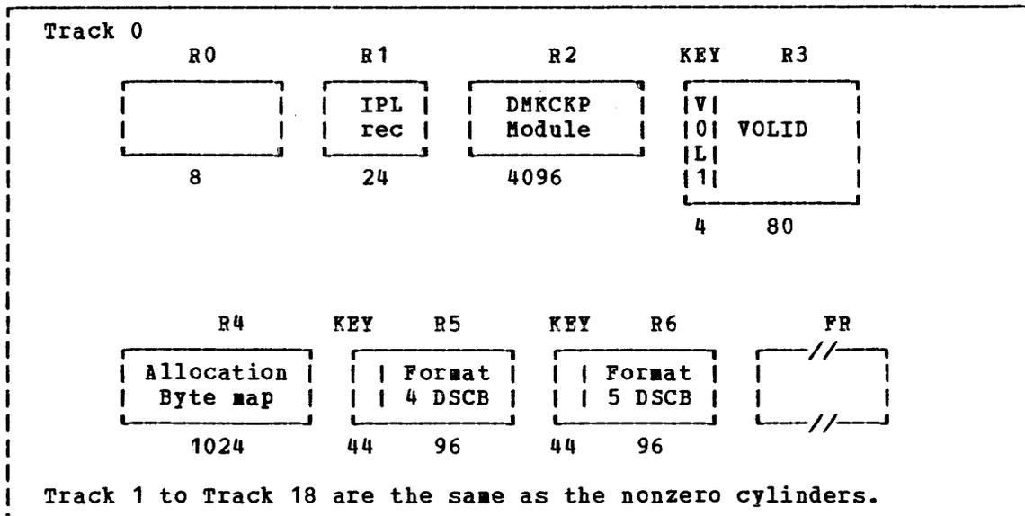
Figure 8. 3330, 3340, or 3350 Cylinder 0 Format
