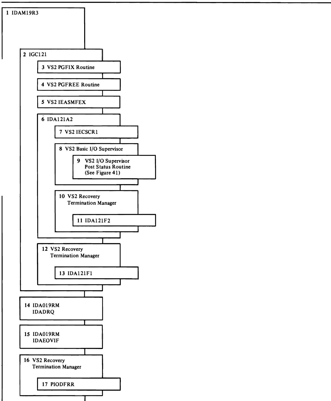
Figure 40. I/O Management: Translating Virtual Addresses to Real Addresses and Completing a Channel Program for I/O
