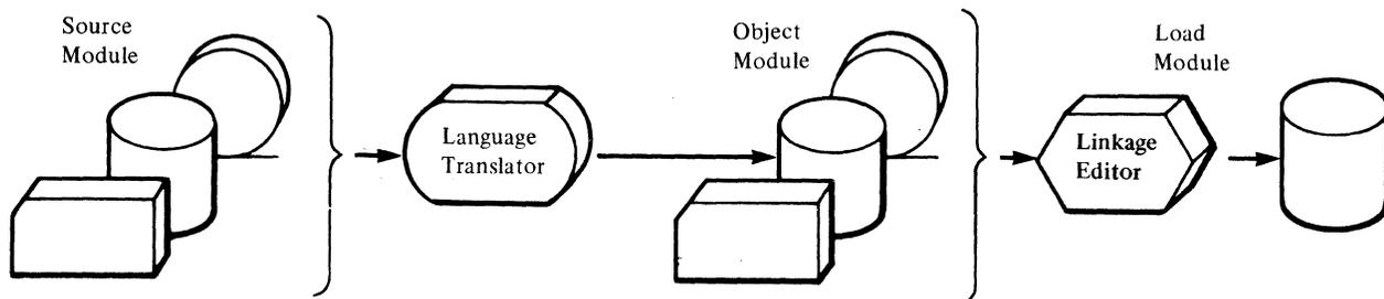
Figure 1. Preparing a Source Module for Execution
