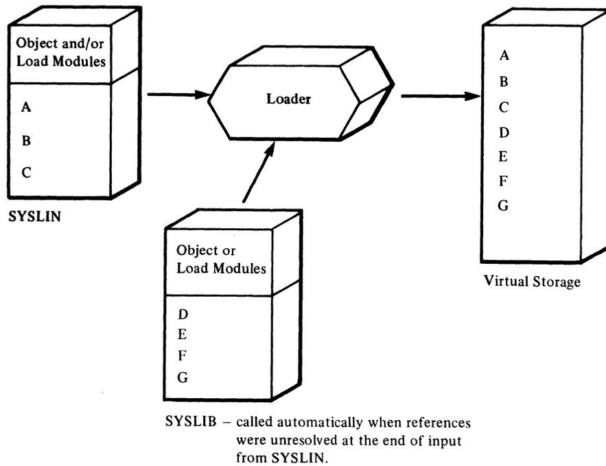
**Figure 38. Loader Processing—SYSLIB Resolution**
