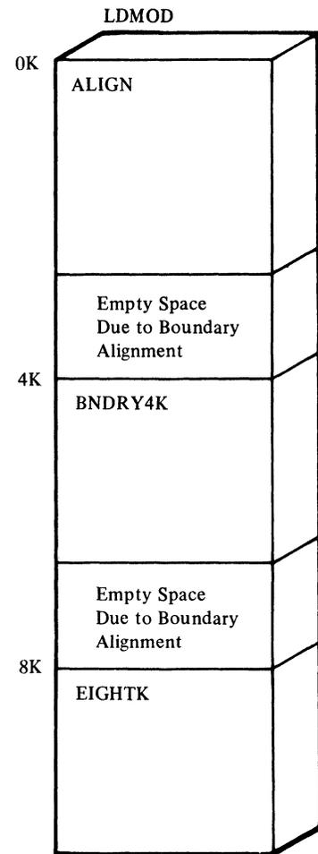
Figure 26. Output Load Module for PAGE Statement Example
