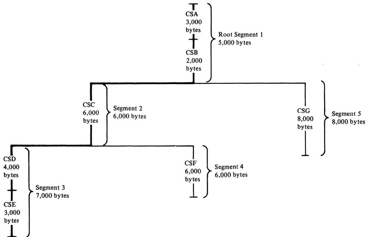
Figure 63. Length of an Overlay Module
