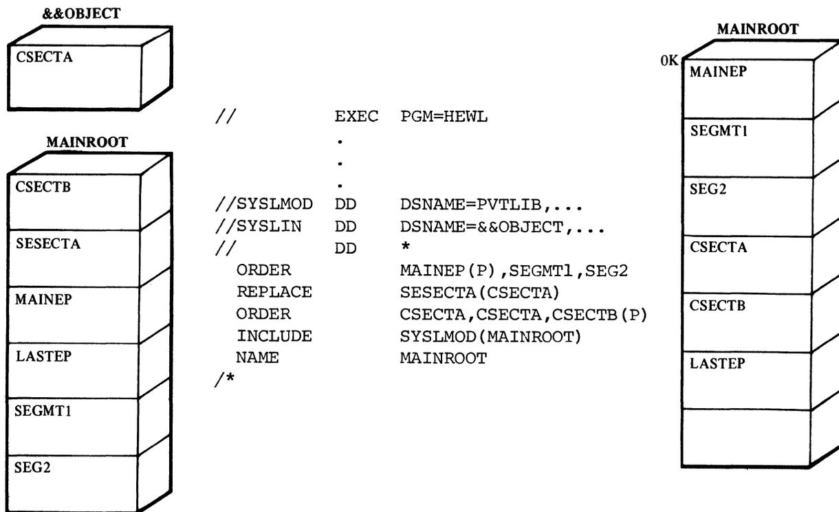
**Figure 32. Ordering Control Sections**
