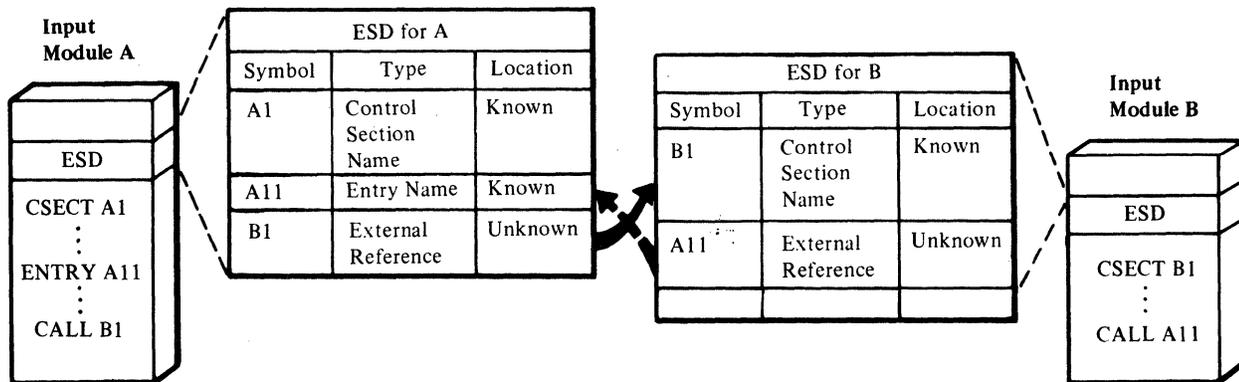
Figure 4. Use of the External Symbol Dictionary
