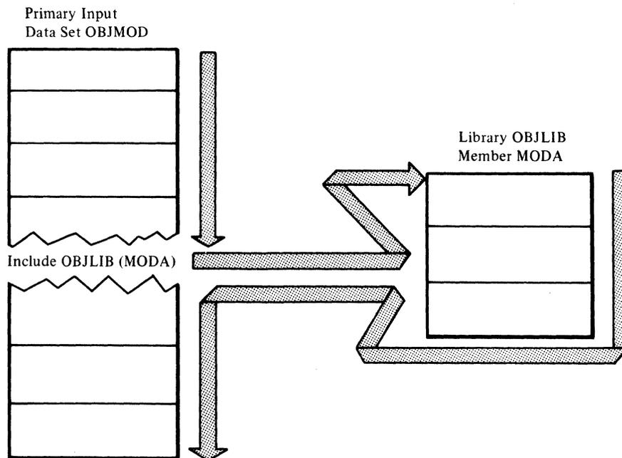
Figure 11. Processing of One INCLUDE Control Statement
