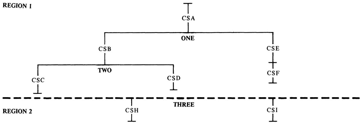
Figure 25. Overlay Structure for OVERLAY Statement Example
