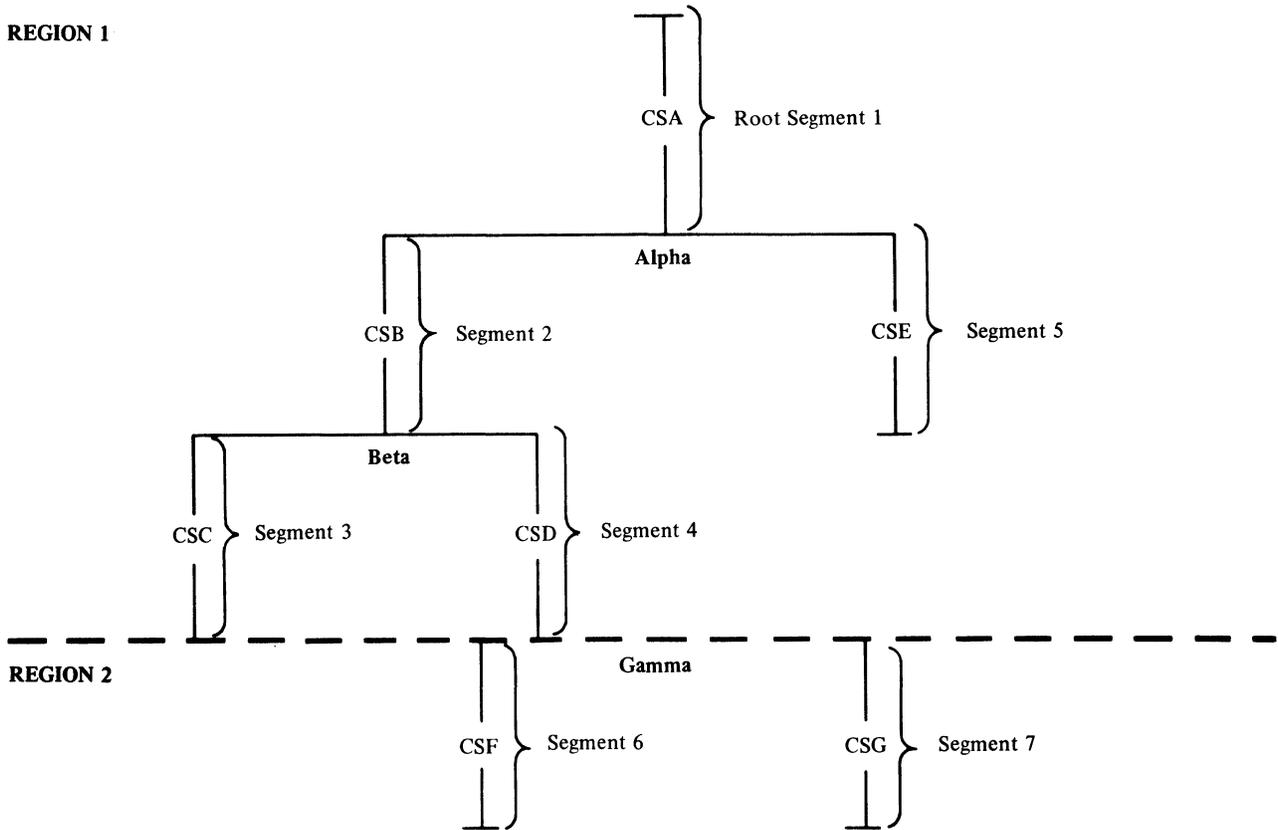
Figure 55. Overlay Tree for Multiple-Region Sample Program REGNOVLY
