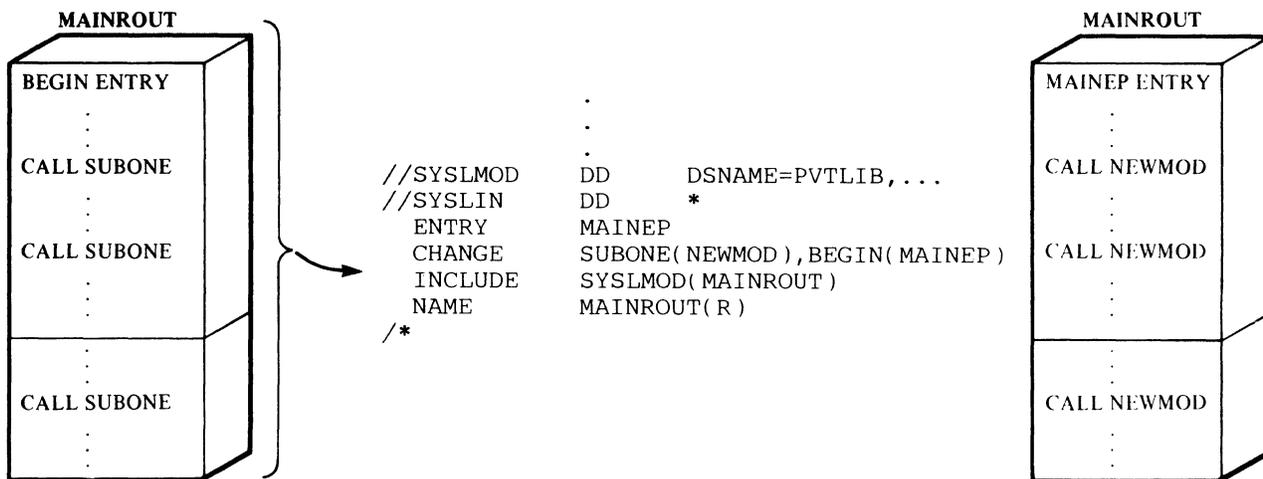
Figure 28. Changing an External Reference and an Entry Point
