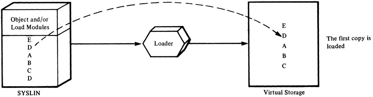
Figure 40. Loader Processing—Automatic Editing
