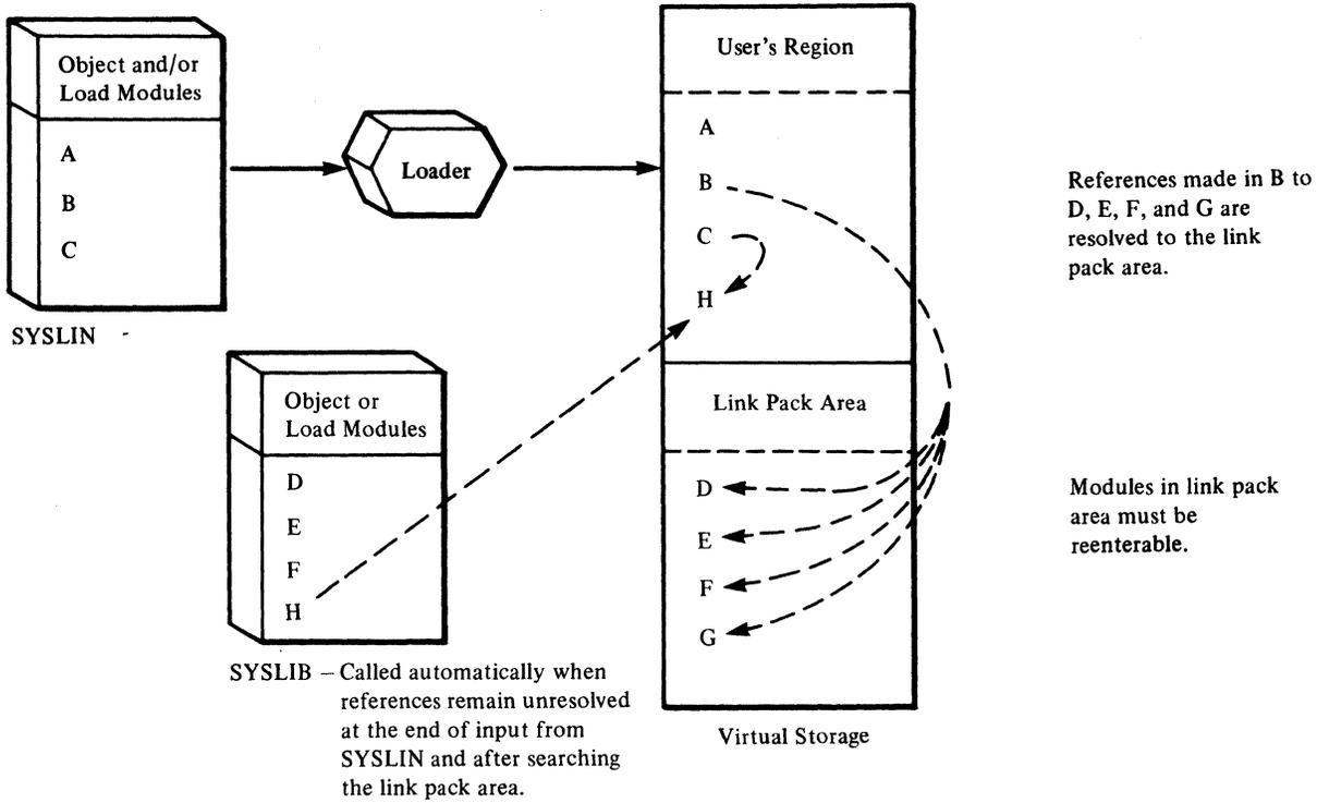
Figure 39. Loader Processing—Link Pack Area and SYSLIB Resolution
