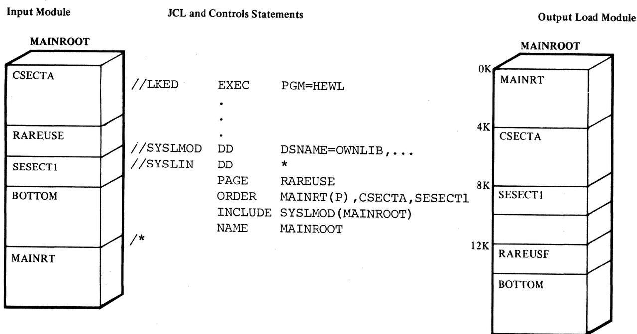
Figure 33. Aligning Control Sections on Page Boundaries
