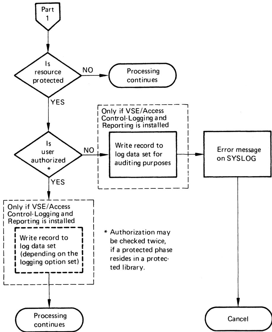
**Figure 3. Overall Structure of the Access Control Function of the VSE System (Part 2 of 2)**
