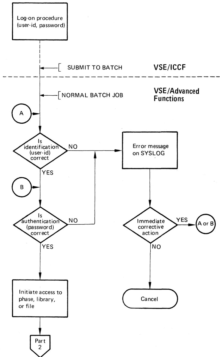
**Figure 3. Overall Structure of the Access Control Function of the VSE System (Part 1 of 2)**
