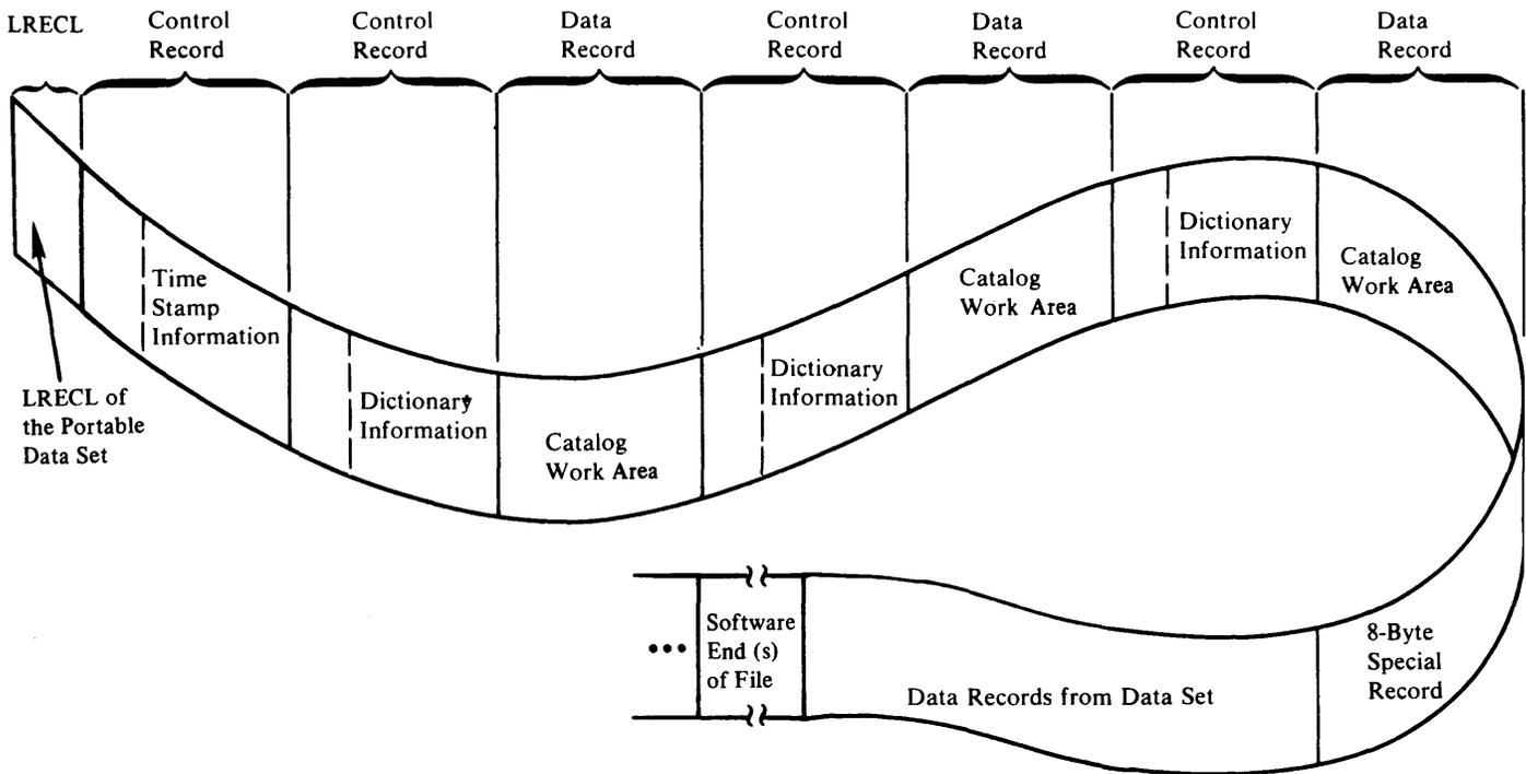
Figure 31. Layout of Control Records and Data Records in the Recovery Portable Data Set
