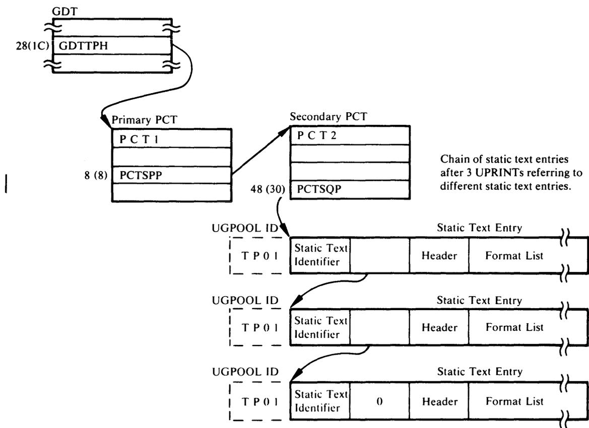
Figure 18. Text Processor Format Structure Queue
