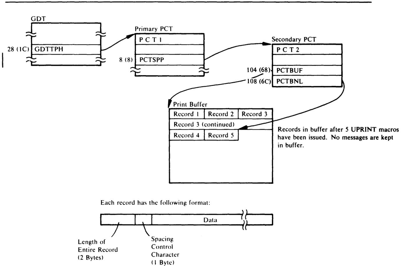
Figure 19. Text Processor Print Buffer
