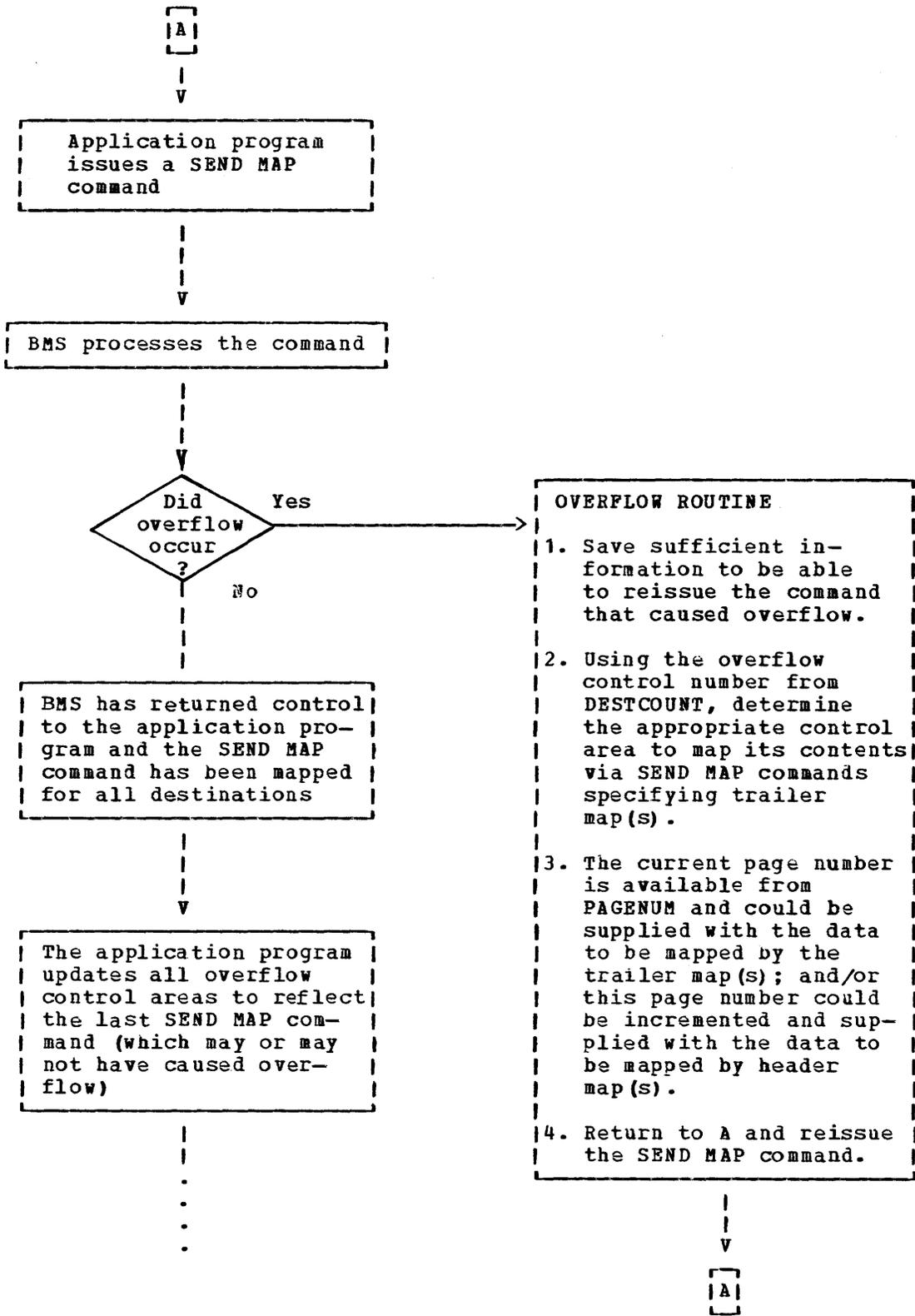
Figure 3.3-3. Overflow Processing
