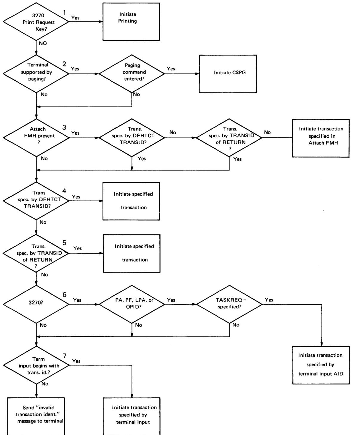
Figure 3.2-1. Terminal-Oriented Task Identification
