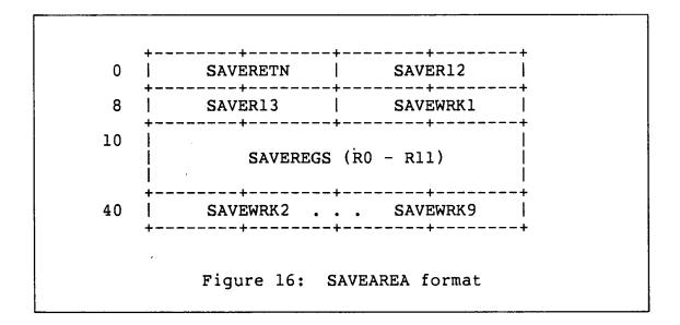
To improve system efficiency, CP initialization constructs a list of pre-allocated SAVEAREAS. SVC 8 (CALL) obtains the next element from the list, if available, and SVC 12 (EXIT) places the SAVEAREA back onto the list for re-use.
