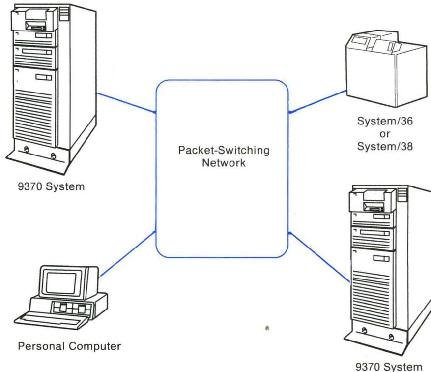
**Figure 3-19. Example of a Packet-Switching Network**
