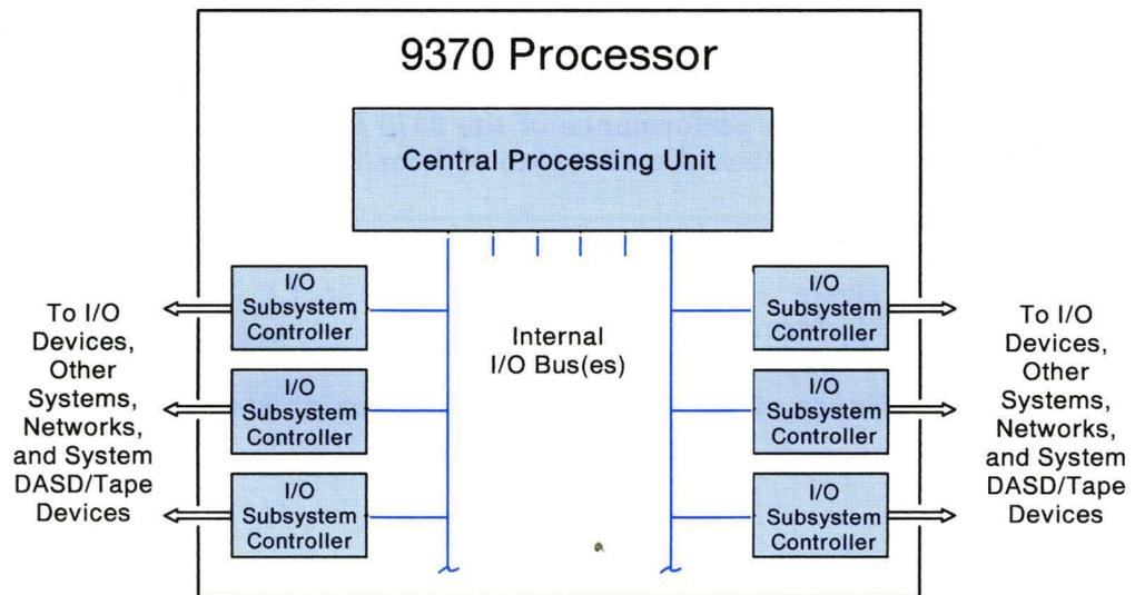
Figure 2-4. Basic 9370 Processor Structure
