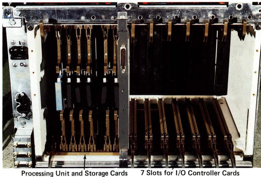
Figure 2-7. 9373 Processor Card Enclosure
