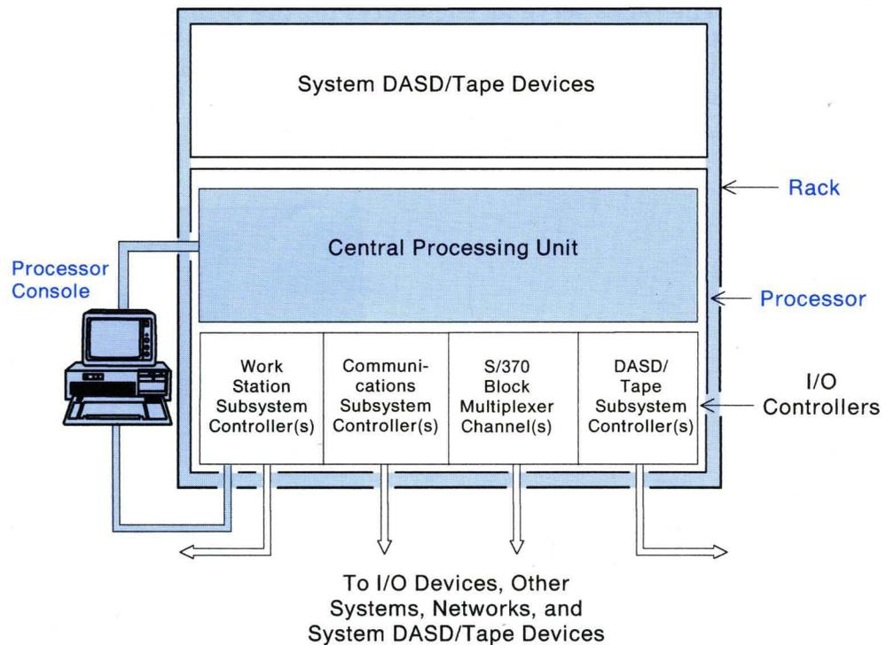
**Figure 2-1. Overview of System Components Described in Chapter 2**
