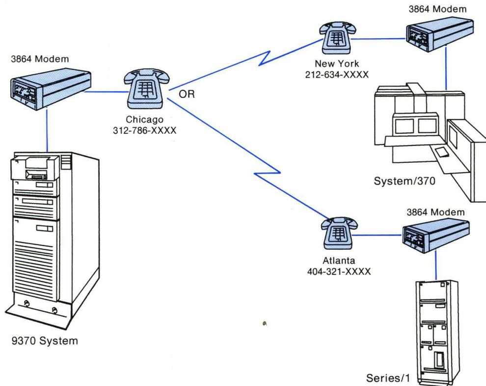
Figure 3-17. Example of a Switched Point-to-Point Network
