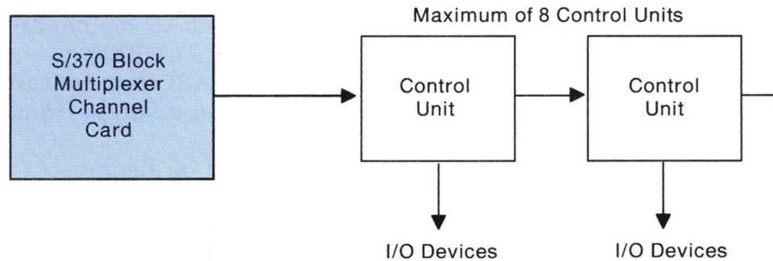
**Figure 3-8. S/370 Block Multiplexer Channel – Configuration Summary**
