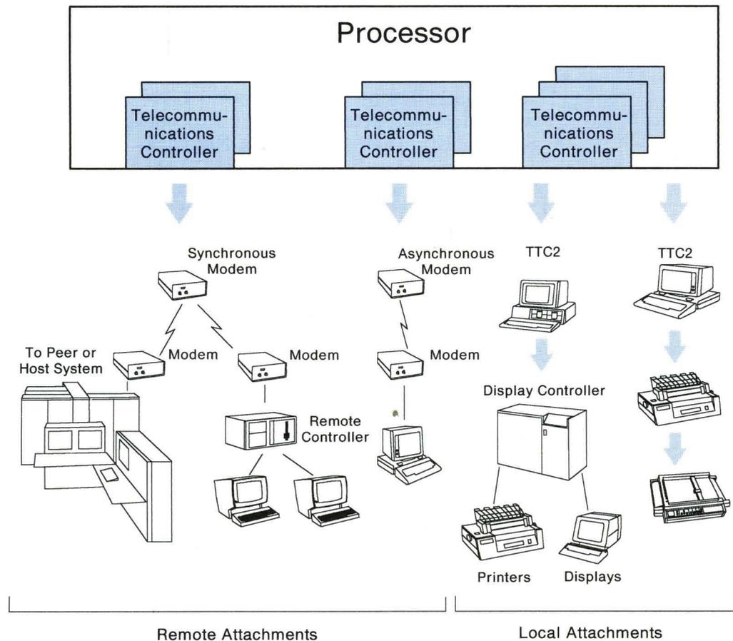
Figure 3-9. Telecommunications Subsystem
