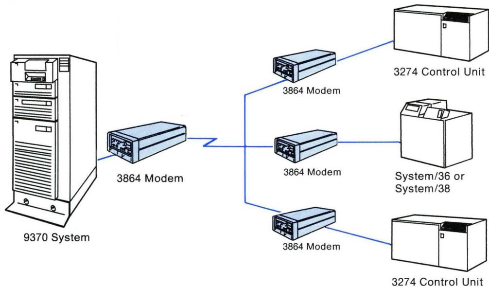
Figure 3-18. Example of a Nonswitched Multipoint Network
