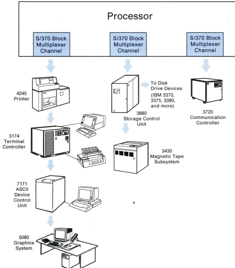
Figure 3-7. S/370 Block Multiplexer Channel and Attachable Devices
