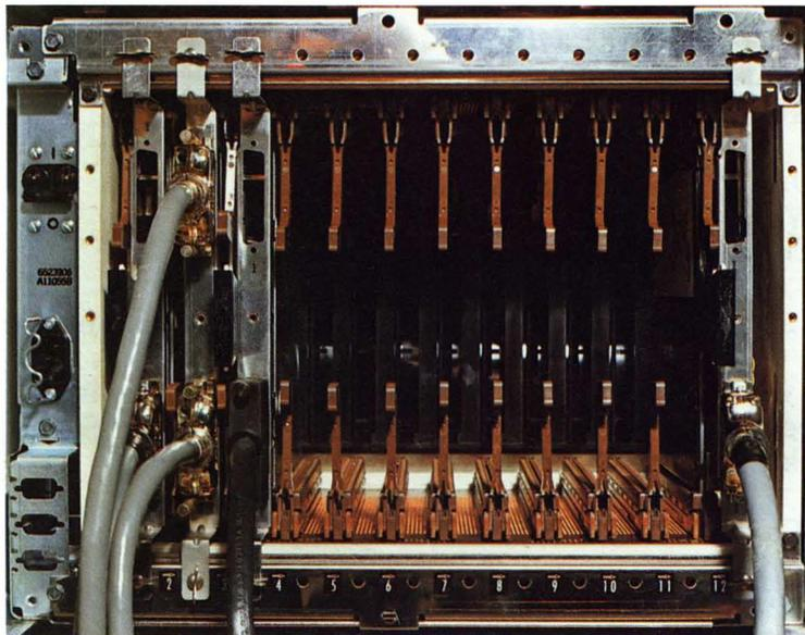
Figure 2-13. 9377 Processor I/O Card Unit With Two I/O Buses
