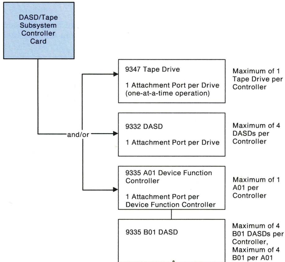
**Figure 3-4. DASD/Tape Subsystem Controller – Configuration Summary**
