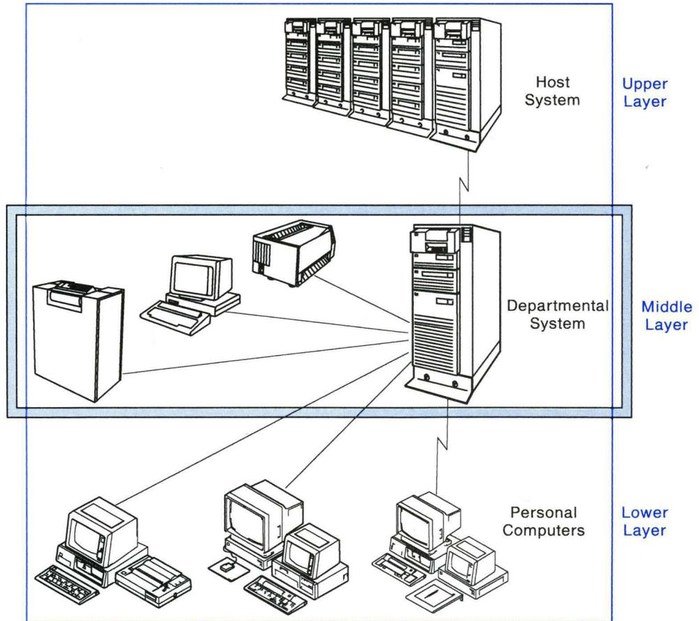
Figure 1-1. The 9370 System and its Environments
