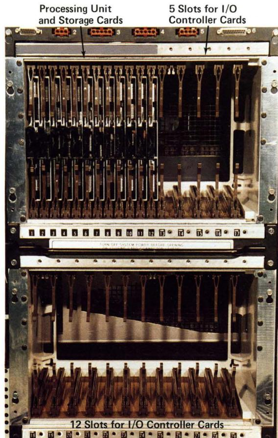
Figure 2-9. 9375 Processor Card Enclosures
