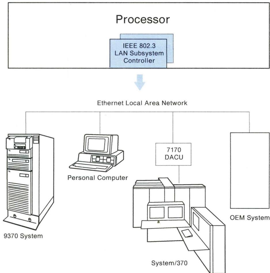
**Figure 3-15. IEEE 802.3 LAN Subsystem**
