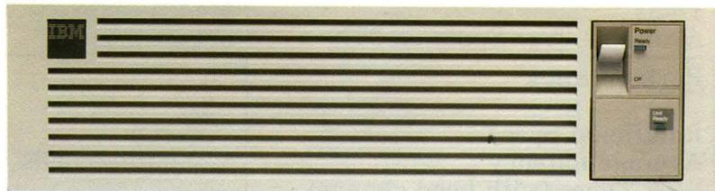
Figure 4-2. 9332 Direct-Access Storage Device
