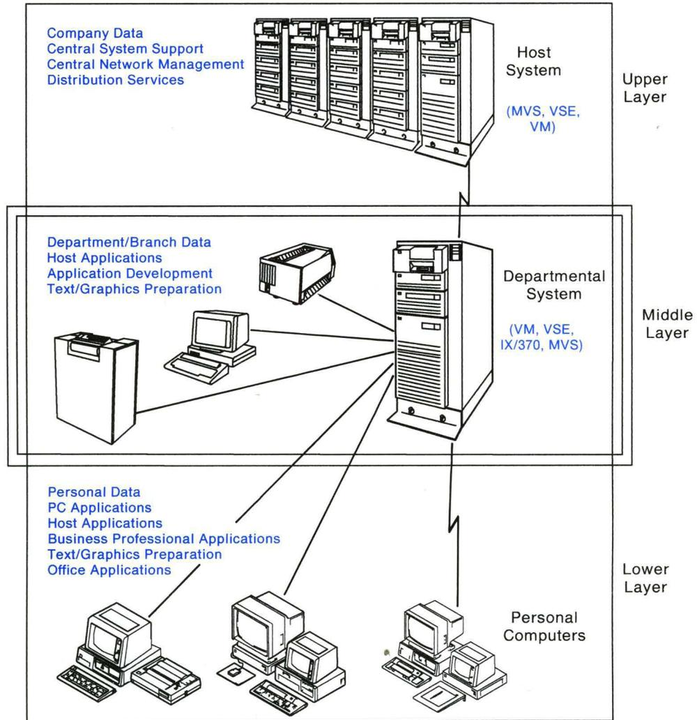
Figure 5-2. 9370 System, Operating Systems, and Environments
