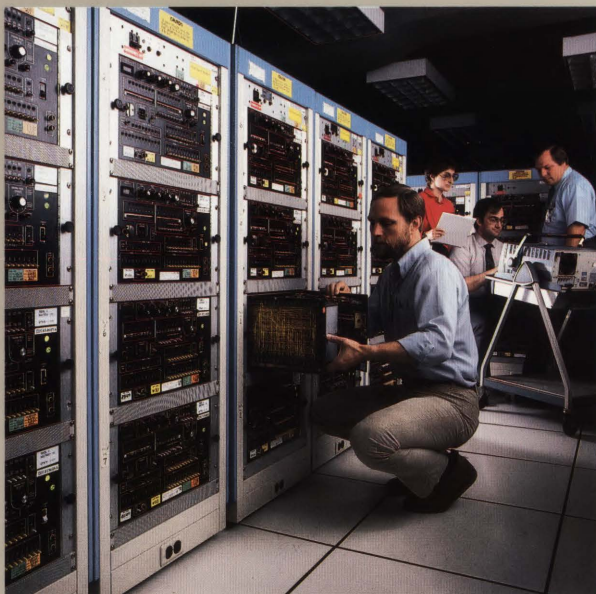
Systems product assurance personnel perform a series of tests to ensure that IBM 9370 systems meet design specifications.
