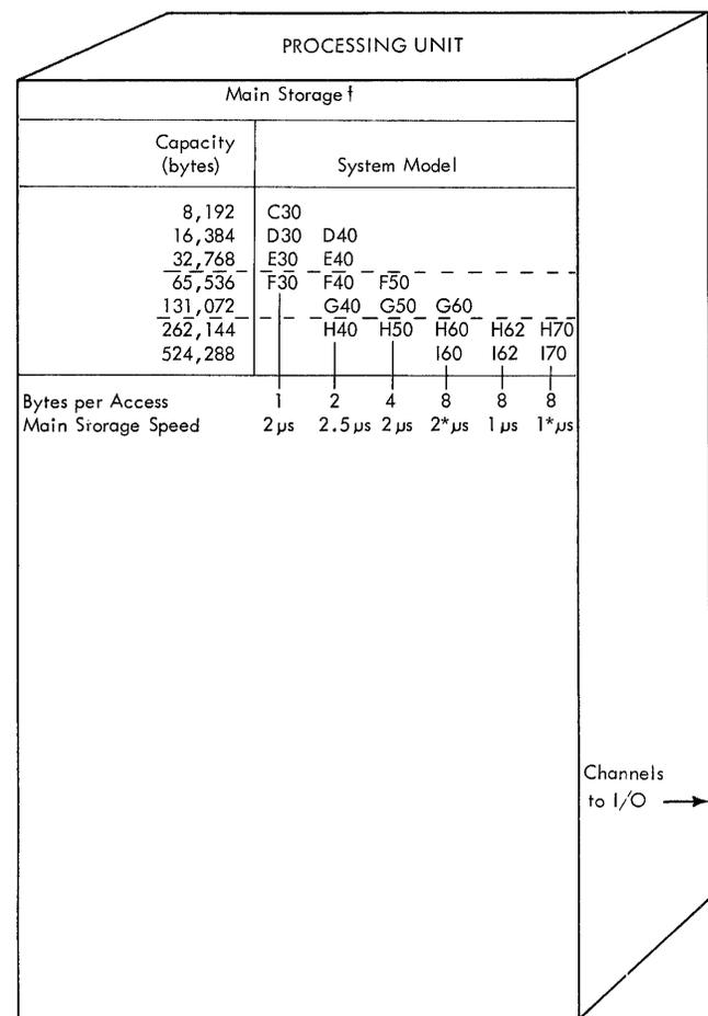
† Main Storage in Models 60-70 is housed externally to the processing unit.
