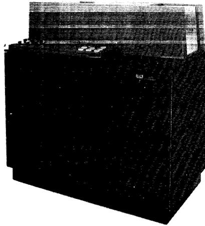
Figure 25. IBM 1231 Optical Mark Page Reader
