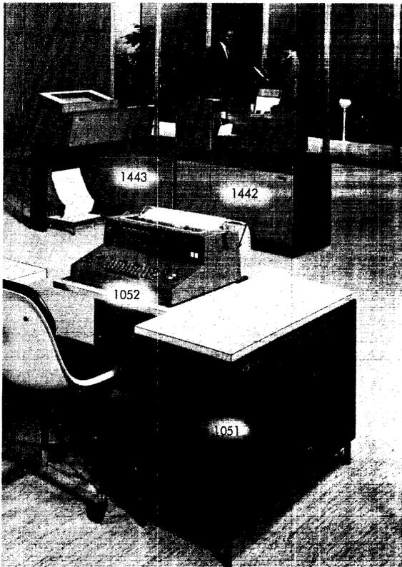
Figure 10. IBM 1052 Printer-Keyboard, 1051 Control Unit, 1443 Printer, and 1442 Card Read Punch
