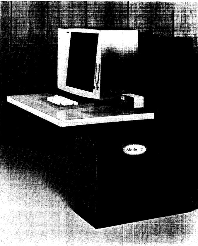
Figure 8. IBM 2250 Display Unit
