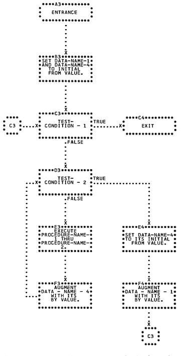
Figure 22. Logical Flow of Option 4 PERFORM Statement Varying Two Data-names.
