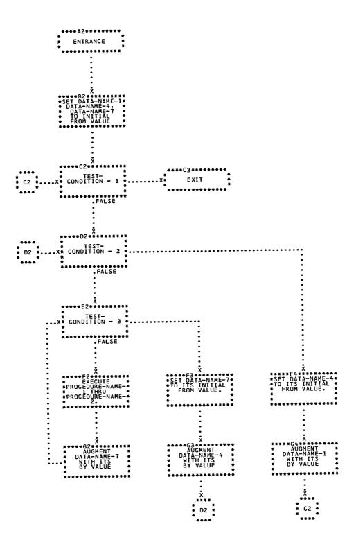
Figure 23. Logical Flow of Option 4 PERFORM Statement Varying Three Data-names.
