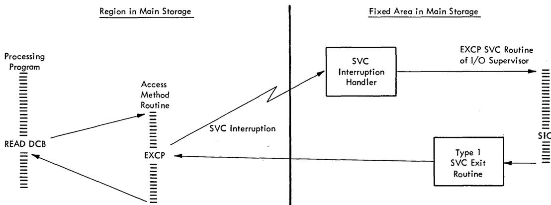
Figure 28. Flow of Control for an I/O Operation
