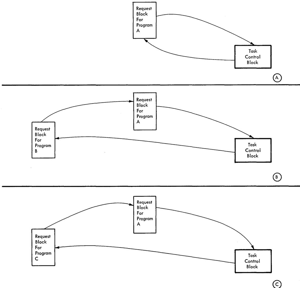
Figure 22. Example of the Modification of the RB Queue During a Task
