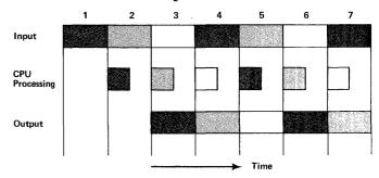
Figure 8. Concurrent Input, Processing, and Output
