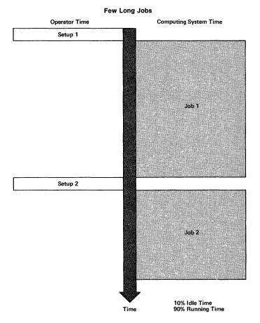
Figure 19. The Running Time of a Computing System When Processing a Few Long Jobs
