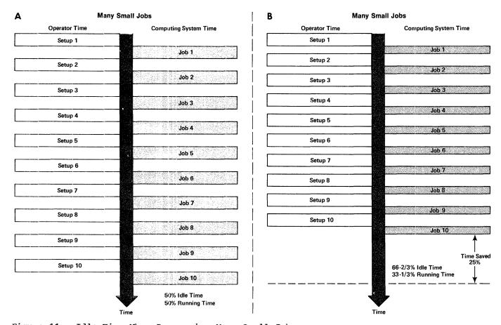
Figure 11. Idle Time When Processing Many Small Jobs
