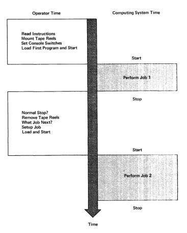
Figure 10. Idle Computing System Time Between Jobs
