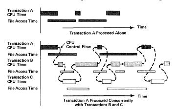
Figure 22. Comparison Between the Processing of Transactions Singly and Concurrently
