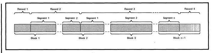
Figure 52. Spanned Variable-Length Records
