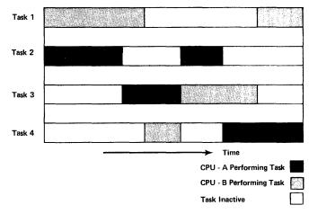
Figure 60. Two CPUs in Multisystem Mode, Balancing the Execution of Four Tasks
