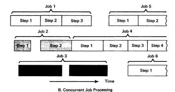
Figure 47. Sequential and Concurrent Job Processing
