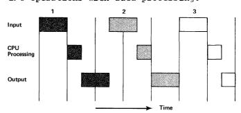
Figure 7. Sequential Input, Processing, and Output
