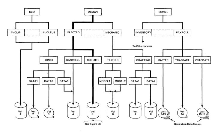
Figure 53. Simplified Diagram of Catalog System for Locating a Volume
