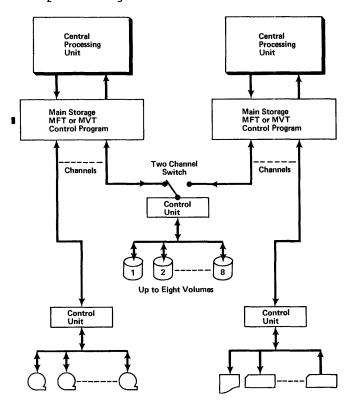
Figure 58. Multiprocessing With Shared Direct Access Storage Devices
