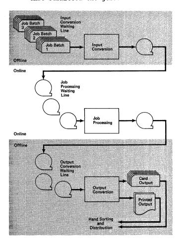
Figure 48. Offline Peripheral Operations
