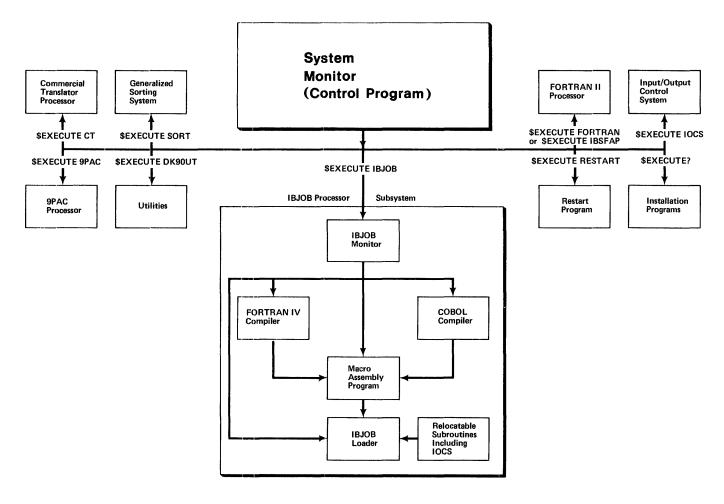
Figure 18. IBM 7090/7094 IBSYS Operating System
