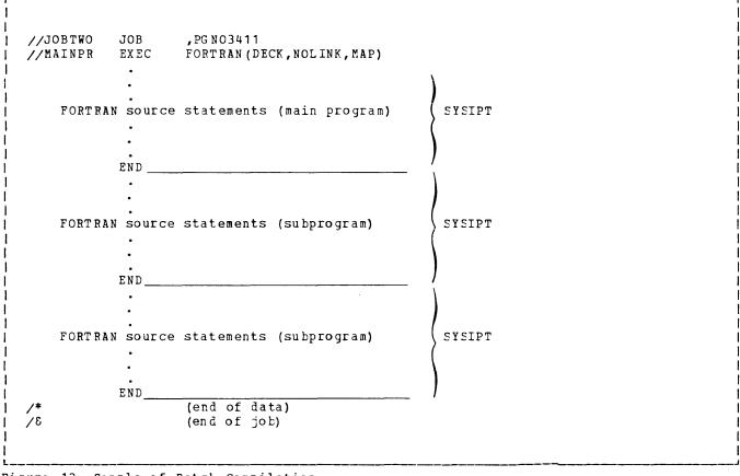
Figure 12. Sample of Batch Compilation
