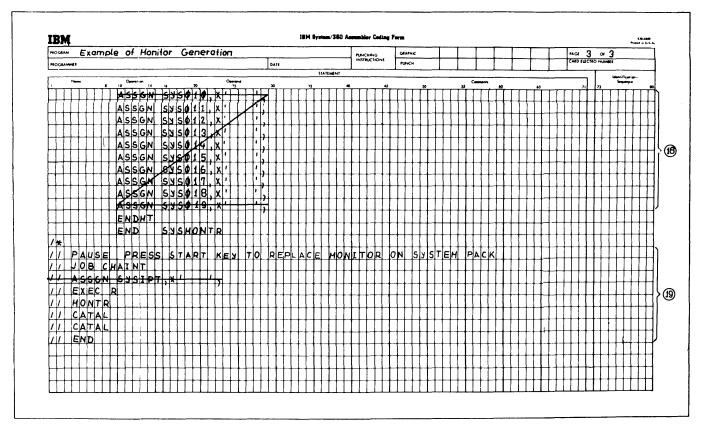
Figure 10. Monitor Generation, Example D (Part 2 of 2)
