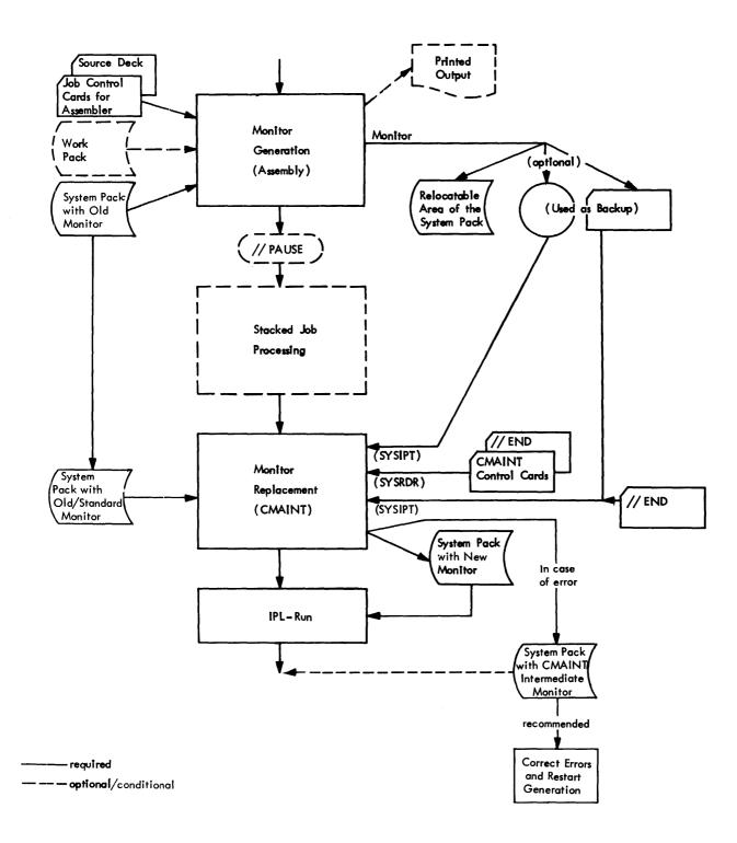
Figure 11. Generating a Disk-Resident Monitor and Including It on the System Pack
