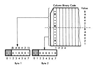
Figure 15. Column Binary Reading of the \$-Sign
