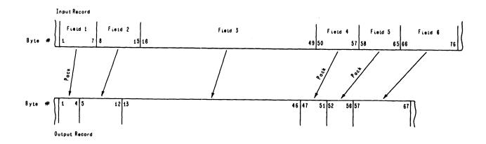
Figure 7. Record Formats for Disk-to-Disk Transfer Problem
