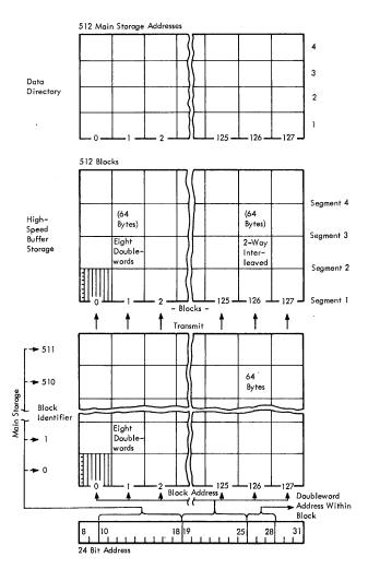
Figure 5. High Speed Buffer Storage
