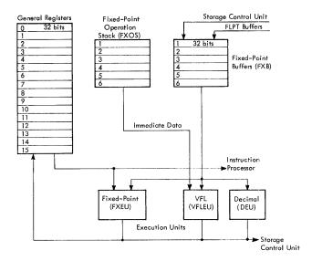
Figure 7. Fixed-Point/VFL/Decimal Execution Element
