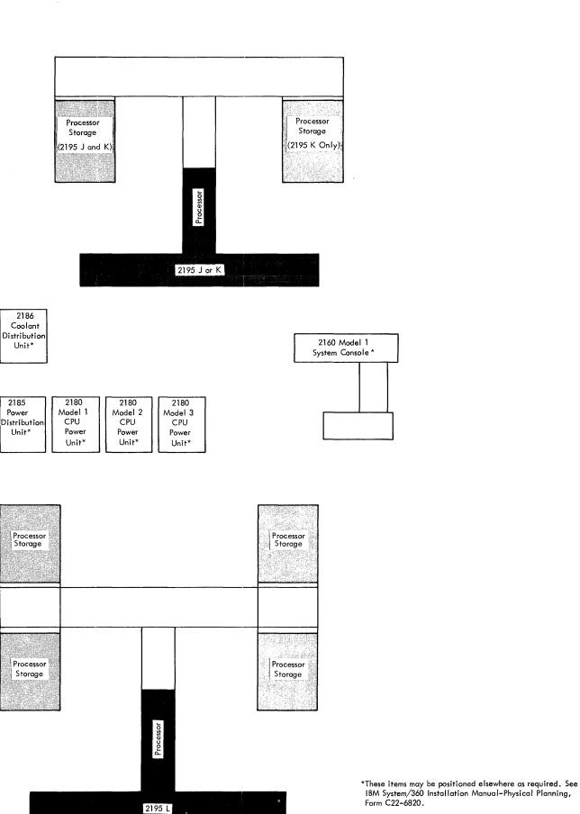
Figure 2. IBM 2195 J, K, L Processing Unit and Processor Storage Configurations
