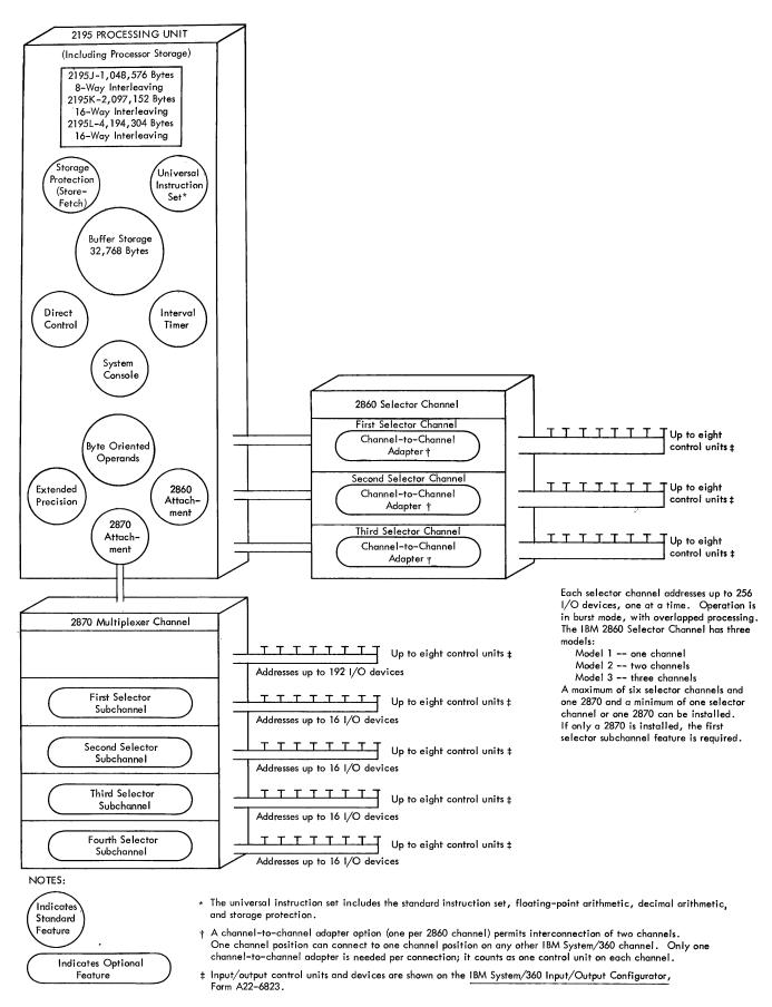
Figure 1. System/360 Model 195 Configurator
