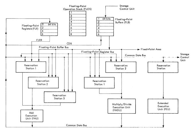
Figure 8. Floating-Point Execution Element
