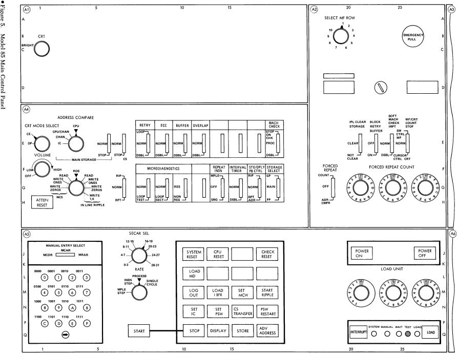
Figure σι Model 85 Main Control Panel
