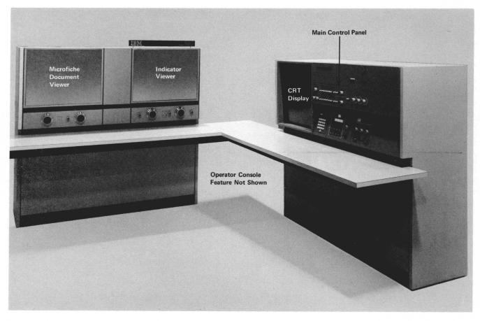
• Figure 3. Model 85 System Control Panel
