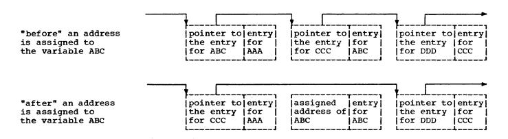
Figure 60. Removing an Entry From the Middle of a Dictionary Chain
