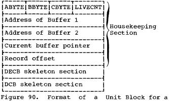
Figure 90. Format of a Unit Block for a Sequential Access Data Set
