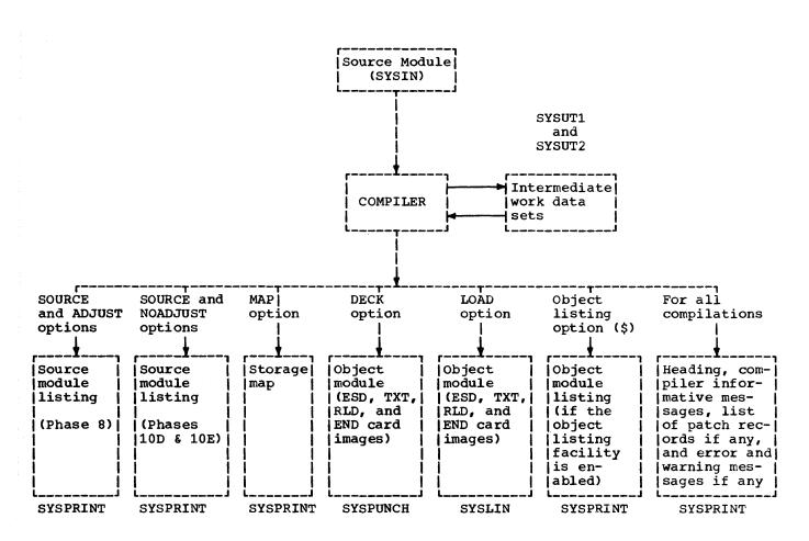
Figure 1. Compiler Input/Output Structure
