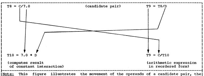
Note: This figure illustrates the movement of the operands of a candidate pair, the text entries of which both have multiplicative operators. The operators in the resultant text entries, T10=7.0\*D and T9=C/T10, are obtained from the operator table. The text entry T10=7.0\*D which computes the result of the interaction of the constants, is placed into the back target. (In this application; D is assumed to be a stored (constant.)
