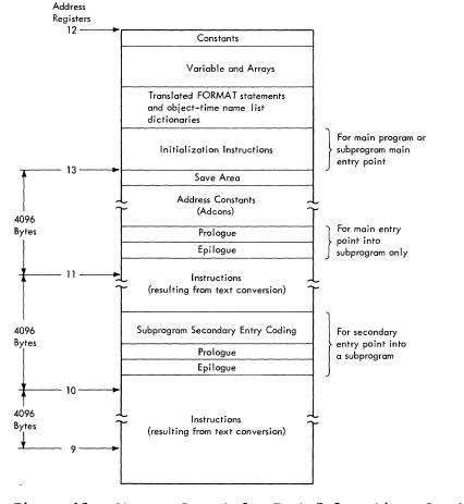
Figure 12. Storage Layout for Text Information Construction
