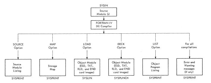
Figure 0. Input/Output Data Flow
