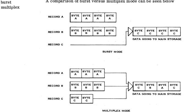
A comparison of burst versus multiplex mode can be seen below
