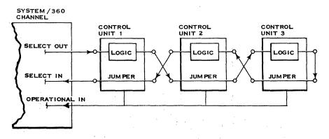
As can be seen in the illustration, the Select Out line proceeds through each I/O unit in series and returns to the channel as the \_\_\_\_\_\_ line.
