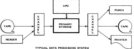
The preceding figure shows a typical data processing system, such as System /360. Data processing consists of three steps: Input, Processing, and Output. The elements of the system which perform these steps are:
