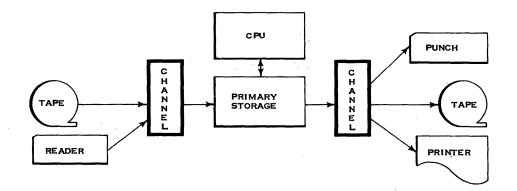
Channels are logical concepts in I/O operations. In the System/360, they may be stand-alone units as in the Model 75 or may be packaged along with main storage in the CPU housing as in the Model 30. In the lower models of the System/360, many of the processing units' circuits are used by the channels for their functions. There are two types of channels used by System/360: 1) selector channels, and 2) multiplexor channels. Let's discuss the selector channels first.
