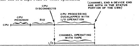
After it has been stored, the CPU program can interrogate the device status byte. If both the channel end and device end bits are present, the CPU program knows that both the I/O device and the channel are available for another operation.
