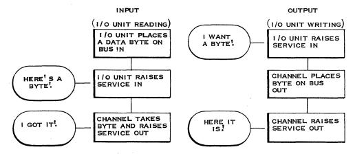
NOTE: For channels operating in multiplex mode, the I/O device would have to be re-selected for each data handling sequence.
