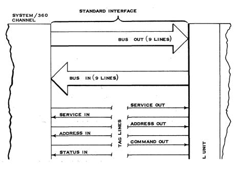
The three "out tag lines" would identify the byte on the Bus Out lines while the three "in tag lines" would identify the byte on the \_\_\_\_\_ lines.
