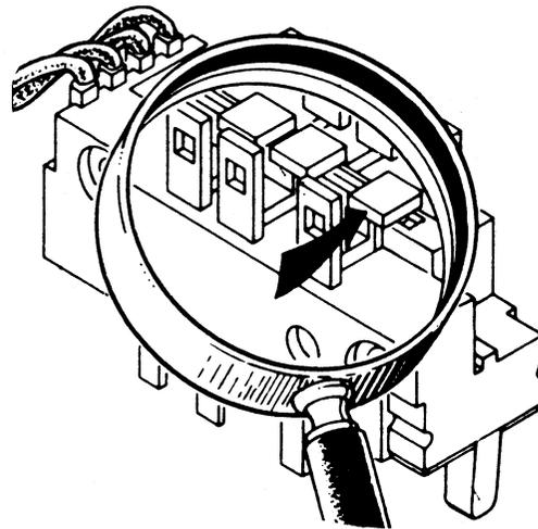
Figure 2-27. Checking Common Contact
