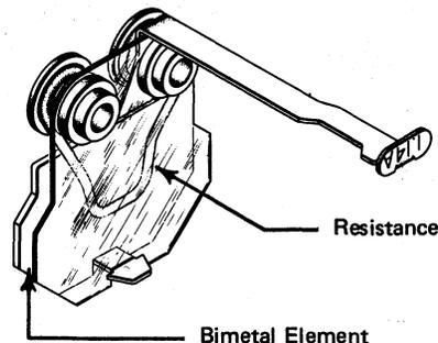
Figure 1-2. Thermal Switches
