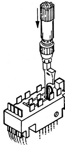
Figure 2-24. Positioning Contact Wire
