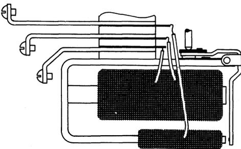
Figure 2-47. Three-Coil Duo Relay
