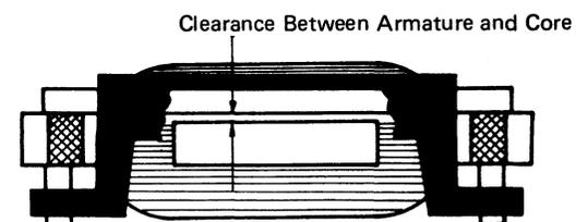
Figure 2-18. PM Relay Armature and Core
