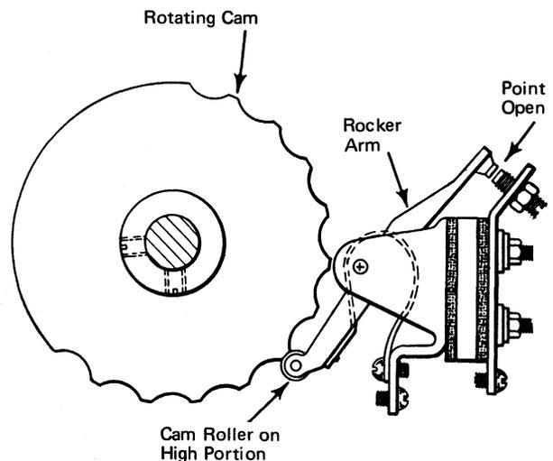
Figure 3-1. Rocker Arm Circuit Breaker
