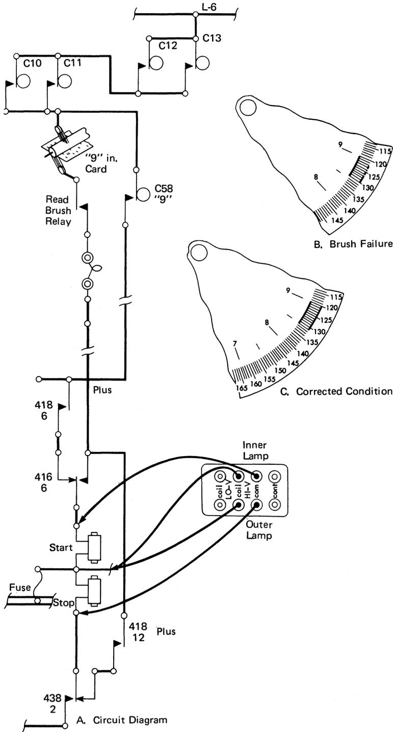
Figure 4-22. Checking Reading Brush Impulses
