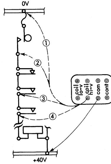
Figure 4-24. Checking Continuity +40V Common
