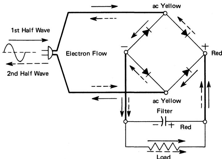
Figure 5-4. Full-Wave Metallic Rectifier Circuit
