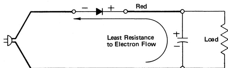
Figure 5-3. Half-Wave Metallic Rectifier Circuit
