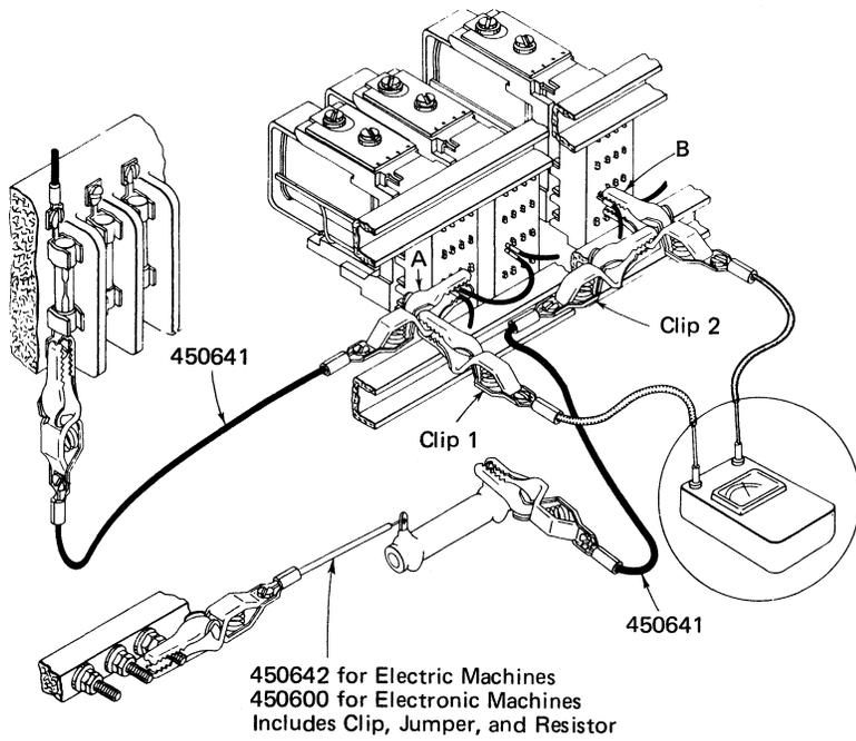
Figure 5-11. Connections for Measuring Contact Resistance
