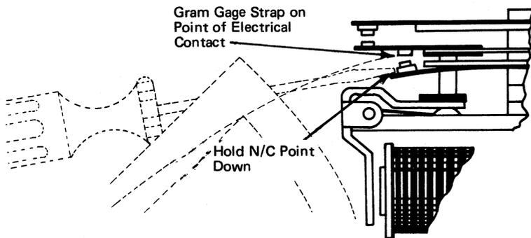
Figure 2-43. Contact Strap Tension
