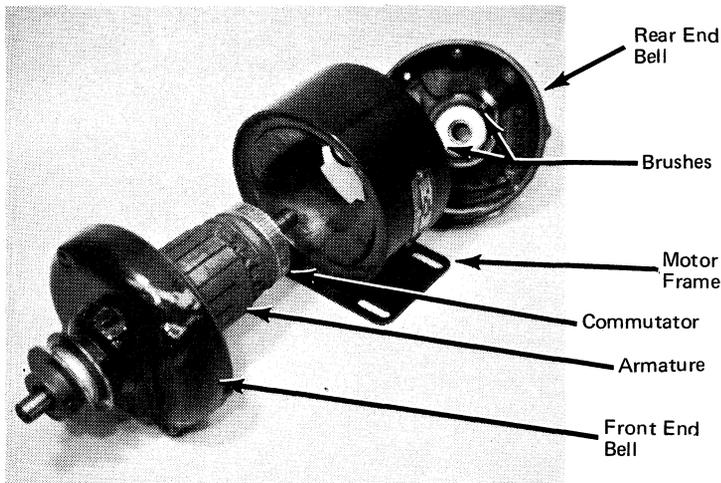
Figure 1-21. Typical DC Motor
