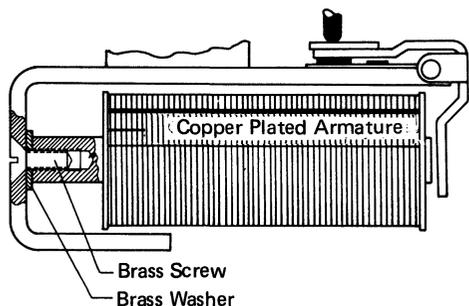
Figure 2-36. Copper Plated Armature
