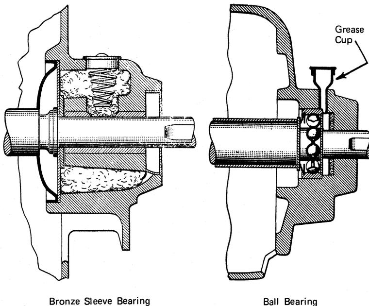
Figure 1-3. Motor Bearings
