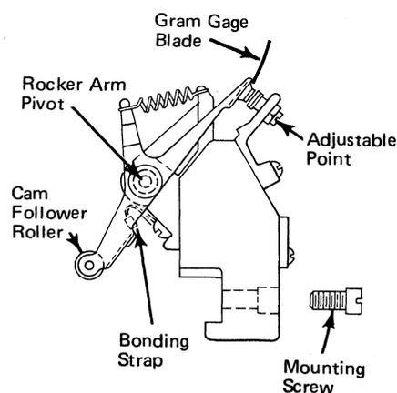
Figure 3-5. Unitized Rocker Circuit Breaker
