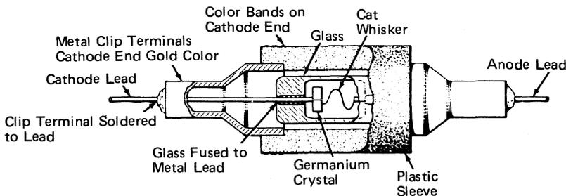
Figure 5-10. Plastic Enclosed Germanium Diode
