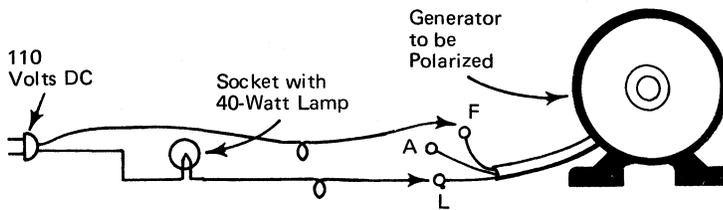
Figure 1-27. Temporary Wiring to Use 110 Volts DC for Polarization of a Generator
