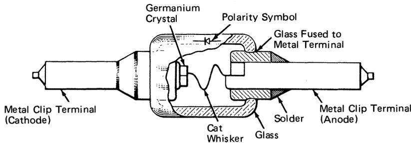
Figure 5-9. Glass Enclosed Germanium Diode
