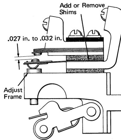
Figure 3-20. Plunger Circuit Breaker Roller Type—Adjustment 2
