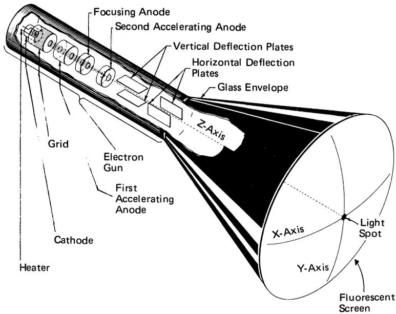
Figure 4-30. Cathode-Ray Tube
