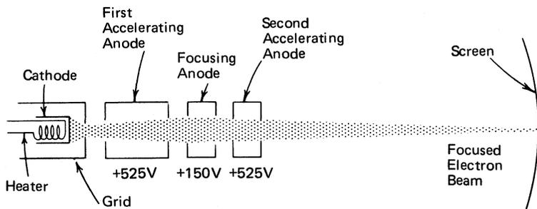
Figure 4-31. Electronic Focusing
