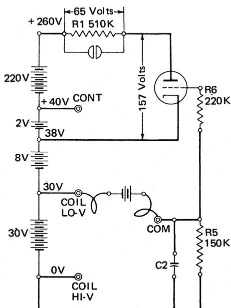
Figure 4-19. Coil Low-Voltage Connection Schematic
