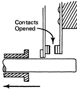
Figure 1-13. Start Switch in Running Position
