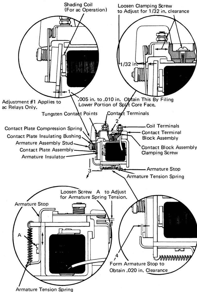
Figure 2-58. IBM Unit Heavy-Duty Relay Adjustments
