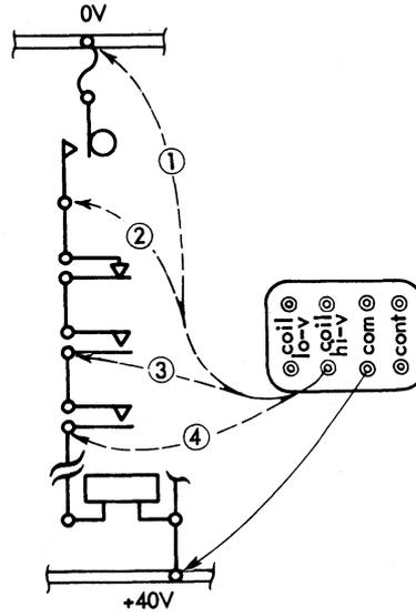
Figure 4-24. Checking Continuity +40V Common
