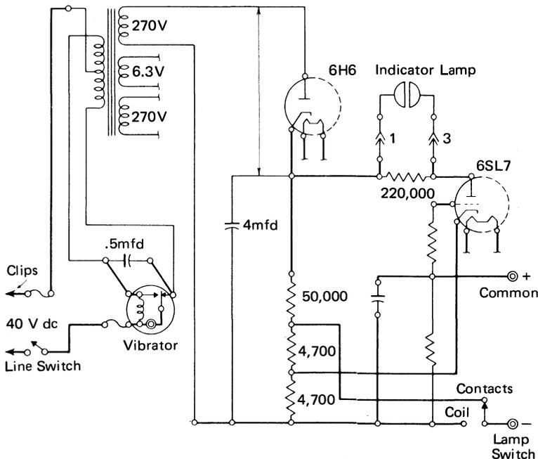
Figure 4-12. Power Pack Block Diagram
