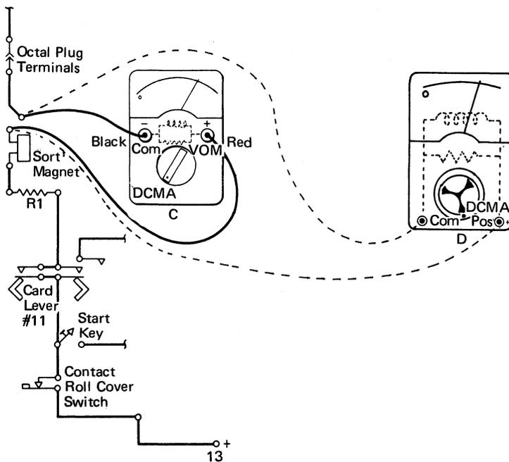
Figure 4-4. Current Measurement Style C and D Meters
