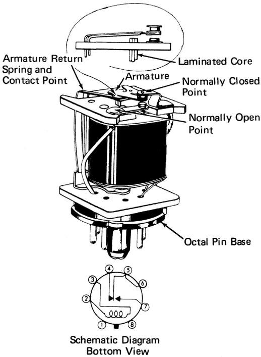
Figure 2-61. Octal-Base Pluggable High-Speed Relay
