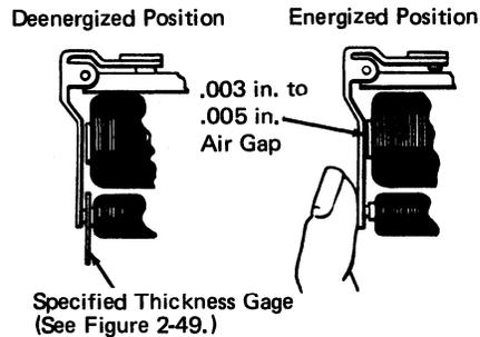
Figure 2-41. Armature Air-Gap Double Coil
