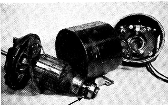
Bearing Retaining Plate
