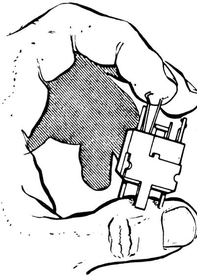
Figure 2-28. Replacing Contact Wires
