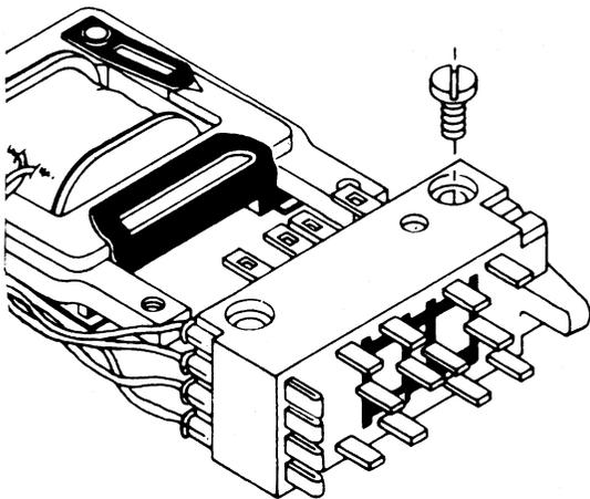
Figure 2-25. Disassembling Relay
