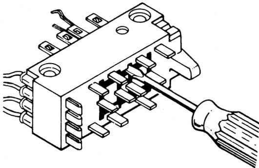
Figure 2-26. Removing Contact Wire
