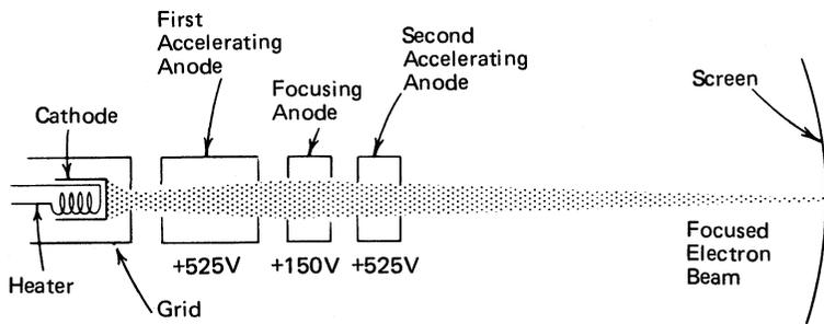
Figure 4-31. Electronic Focusing
