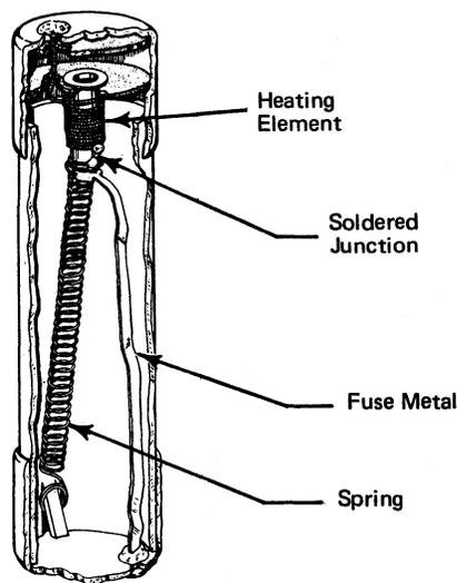
Figure 1-1. Thermal Fuse
