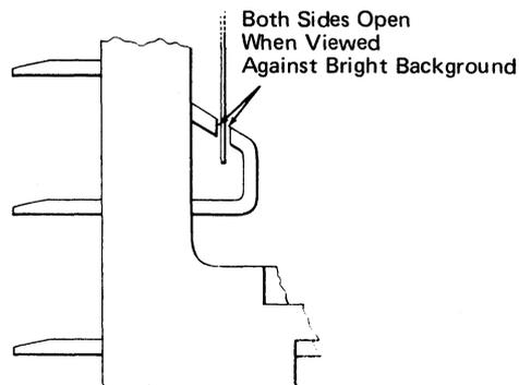
Figure 2-6. Checking Wires
