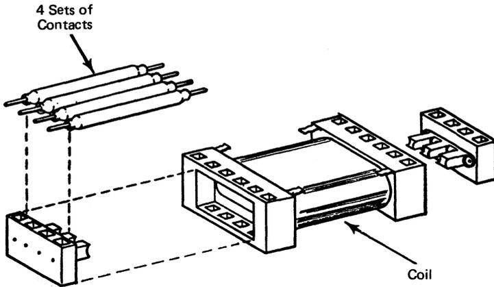
Figure 2-53. Reed Relay Construction
