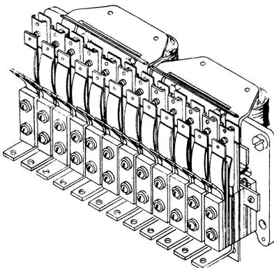
Figure 2-65. Multi-Contact Relay
