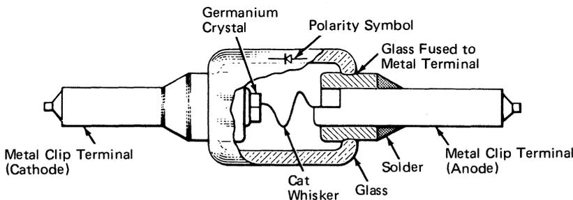
Figure 5-9. Glass Enclosed Germanium Diode
