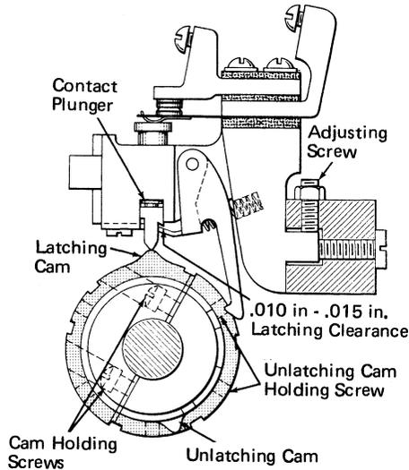
Figure 3-13. Latching Plunger Circuit Breaker
