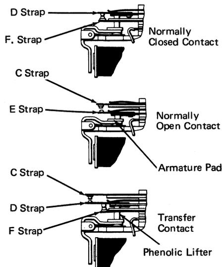
Figure 2-37. Contact Strap Tension
