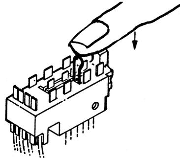
Figure 2-23. Replacing Contact Wire
