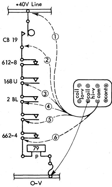
Figure 4-23. Checking Continuity 0V Common
