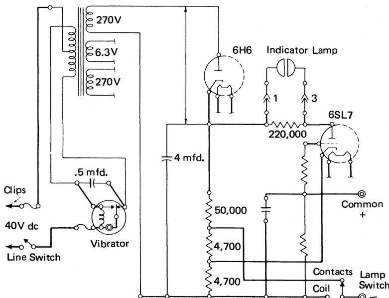
Figure 4-27. Portable Dynamic Timer Circuit Schematic
