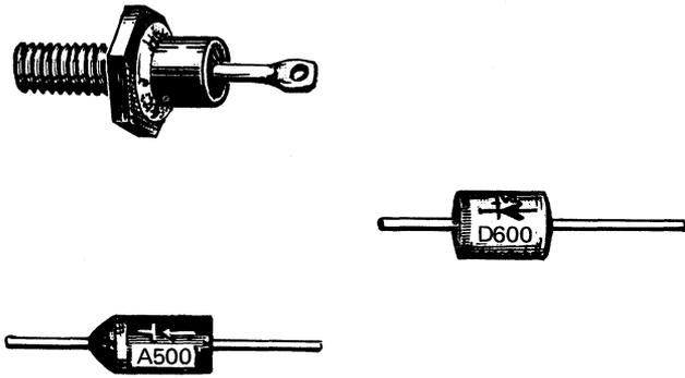
Figure 5-8. Types of Silicon Rectifiers
