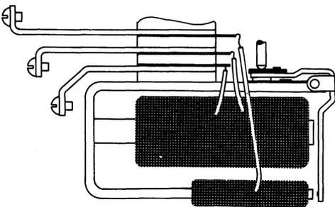
Figure 2-47. Three-Coil Duo Relay
