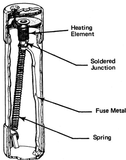
Figure 1-1. Thermal Fuse
