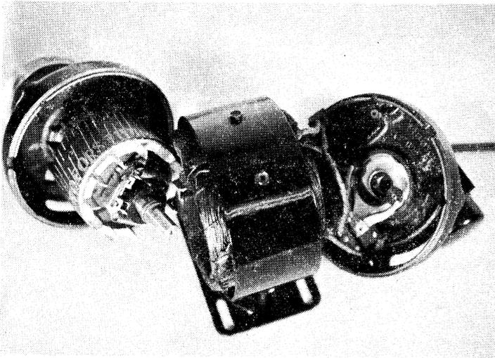
Figure 1-5. Typical AC Motor
