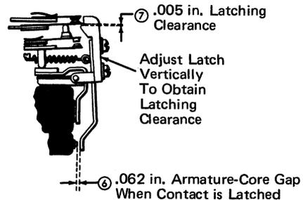
Figure 2-48. Duo Latch Relay
