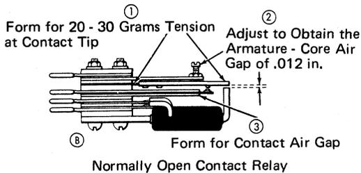
Figure 2-59. Pluggable High-Speed Relay
