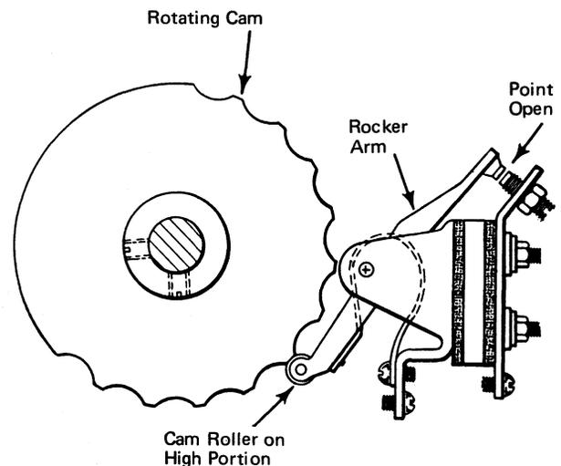
Figure 3-1. Rocker Arm Circuit Breaker
