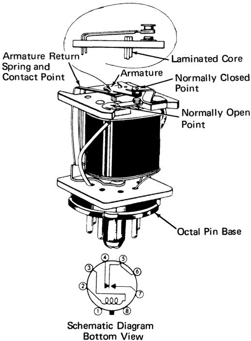
Figure 2-61. Octal-Base Pluggable High-Speed Relay
