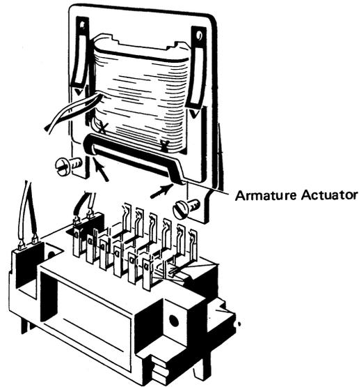
Figure 2-32. Defective Armature
