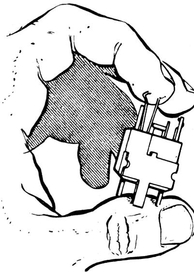
Figure 2-28. Replacing Contact Wires
