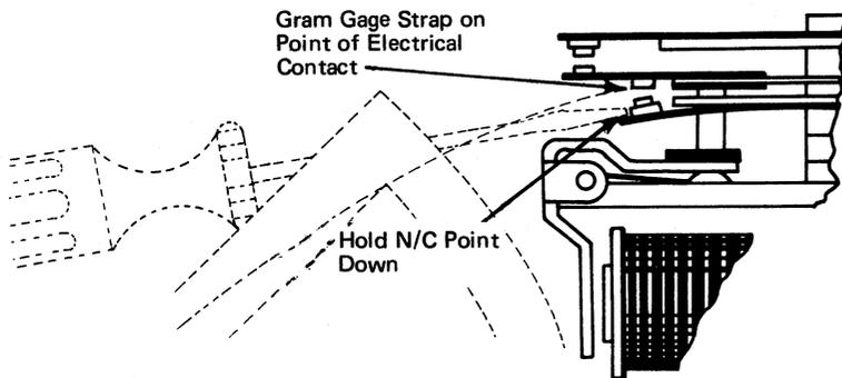
Figure 2-43. Contact Strap Tension
