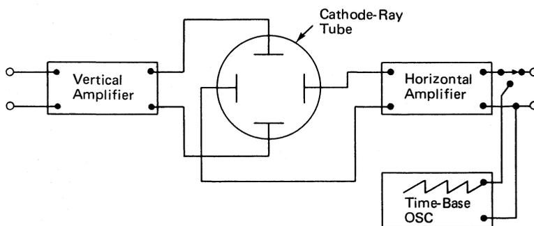
Figure 4-29. Oscilloscope Block Diagram
