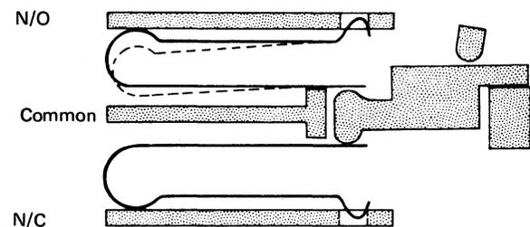
Figure 2-17. PM Relay Contacts—Operated
