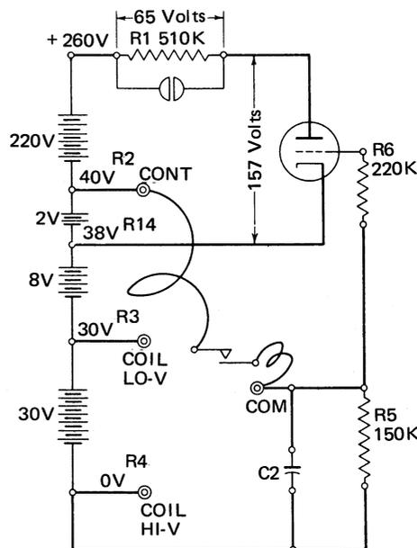
Figure 4-18. Contact Connection Schematic
