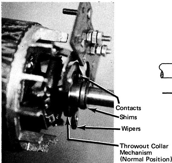
Figure 1-12. Start Switch in Normal Position
