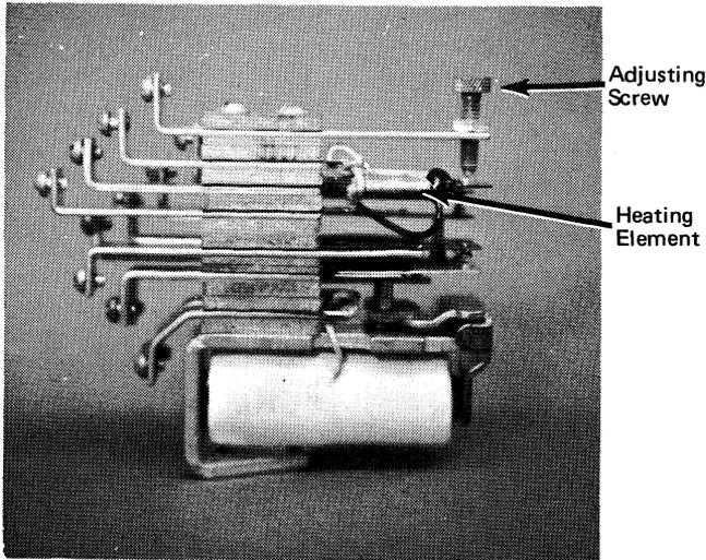
Figure 2-46. Thermal Delay (TD) Relay
