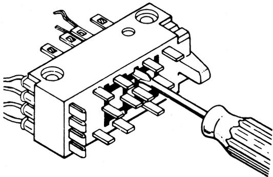
Figure 2-26. Removing Contact Wire
