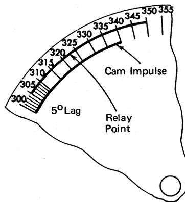
Figure 4-25. Checking Relay Pick Time
