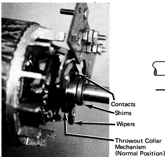
Figure 1-12. Start Switch in Normal Position
