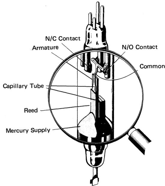
Figure 2-72. Mercury Relay Construction
