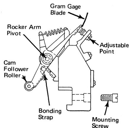
Figure 3-5. Unitized Rocker Circuit Breaker
