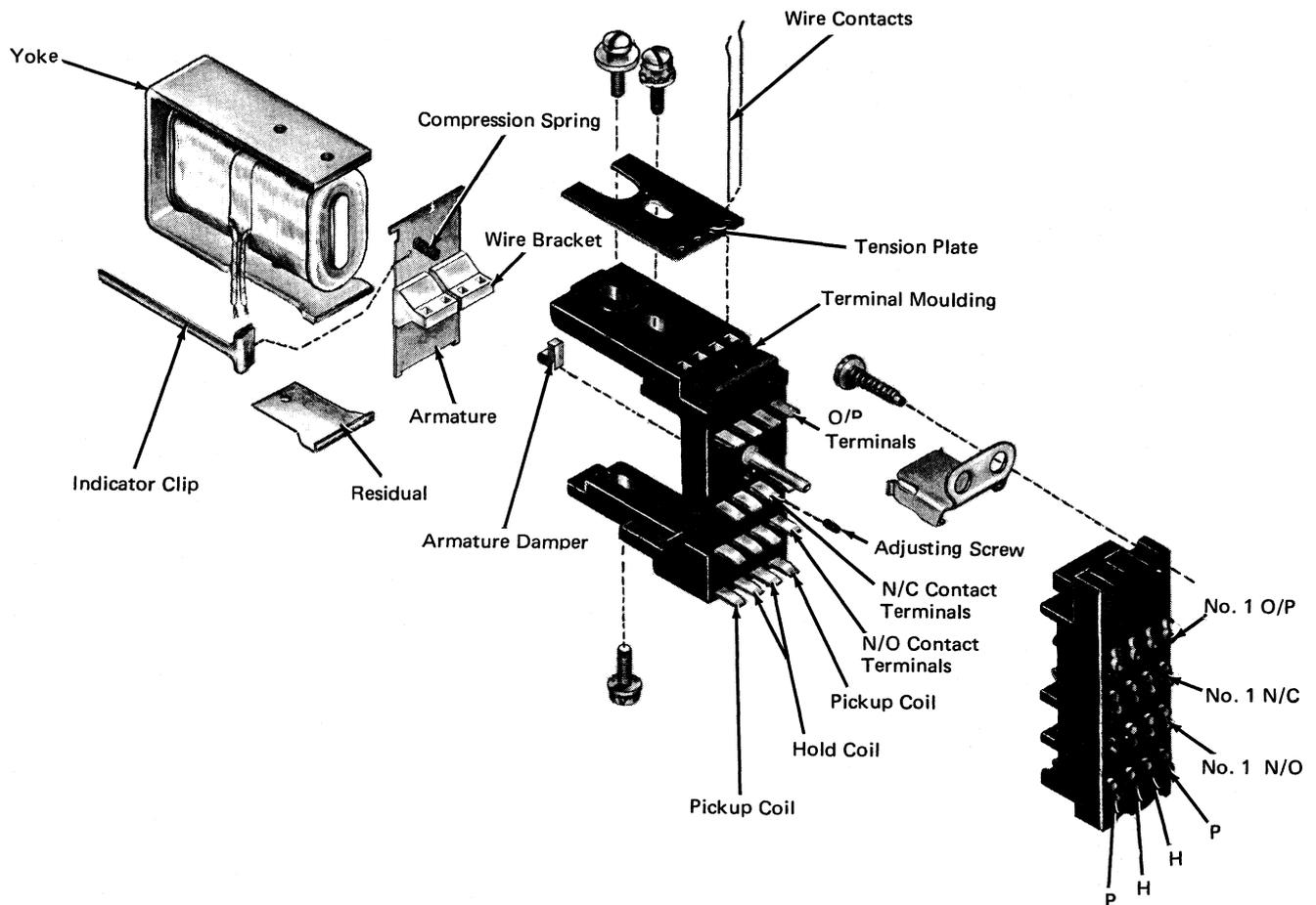
Figure 2-3. Wire Contact Relay
