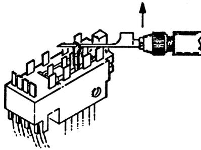
Figure 2-22. Removing Contact Wire
