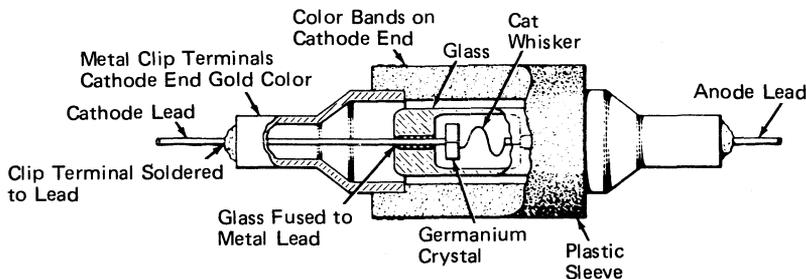
Figure 5-10. Plastic Enclosed Germanium Diode
