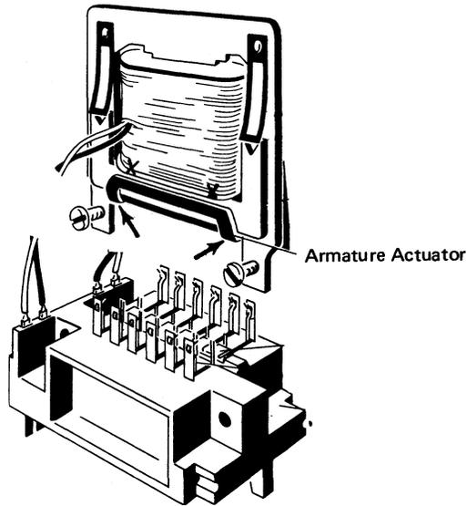
Figure 2-32. Defective Armature
