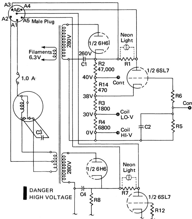
Figure 4-13. Power Pack Circuit
