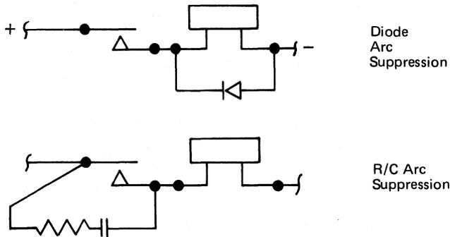
Figure 2-1. Relay Arc Suppression
