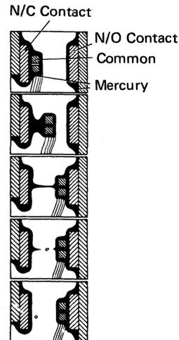
Figure 2-73. ARC Absorption
