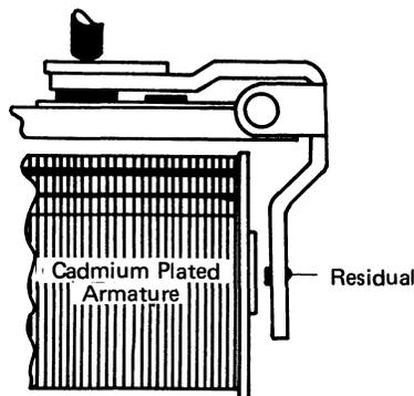
Figure 2-35. Residual Type Armature
