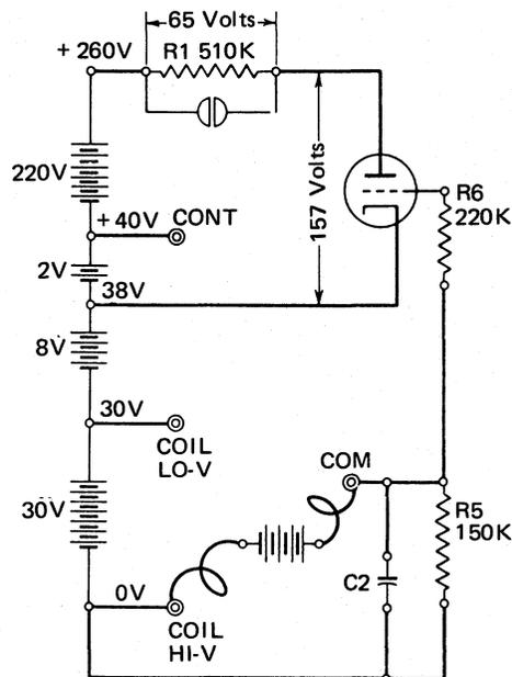
Figure 4-20. Coil High-Voltage Connection Schematic
