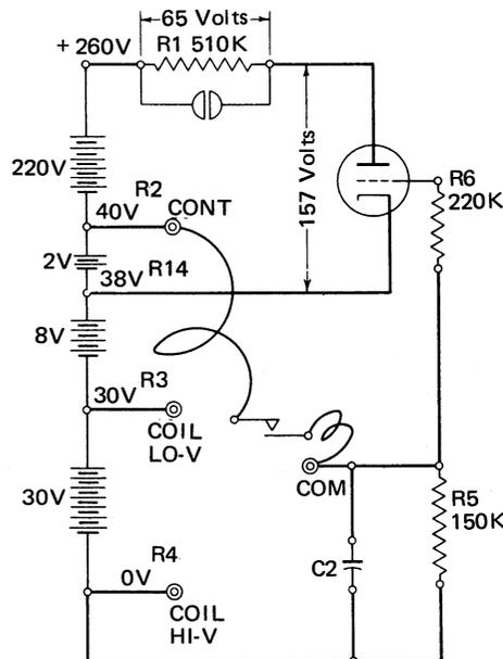
Figure 4-18. Contact Connection Schematic
