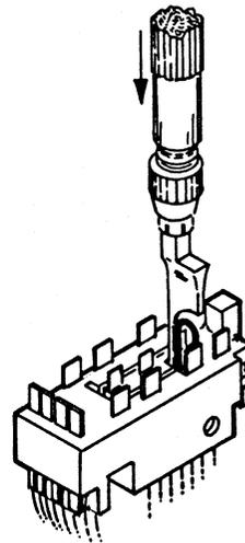
Figure 2-24. Positioning Contact Wire
