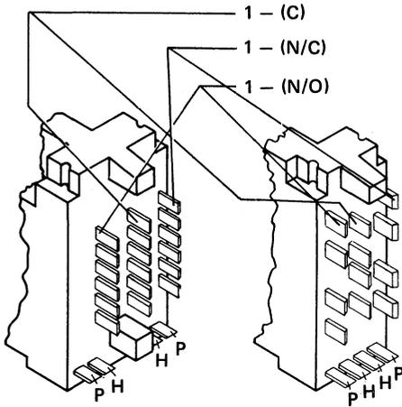
Figure 2-19. PM Relay Moldings
