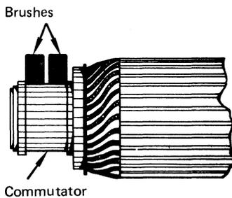
Figure 1-24. Worn Commutator
