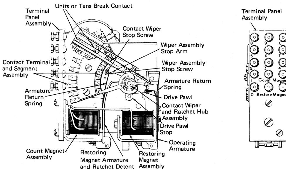
Figure 2-68. Dial Type Relay
