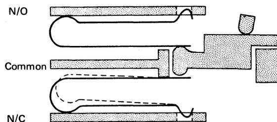
Figure 2-16. PM Relay Contacts Normal
